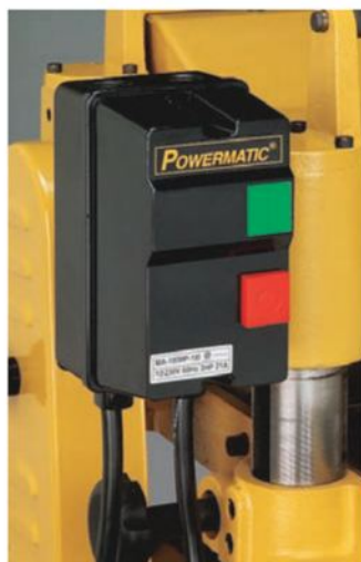
Above: Big planers use three V-belts to transmit power. Right: A magnetic motor starter switches the tool on and off while ensuring better safety.
