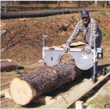
The track and bed of the economical Lumber Smith portable band saw mill are built from wood by the purchaser.
