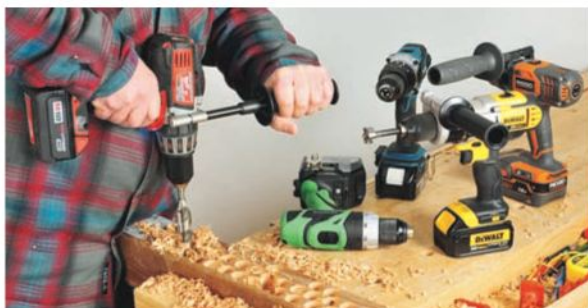
A 1"-dia. self-feeding auger bit pushes a cordless drill to its limits.
