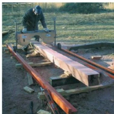
A portable band saw mill transforms fallen trees or salvaged logs into beams and boards for building projects.
