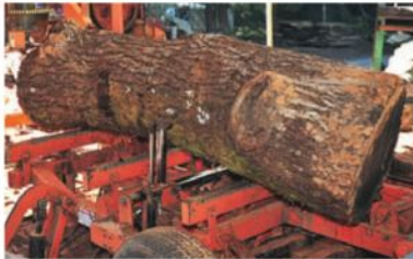
Hydraulically powered devices help position the log on the mill's bed before securing it.
