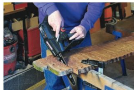
Even a small, 18- to 24-volt, cordless chainsaw can be extremely useful around the workshop for carving tasks, trimming large planks or roughing out large joinery.
