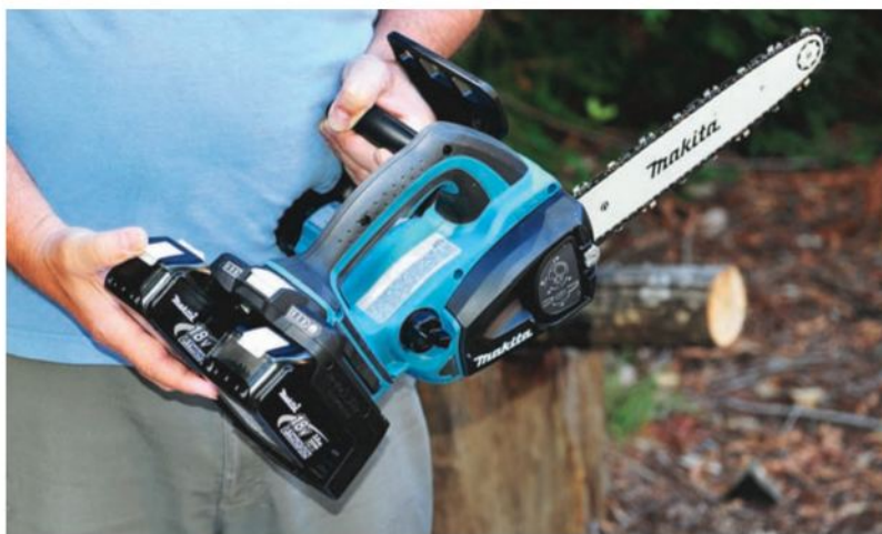
Makita's latest cordless chainsaw will run on either a single 36-volt battery or a pair of 18-volt packs, attached via an adapter plate.
