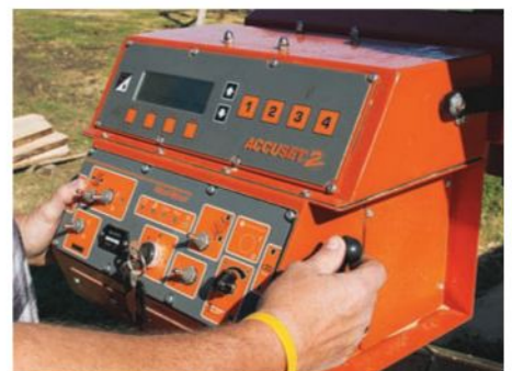
The setwork's controls are used to adjust the saw's depth of cut.
