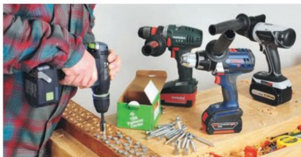
Each drill drove as many 5/16" lag bolts as possible on a single charge.
