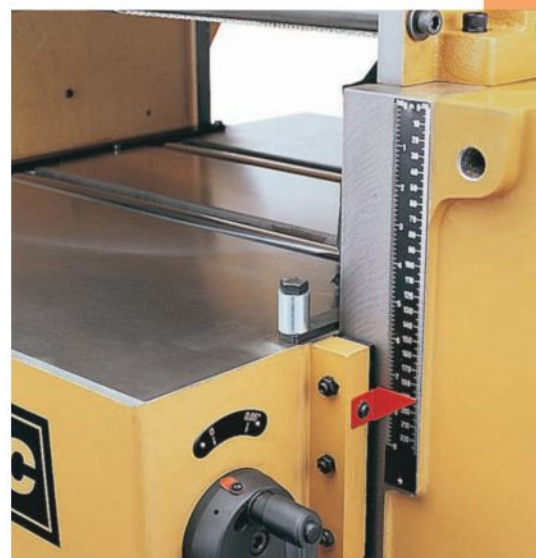
Adjustable bed rollers on this Powermatic planer help rough or resinous boards glide across its stationary bed.
