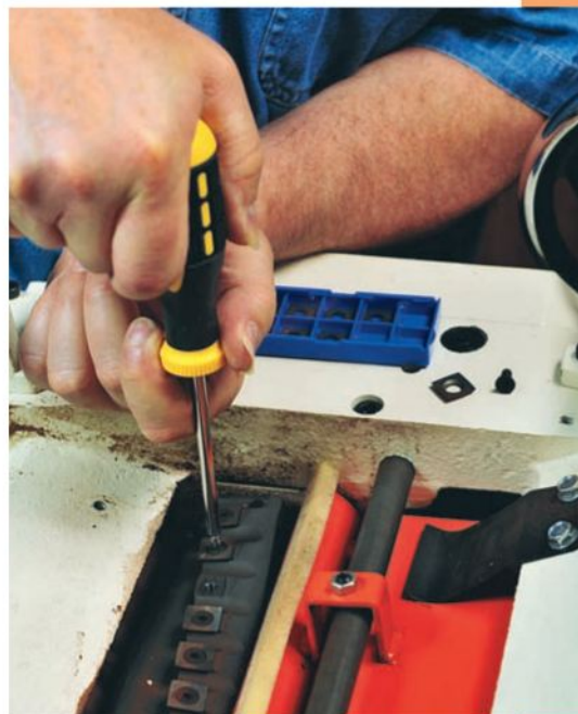
A helical cutterhead's individual carbide inserts can be loosened and rotated to a fresh edge or replaced as necessary.
