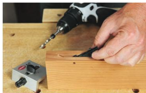
Special Clamex fasteners slide into curved T-slots cut into each half of the parts to be joined.
