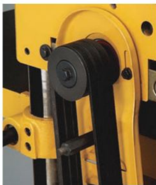
Above: Big planers use three V-belts to transmit power. Right: A magnetic motor starter switches the tool on and off while ensuring better safety.
