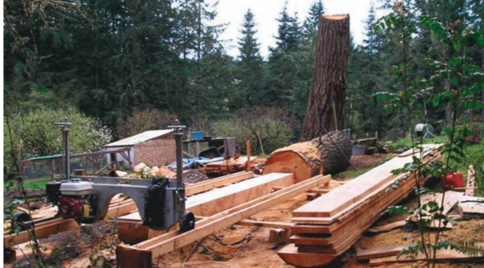
The portability of band saw mills allows trees to be milled where they are cut.
