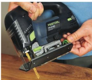
Festool's Carvex jigsaw features (left to right): stroboscopic LEDs that make it easier to see the line of cut; an optional angle-adjustable beveling base; and an innovative circle-cutting jig attachment.
