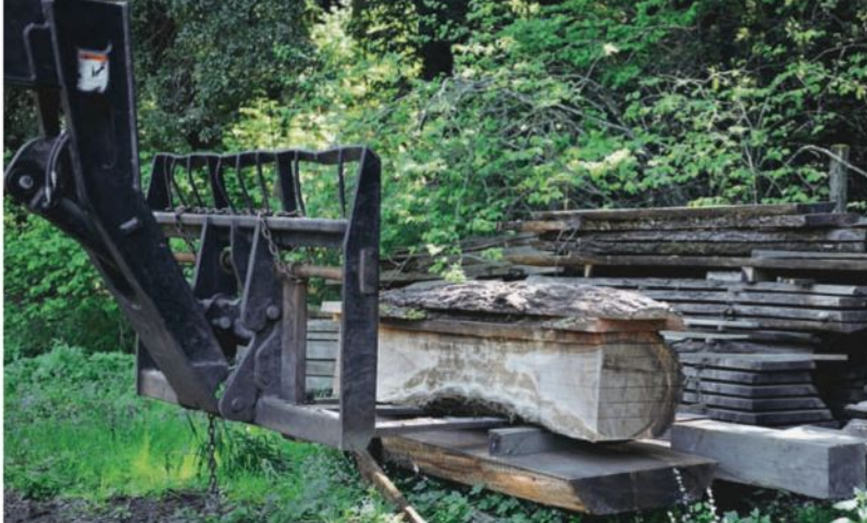
The fully cut log is placed atop a pair of spacers, then the boards are stickered and left to air dry.
