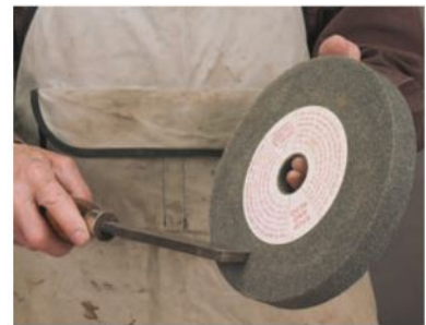
Your grinding wheel needs both sight and sound inspection: a solid wheel should ring if you tap it with a gouge.
