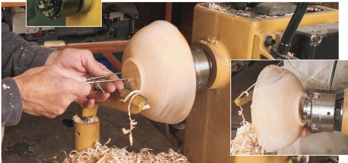
Below, the author prepares a dovetail-shaped mortise for mounting in the NOVA chuck (inset below).
