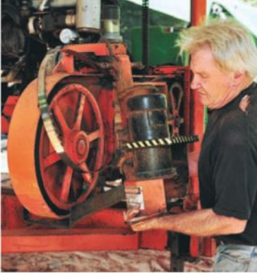
Professional sawyer Chuck Pyle removes the 1¼"-wide blade on his Wood-Mizer band saw mill.
