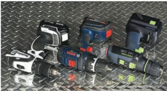
Portable power tools can run on any of three different kinds of motors (left to right): brushed, four-pole or brushless.
