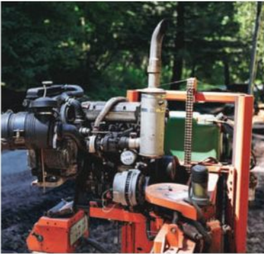
A four-cylinder turbo diesel engine provides plenty of power to cut through even big hardwood logs.
