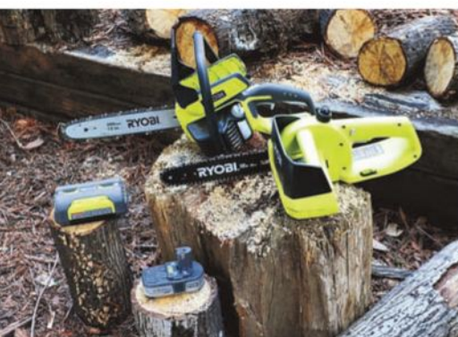
As a rule, the lower a saw's battery voltage, the shorter its bar. The 18-volt Ryobi in front has a 10" bar; the 40-volt model, a 12" bar.
