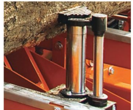
A hydraulic clamp holds a log firmly to the bed.
