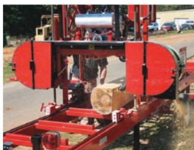
A Mobile Dimension sawmill (above) and portable band saw mill (top) both cut with motorized cutterheads that ride on a track.
