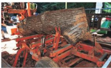
A hydraulic lifter is used to rotate the log 90 degrees in preparation for the second cut.
