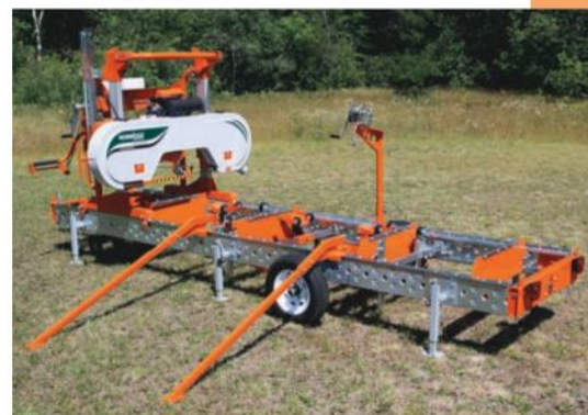
The rigid bed of a band saw mill firmly supports a log or plank as the cutterhead travels along it to take a cut.
