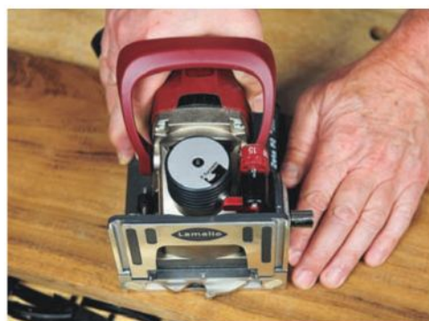
Lamello's Zeta P2 joinery machine cuts curved T-slots for creating strong, glue-less joints.
