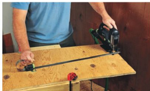
Festool's Carvex jigsaw features (left to right): stroboscopic LEDs that make it easier to see the line of cut; an optional angle-adjustable beveling base; and an innovative circle-cutting jig attachment.
