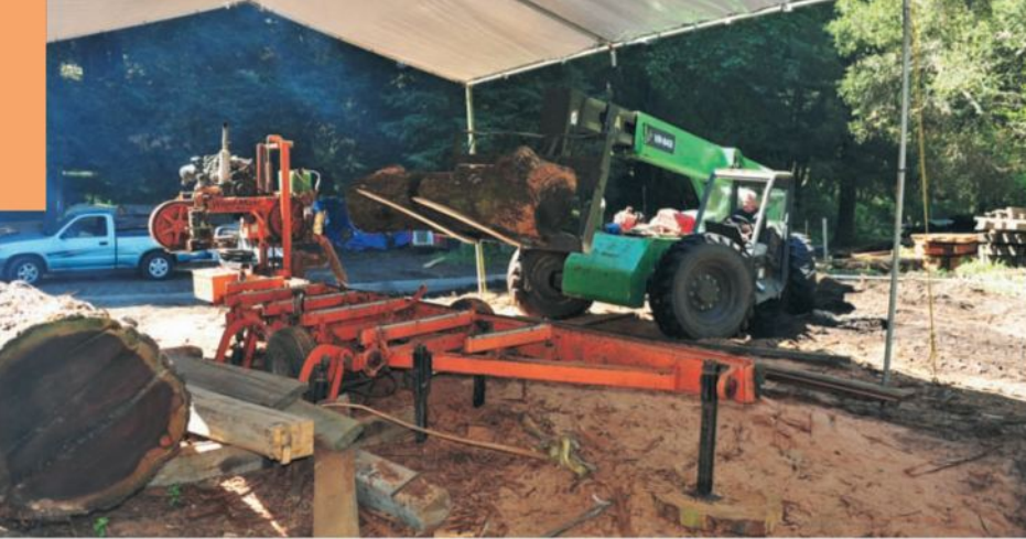
Pyle loads a large walnut log onto the bed of his portable band saw mill, maneuvering it into place with his trusty telescopic forklift.
