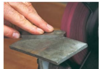
Rests should be no more than 1/8" from the grinding wheel. Rest adjustment is made with the grinder stopped.
