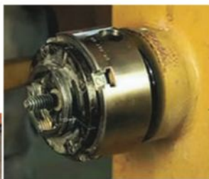
A screw in a Oneway chuck (left) turns it into a heavy-duty screw chuck for roughing bowls.
