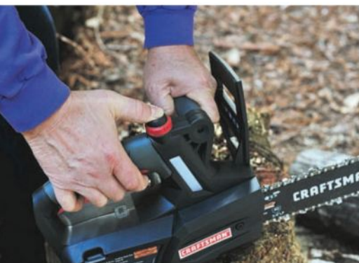
On cordless chainsaws lacking an automatic oiler, the bar must be regularly lubricated by pressing a button that forces oil onto the chain.
