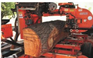
With two flat, square sides cut, the remainder of the log is sawn into accurately dimensioned planks.
