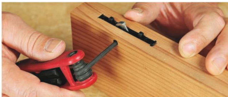
Once Lamello's Zeta P2 joinery machine has created the slots for interlocking Clamex P connectors, an Allen wrench is used to lock together the two halves of each Clamex fastener.
