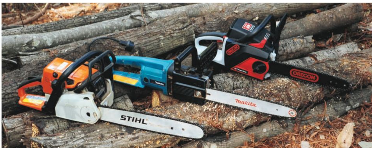
The three types of chainsaws: a gas-powered saw (the STIHL), a corded electric saw (the Makita) and a cordless saw (the OREGON).
