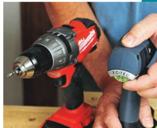
Instead of a traditional mechanical clutch (left), Festool's T18+3 cordless drill uses electronics to monitor and limit torque output, set via a 25-position dial.
