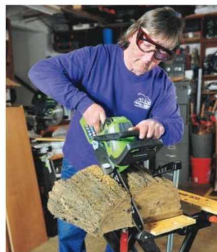
Larger cordless chainsaws with 36- to 40-volt batteries and 12"- or 14"-long bars are great for cutting logs and burls into turning blanks.
