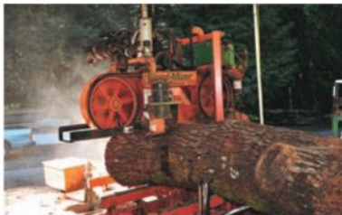
The mill's cutterhead carriage travels the length of the bed as the band saw takes the first cut.
