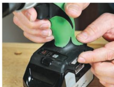
A small button at the base of Hitachi's DS 18DBL brushless-motored cordless drill sets the tool's power output to suit the task.
