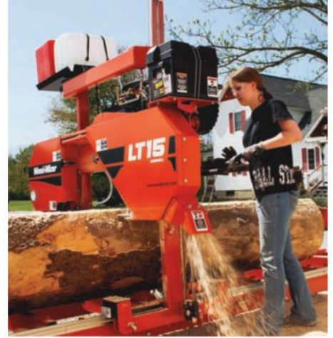
Often referred to as "walkers" or "pushers," manual portable band saw mills have a cutterhead that must be pushed along its bed/track for cutting. This allows the user to adjust the feed speed as necessary.
