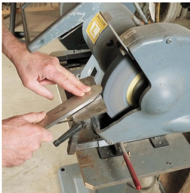
Grinding is the easiest way to raise a burr. With a grinding rest set at 15° to 25°, start moving the scraper edge as soon as it touches the wheel.
