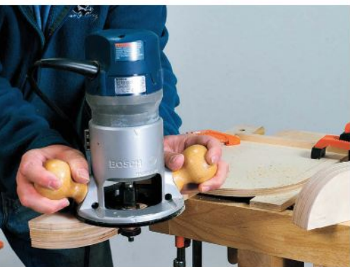
A router fitted with a flush-trim bit trims the leg's feet to final shape. The bit's guide bearing rides on the already cut and sanded longer foot piece.
