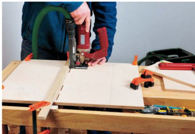
All of the parts are joined with #10 plate joinery biscuits. A straight wood strip clamped across both of the desk's sides acts as a fence to accurately position the biscuit joiner and assure that mating parts will align properly.
