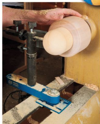
When half the ball is finished, rotate it in the jam chuck and adjust equator position. Spindle turn away as much wood as possible and reposition the sphere tool to turn the second half.
