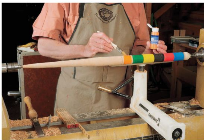
The easiest way to paint the starting stake is in the lathe with it going very slow. The author used acrylic paint from an art store.
