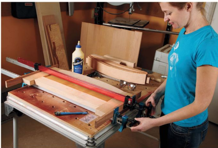
Pre-finish the panels and the inside edges of the rails and legs before gluing and clamping them into two end frames. Scraps under the clamp heads prevent them from marring the soft fir lumber.
