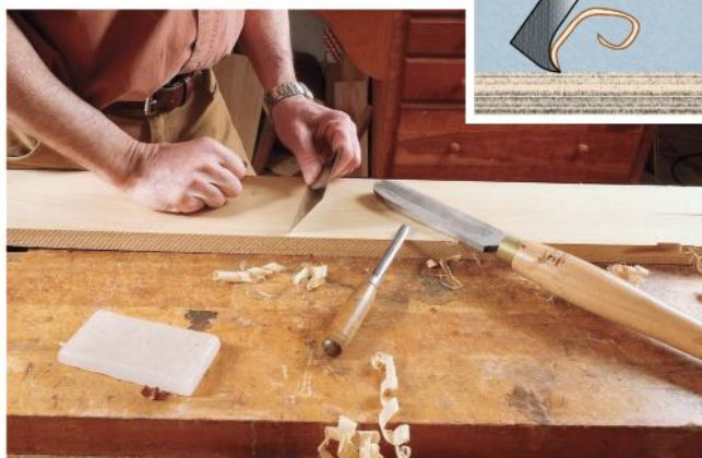
A turning scraper, just like a cabinet scraper (in photo and drawing), has a burred edge that limits the depth of cut to 1/1,000ths of an inch.
