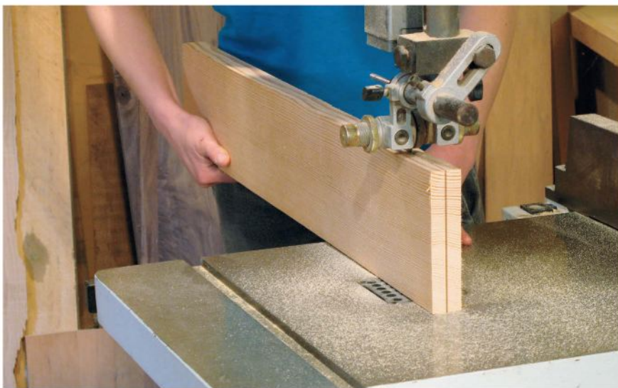
Our author was able to achieve excellent grain match for the bed's solid wood panels by first resawing thicker Douglas fir into thinner, book-matched slats. It's easy to do on the band saw.
