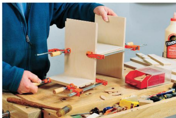
The hobby desk's upper dividers, shelves and cubbies are first glued together as a subassembly. Biscuits help keep all the parts correctly aligned.
