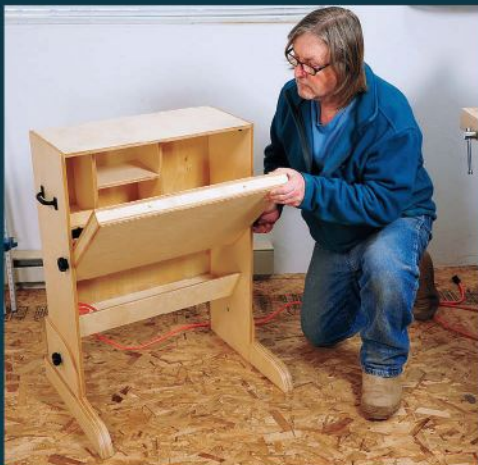
Built with torsion box construction, the desk's fold-down top pivots on a pair of hanger bolts. It flips up to conceal the interior and lower shelf/cubby.
