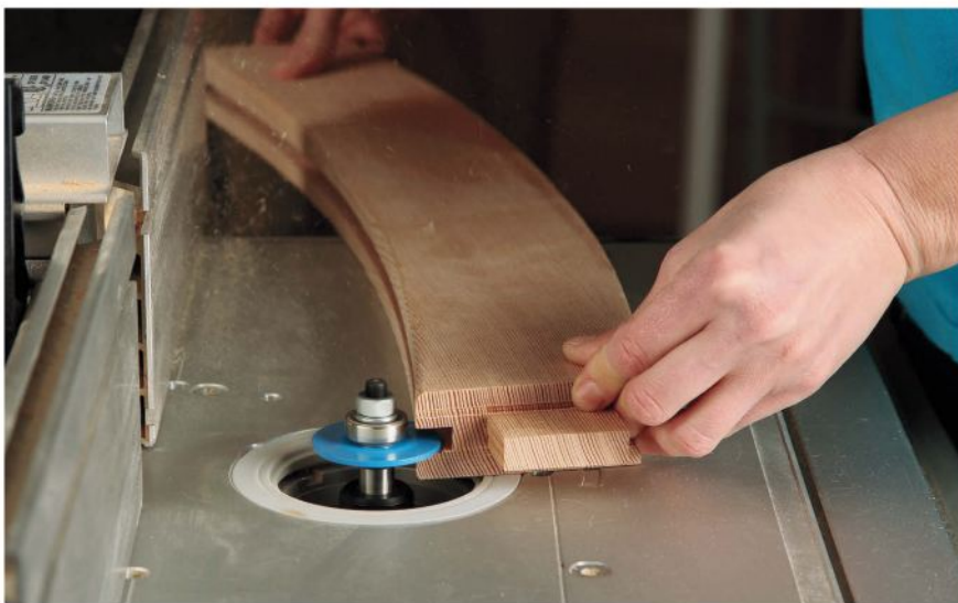
Several passes with a piloted slot cutter formed grooves on both the curved and straight rails, as well as the legs. These grooves house glued-up panels in the end frames.
