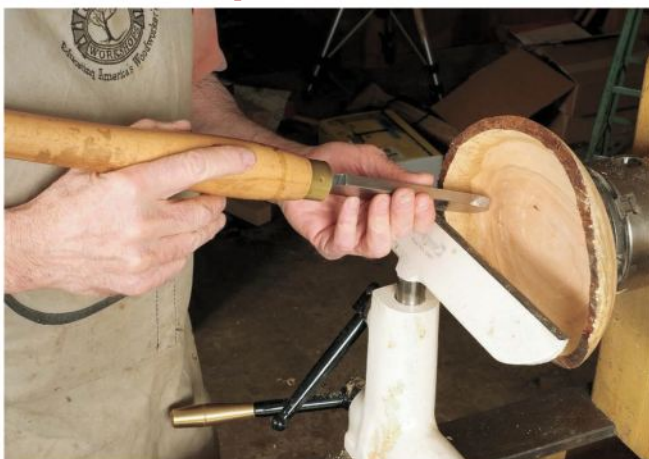
A large dome scraper is excellent for all faceplate work, but especially bowls. The author uses the large size shown here the most, but also finds its smaller brother to be useful. It is often more effective to tilt the scraper on the sidewall of a bowl, as seen in this photo.
