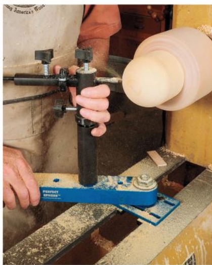
Remove the rest of the material by swinging the arm of the tool 90°. Make light cuts, removing a few thousandths at a time. The tool works better if you swing from the center to the equator.
