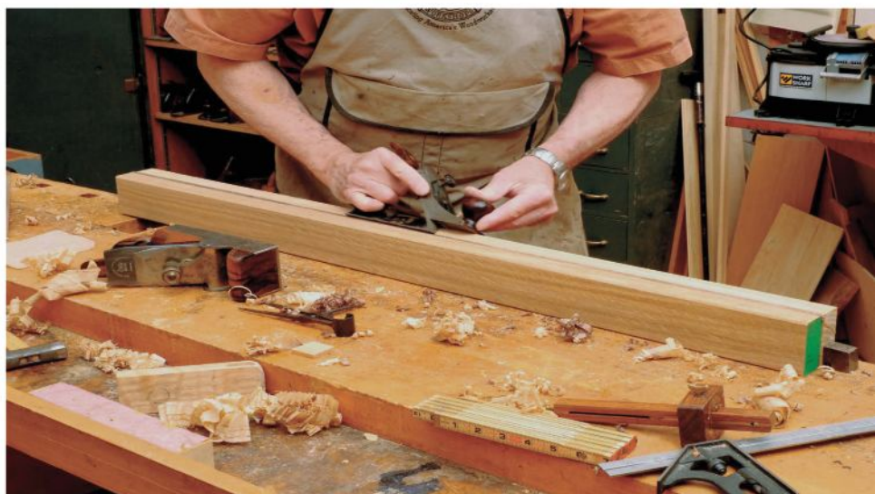
To make a 2 \frac{5}{8} "-high by 2 \frac{3}{8} "-wide rectangular mallet head, the author bought \frac{3}{4} " wood and glued it up. With his glue line centered on the 2 \frac{3}{8} " dimension, he surface planed the blank to final dimension, then milled a groove centered on the glue line for a contrasting sight line inlay. He finished up the mallet head by crosscutting to length and then drilling a hole for the shaft.
