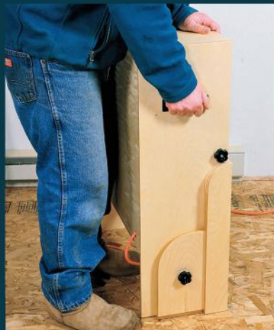
After you've loosened the hand screws far enough for clearance, the desk's legs pivot up for easy transport and compact storage.
