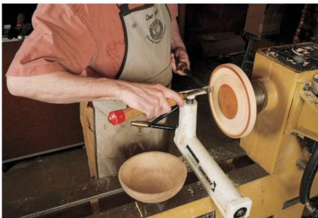
Diamond scrapers are useful for much more than incising lines: their real purpose is for exact fits. Here, the author is using one to fit a jam chuck for a bowl with the aid of an armrest, which eliminates the need to move the tool-rest all the time to check fit.
