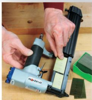
A long magazine on Spotnails' "The Striker" gun will hold two full clips for extended nailing jobs.
