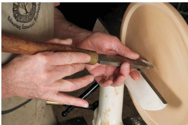
The author has designed his straight edge scraper — used for making things flat — into what he calls a boat-tailed scraper. It has a rounded left corner so as to be able to cut to the left and a beveled right corner, which looks like the back of a boat when viewed from the top.
