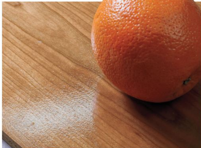
A pebbly surface on your project, with the texture of an orange peel, is the result of finish droplets that are too large or too thick to dry properly.
