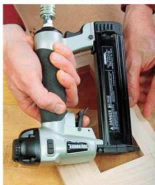
Without a second safety trigger, Surebonder's grip offers more room for a natural, three-finger grasp.
