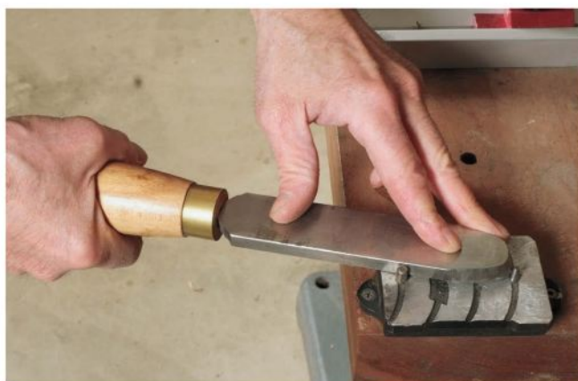
The tungsten carbide cone in the Veritas Scraper Burnisher is sufficiently hard, and its fulcrum point provides sufficient force, to roll a burr in HSS.
