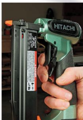
Hitachi's two-trigger system makes firing the pinner a conscious, two-step operation.
