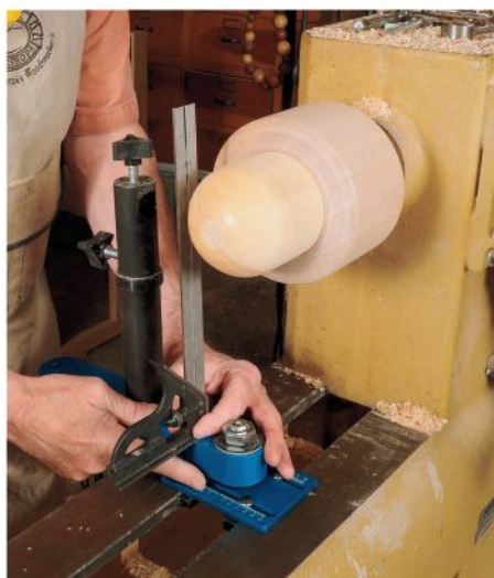
Set up the Carter Products Perfect Sphere Tool base plate exactly under the equator. If this is not positioned exactly, your ball will be too short or too long between the poles.
