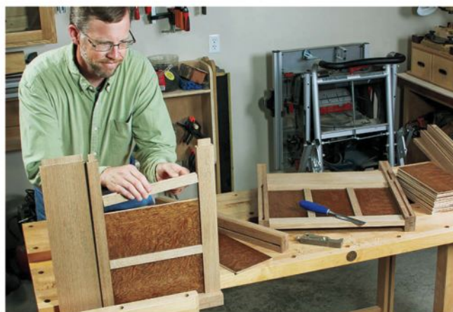
To glue or not to glue? For this project, seasonal expansion is not a factor — but it does make a difference in alignment during assembly.
