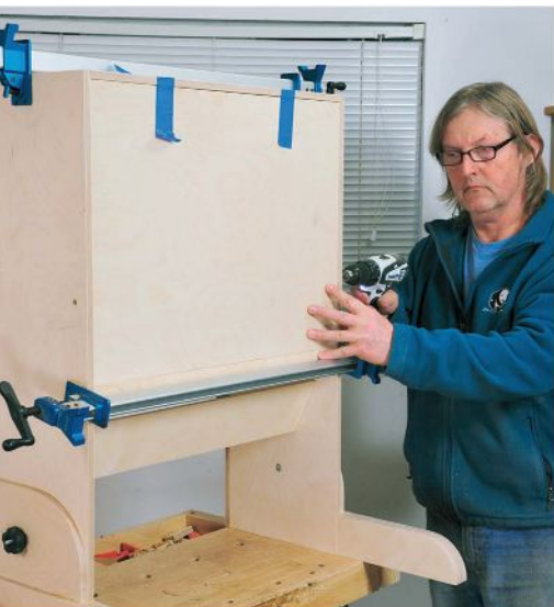
With the hobby desk's top temporarily clamped in place, the author drills a pilot hole for the 5/16" hanger bolt that it will pivot on.
