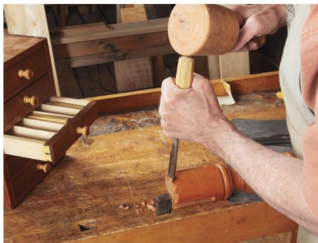
To complete the carving, use the 8-sweep gouge to carve arches between each of your three Vs and the dovetail slots (a total of 3 Vs and 6 arches).
