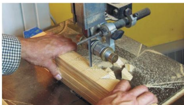
The back slats were secured to the carcass by a single screw at each end of the slats. The author chose to gang-cut the notches into the shelf stiles on his band saw (below). The primary advantage to that technique was to save time both on marking out the shelf stiles and in cutting all the notches.
