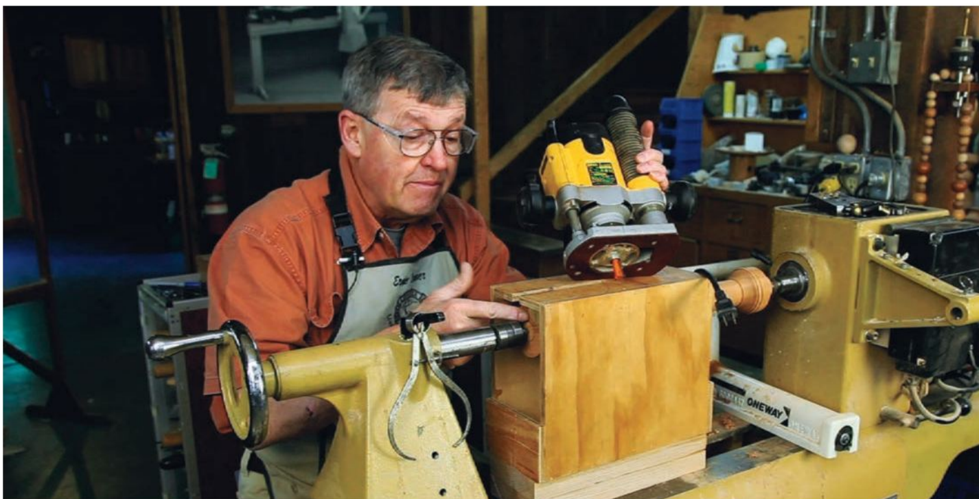
The author prepares to use a simple box-like jig keyed to the lathe bed. This allows milling of dovetail-shaped slots to attach legs to the base of the stem.
