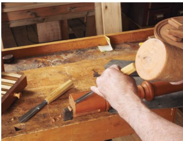
On the leg end of the stem, at exactly the center point between two dovetail slots, carve a V with a veining chisel and carver's mallet.
