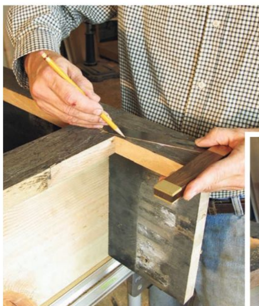
The author used a sliding bevel gauge to trace the angle of the legs (above left). He cut the shape of the legs into the cabinet with a handheld jigsaw (inset, right).
