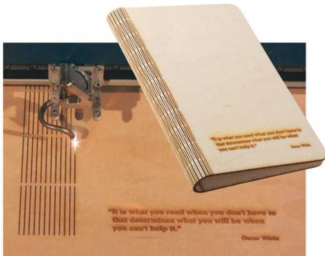
A powerful computer-controlled laser machine can cut out and engrave even the most intricate wooden parts with great precision.
