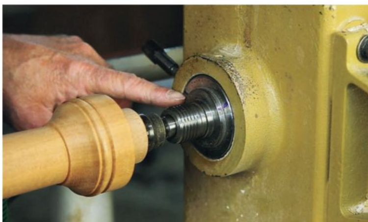
If your lathe has indexing, there will be 12, 24 or 60 positions. All are divisible by 3, allowing 120° between slots. Marking the spindle with a marker greatly simplifies indexing during the anxious moments of routing.
