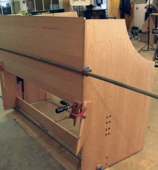
The author had some extra-long clamps that came in very handy while assembling the case section of the desk/bed.
