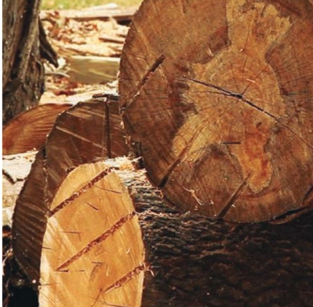
End Grain Checking: Because a log or a board loses water faster from the end grain than from the face, or plank, it's normal to see grain checking at the exposed ends. The checking must be cut away.
