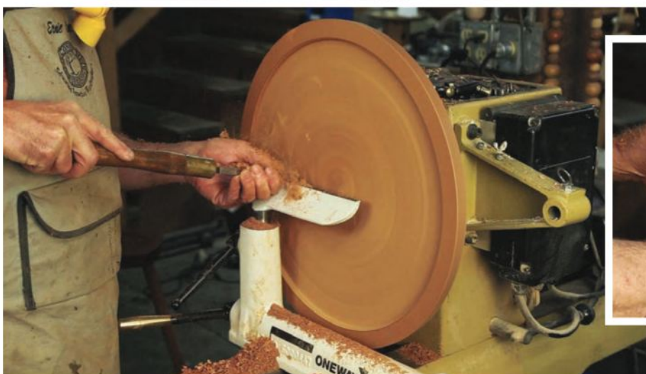
Use the Boat Tailed Scraper downhill and use the tool-rest to guide your left hand to obtain a flat surface on the table's face.
