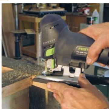
The author used a sliding bevel gauge to trace the angle of the legs (above left). He cut the shape of the legs into the cabinet with a handheld jigsaw (inset, right).
