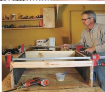
Rabbets on the top of the sides are cut to accept the stretchers (top photo). They are routed to the same depth as the bottom's dadoes. A section of the 3/4" pine is used to test the rabbet's accuracy. This cabinet was assembled with standard blue-collar joinery (inset photo) — plain old yellow glue, finish nails and clamps.
