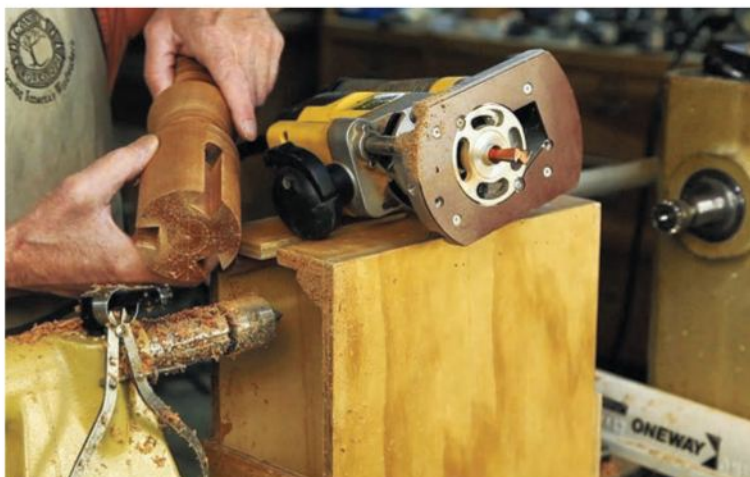
When the dovetailed slots are completed on the lathe, the next step will be to square up the ends of each slot using a sharp chisel.
