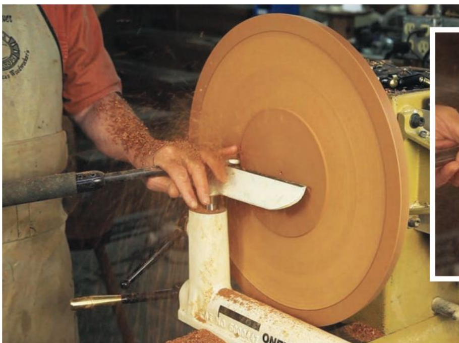
A bowl gouge is used to excavate the 1"-thick top to a depth of about 1/2". The 1"-wide band at the perimeter is left at its original 1" thickness to lend strength to the top and a decorative accent (photos above).
