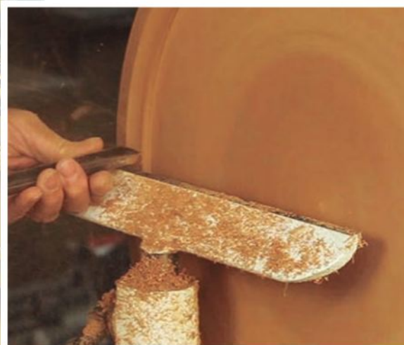
A bowl gouge is used to excavate the 1"-thick top to a depth of about 1/2". The 1"-wide band at the perimeter is left at its original 1" thickness to lend strength to the top and a decorative accent (photos above).
