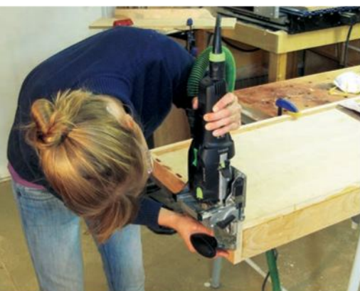
While the author used Dominos for her construction, biscuits would work, too. Use the best solution you have at hand.
