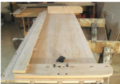
The tri-bearer needs to be mounted before the desk components are assembled. Part of the hardware will be captured by the wood.
