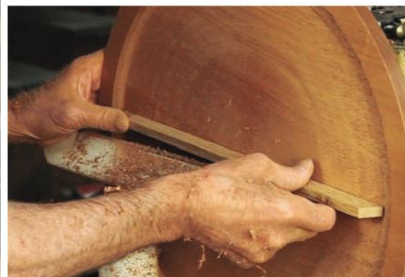
Use the Boat Tailed Scraper downhill and use the tool-rest to guide your left hand to obtain a flat surface on the table's face.
