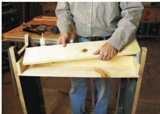
The components of the "brick shelf" are attached under the bottom at the rear of the cabinet (photo above). The shelf allows weight to be added that will counterbalance the weight of the door and the force of momentum created when the door is opened — it keeps the cabinet from tipping (photo bottom right, opposite page).
