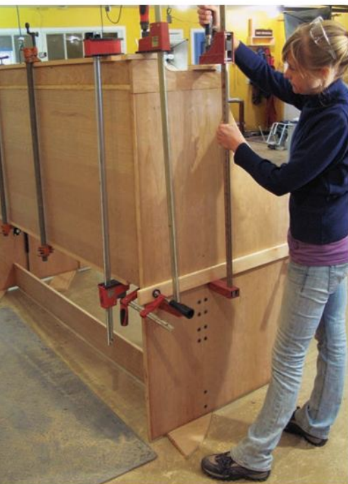
With scrap wood pieces securely clamped to both faces of the case sides, the author uses them to clamp down the top subassembly.
