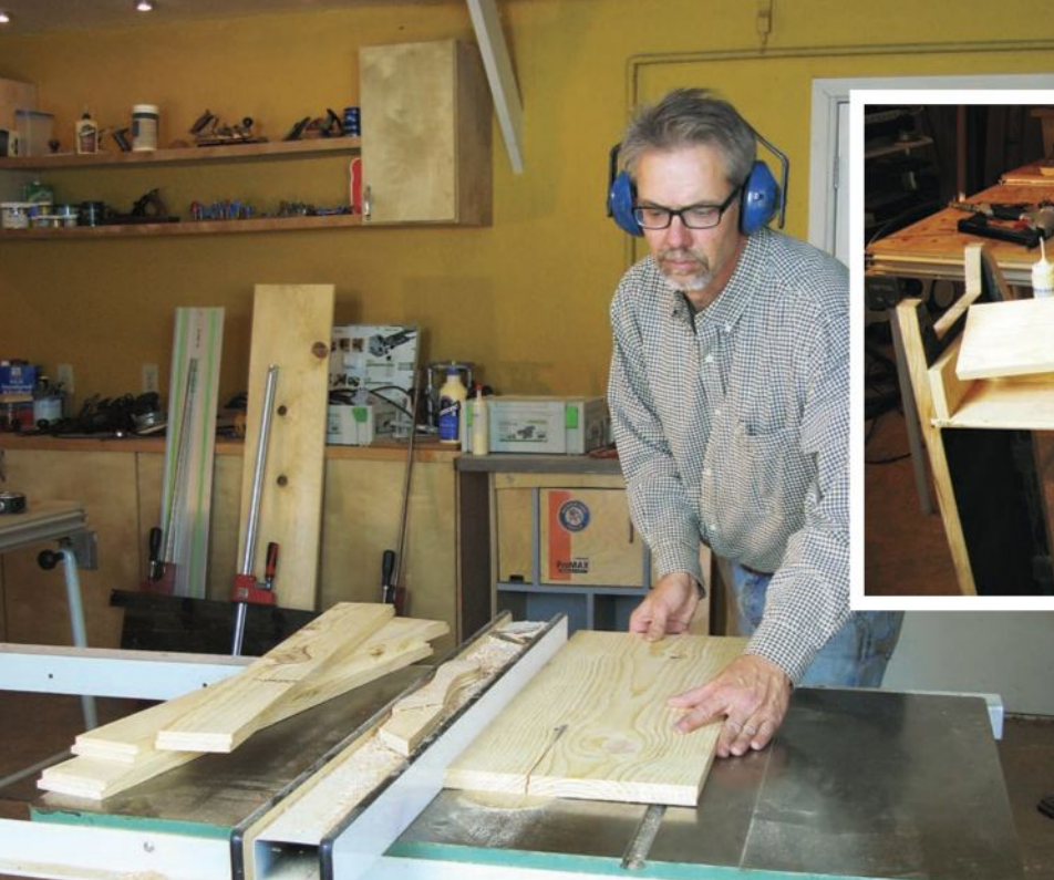
Ripping the back slats and other pine components from 1 x 12" stock gave the author more options. Wider lumber provides you with the opportunity to select the best-looking sections of the board for each component.
