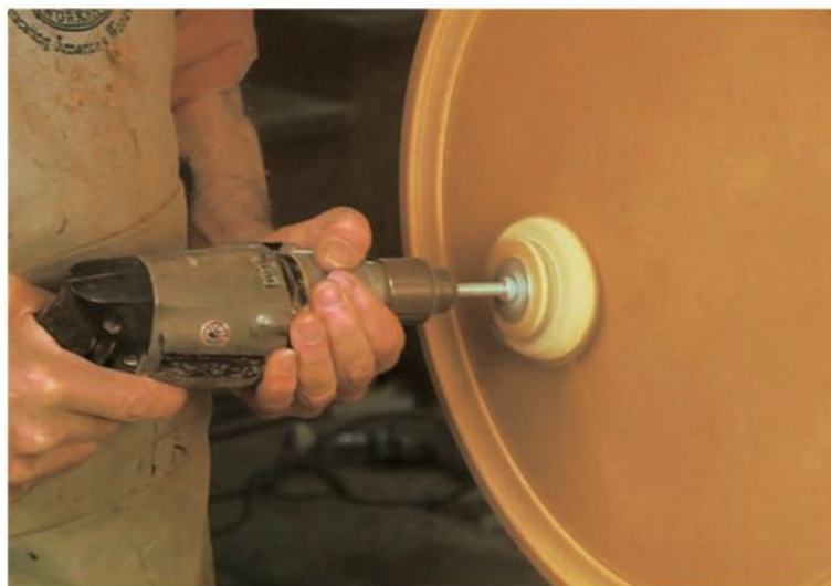
Flatness and smoothness are best obtained with a sanding pad mounted in an electric drill. Start with 60- or 80-grit paper and work up to 180. An orbital sander is a good last step after you've demounted the blank.
