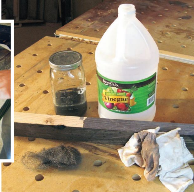
A light sanding with 100-grit paper on a rotary sander brought out highlights of the oak hidden by the ultra-dark patina (above). Soaking steel wool in white vinegar creates a solution that will darken oak by reacting with tannin in the wood fibers. The results on these pieces matched the exposed oak edges to the recycled lumber.
