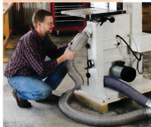
Band saws produce copious fine dust. Double 4" dust ports on RIKON's 10-370 effectively manage it.
