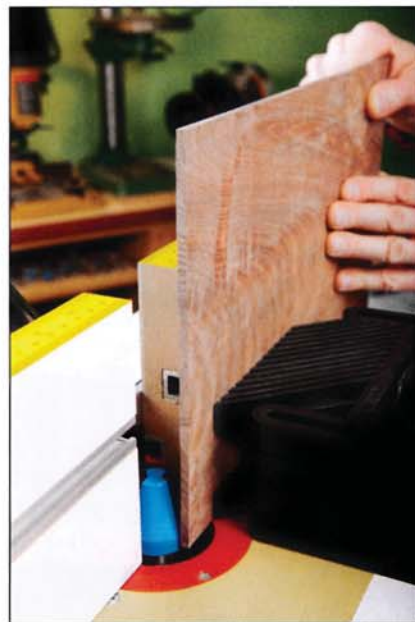
Freud adds precision to edge jointing operations, thanks to two micro-adjust controls on the fence's infeed and outfeed facings (top). MLCS's tall fence offers ample support for vertical panel-raising (bottom).
