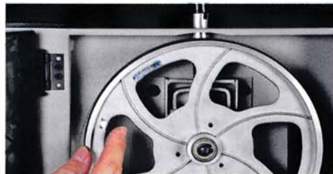
The 9" Craftsman BAS230 has a couple of features that distinguish it from its rivals, including balanced wheels (left) and a ribbed cast-alloy table (right).
