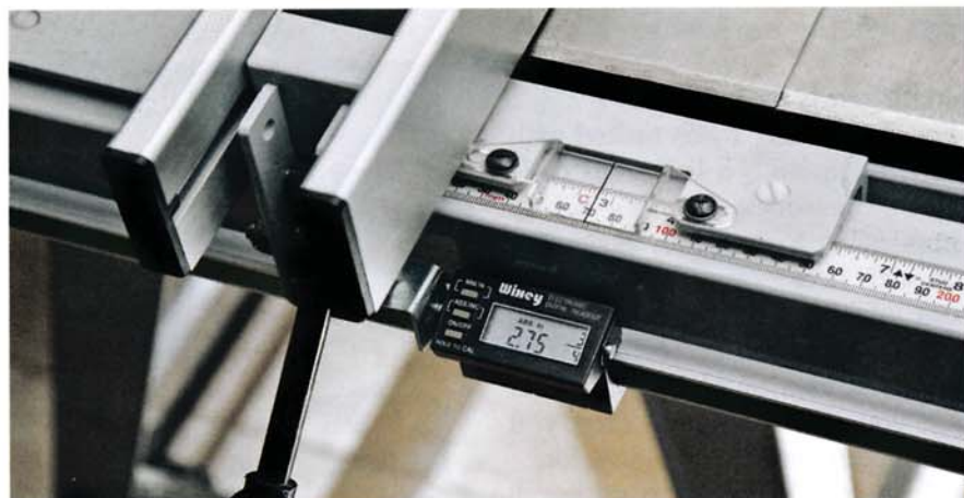
Add a digital readout to your rip fence for accurate settings to within hundredths of an inch.
