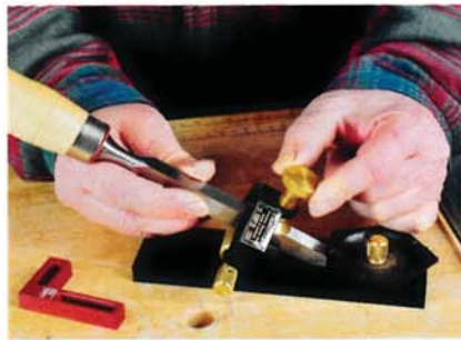
A knurled wheel on the Veritas Precision honing guide (left) resets its eccentric roller to a higher angle for honing a secondary bevel. An angle-setting jig (right) that comes with the Veritas guide is used to set the blade at 15, 20, 25, 30 or 35 degrees.
