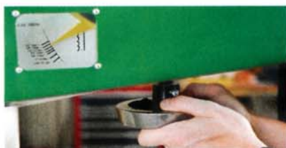
Variable-speed (top) enables the 10-370 to cut metal and wood. Large hand wheels (bottom) ease setup tasks.
