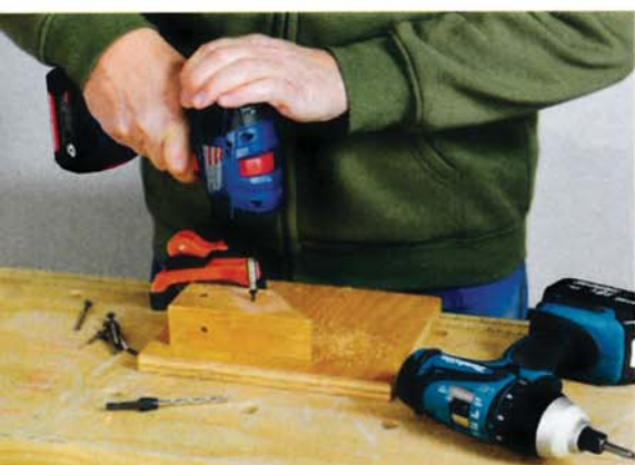
Hybrid drill/drivers that combine both a drilling function and an impact driver function are one of the recent innovations offering more options to woodworkers.
