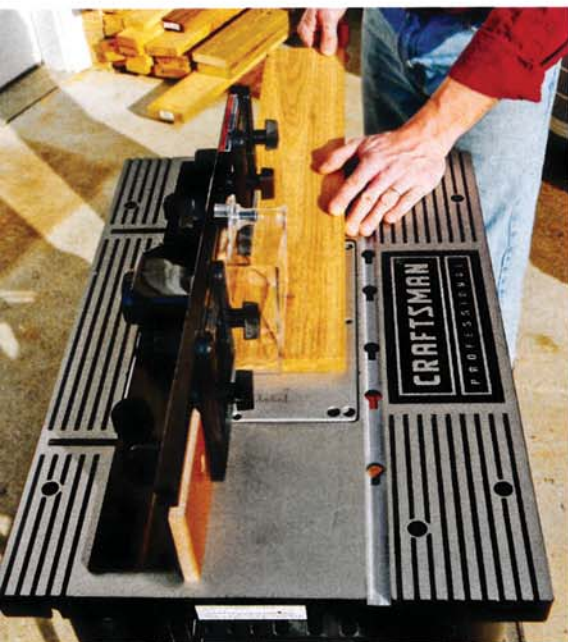
Kreg equips its table with Allen screws for insert plate leveling (top). Craftsman's aluminum table (bottom) is impervious to moisture, for routing indoors and out.
