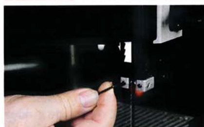
The steel pin friction side guides on the Skil 3386 (top) are slightly larger in diameter than the identical pins found on the Craftsman, Ryobi or Central Machinery (bottom).
