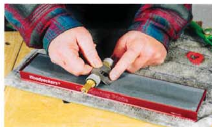
The Kell #2 honing guide's side-gripping design allows it to hold even short chisels and plane irons very solidly.
