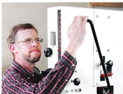
An included resaw bar (top) and blade quick release (bottom) are two of JET's useful features.
