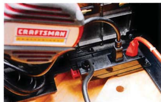
Craftsman's Professional Router Table (model 61181) comes with an On/Off switch that powers two receptacles — one for the router and the other for a shop vac.
