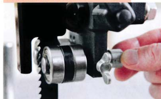
The author appreciated the precision and ease of JET's eccentric blade guide adjusters.
