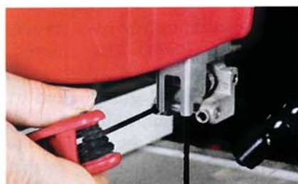
Two features the Ryobi BS903 shares with similar-looking 9" models are its blade tension release lever (left) and plastic and aluminum miter gauge (right).
