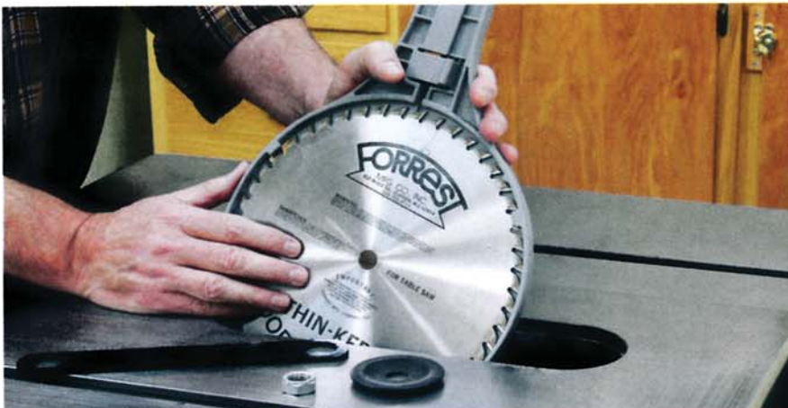
The Saw-Jaw rigidly holds blades for easy changing while protecting you from sharp edges and the teeth from possible damage.
