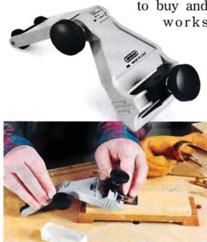
The knob in the center of the General 809 honing guide is used to set the blade to the desired honing angle.
