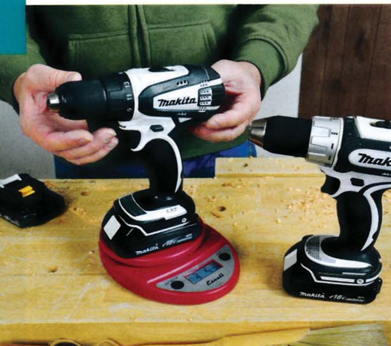
Makita's LXFD01, featuring a four-pole motor, also employs a new drive train with larger front-end ball bearings and a redesigned planetary gear system and transmission.
