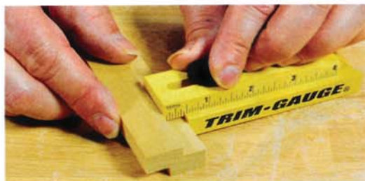
Scribing irregular shapes is made easier with M-Power's Perfect Butt stylus and wheel system (top). Measuring joint heights and offsets is the bailiwick of Brumley's Trim Gauge (bottom).
