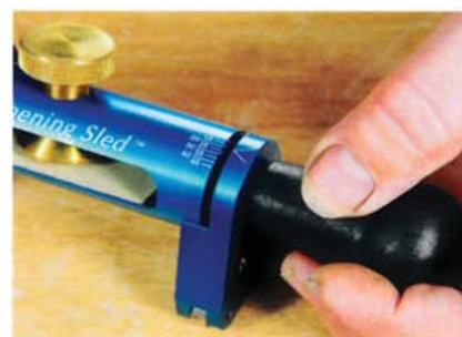
Spring-loaded front wheels on the Alisam (left) let you press the tool down during honing. A series of tiny detents (right) set the exact honing angle. Tightening the side handle locks the setting in place.
