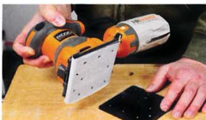
RIDGID's paper punch creates many small holes, allowing for very good dust collection.
