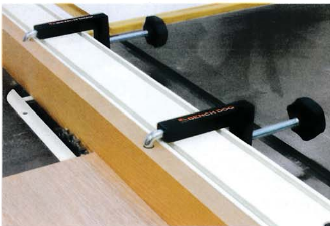
Sacrificial fences can be installed easily, quickly and unobtrusively, using a pair of specialty clamps that wrap over the fence beam.
