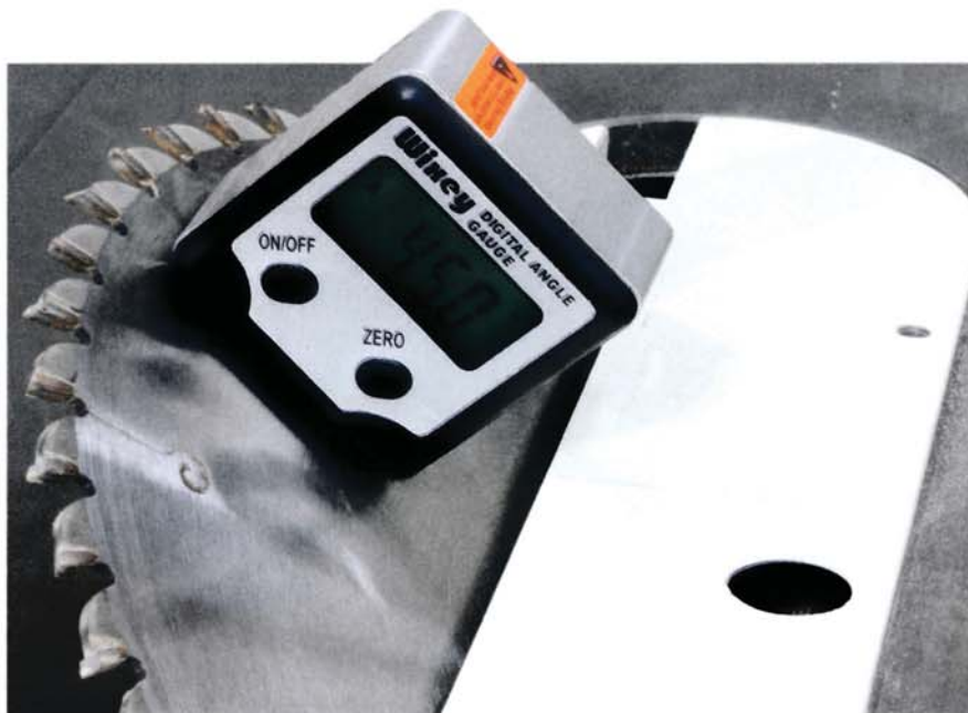
Set blade tilts off of a digital angle gauge, then find a multitude of other machine tool uses for this device.
