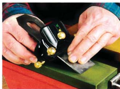
The Veritas MkII guide (left) has a good heft and rolls very smoothly atop any kind of whetstone or honing plate. The registration jig (right) that comes with the MkII can be set to a multitude of honing angles to suit multiple sharpening chores.
