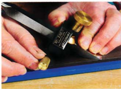
A knurled wheel on the Veritas Precision honing guide (left) resets its eccentric roller to a higher angle for honing a secondary bevel. An angle-setting jig (right) that comes with the Veritas guide is used to set the blade at 15, 20, 25, 30 or 35 degrees.
