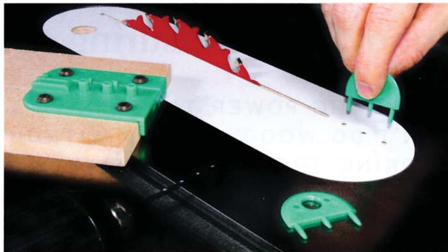
Aftermarket splitters added to zero-clearance inserts help prevent kickback accidents. The MJ Splitter from Micro Jig shown here includes two splitters that can be reversed or swapped for fine-tuning.
