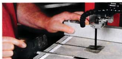
The 9" Skil 3386's miter gauge features a bar with a T-shaped profile, to keep it from lifting in the slot.
