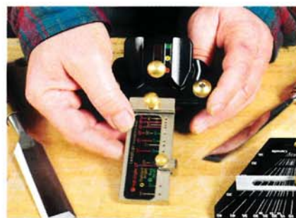
The Veritas MkII guide (left) has a good heft and rolls very smoothly atop any kind of whetstone or honing plate. The registration jig (right) that comes with the MkII can be set to a multitude of honing angles to suit multiple sharpening chores.
