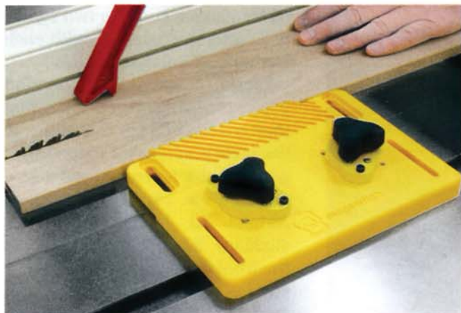
A featherboard acts like a third hand and keeps yours out of harm's way. Magnetic versions like this can be easily positioned wherever needed.
