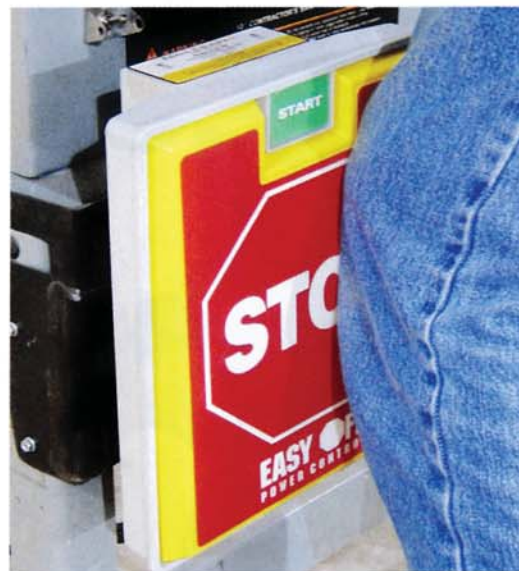
Large replacement power switches let you turn the saw off quickly by bumping the switch with your knee.
