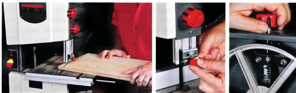
The 10" JET JWBS-100S has several unique features, including (photos from left to right) a pull-out stock support, upper blade guides that adjust tool-less, and a blade tension gauge that shows the correct amount of tension for any blade that the saw accepts.
