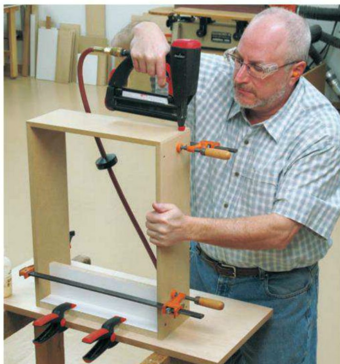
Photo 6: Glue and nail the drawers together. I made a 14 1/16"-long L-shaped support from white melamine to hold the drawer front and back (pieces 8) upright and square as I attached the first drawer side (piece 9).
