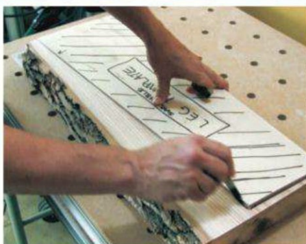
To get identical leg sizes and shapes (above, left), the author used a template to mark them out.
