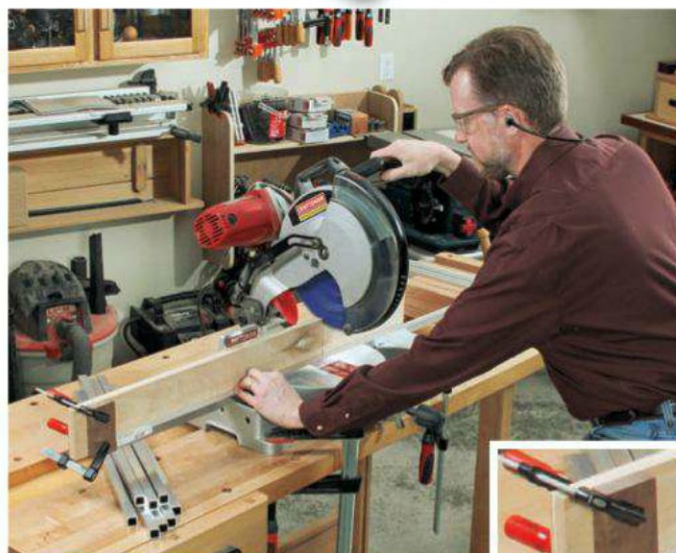
A miter saw with a fine-tooth, carbide-tipped woodworking blade makes easy work of cutting the aluminum tubing to size. Use a stop block (see inset) clamped to a long fence to ensure consistent lengths for the tray and cart top tubing.
