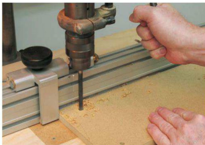
Photo 4: Drill the 5/16"-dia. holes in the drawer fronts (pieces 8) for the screws used to attach the drawer faces (pieces 7).
