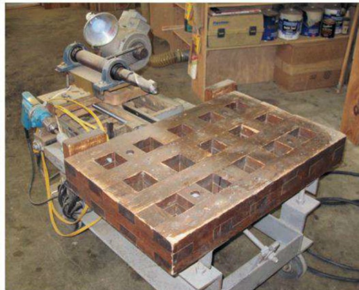
Steve Timm stands at an Italian band saw (above), useful for cutting architectural components like the large corbel at left. The saw moves on an articulated arm as the wood remains stationary. Timm's shop-made mortising machine (below) is used to assist in post and beam construction.
