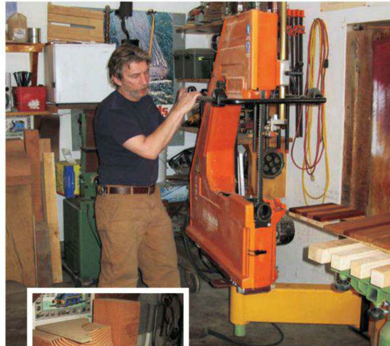
Steve Timm stands at an Italian band saw (above), useful for cutting architectural components like the large corbel at left. The saw moves on an articulated arm as the wood remains stationary. Timm's shop-made mortising machine (below) is used to assist in post and beam construction.
