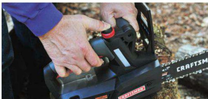
On cordless chainsaws lacking an automatic oiler, the bar must be regularly lubricated by pressing a button that forces oil onto the chain.
