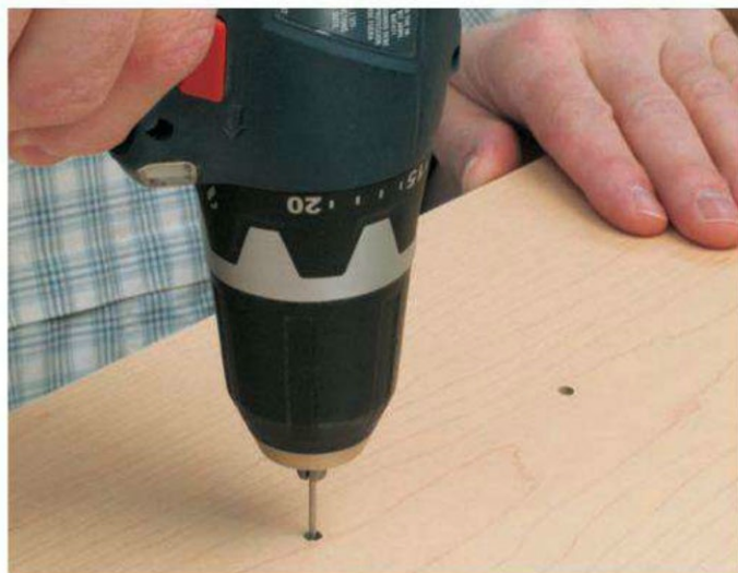
Photo 12: Drill 3/32 "-diameter holes through the pull holes in the drawer faces and through the drawer fronts to locate the pull bolt holes on the insides of the drawer fronts.
