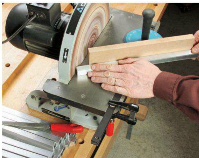
A benchtop disk sander and clamped miter gauge are a good combination for easing the sharp edges and corners of the tubing pieces. Once they're beveled, round over and smooth the ends further with a file.
