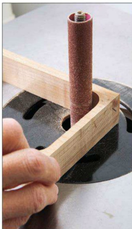
Smooth the inside edges of the box and remove all evidence of sawing with a small-diameter sanding drum.
