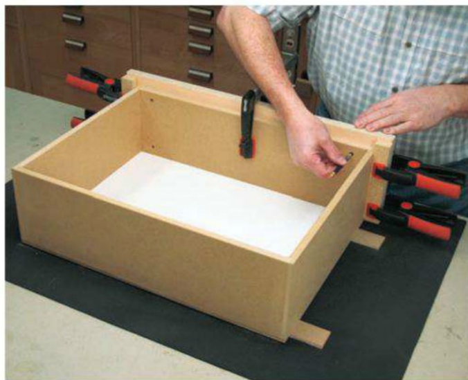
Photo 9: Mark the pilot hole locations for attaching the drawer faces to the drawer boxes. Use 1/8"-wide spacers to center the drawer face side to side, and 1/4" "lifts" to align the height.
