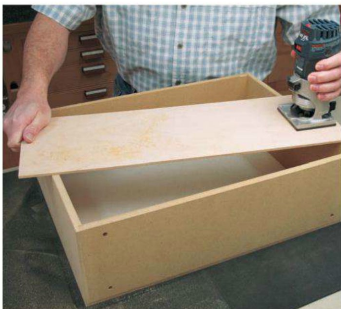
Photo 7: Rout the 1/8"-radius roundover top edges on the assembled drawers. Don't rout the front edges. I screwed a long auxiliary base to the palm router for added support and control.
