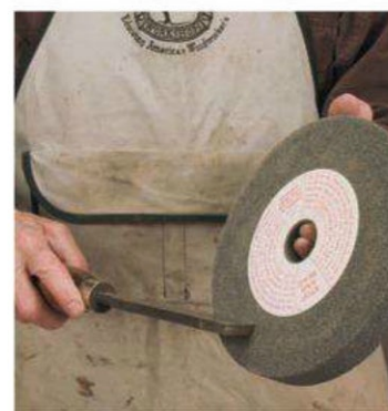
Your grinding wheel needs both sight and sound inspection: a solid wheel should ring if you tap it with a gouge.
