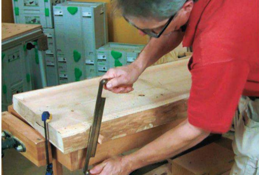
The first step in making this table was to take the bark off the waney edges with a drawknife, as shown above.
