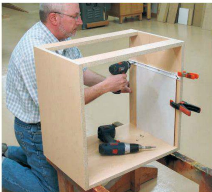
Photo 10: I used spacers to position and mount the drawer slides. Work from the top down, starting at 14\frac{15}{16} " up from the carcass bottom, then 7\frac{1}{4} ", and finally 1\frac{1}{4} ".
