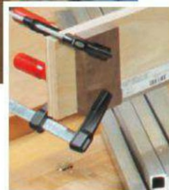
A miter saw with a fine-tooth, carbide-tipped woodworking blade makes easy work of cutting the aluminum tubing to size. Use a stop block (see inset) clamped to a long fence to ensure consistent lengths for the tray and cart top tubing.
