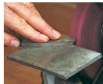
Rests should be no more than 1/8" from the grinding wheel. Rest adjustment is made with the grinder stopped.
