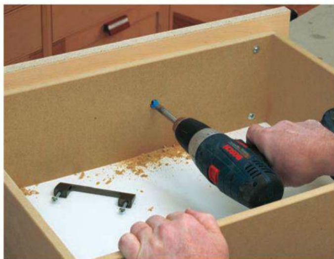
Photo 13: Drill 1/2 "-diameter pull bolt counterbore holes through the drawer fronts. Use a Forstner bit centered in the locator holes you just drilled. Don't drill into the drawer face.
