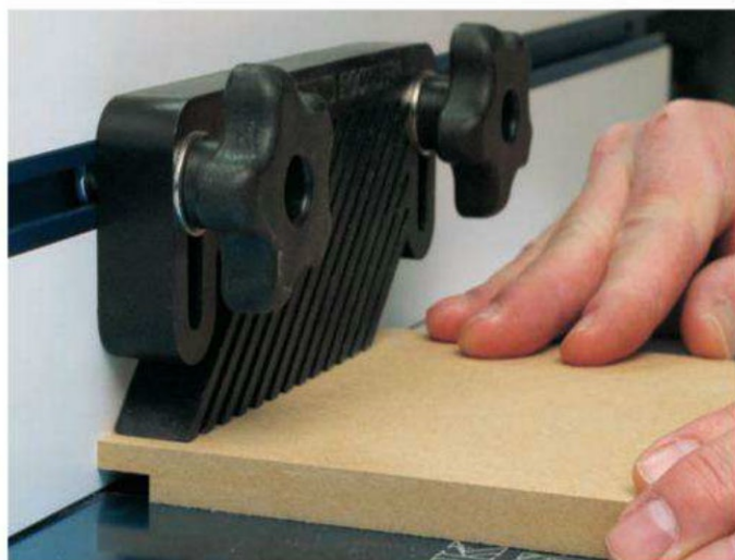
Photo 5: Rout the 1/4" x 1/2"-wide rabbets on the ends of the drawer sides (pieces 9). The total finished width of the drawers needs to be 21".
