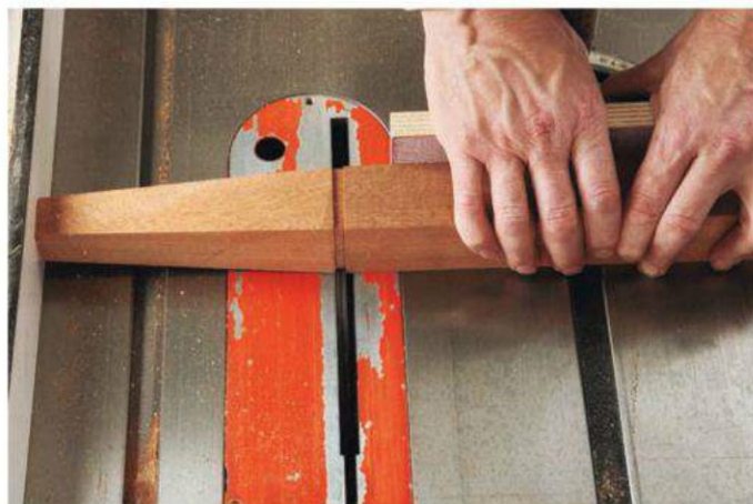
Make four grooves for leg inlay around the tapers by backing each leg blank up against the miter gauge and using the rip fence as a stop block.
