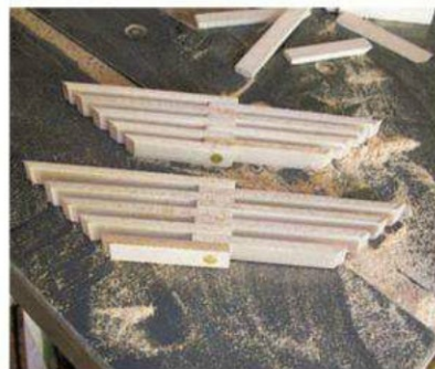
As demonstrated in the three boxes shown on the second page of this article, there are lots of options available with comb hinges. In this sequence, bevels are made, a second set of leaves are added, and edge leaves are employed to cover the pivot.
