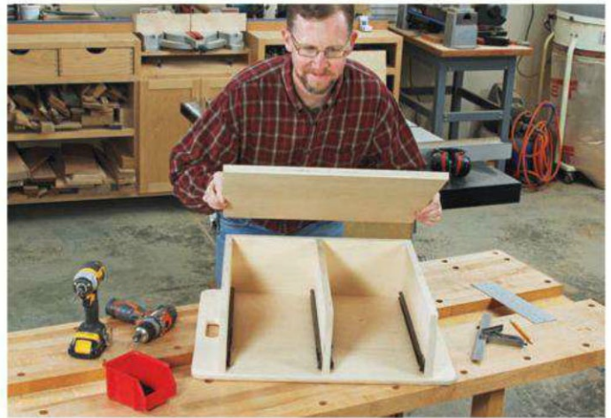
Install the drawer slide hardware before assembling the sides, divider and back panel on the base. The roller tracks would be much harder to install after you've undertaken the assembly.
