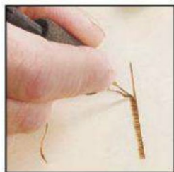
Using a skew to hatch an edge
