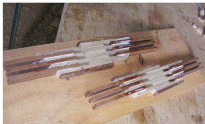
Once the glue sets, everything is sanded, the new leaves are cut to length, and their bevels and tapers (see finished photo above) are added.
