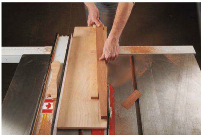
A scrap-made tapering jig with supports nailed in place held each leg blank securely for ripping the short tapers to shape.
