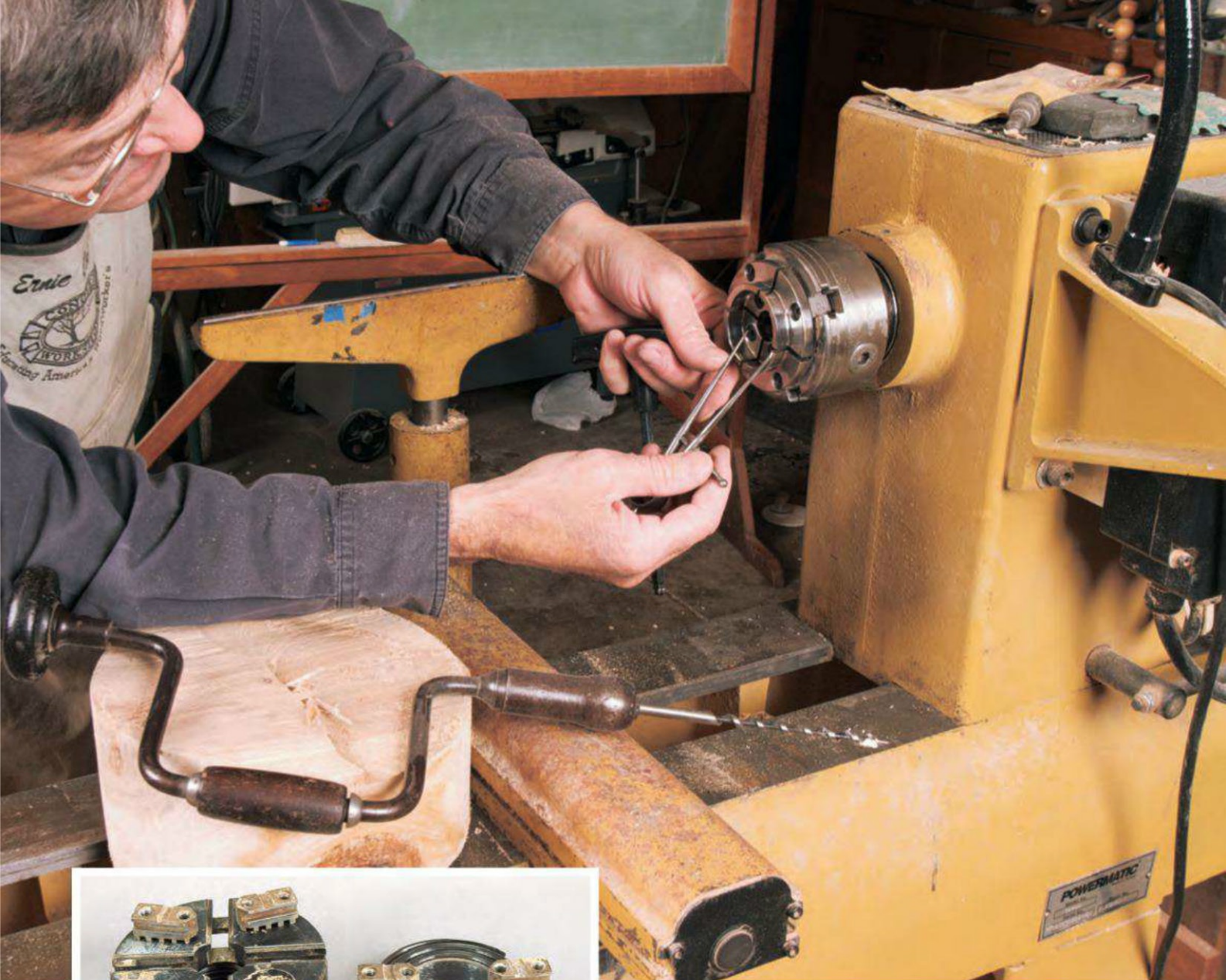
Scroll chuck jaws are two-piece. The bottom half (left) engages the scroll, so the jaw closes or opens in unison. You can screw a variety of jaw extensions to the bottom jaw (right, below) for different needs.
