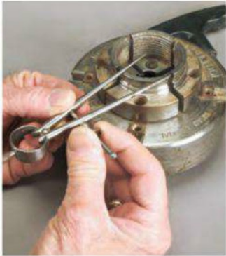
Setting dividers to the radius of the jaws when they form a perfect circle helps get a sure hold when reversing a bowl to turn its inside.
