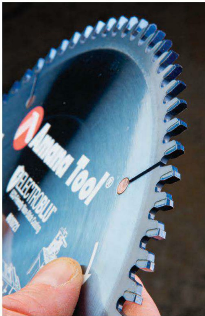
A quality blade coating isn't just eye candy — it's a functional component that reduces pitch deposits, corrosion and heat buildup.
