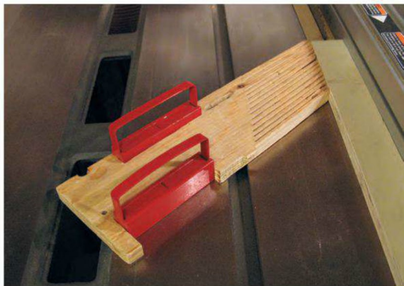
Clamp-free magnetic featherboard
