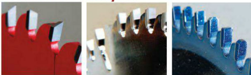
Blades are outfitted with three typical styles of teeth: alternating bevel-topped teeth (left), groups of beveled teeth followed by a flat-topped raker tooth (center) and triple-chip teeth (right) that may also be accompanied by flat-topped raker teeth.
