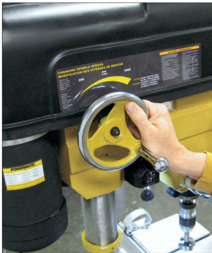
The revolutions per minute (rpm) of the drill bits is adjustable on the fly using the wheel shown at left. The digital readout (above) reports the actual speed — and is variable from 250 to 3,000 rpm.
