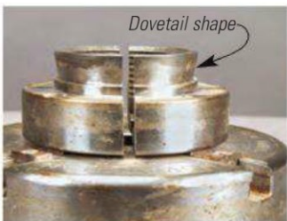
Most manufacturers taper the outside and inside of their jaws to form a dovetail shape.
