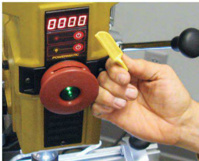
A safety key must be in place or the machine will not turn on. Once removed, the machine will not start even if the large red button is pulled out. If the machine is plugged in, the green light is on.
