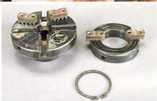
Scroll chuck jaws are two-piece. The bottom half (left) engages the scroll, so the jaw closes or opens in unison. You can screw a variety of jaw extensions to the bottom jaw (right, below) for different needs.
