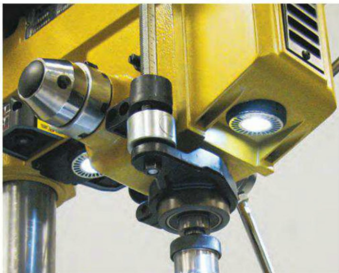
Two LED lights provide virtually shadow-free illumination to the workpiece. Also, note the left-hand optional placement for the quill handles to accommodate ambidextrous drilling operations.
