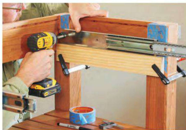
Before the author cut the drawer parts to final size and created the corner joinery (left), he mounted the drawer slides to the legs to determine the actual span between the hardware (center). That distance impacts the length of the drawer front and back workpieces. For a perfect fit, the drawer box was built slightly wider than necessary, then the sides were "shaved" incrementally at the jointer (right) until the box slid easily into position.
