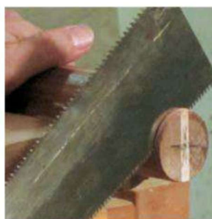
Once holes for the tenons were bored in the tabletop (far left), the author marked them first with a knife to indicate the level of the tabletop on the tenon, then with a saw — with a 1/4" spacer taped to one face — to establish the top of the leg (left). He cut the legs to length (center) and then gently rounded them using a sander (right).
