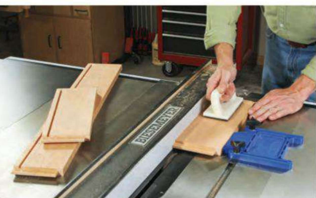
Mortises for the stretchers and aprons all were milled on the router table with spiral bits (above). Squaring their ends is simple chisel work (right). The three aprons received shallow grooves (bottom) to fit wooden tabletop fasteners.
