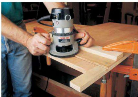
Figure 1: Make your T-square jig using an extra-wide piece of 1/4" plywood for the base. Trim it to size with your router and a 1/4" straight bit. Now you can align the edge of the base with your layouts and rout grooves using a dovetail bit.
