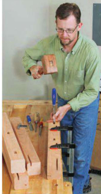
Mortises for the stretchers and aprons all were milled on the router table with spiral bits (above). Squaring their ends is simple chisel work (right). The three aprons received shallow grooves (bottom) to fit wooden tabletop fasteners.
