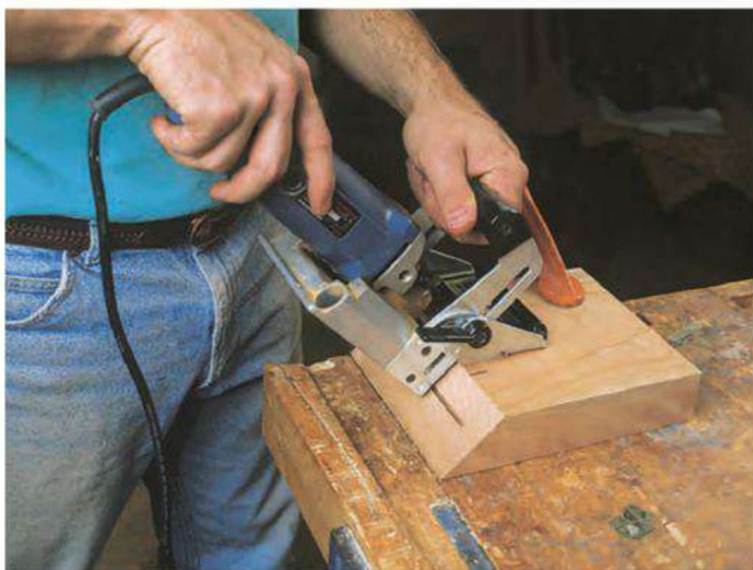
Figure 4: After mitering the front feet, cut slots with a biscuit joiner and join the pieces with biscuits. If you don't have a biscuit joiner, use splines.
