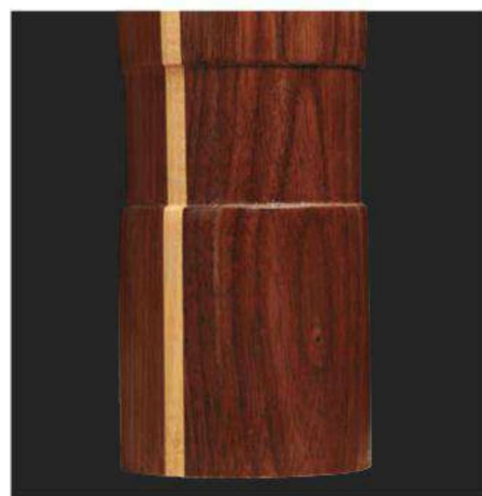
Tenons on the legs come all the way through the tabletop (above left). The legs are joined to the stretchers by large mortise-and-tenon joints that provide a solid connection (center). The ends of the legs present wide, flat feet that help to keep the table from wobbling when in use (above right). Plainsawn walnut with a clear finish applied gives this modern-looking game table a classic feel.
