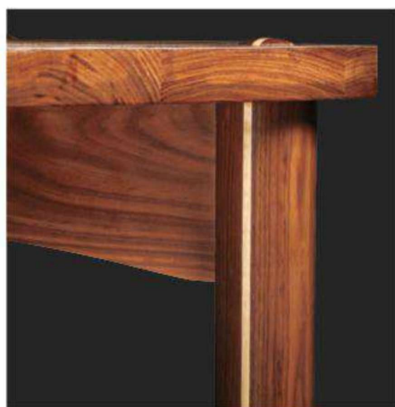
Tenons on the legs come all the way through the tabletop (above left). The legs are joined to the stretchers by large mortise-and-tenon joints that provide a solid connection (center). The ends of the legs present wide, flat feet that help to keep the table from wobbling when in use (above right). Plainsawn walnut with a clear finish applied gives this modern-looking game table a classic feel.
