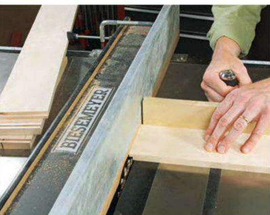
Before the author cut the drawer parts to final size and created the corner joinery (left), he mounted the drawer slides to the legs to determine the actual span between the hardware (center). That distance impacts the length of the drawer front and back workpieces. For a perfect fit, the drawer box was built slightly wider than necessary, then the sides were "shaved" incrementally at the jointer (right) until the box slid easily into position.
