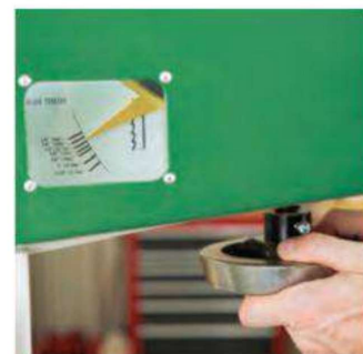
Variable-speed (above) enables the 10-370 to cut metal and wood. Hand wheels (below) ease setup tasks.
