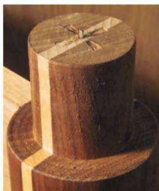
After clamping the legs to the stretcher with V-blocks as cauls (above), the author placed clipped nails in the recess made by the turning center (right) to mark the legs' locations on the top.
