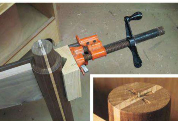
After clamping the legs to the stretcher with V-blocks as cauls (above), the author placed clipped nails in the recess made by the turning center (right) to mark the legs' locations on the top.
