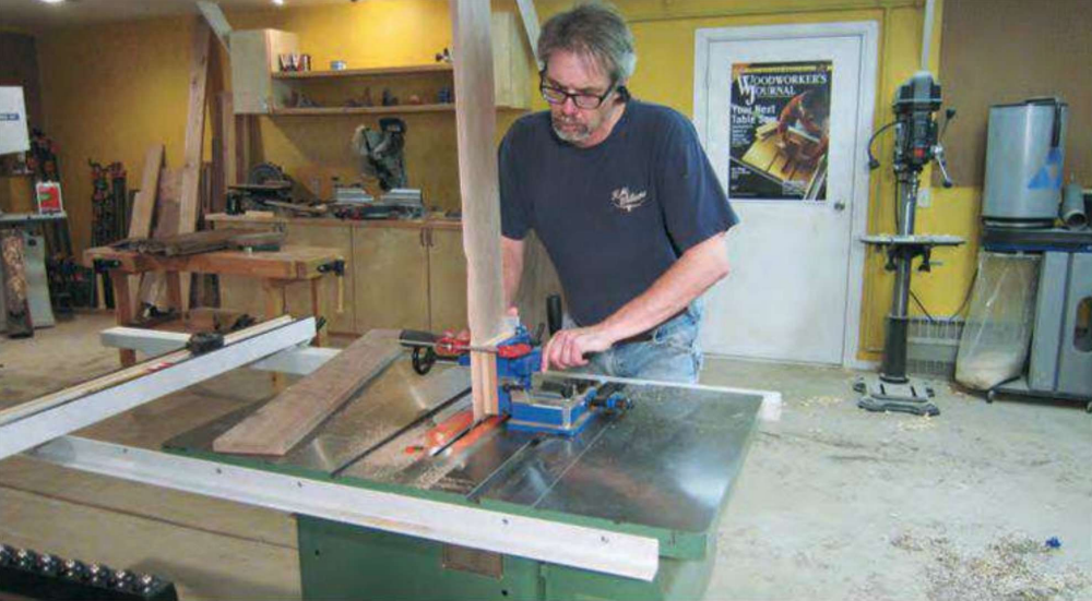
The author used a tenoning jig on the table saw to raise the tenons on the ends of the stretchers.
