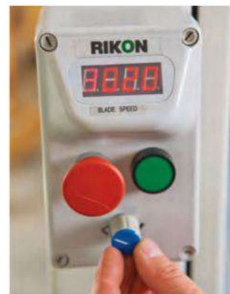
Variable-speed (above) enables the 10-370 to cut metal and wood. Hand wheels (below) ease setup tasks.
