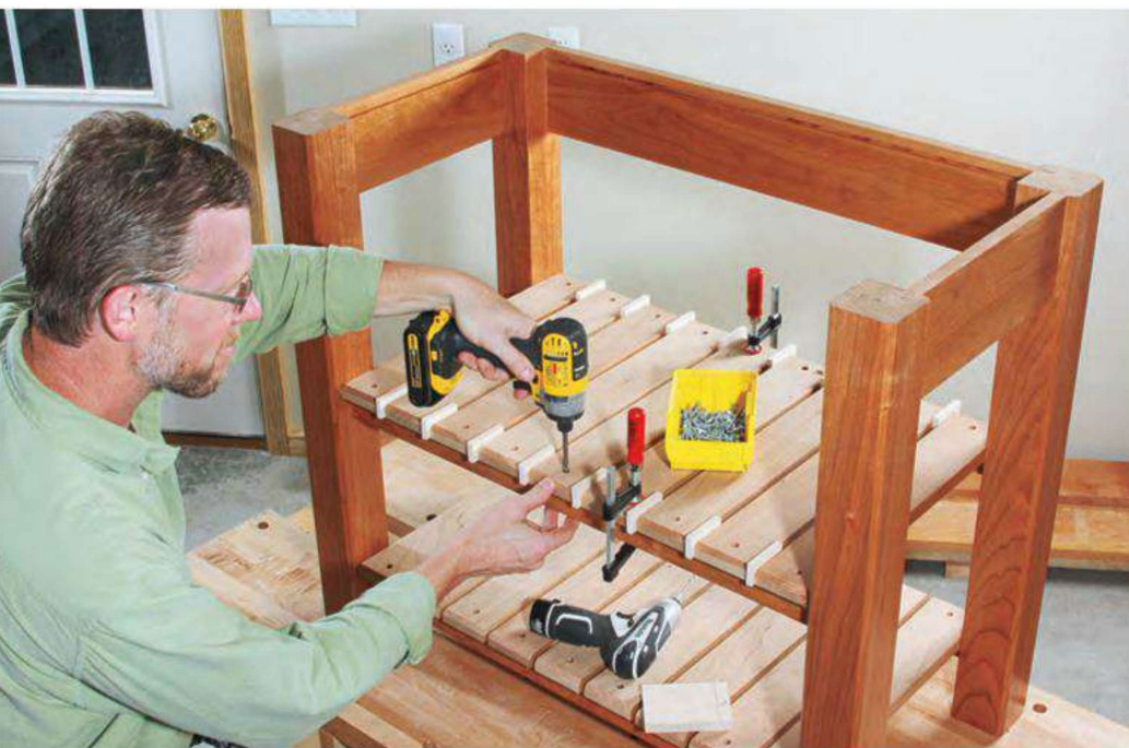
Shelf slats — spaced 5/16" apart and secured with screws — form the lower shelves (left). A scrap of matching cherry stock provided the raw material for shop-made tapered wood plugs (above). They are secured with glue to cover the screw heads and then trimmed flush.
