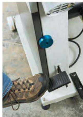
The LT18 came with a wheel kit for mobility (above). A foot brake (below) increases the saw's safety.
