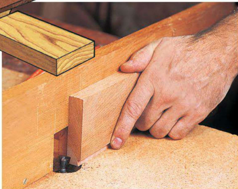
Figure 2: Test the setup for the sliding dovetail construction carefully. Here the author is cutting a test piece to size — it should develop a friction "push fit."
