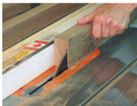
The author resawed the 1 3/4" walnut leg blanks down to size and saved the drop pieces for another time and another project.
