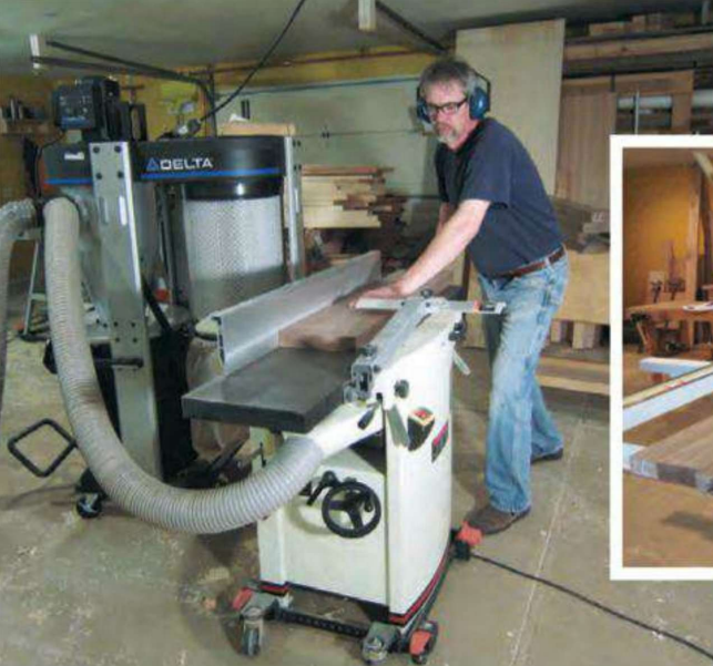
The author prepared the stock for the tabletop through face-planing the walnut. By examining how the various boards look in relationship to one another, he formed an attractive top.
