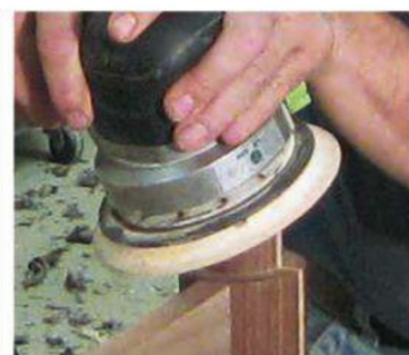
Once holes for the tenons were bored in the tabletop (far left), the author marked them first with a knife to indicate the level of the tabletop on the tenon, then with a saw — with a 1/4" spacer taped to one face — to establish the top of the leg (left). He cut the legs to length (center) and then gently rounded them using a sander (right).
