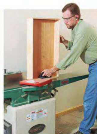
Before the author cut the drawer parts to final size and created the corner joinery (left), he mounted the drawer slides to the legs to determine the actual span between the hardware (center). That distance impacts the length of the drawer front and back workpieces. For a perfect fit, the drawer box was built slightly wider than necessary, then the sides were "shaved" incrementally at the jointer (right) until the box slid easily into position.
