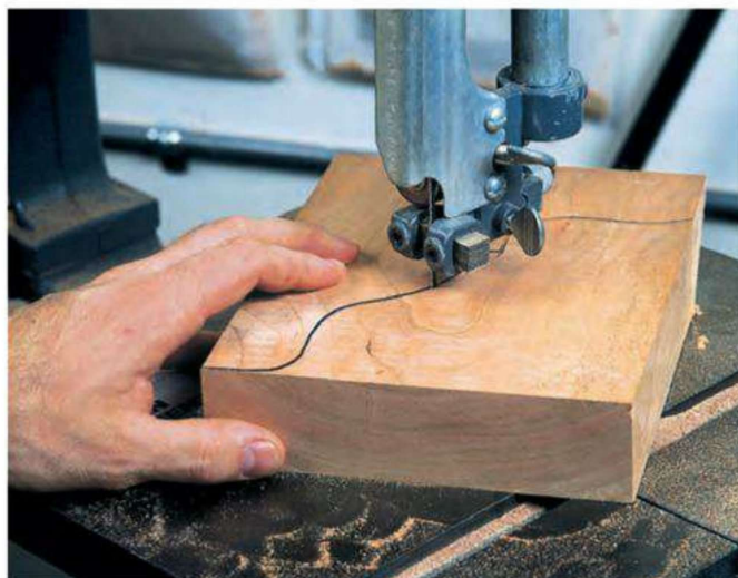
Figure 5: Use a 1/4" or narrower hand saw blade for making the tight cuts along the outline of each foot. Set the saw guides just above the wood to keep the blade from wandering.
