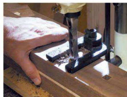
Using a mortising machine, the author chopped out the mortises when the legs were glued up but still in rectilinear form.
