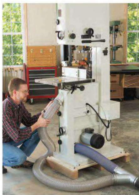
Band saws produce copious fine dust. Double 4" dust ports effectively manage it.
