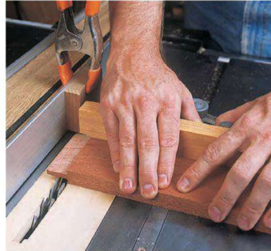
Figure 3: Clamp a setup block to your fence to align the shoulder of your tenon layout with the 1/2" dado blade. Make two passes to cut each cheek.
