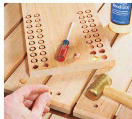
Shelf slats — spaced 5/16" apart and secured with screws — form the lower shelves (left). A scrap of matching cherry stock provided the raw material for shop-made tapered wood plugs (above). They are secured with glue to cover the screw heads and then trimmed flush.
