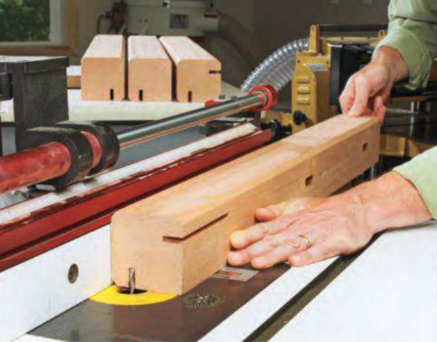
Mortises for the stretchers and aprons all were milled on the router table with spiral bits (above). Squaring their ends is simple chisel work (right). The three aprons received shallow grooves (bottom) to fit wooden tabletop fasteners.
