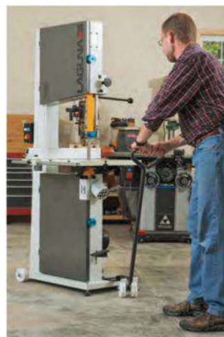
The LT18 came with a wheel kit for mobility (above). A foot brake (below) increases the saw's safety.
