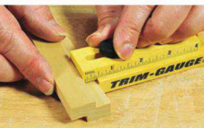
Scribing irregular shapes is made easier with M-Power's Perfect Butt stylus and wheel system (top). Measuring joint heights and offsets is the bailiwick of Brumley's Trim Gauge (bottom).
