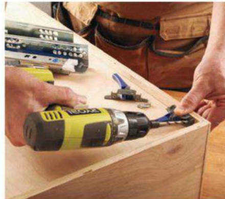
The drawer faces are made from Baltic birch plywood. The author sealed the shaped edges of the drawer faces with a coat of epoxy.
