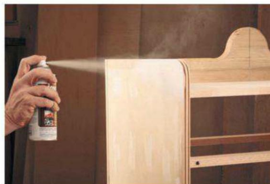
Finish sprayed from a can is perfect for a small project like this. It does lay down thin coats, so multiple applications are required.
