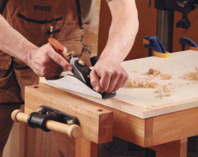
The hardwood trim that is glued onto the top and front edge of the sides is planed flush to the surface of the plywood. The author finds hand planing faster than sanding.
