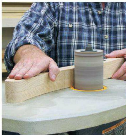
With all components cut out, refine the curves smoothly by sanding down to the marked line. A benchtop disc sander easily handles outside curves, while an oscillating spindle sander takes care of inside curves. Following that, do the finish sanding by hand in combination with a random orbit sander.
