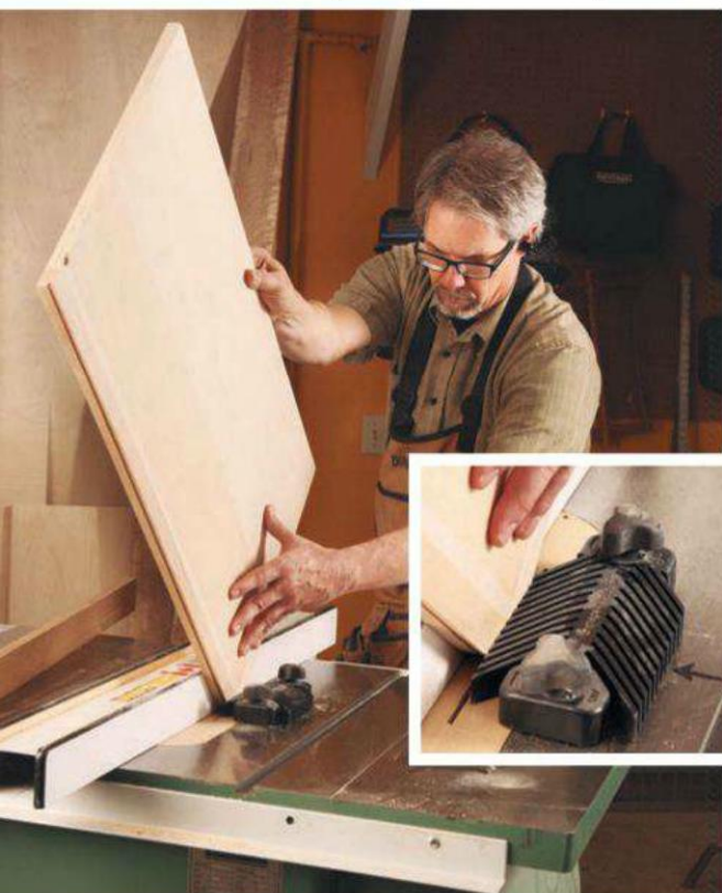
In a "not at all dangerous" technique, the author used a saw blade raised just above a zero clearance insert to groove around the forward edges of the sides. An arrow is drawn on the tabletop (inset photo) to indicate the saw blade's center.
