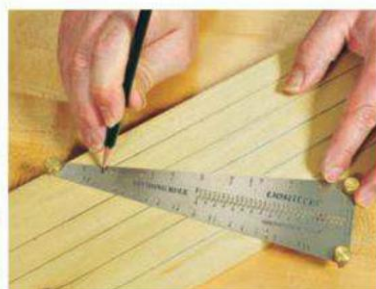
From striking extremely large curves to scribing accurate divided lines, there is a marking tool for the task. The dividing rule by Veritas (at right) is a shop favorite. Brat Manufacturing's Rotape is above left.
