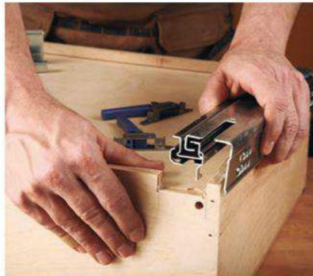
Mahogany lipping is glued to the top edge of the drawer. The shallowest drawer is on the top and the next two get successively deeper.
