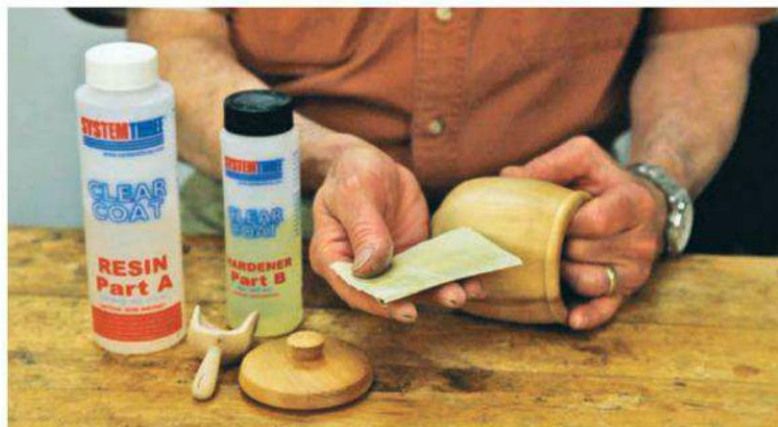
The easiest way to apply Clear Coat is to wipe it on with a 2" square of towel (inset above). Sanding between coats is a must, but easy to do.
