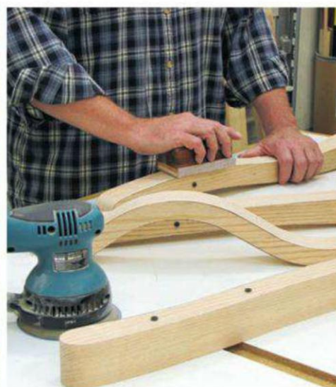
With all components cut out, refine the curves smoothly by sanding down to the marked line. A benchtop disc sander easily handles outside curves, while an oscillating spindle sander takes care of inside curves. Following that, do the finish sanding by hand in combination with a random orbit sander.
