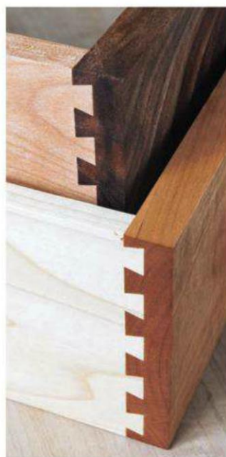
Two examples of half-blind dovetails from a router jig.
