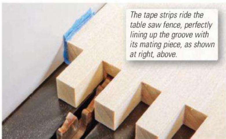
The tape strips ride the table saw fence, perfectly lining up the groove with its mating piece, as shown at right, above.
