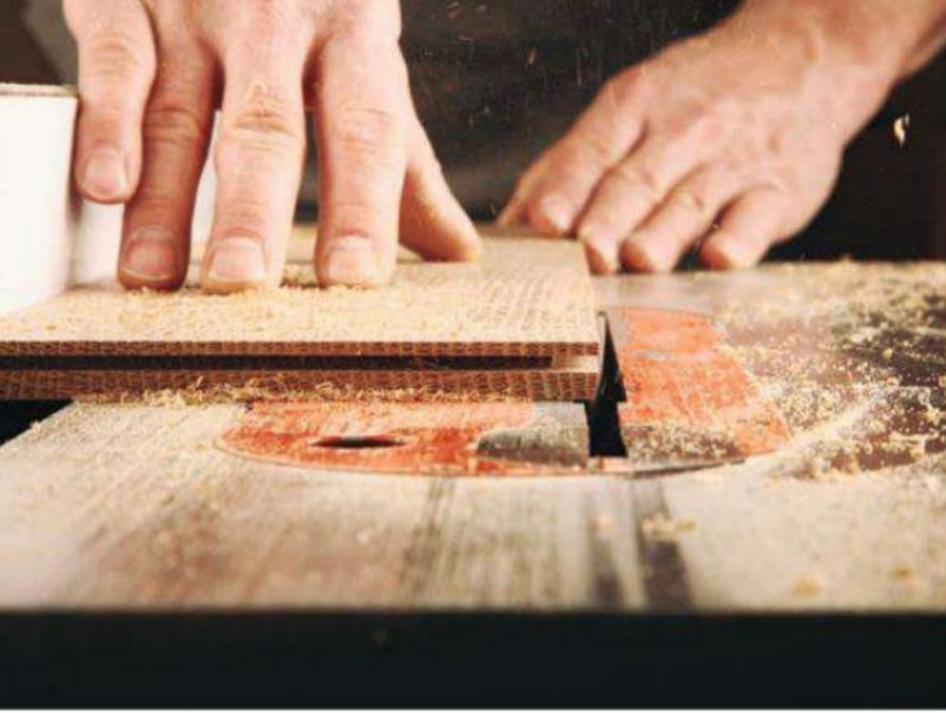
Set the saw blade to make the 15° angle cut on the overlay edges of the panels. The author takes a couple of passes with a hand plane to smooth out the machine marks on these angled surfaces.
