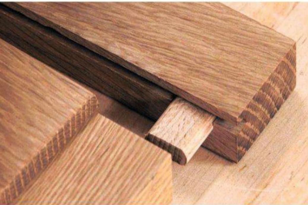
After plowing the groove for the panel, the loose tenon (in this case a Domino) is fit into the stile and rail. Note that the groove runs all the way through the end of the stile.
