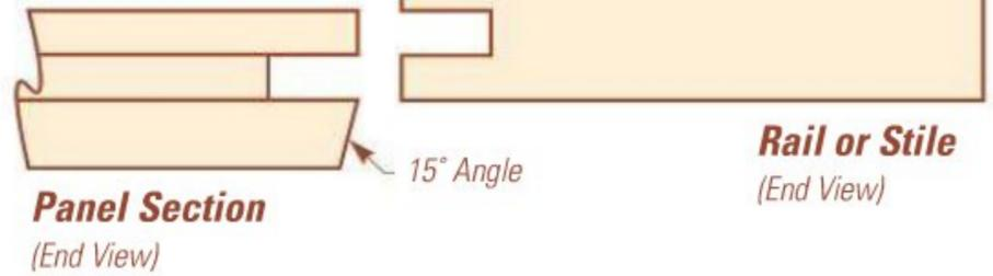
The Domino loose tenon system worked well for this cabinet. Other loose tenon techniques or dowel joinery would work perfectly well to make these joints. The panels must float freely in the grooves to accommodate seasonal wood movement.
