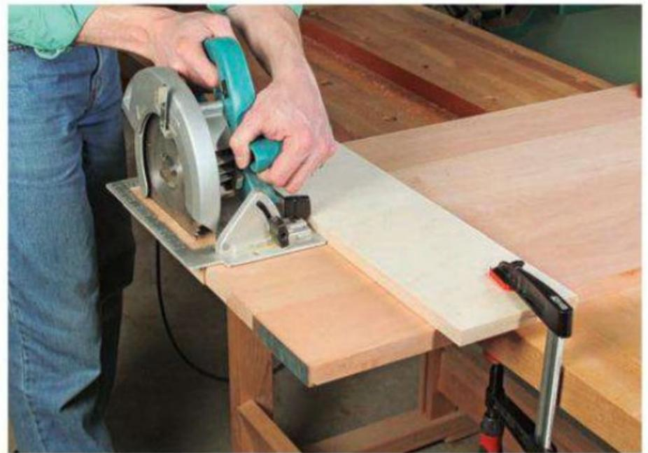
position, you won't achieve those flush ends. Here's my suggestion: glue up the panel now, with the boards overly long. When it dries, install a plywood-cutting or fine-tooth blade in your handheld circular saw and use it to crosscut the panel to length. Run the edge of your saw's base against a straightedge clamped to the panel. Done carefully, you'll
