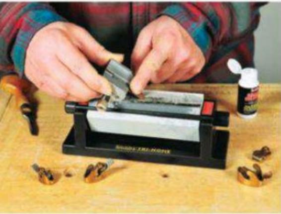
*Grooves in the side-clamping honing guide are capable of holding even very short blades and narrow chisels.*
