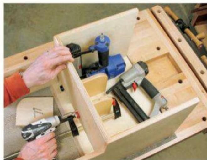
*Use your nail guns as spacers to position the dividers. Clamp each before securing it to the back panel and shelf with countersunk screws.*
