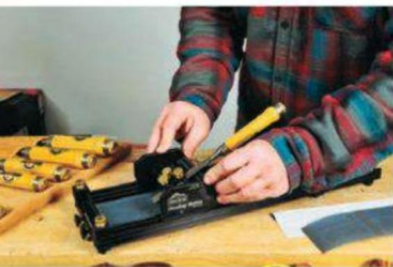
With the blade locked in place (top), you move the Pinnacle guide's carriage back and forth over the whetstone during honing. Small thumbscrews (below) on the side of the carriage let you set both primary and secondary honing angles.
