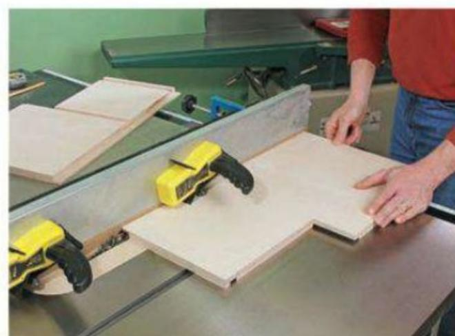
*Feed your side panels along the rip fence to mill the back panel rabbets. Hold-downs of any sort will help to ensure consistent-depth rabbet cuts.*
