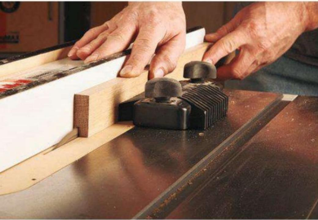
**The grooves in the frame and the panel parts are all made with the same cutter setting. They are easily made on a table saw or a router table.**
