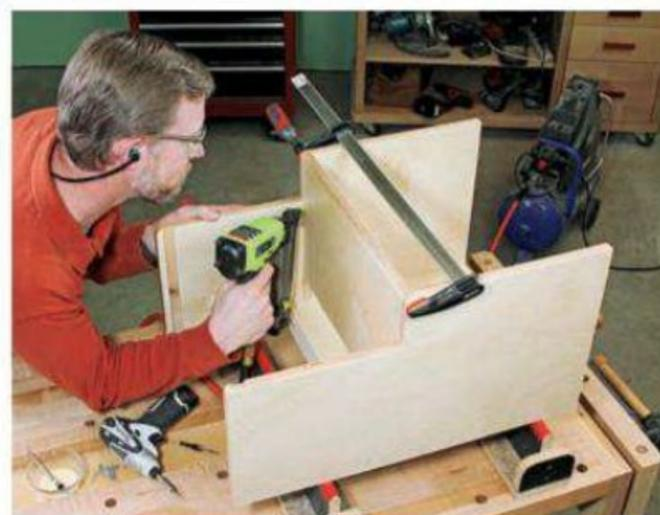
*Clamp the top shelf between the sides, and secure it with glue and 3/4" brads driven into the dadoes from below at a steep angle.*
