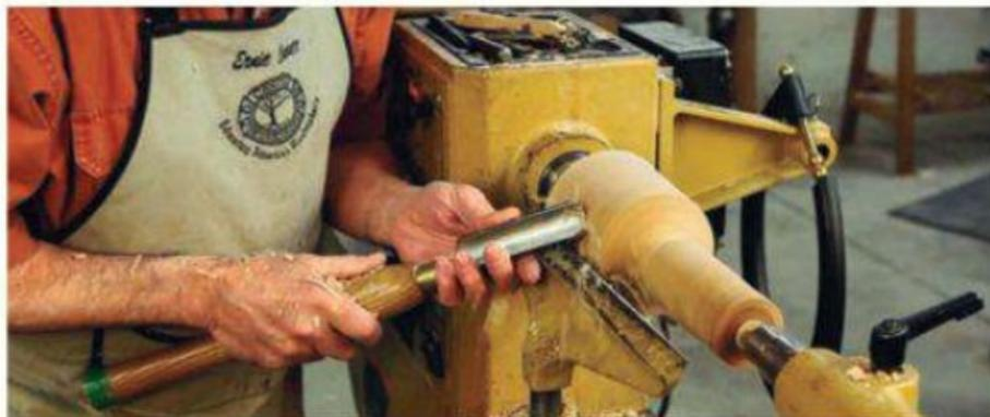
A finish nearly as good as a skew may be obtained by angling a spindle roughing-out gouge, with a long grind, to the work. The tool's handle should remain at the same angle to the tool-rest throughout the cut.
