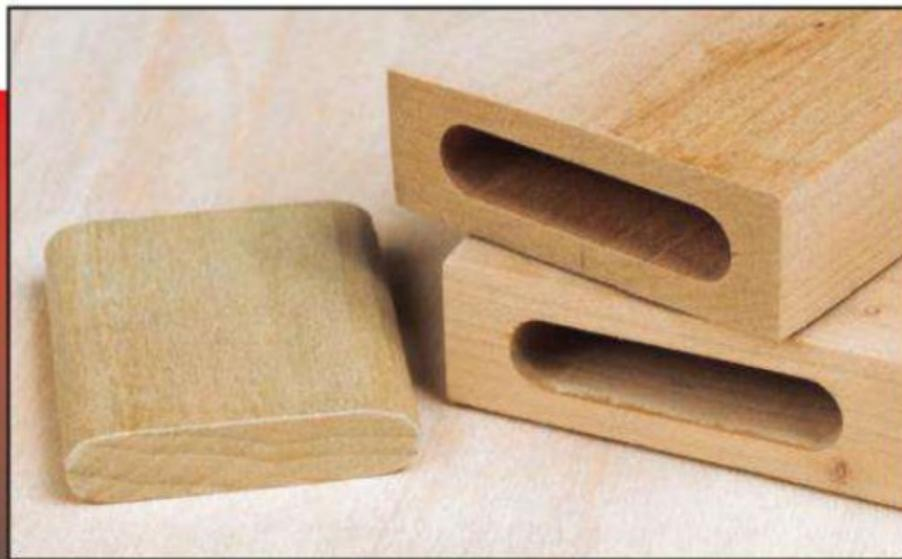
The author's mortising jig, shown on the facing page, only requires you to mark up one piece (left) to set up for cutting both stiles and rails (above).
