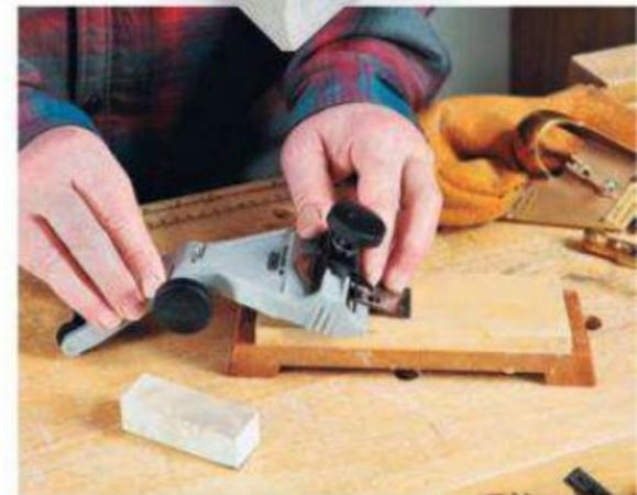
**The knob in the center of the General 809 honing guide is used to set the blade to the desired honing angle.**
