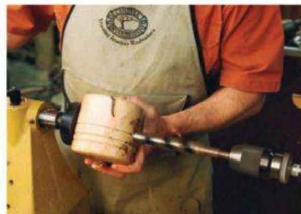
Using your lathe with a crotch center locating the mallet head makes the drill pass through the exact center of the cylinder.
