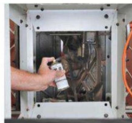
**Cleaning and lubricating your table saw is the first step in troubleshooting sticky gears.**
