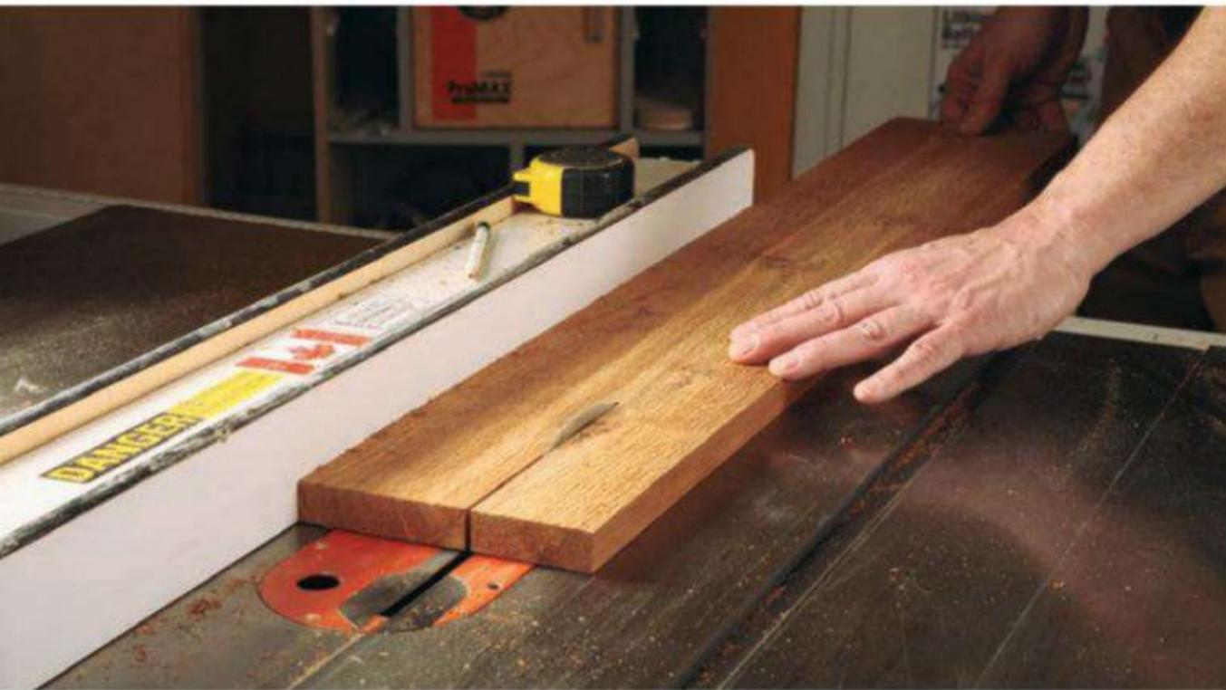
**Although dimension lumber is milled to specific sizes and thicknesses, it is a good practice to rip all your parts to their exact size and not count on the accuracy of the pre-milled pieces.**
