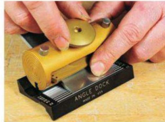
The angle dock that comes with the Sharp Skate III is used to set the blade to be honed at a precise angle.
