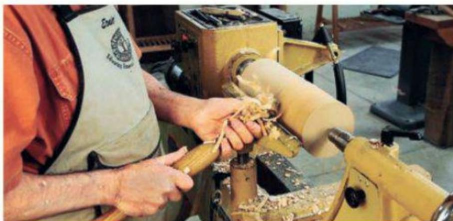
Start with a 3"- to 5"-diameter by 10"- to 12"-long cylinder of green wood to turn a carver's mallet. Turning green wood is fun, because shaping happens fast with long streaming chips flowing off your tools.
