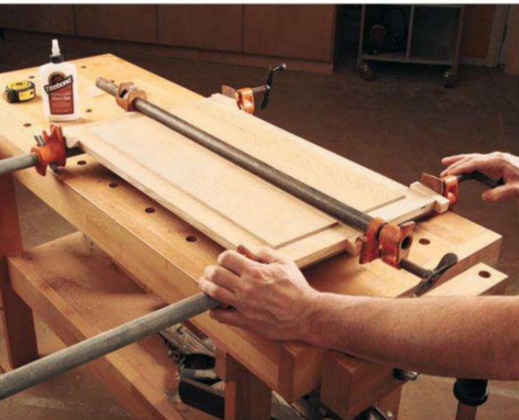
The panels with a muntin can be clamped together in one shot – as shown above. Make the process less hectic by gluing the muntin joints first and then assembling the rest of the panel components.
