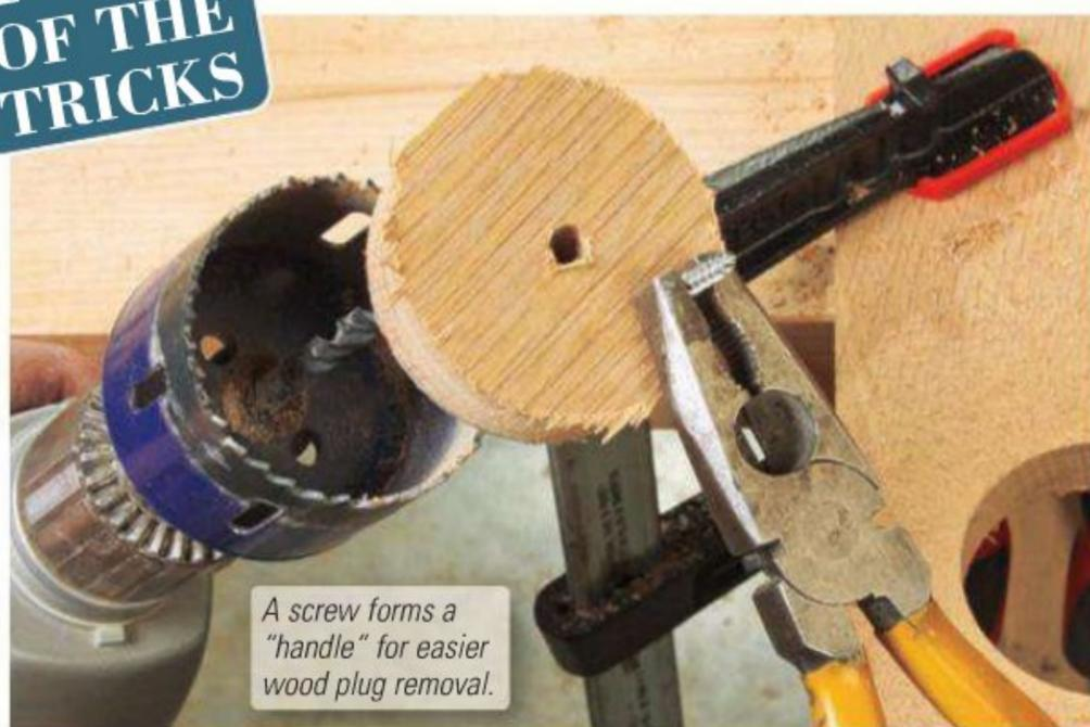
A screw forms a "handle" for easier wood plug removal.
