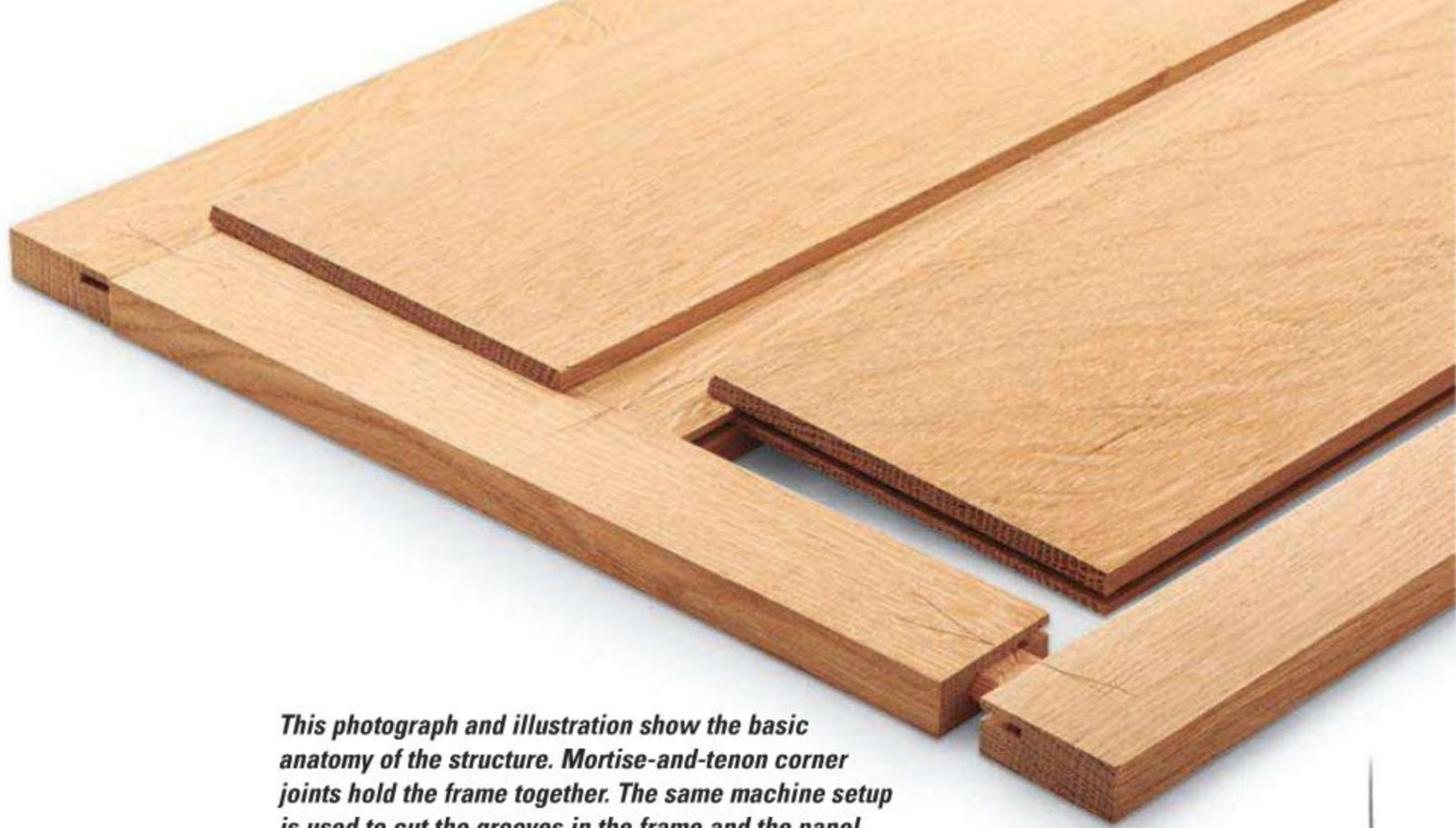
*This photograph and illustration show the basic anatomy of the structure. Mortise-and-tenon corner joints hold the frame together. The same machine setup is used to cut the grooves in the frame and the panel.*
