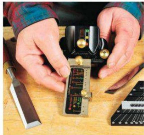
The Veritas MkII guide (top) has a good heft and rolls very smoothly atop any kind of whetstone or honing plate. The registration jig (bottom) that comes with the MkII can be set to a multitude of honing angles to suit multiple sharpening chores.
