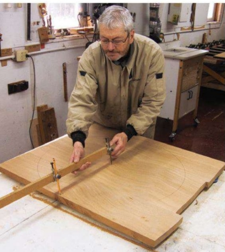
The author laid out the top with a set of trammel points (left), then rough-cut the shape with a jigsaw (center), leaving about 1/8" to be trimmed. Spacers (top right) hold up the top while it is milled to its finished diameter — with a plunge router mounted to a shop-made trammel jig (bottom right). The trammel jig will help you form a perfect circle.
