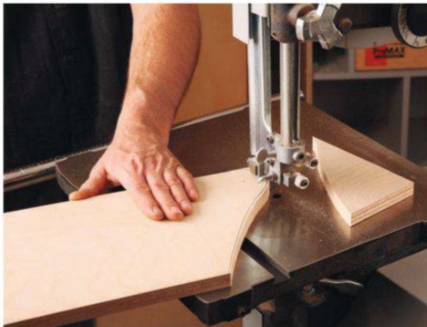
The author made a template to the exact shape of the base front and back curved ends. He transferred the shape to the pieces and rough cut the shape using a band saw. Note that he stayed outside of the pencil line. He refined the cuts to match his template using a pattern-routing bit.
