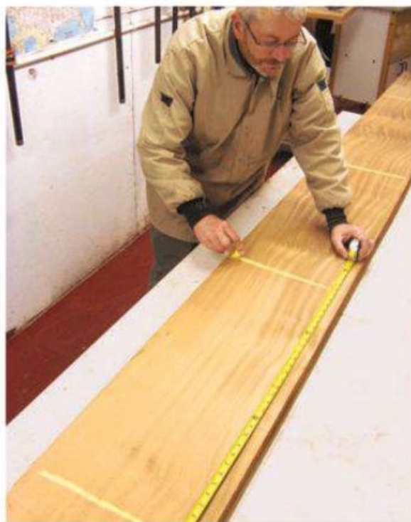
The author chose the workpieces for this table carefully, chalking out their rough proportions on a huge plank of ribbon stripe mahogany before rough-cutting them to size. Above: the wood is allowed to acclimate to his shop.
