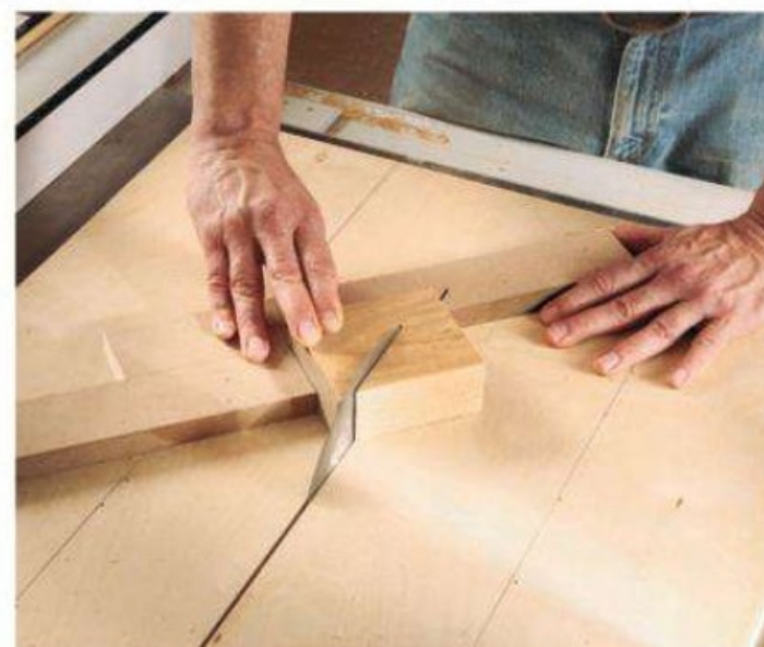
Make yourself a sled, like the one shown above, to safely cut pieces 4. A second cut is then made on each piece, as illustrated at left.
