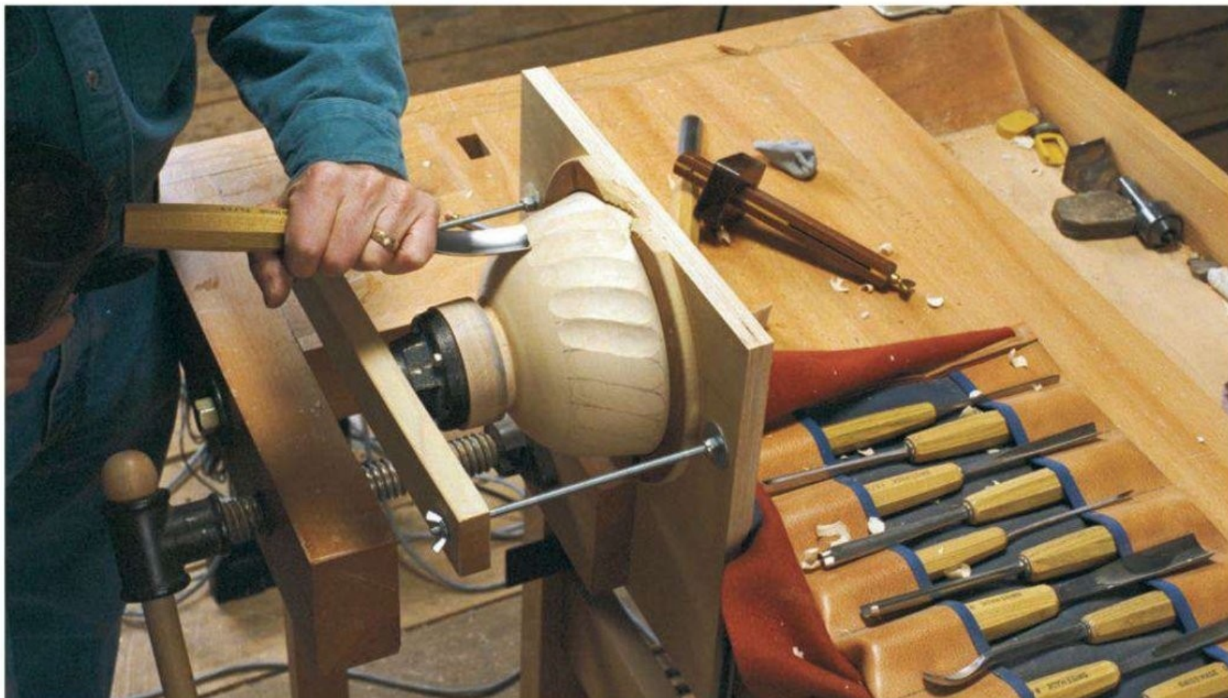
This simple setup for holding your bowl while carving is made from a plywood piece with threaded rods going through it, and a smaller board drilled for the rods, as shown above. Squeeze the bowl between the pieces. The plywood extends below the circumference of the bowl so that it can be captured in a vise, securing it for carving.
