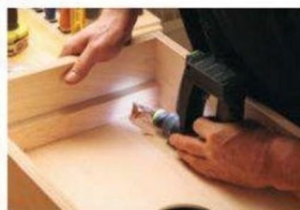
With 1/4" spacers in place and 1" spacers positioned inside the vacuum chamber, slide the bottom subassembly down until it stops on the 1" spacers. Screw it in place.
