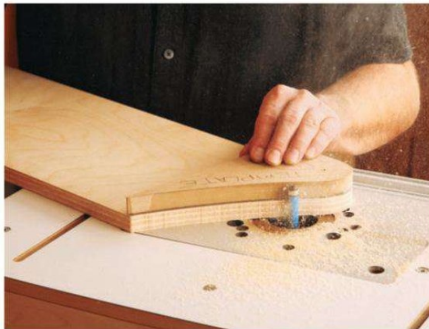
The author made a template to the exact shape of the base front and back curved ends. He transferred the shape to the pieces and rough cut the shape using a band saw. Note that he stayed outside of the pencil line. He refined the cuts to match his template using a pattern-routing bit.
