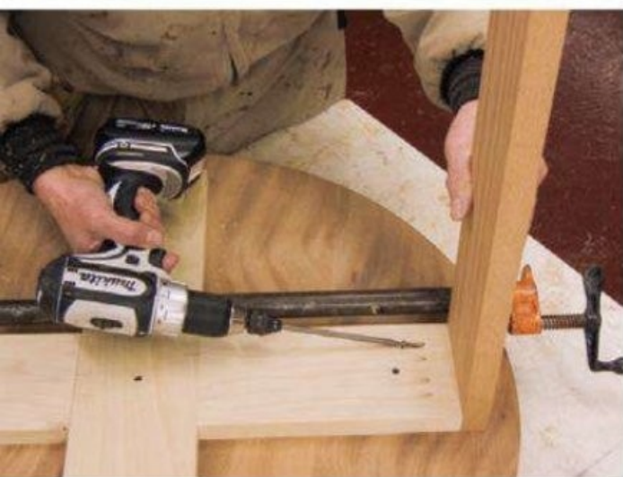
The author attached the legs to the cross-braces with pocket screws. They make strong connections and yet enable the table to be dismantled easily for finishing or transporting.
