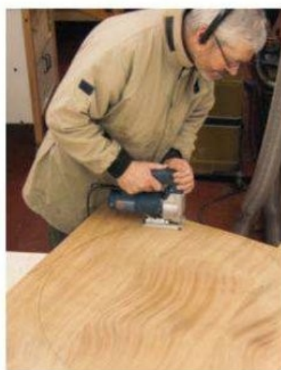
The author laid out the top with a set of trammel points (left), then rough-cut the shape with a jigsaw (center), leaving about 1/8" to be trimmed. Spacers (top right) hold up the top while it is milled to its finished diameter — with a plunge router mounted to a shop-made trammel jig (bottom right). The trammel jig will help you form a perfect circle.
