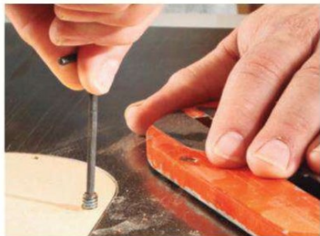
To level a shop-made zero-clearance insert made from MDF, simply swap out the set screws from the insert provided with the table saw.
