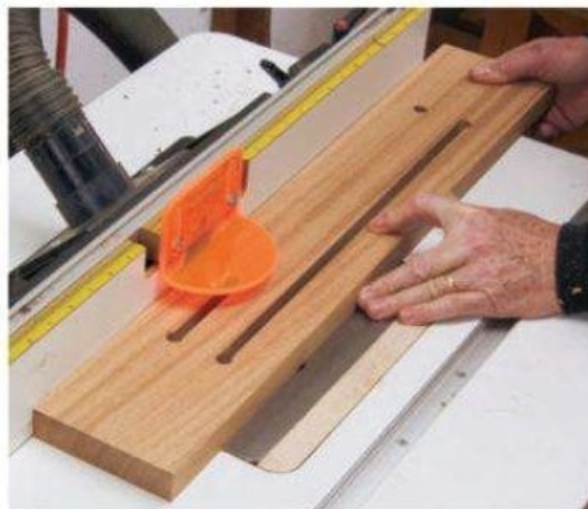
Next, rout a slot between the drilled end holes. Set the fence so the bit is first centered in the hole. Flip the leg over to cut the second slot.
