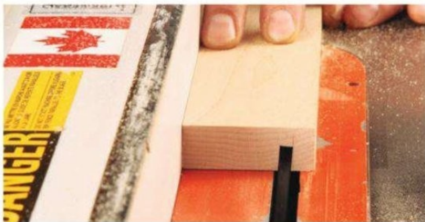
The chamber end cleats have a 7° angle groove plowed down their length. The groove is 1/4" wide to fit the plywood bottom pieces.
