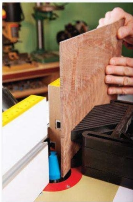
Freud adds precision to edge jointing operations, thanks to two micro-adjust controls on the fence's infeed and outfeed facings (left). MLCS's tall fence offers ample support for vertical panel-raising (right).
