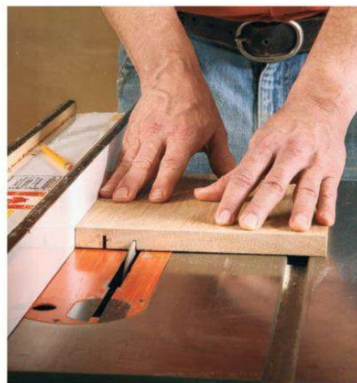
Here, the author is cutting the slots into piece 1. This piece can then be used to set up the rip fence spacing for the matching cuts in piece 2.
