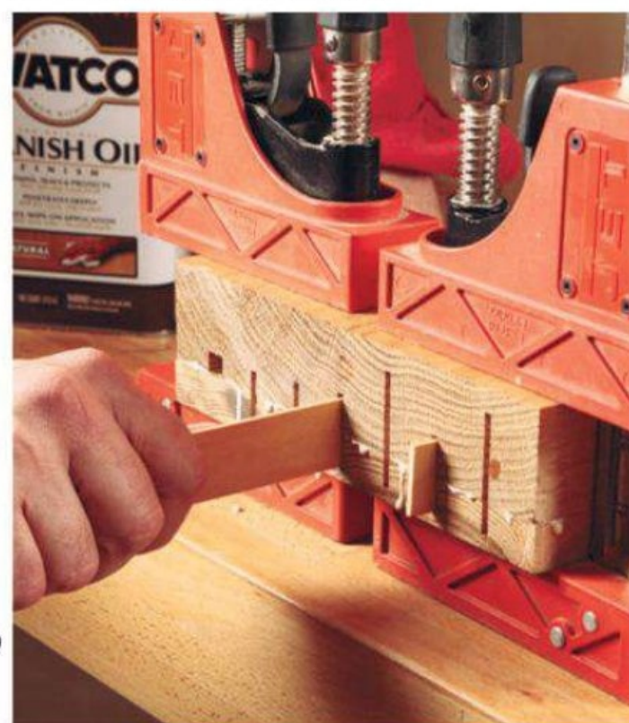
To help keep pieces 1 and 2 aligned during the glue-up process, use oiled 1/8" -thick pieces of plywood placed into the knife slots.
