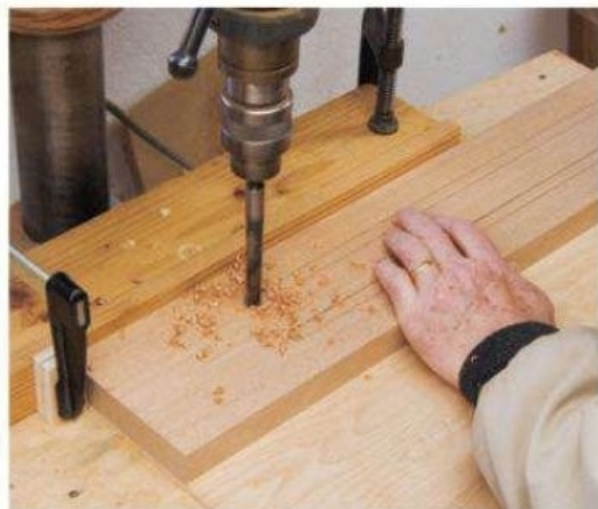
To start the legs, drill 1/2" holes at the beginning and end of each leg slot. A fence and a stop ensure accurate hole placement.
