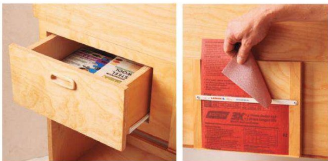
The storage drawer and sandpaper cutting jig are bonus features on this cart, as is the aluminum-covered top (at right), which provides a useful working surface.
