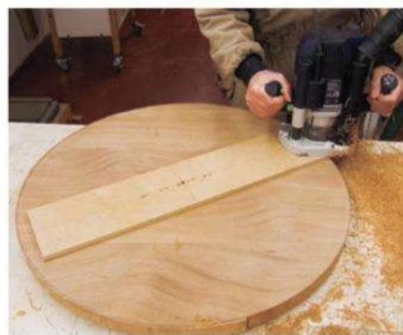
The author laid out the top with a set of trammel points (left), then rough-cut the shape with a jigsaw (center), leaving about 1/8" to be trimmed. Spacers (top right) hold up the top while it is milled to its finished diameter — with a plunge router mounted to a shop-made trammel jig (bottom right). The trammel jig will help you form a perfect circle.
