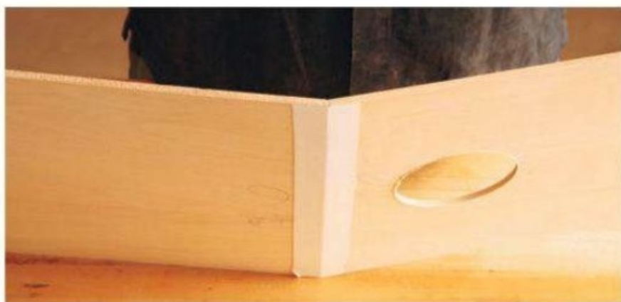
The vacuum chamber's bottom is a bit tricky to assemble and install. Start by using strong tape to join the pieces. Glue the joint and flex as shown.
