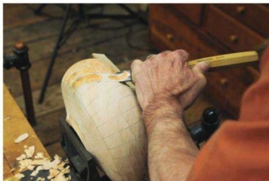
Sometimes refining the shape requires you to carve on the opposite edges of the same trough from different directions to get a clean cut.
