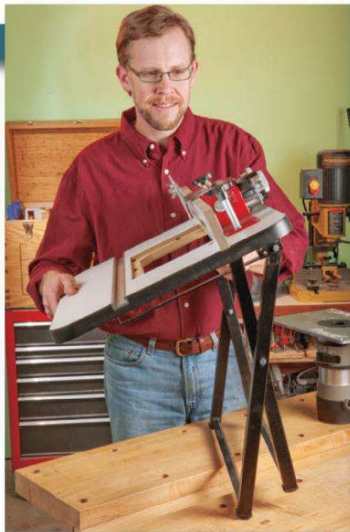
Enclosed bases (top) provide dust collection as well as sound and vibration dampening, but a metal leg base (right) sheds pounds and improves portability.
