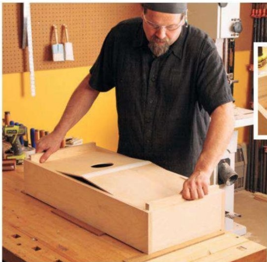
The vacuum chamber's bottom is a bit tricky to assemble and install. Start by using strong tape to join the pieces. Glue the joint and flex as shown.
