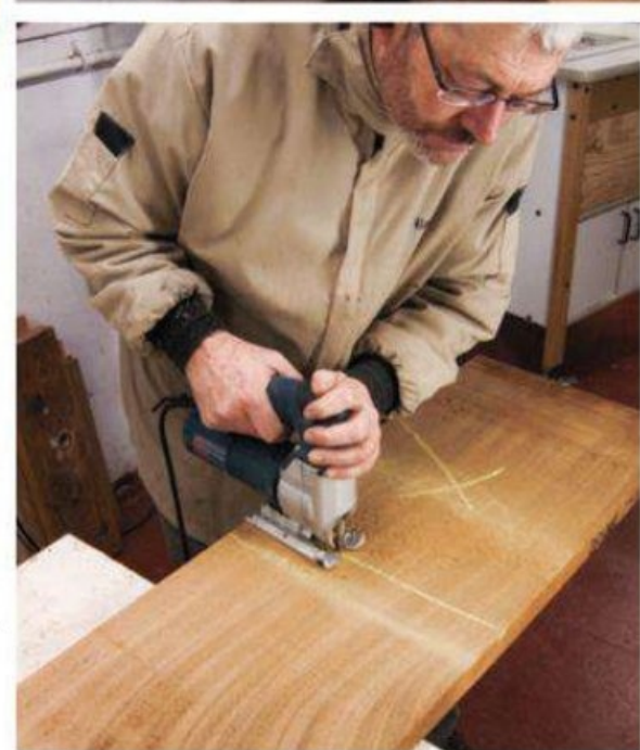
The author chose the workpieces for this table carefully, chalking out their rough proportions on a huge plank of ribbon stripe mahogany before rough-cutting them to size. Above: the wood is allowed to acclimate to his shop.
