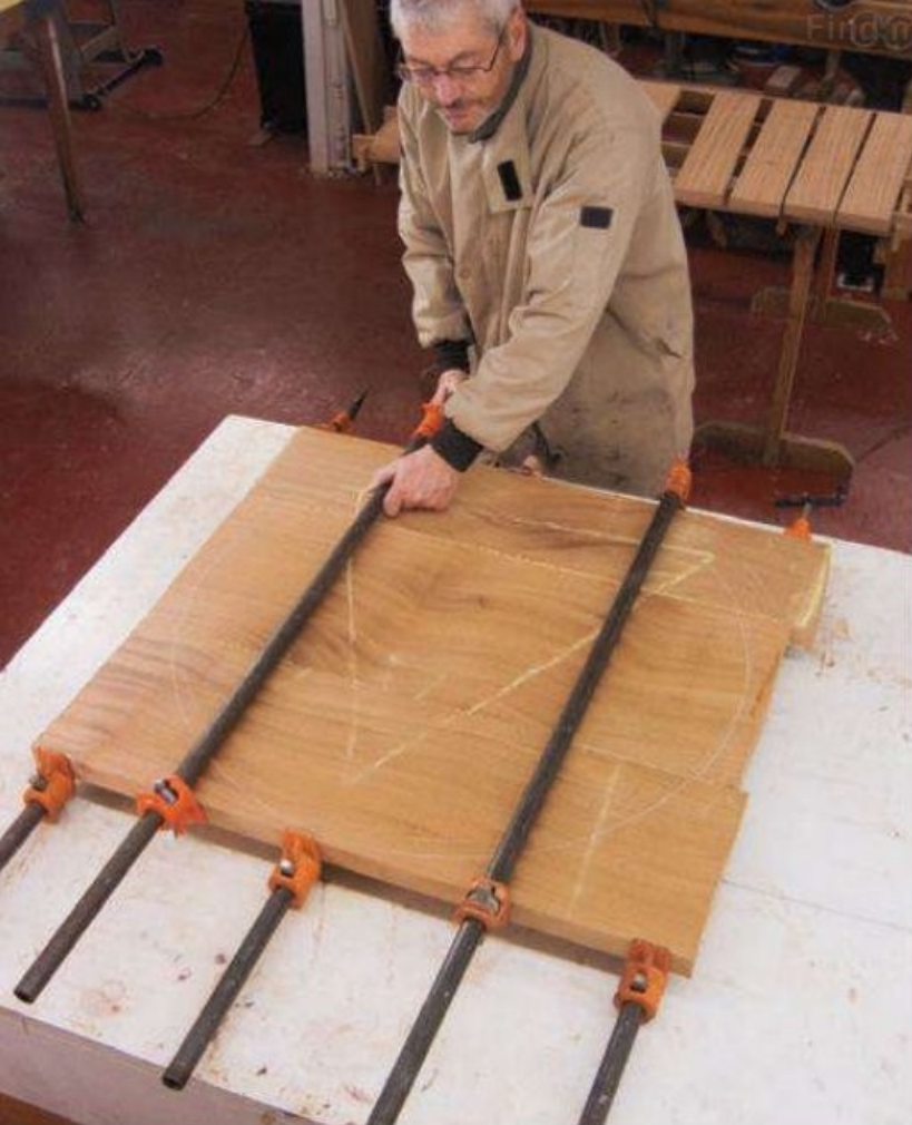
After gluing up blanks for the top and shelf (left), the author uses his shop-made "hand abrasive planer" (above) to surface them smooth and to help tame the wood's reversing grain (right).
