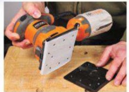
RIDGID's paper punch creates many small holes, allowing for very good dust collection.
