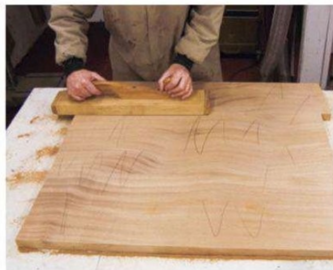
After gluing up blanks for the top and shelf (left), the author uses his shop-made "hand abrasive planer" (above) to surface them smooth and to help tame the wood's reversing grain (right).
