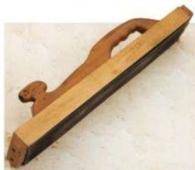
After gluing up blanks for the top and shelf (left), the author uses his shop-made "hand abrasive planer" (above) to surface them smooth and to help tame the wood's reversing grain (right).
