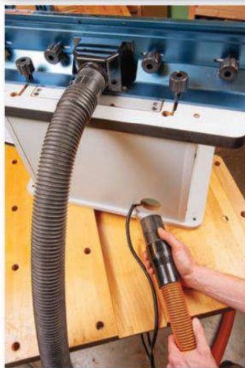
Enclosed bases (top) provide dust collection as well as sound and vibration dampening, but a metal leg base (right) sheds pounds and improves portability.
