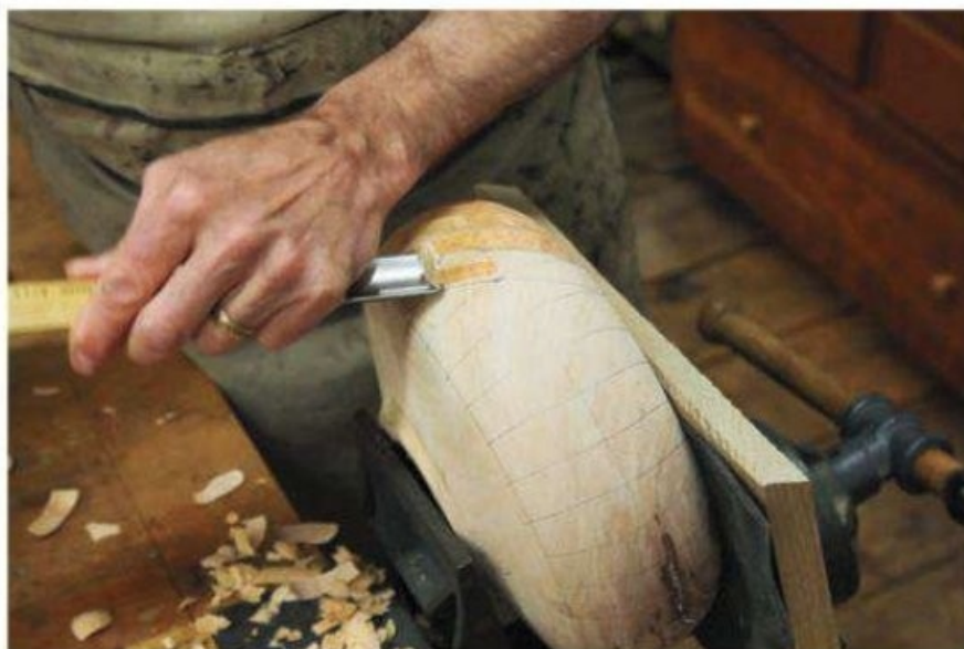
Keep track of grain direction as you carve. Carve "uphill" and don't try to take too much wood off with each cut, refining the shape as you go.
