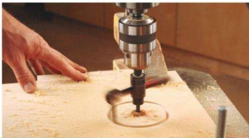
A circle-cutting bit forms the opening for a dust port in the bottom of the vacuum chamber. The bottom is made of two 1/4" plywood pieces.
