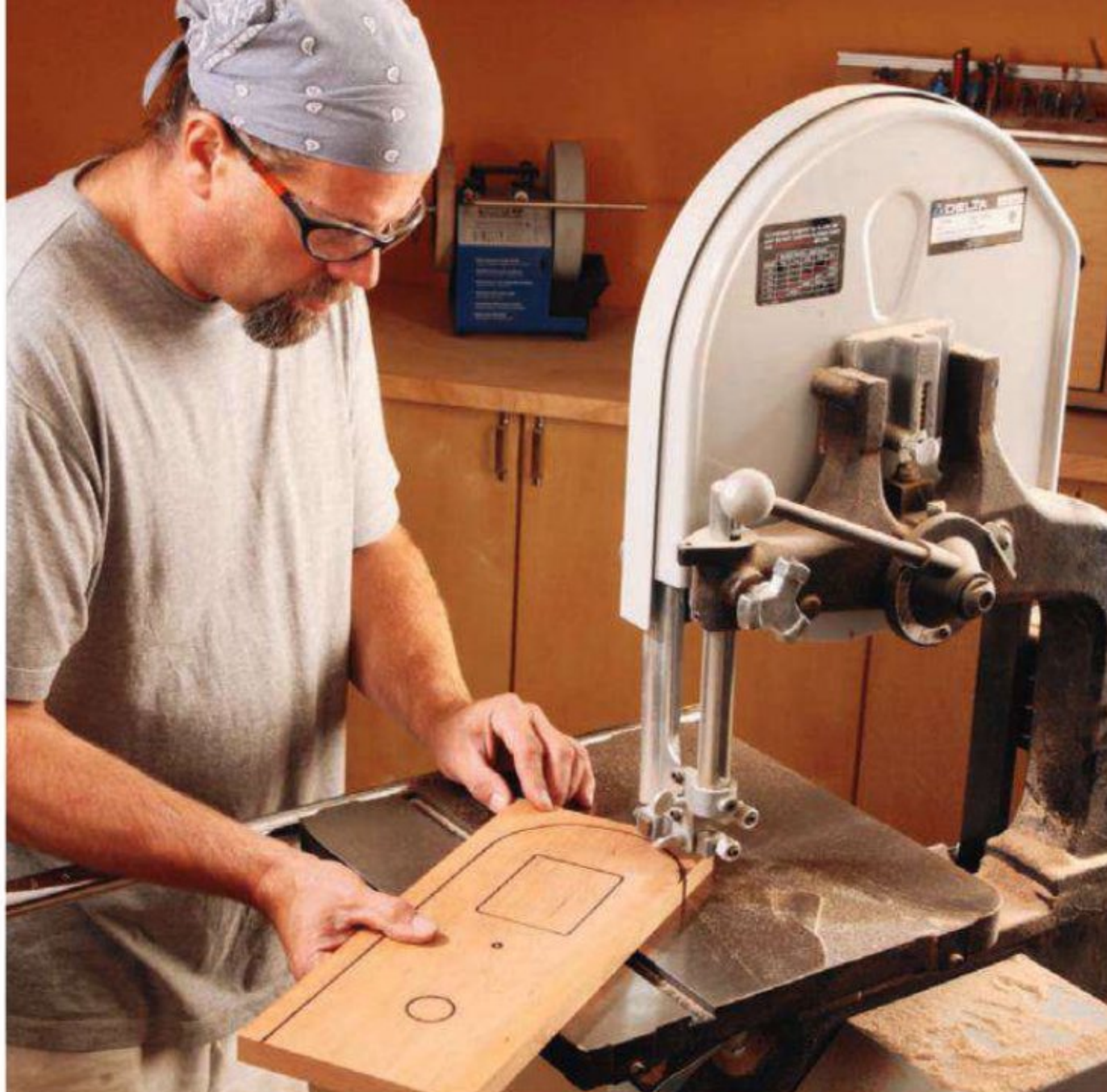
After tracing the core's shape onto a piece of cherry lumber, the author uses a band saw to cut it out. Note that the position of the roto hinge and other details are marked as well.
