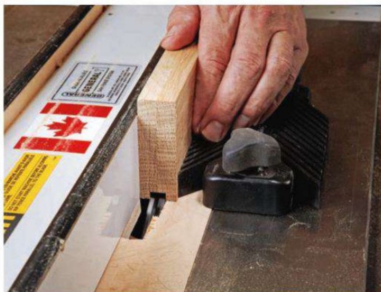
The rails for this table are built up from 1/2" stock laminated together. A groove plowed the length of the rails (left photo) captures the slats and spacers. The lower rails also need tenons raised on their ends. These are through tenons that pierce the 2"-thick legs. The tenons are made on the table saw using a registration block that determines the length of the tenons and also keeps the rail clear of the fence when making the cut (right photo).
