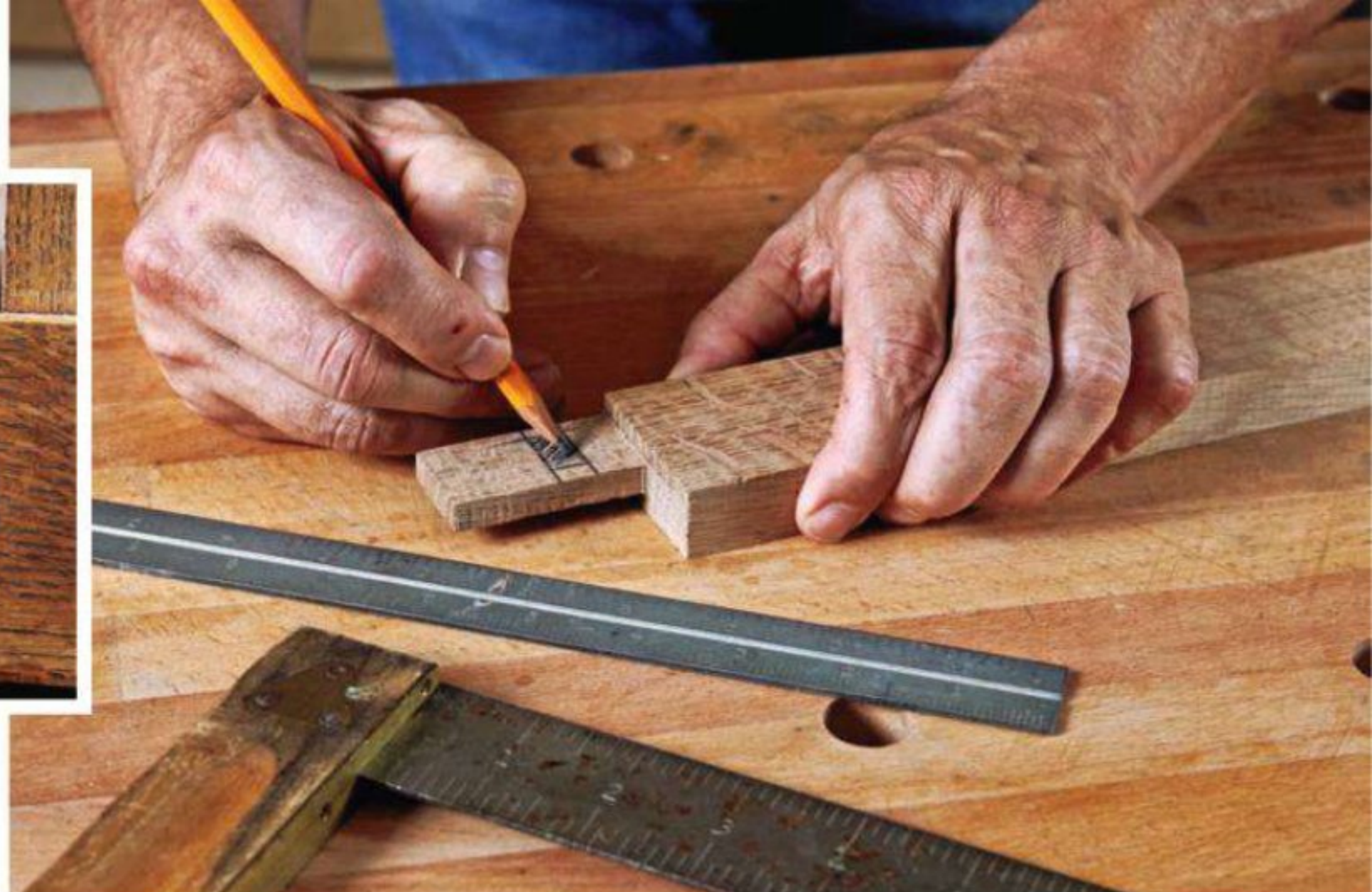
The wedges on the stretcher tenons are simply decorative. The author marked out mortises and chopped the openings with his mortising machine. Note the offset nature of the tenons.
