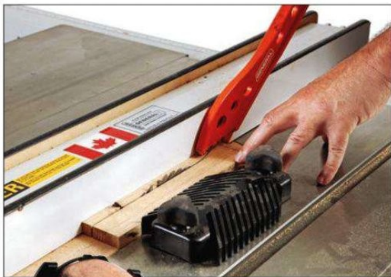
Making a curved slat is a two-step process: Using a table saw, the author first makes a stopped cut, as shown at left. Then, moving to the band saw, he completes the curved aspect of the slat.
