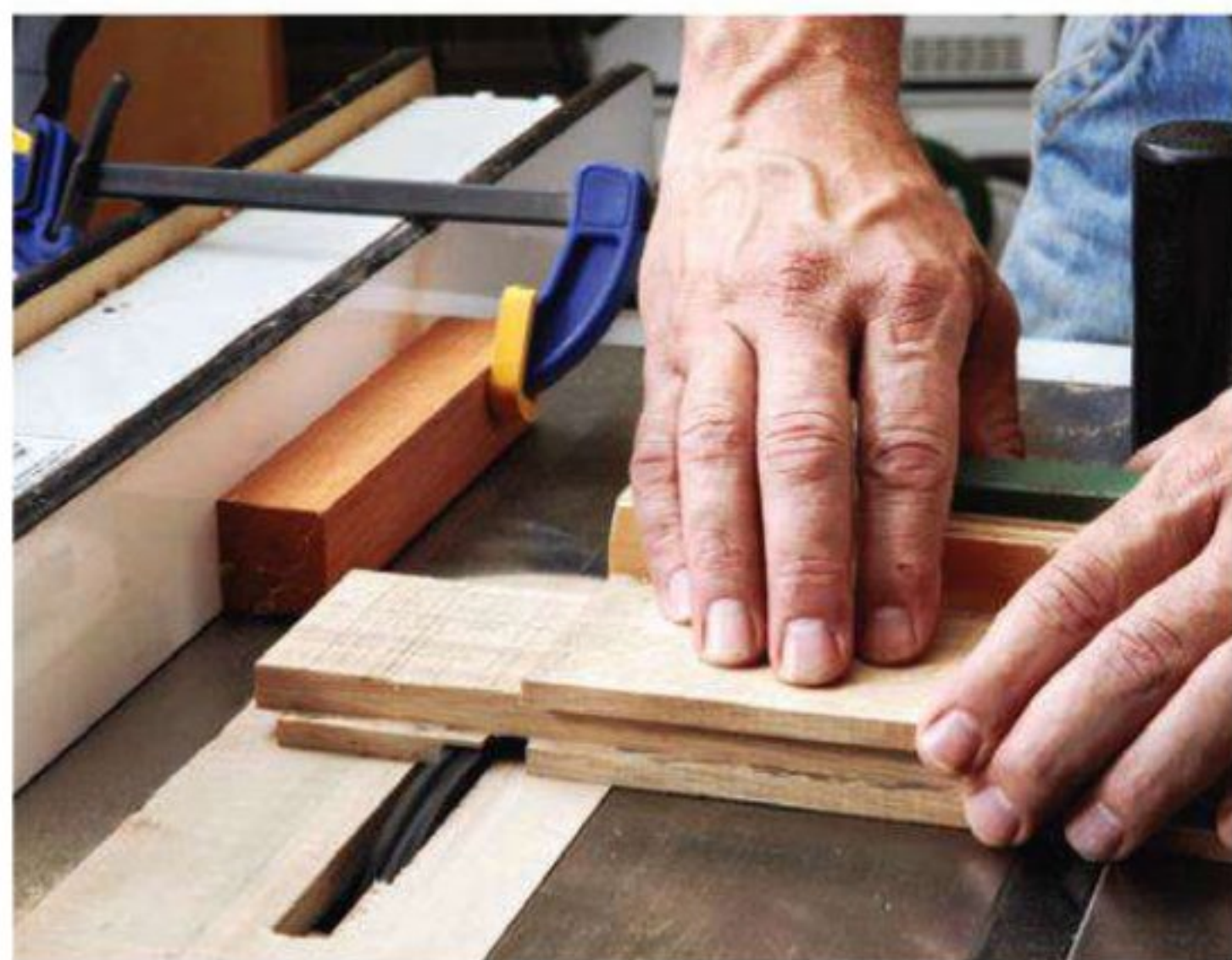
The rails for this table are built up from 1/2" stock laminated together. A groove plowed the length of the rails (left photo) captures the slats and spacers. The lower rails also need tenons raised on their ends. These are through tenons that pierce the 2"-thick legs. The tenons are made on the table saw using a registration block that determines the length of the tenons and also keeps the rail clear of the fence when making the cut (right photo).
