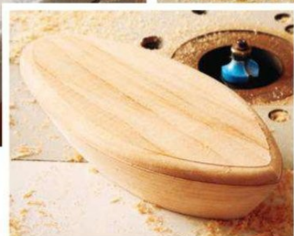
A 3/8" bearing-guided roundover bit shapes the edge nicely. Set it to cut into the top just a bit (inset) — creating a nifty nautical “rub rail.”
