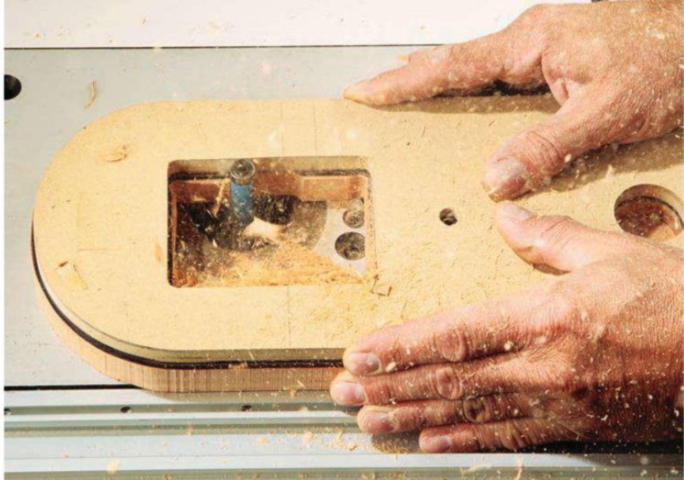
With the template aligned (and attached with double sided tape) to the dark lines marked earlier — which guided the rough cut on the band saw — it was time to start template routing. A pattern routing bit is used to refine the card recess opening and then to shape the exterior profile.
