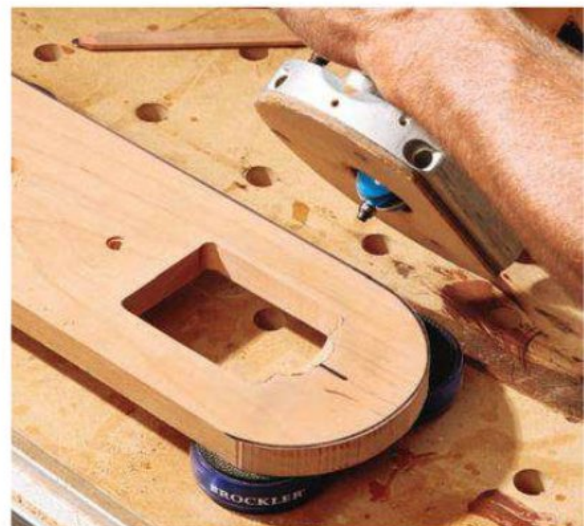
The final bit of shaping on the card recess is made with a large bearing-guided cove bit. The author cut this finger opening "freehand."
