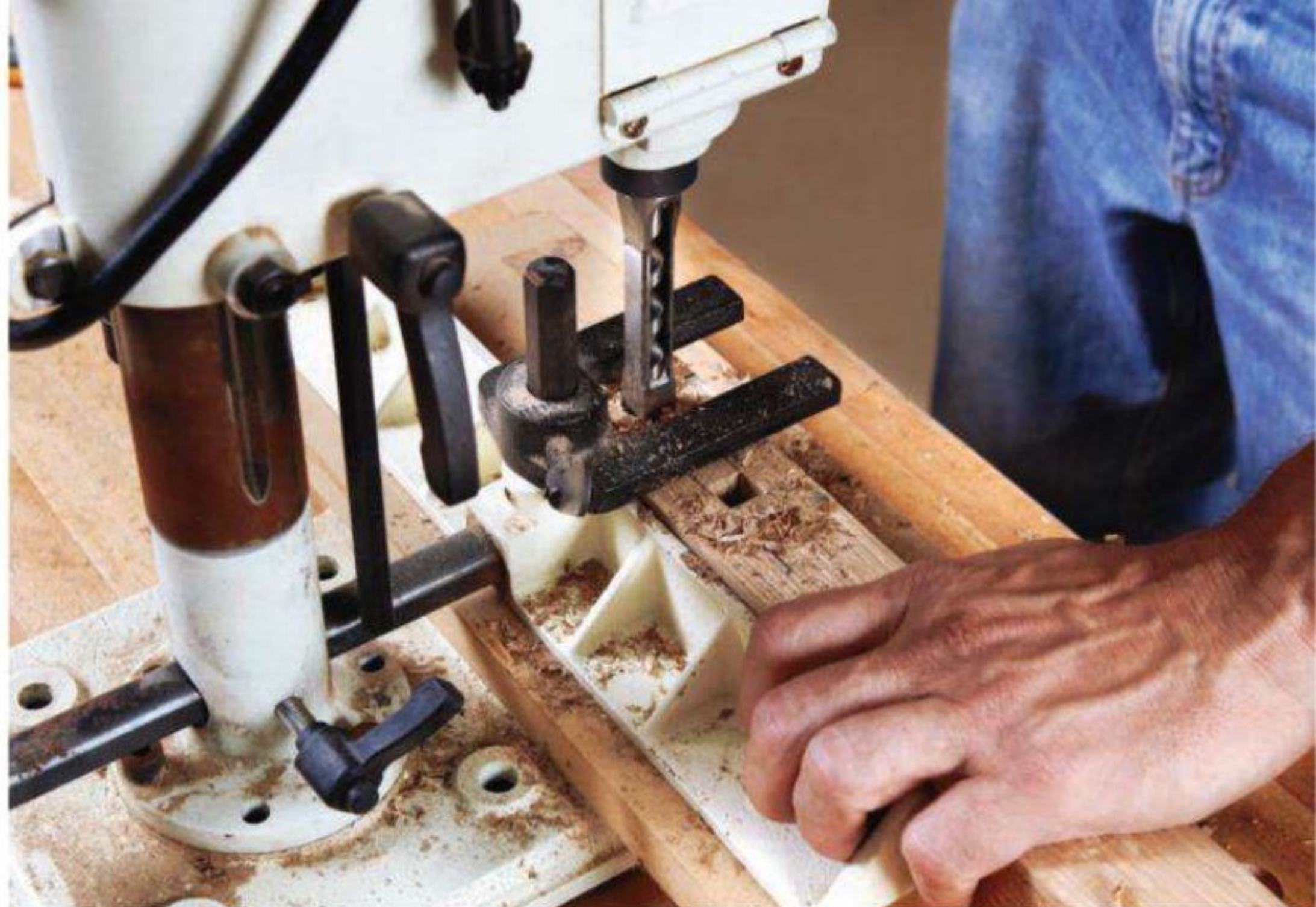
The through mortises on the legs (and the stretchers, not shown here) were chopped out using a mortising machine. Through tenons are not only a sound structural bit of joinery, but they also are a significant part of the Arts & Crafts vocabulary of style.
