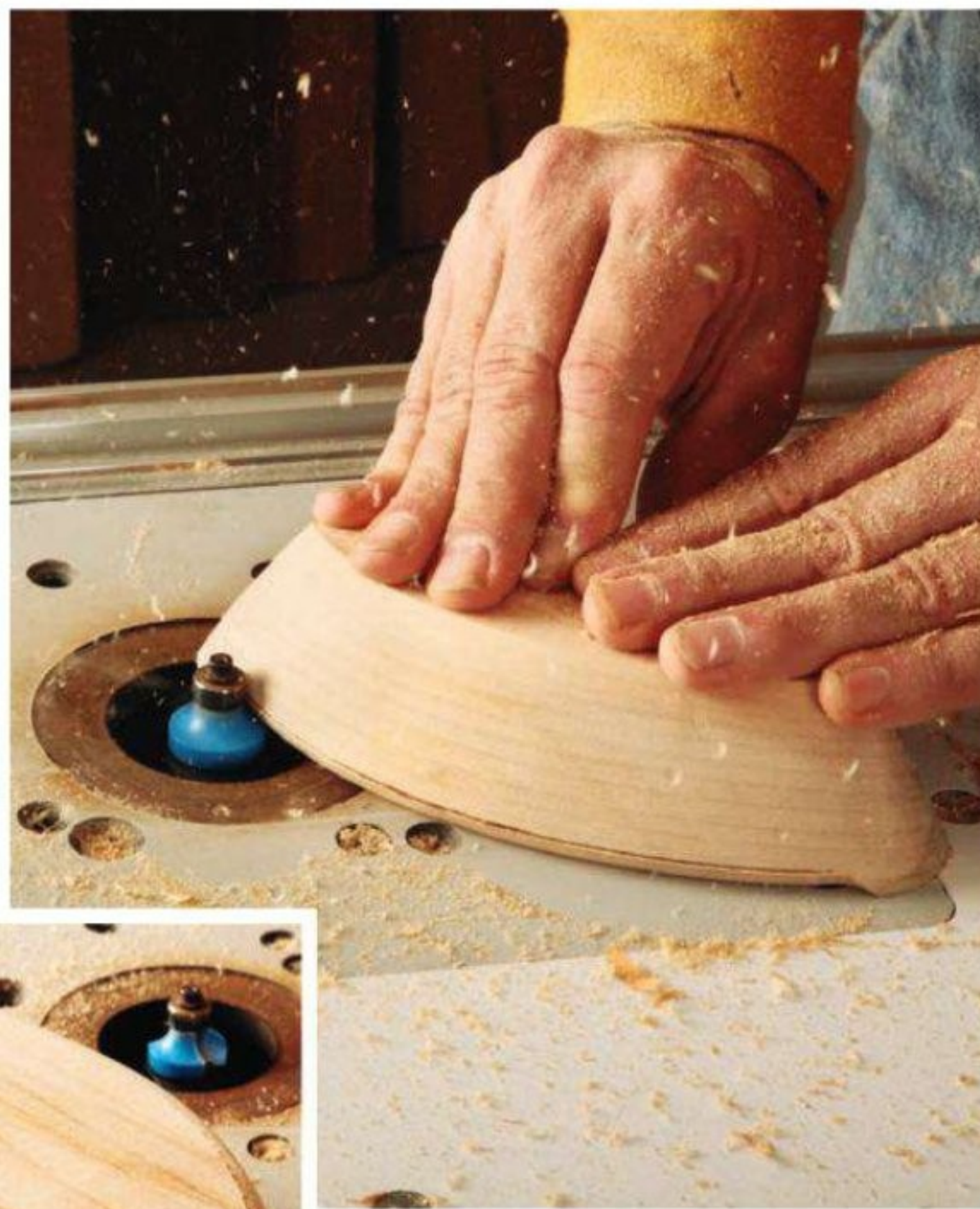
A 3/8" bearing-guided roundover bit shapes the edge nicely. Set it to cut into the top just a bit (inset) — creating a nifty nautical “rub rail.”
