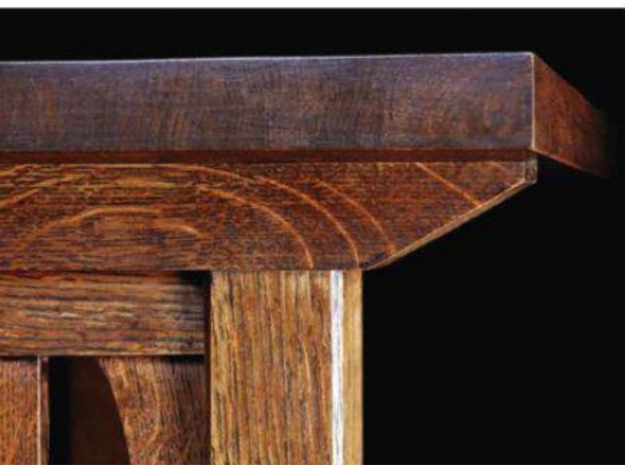
The angled end of the beams were formed on the table saw using a simple rip fence sliding jig. The workpiece is secured to the jig with a C-clamp.
