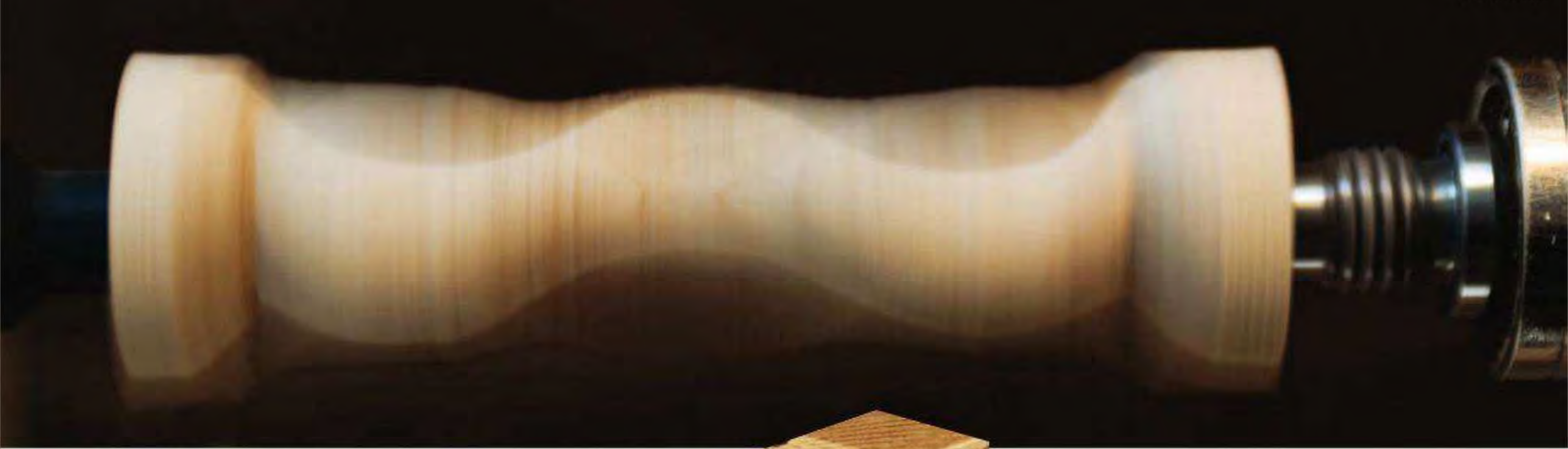
The profile of one shape appears on the lathe after Sfirri resets the centers to turn a second shape.
