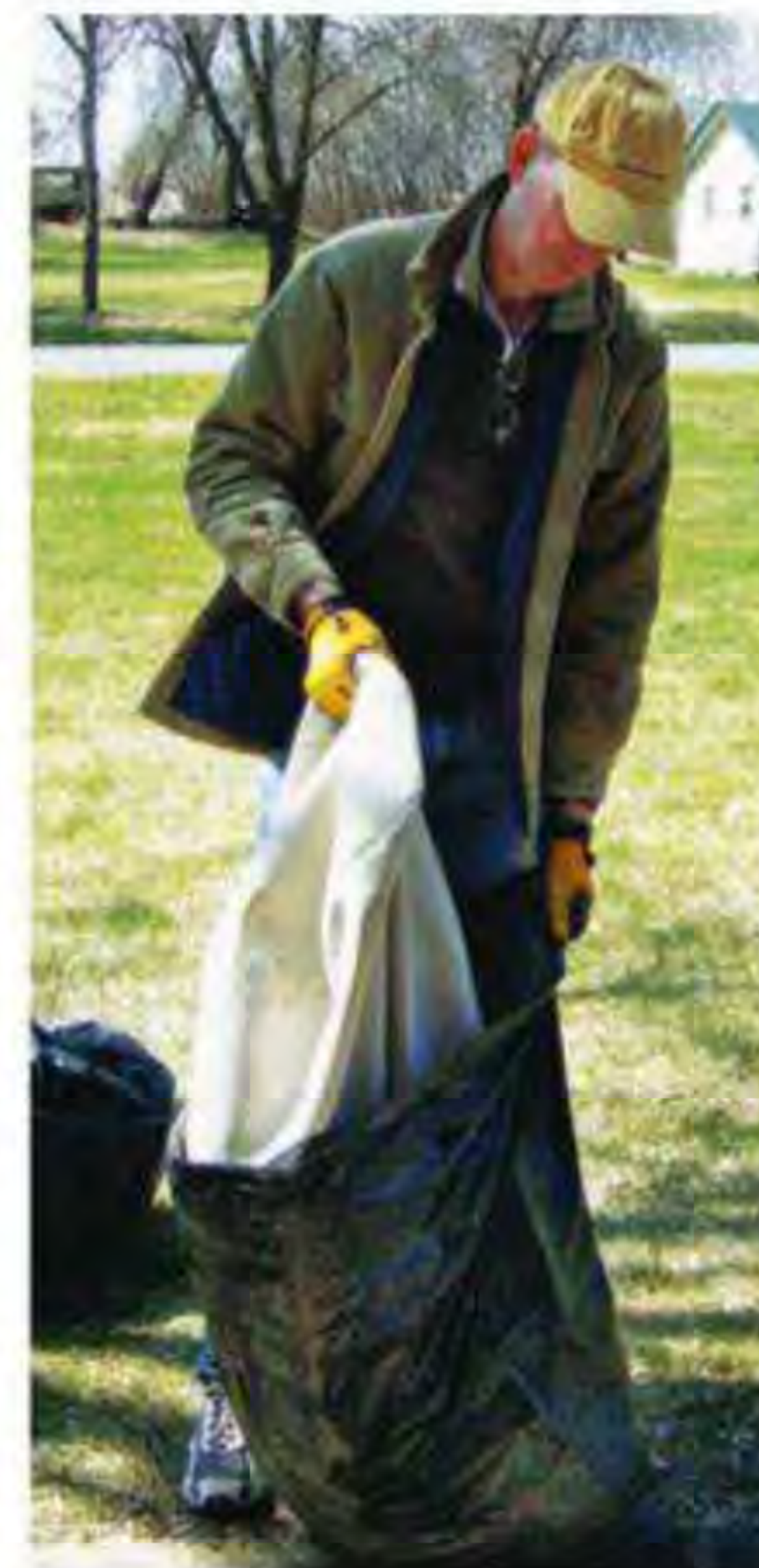
Above: Vigorously shaking out a dust collector bag might, our expert warns, eliminate its "healthy cake." It's best to gently empty and shake the bag into a trash bag (right) and call it a day.
