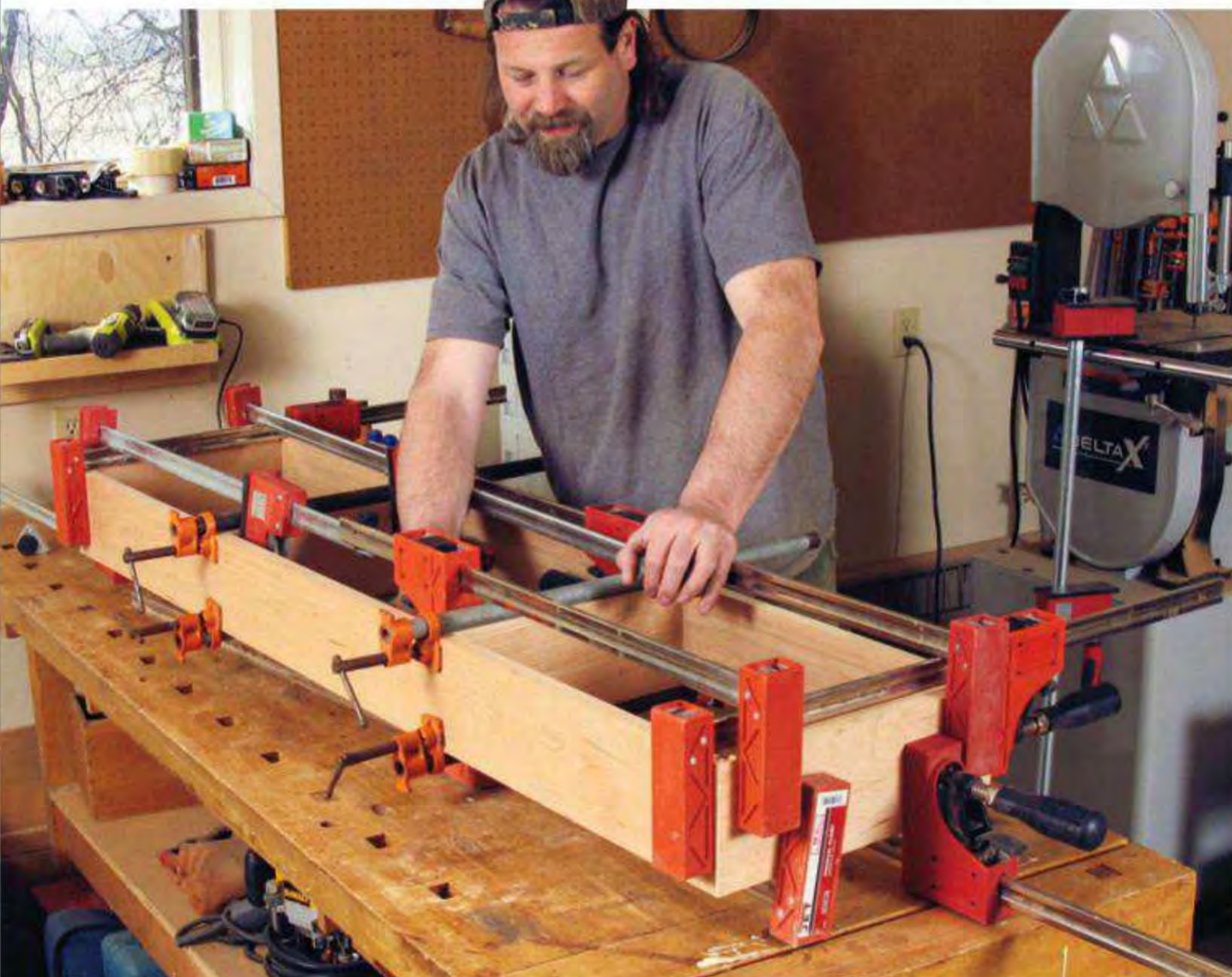
The plinth (or base) is the first subassembly. It needs to support a lot of weight and be leveled when it is set up. Corner blocks (top photo at right) add strength to the framework, and heavy-duty levelers (bottom photo at right) make quick work of the initial setup.
