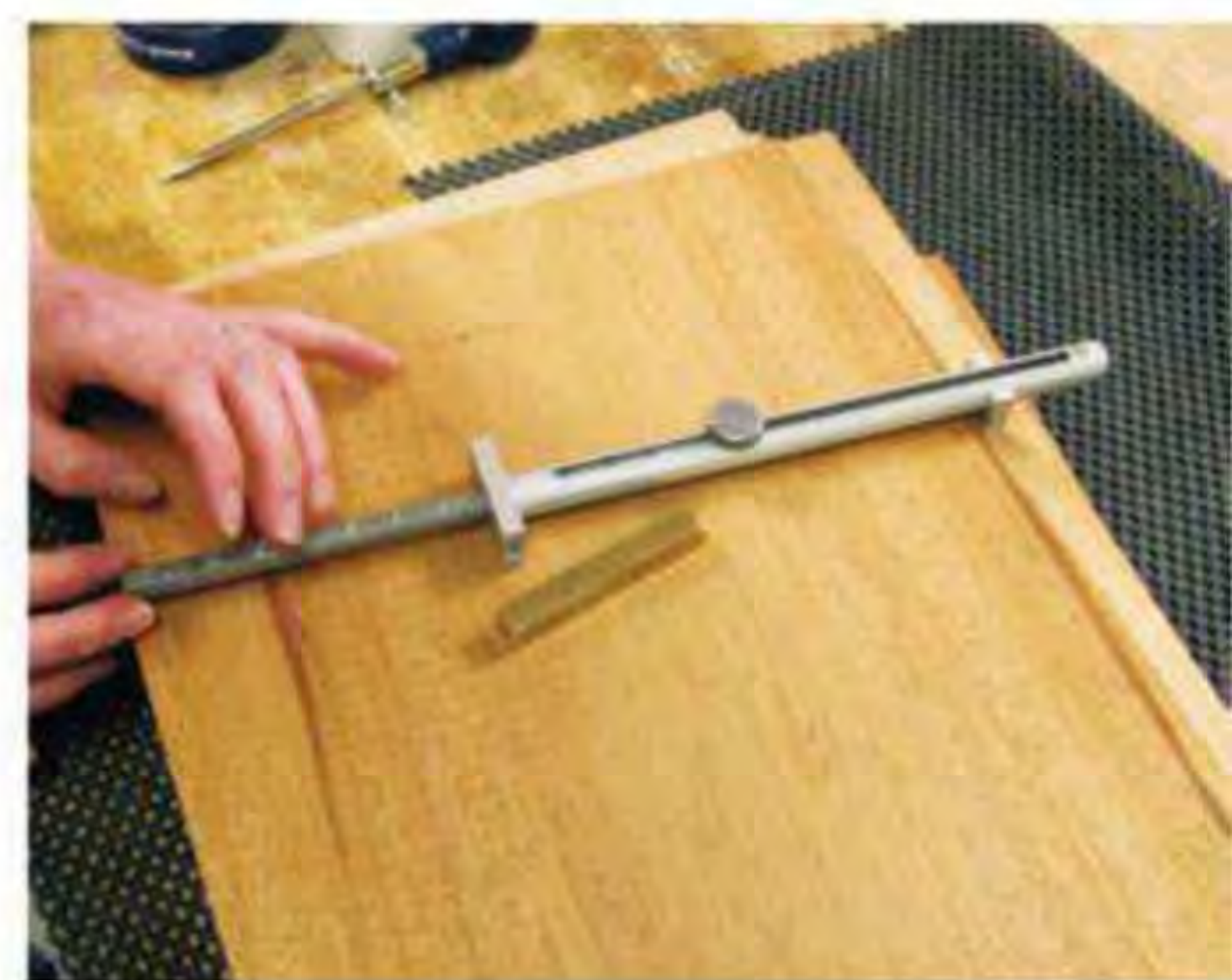
This click rule measuring device is the only specialty tool used by these blind woodworkers.
