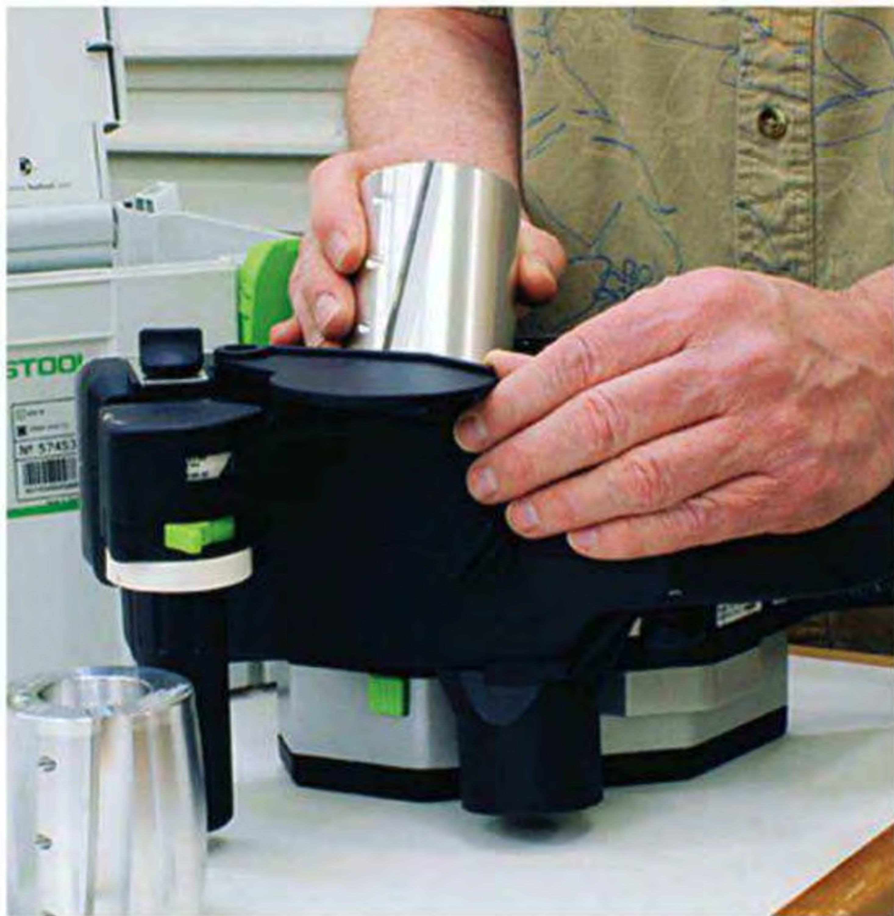
Some high-end planers, like the Festool HL850E, offer quick-change optional heads for specific types of “molding” cuts.
