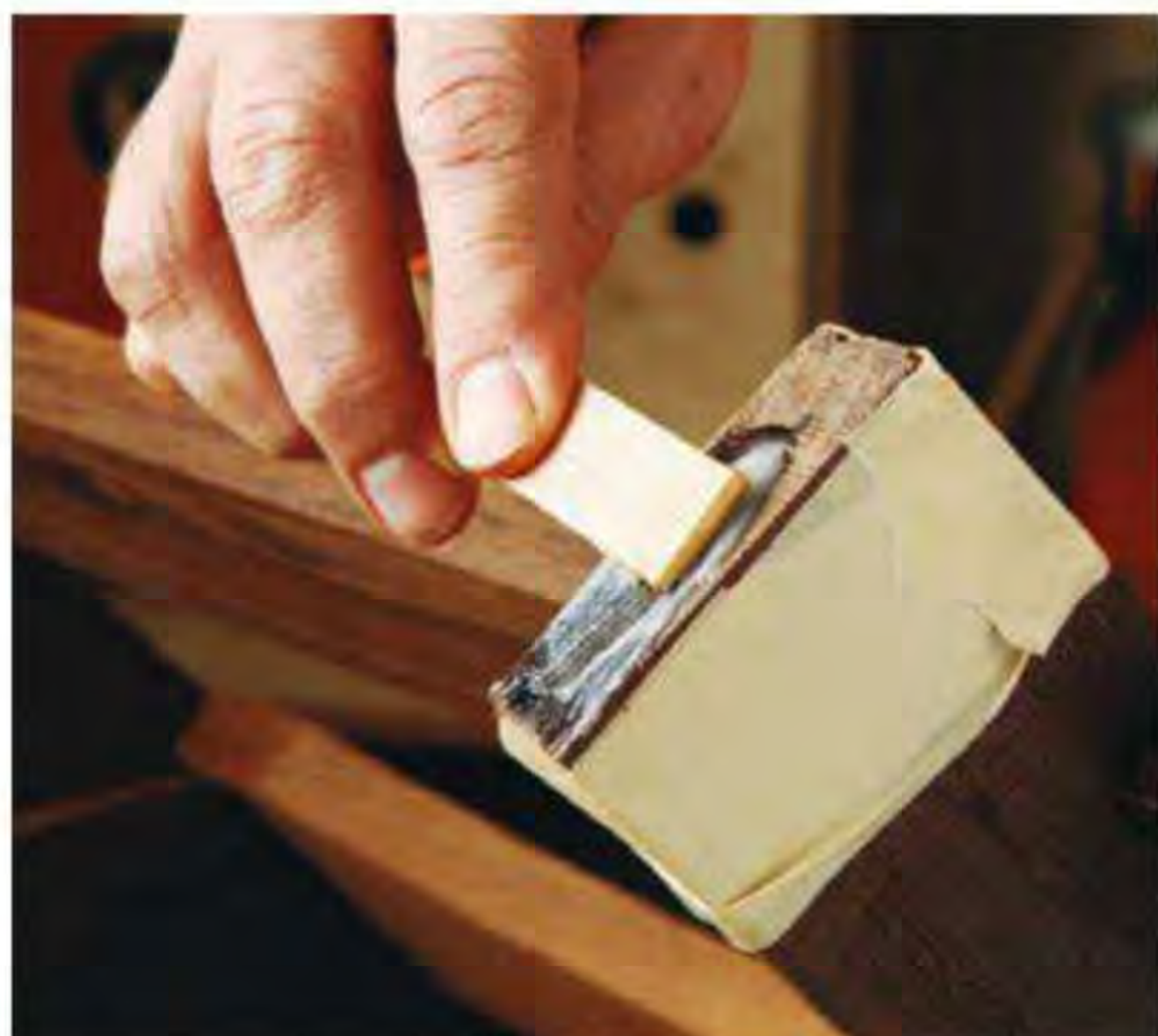
Using an epoxy with a long open time allows the resin to "soak" into the wood fibers. Here the epoxy is being applied to the "Westport Chair" featured on page 44.
