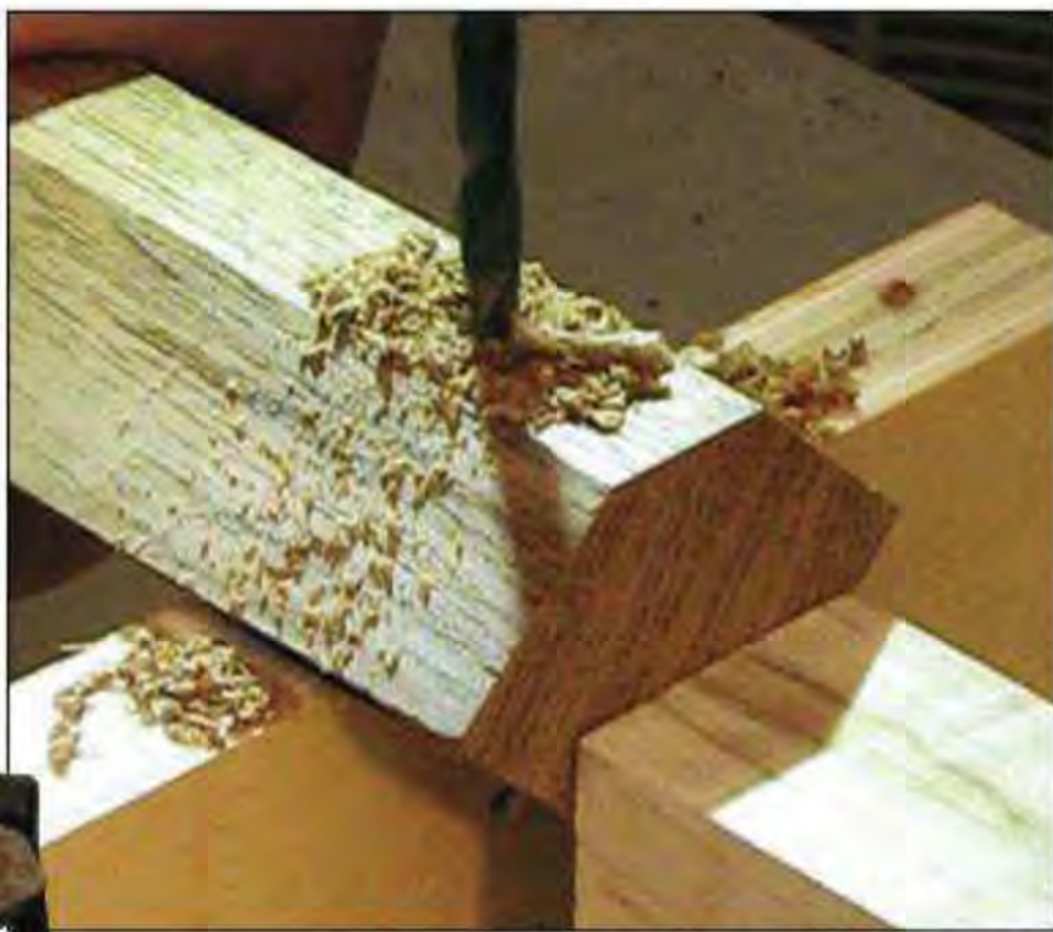
A shop-made cradle jig with a registration stop will help to ensure that the screws and countersinks are perfectly positioned and drilled.
