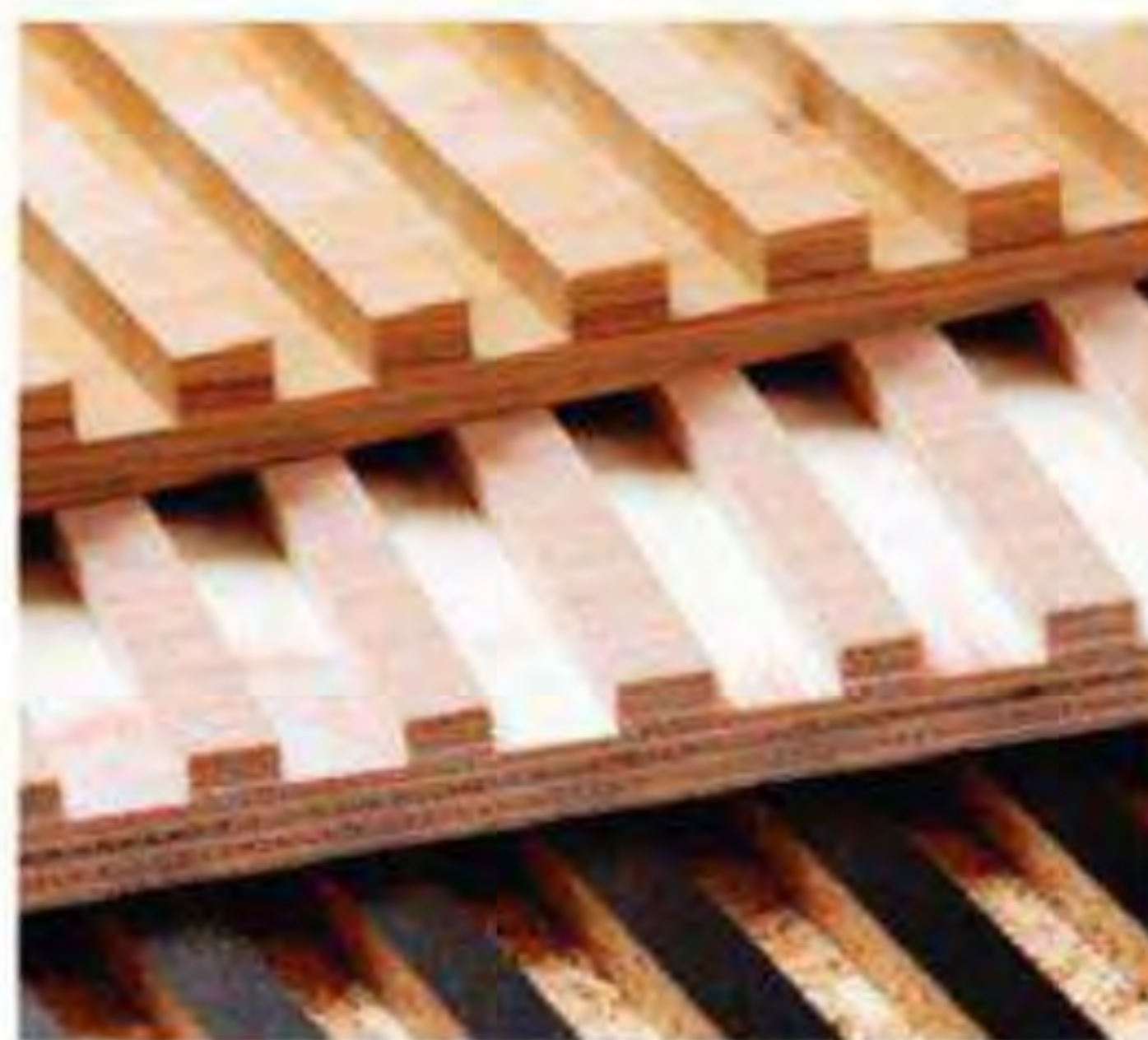
Clean-edged, flat-bottomed dados were the standard to meet here, in various chip- and splinter-prone materials. A low raking light (below) highlighted any defects in the test cuts.
