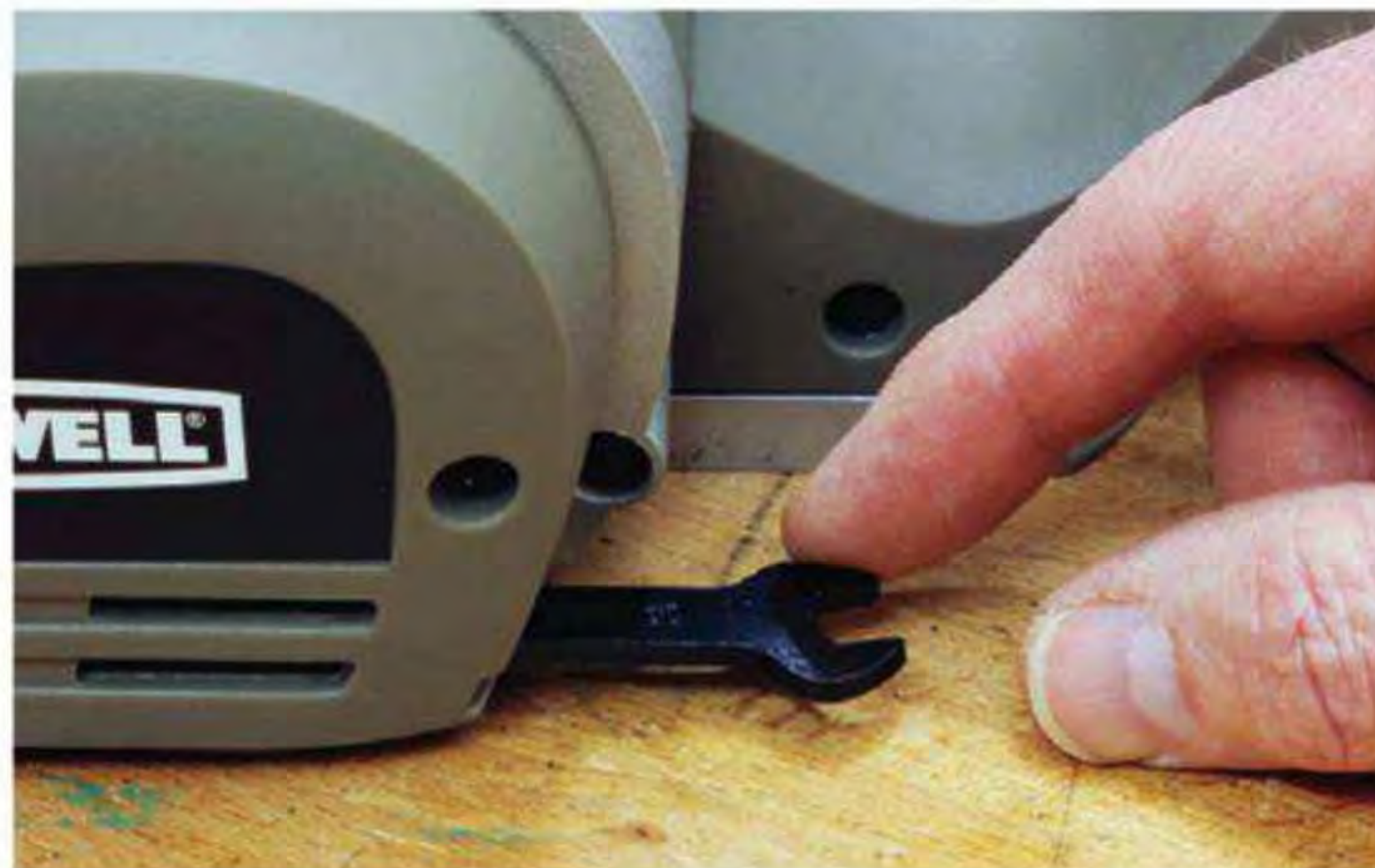
Being able to store necessary tools on the planer itself, as on the Rockwell RK5259K, is a handy feature to look for.
