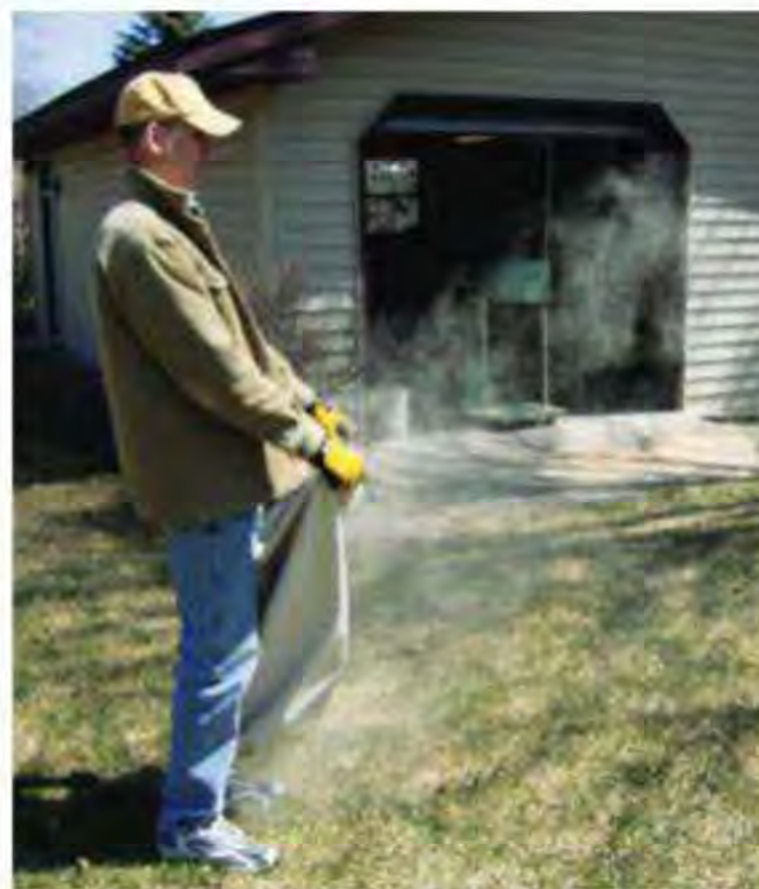
Above: Vigorously shaking out a dust collector bag might, our expert warns, eliminate its "healthy cake." It's best to gently empty and shake the bag into a trash bag (right) and call it a day.
