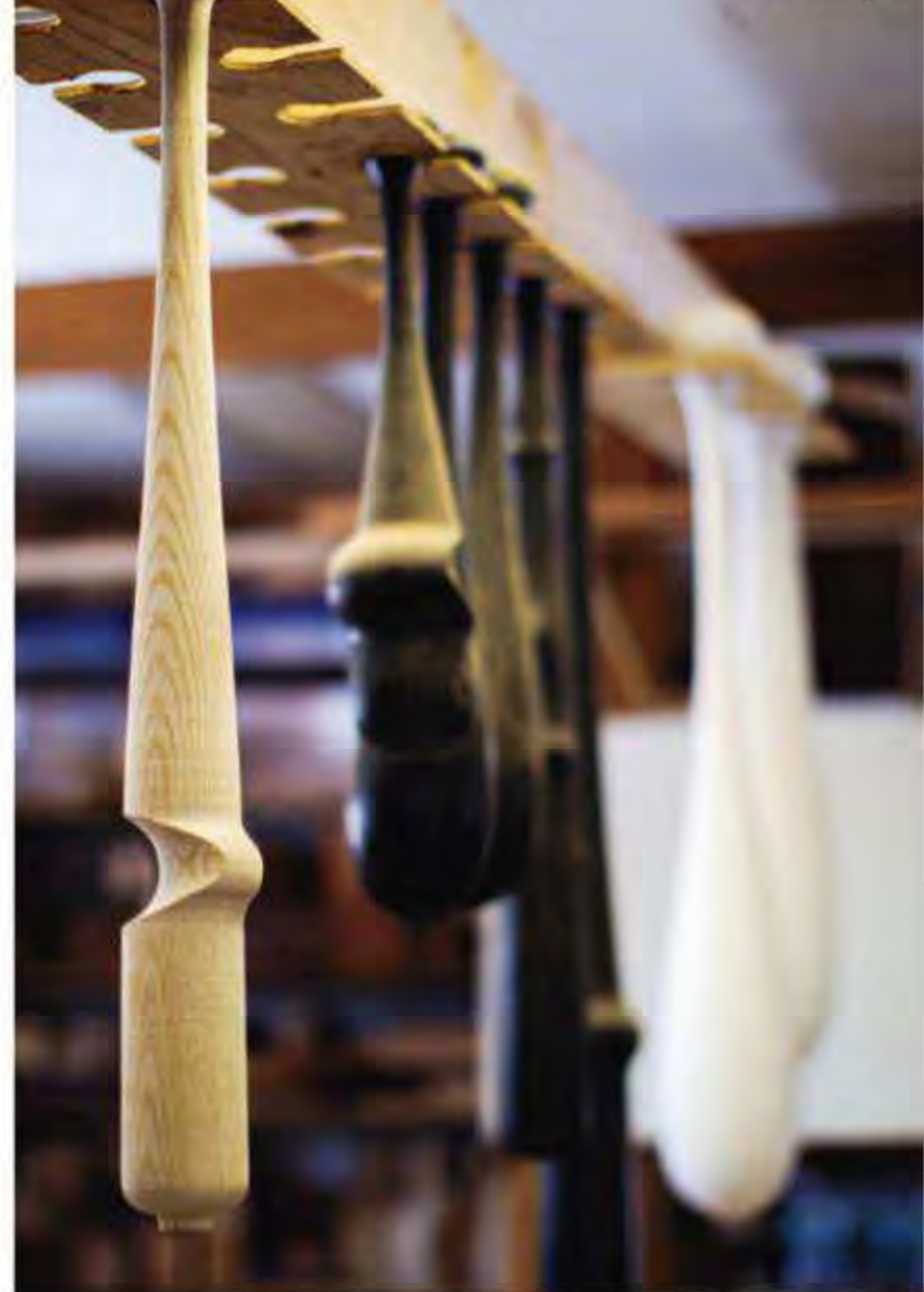
Samples from Rejects from the Bat Factory hang near Sfirri's table saw. Samples help him lay out centers of pieces he wants to recreate.
