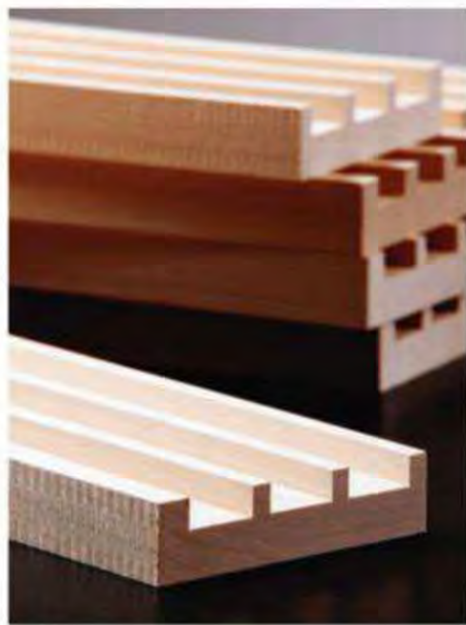
Clean-edged, flat-bottomed dados were the standard to meet here, in various chip- and splinter-prone materials. A low raking light (below) highlighted any defects in the test cuts.
