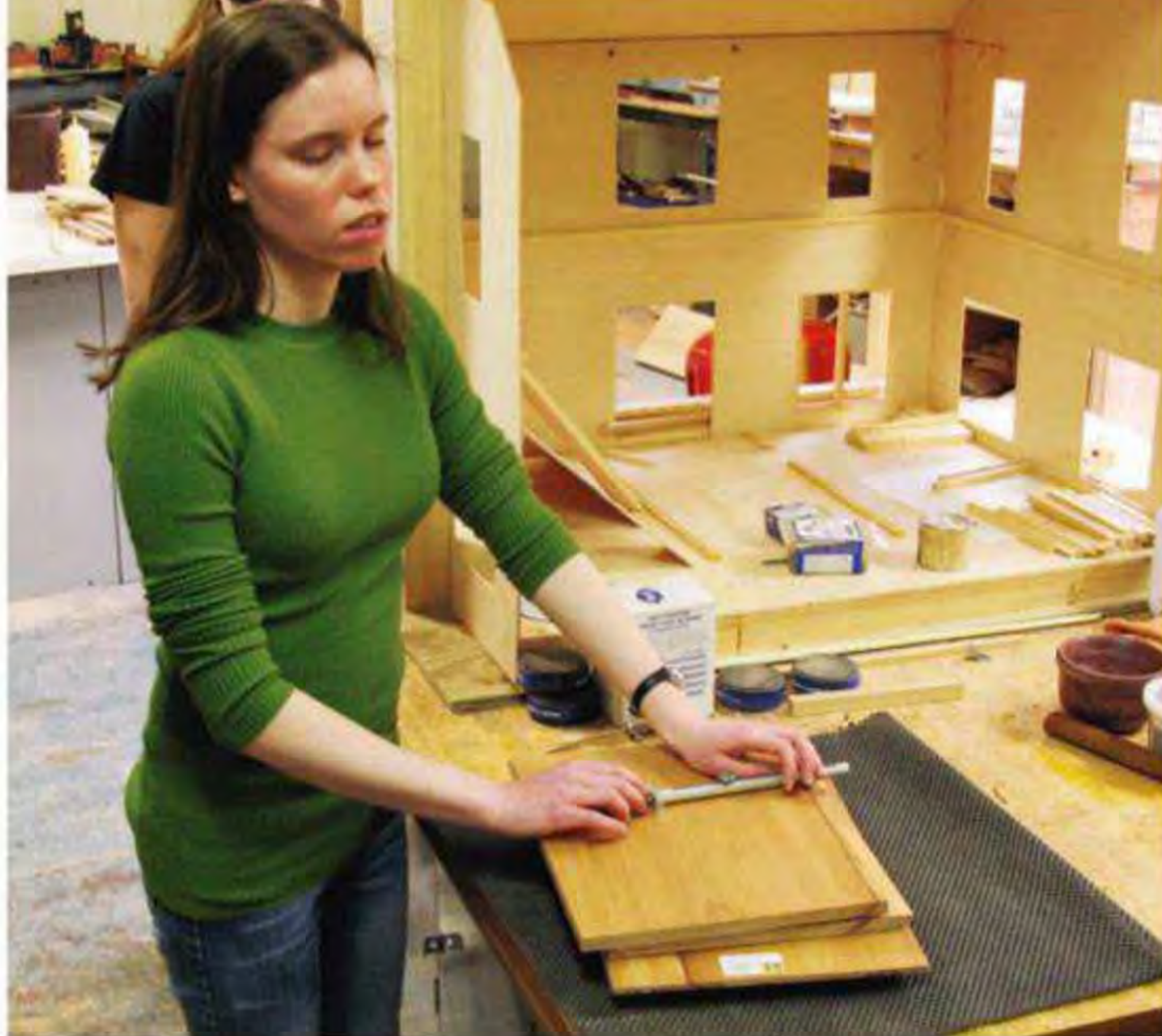
This click rule measuring device is the only specialty tool used by these blind woodworkers.
