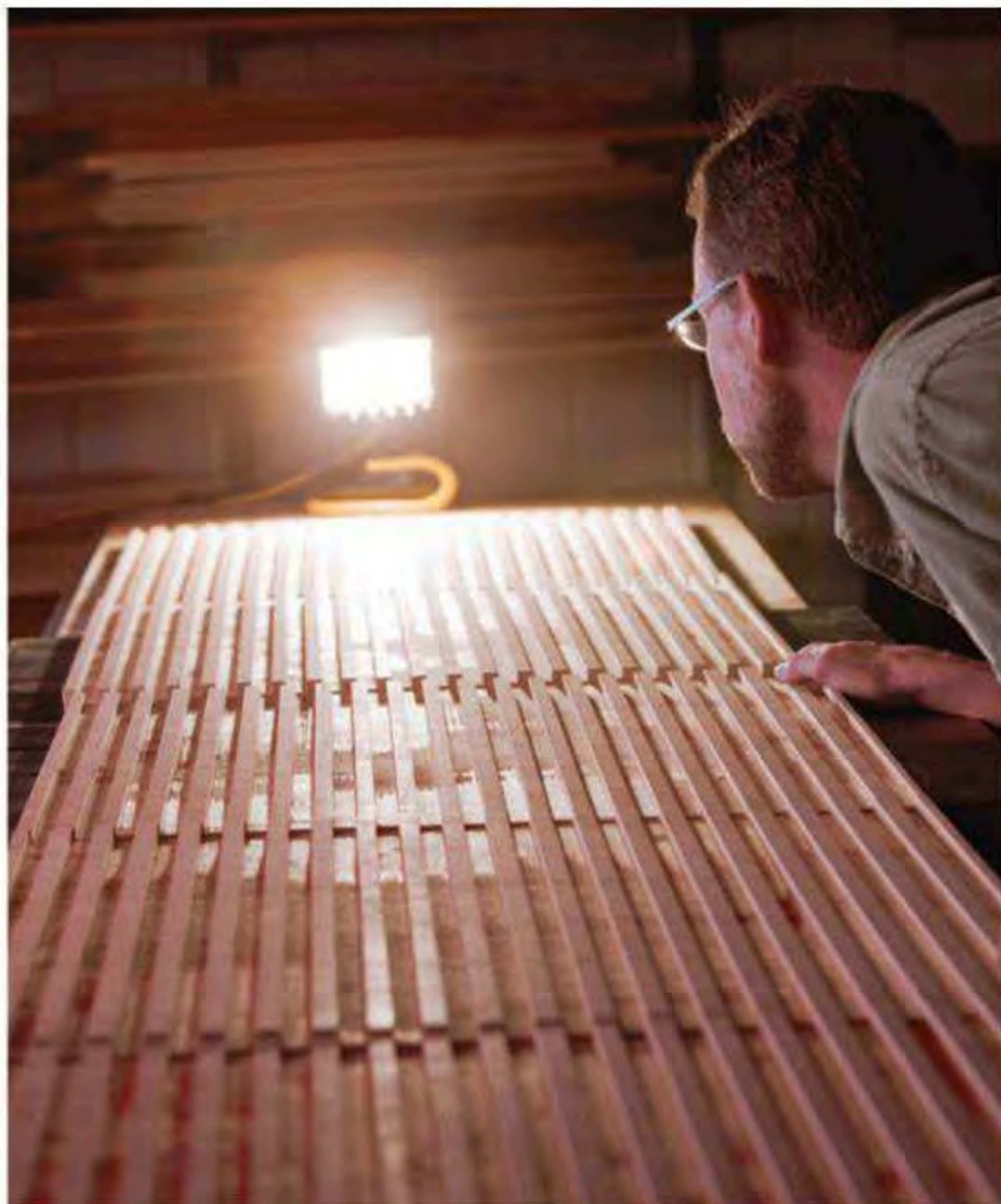
Clean-edged, flat-bottomed dados were the standard to meet here, in various chip- and splinter-prone materials. A low raking light (below) highlighted any defects in the test cuts.
