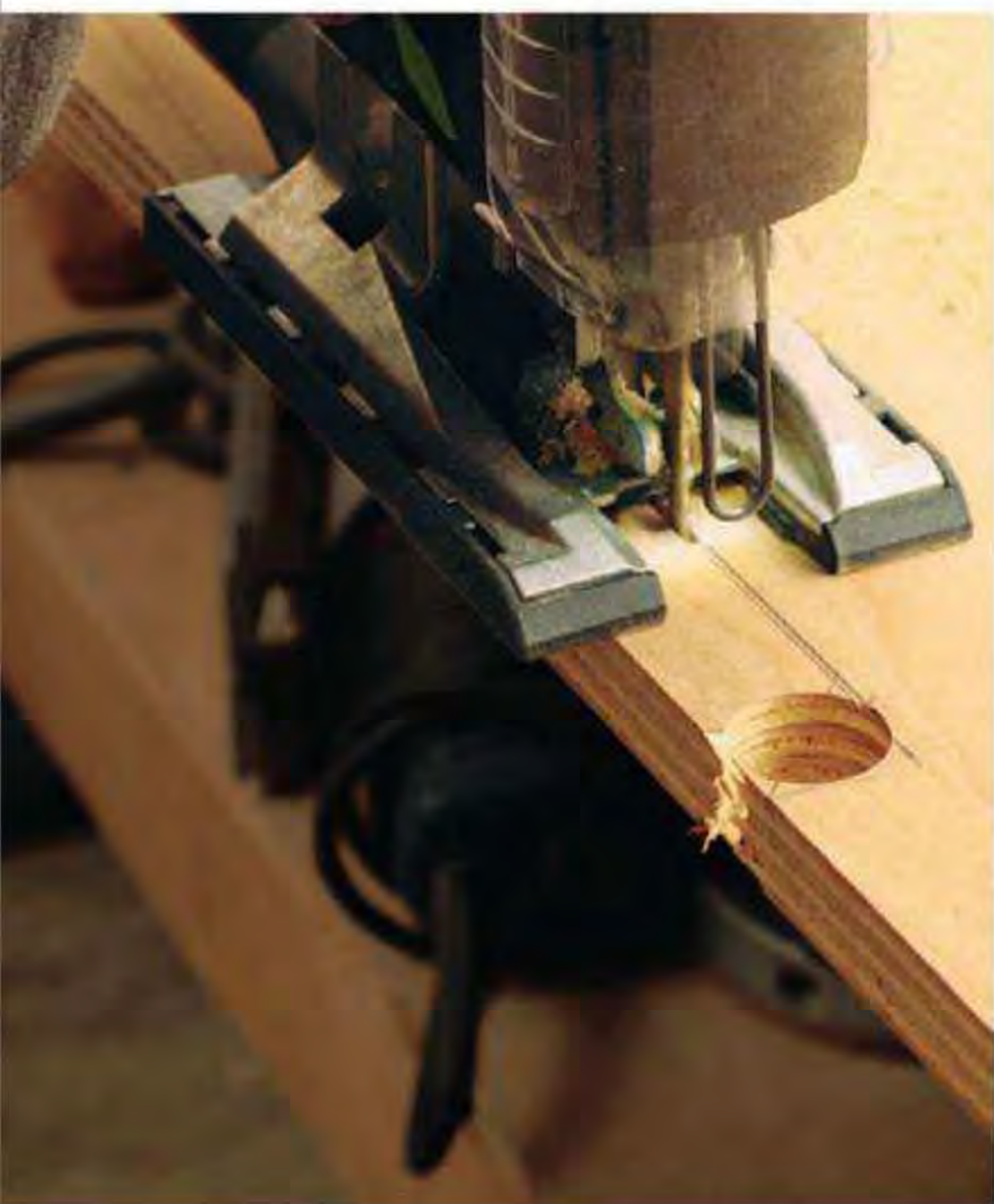
A notch on the back of the carcass bottom allows an array of wiring access to the center console and out past the cabinet.
