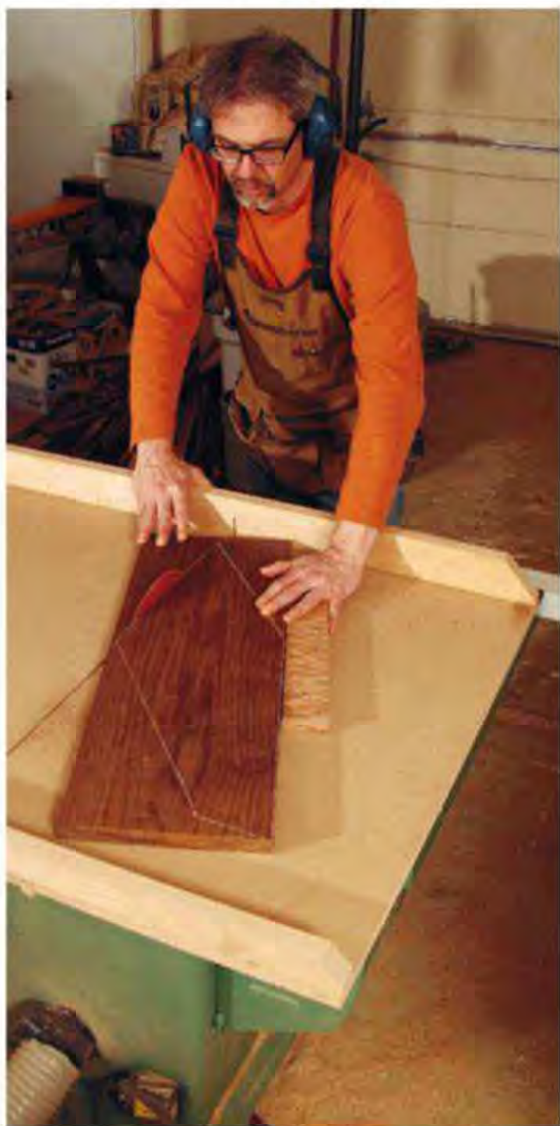
To form the trapezoidal shape of the rear legs, the author used a table saw sled. He lined up the cuts and then screwed a moveable fence to the sled. The shape was first traced onto the workpiece from a template.
