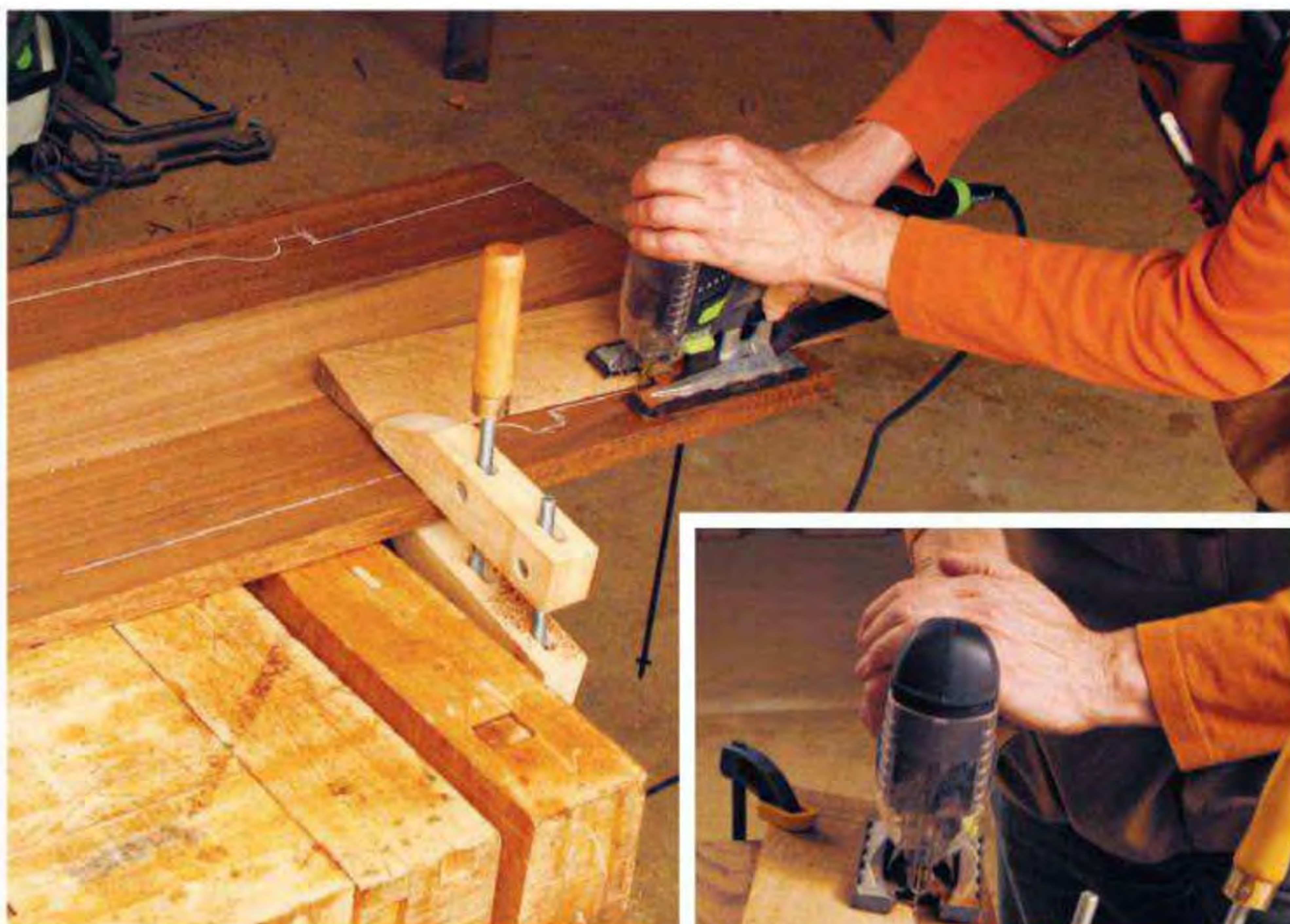
The symmetrical taper at the bottom of the back also has a 12° angle across its thickness. A ramp cut to the proper angle was clamped in place and used to form both angles in a single cut.
