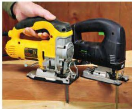
Our author prefers wider triggers for comfort and for shifting hand positions.
