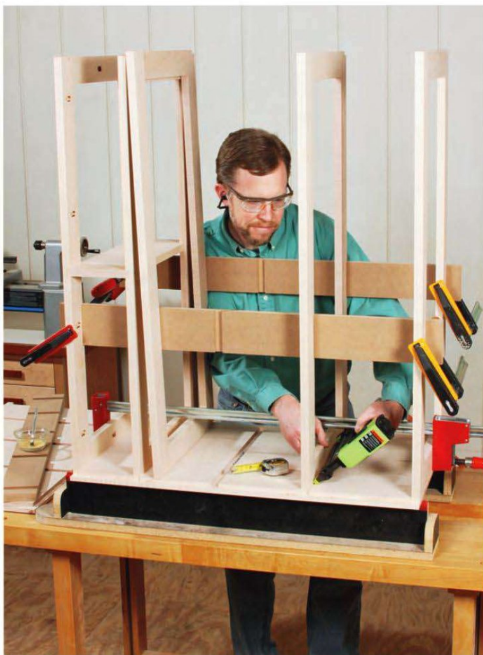
Assembling the carcass involved fixing the web frames into their side-panel dados with a short bead of glue and several brads driven diagonally across the joints. Scrap MDF braces outfitted with dados held the frames square to the side panel and parallel to one another during this process.
