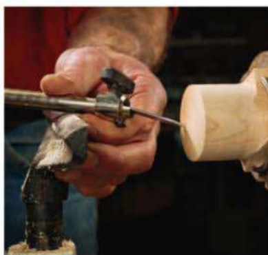
The tool-rest has to be set farther from the work than usual, giving the cutter a chance to flex and "chatter."
