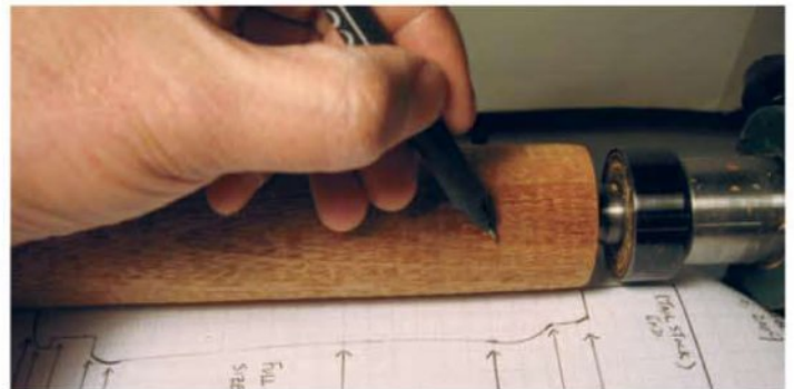
Figure 3: Scribe a circle at each contour point.
