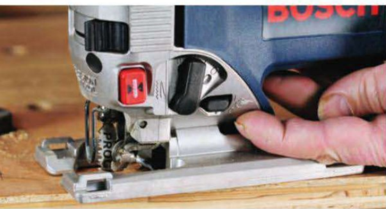
The Bosch saw has an On/Off switch for its dust blower — unique among the tools reviewed here. Only the three least expensive saws have an LED light to help illuminate the line of cut.
