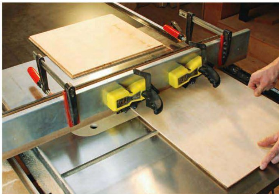
Thick drawer bottoms prepare these drawers for heavy use, but they must be rabbeted on three sides to fit the drawer bottom grooves. Magnetic featherboards ensured consistently thick tongues.
