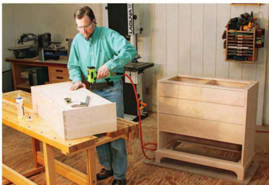
While the design of these drawers was straightforward and conventional, their accuracy and squareness was crucial in order to fit properly inside the dresser's tight tolerances.
