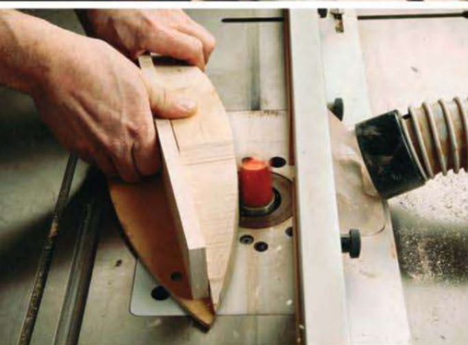
Using carpet (double-faced) tape to secure the leg blanks to the template, the author carefully shapes and smooths the curved faces of the legs with a pattern-routing bit.
