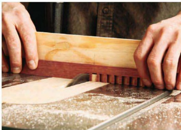
The exacting task of forming the interlocking notches in the long and short lattice requires significant attention to detail ... even to the point of holding your hands in the same position for each cut.
