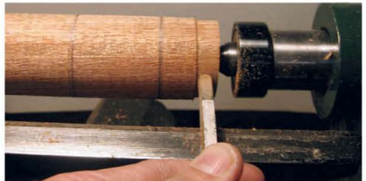
Figure 4: Cut the tenon to size.
