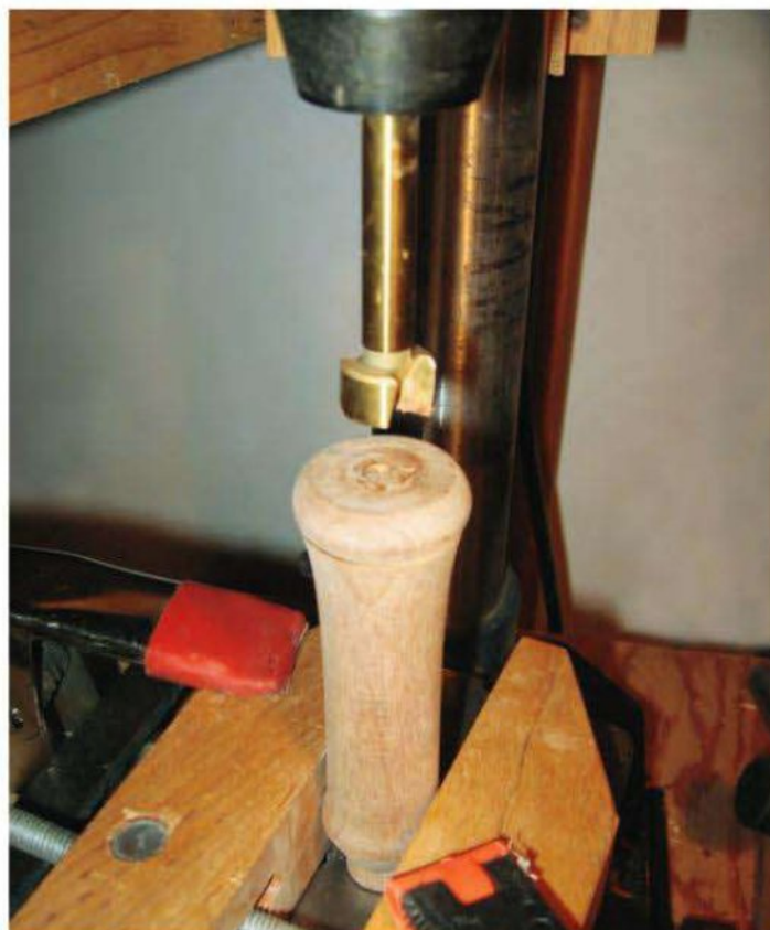
Figure 9: Hollow the handle to create the screwdriver bit compartment.
