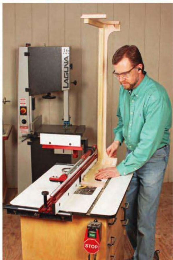
Once the cleats and glue blocks are in place, you can rout the cove profiles around the upper edges of the base at the router table (right). The assembly is tall, but it's still lightweight and easy to control. Fasten the base to the carcass by driving screws up through the base cleats (below), then add blocking to reinforce the back feet.
