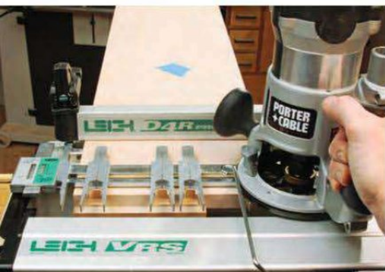
Flipping the finger template over on the jig resets it for cutting sockets and pins in the drawer faces with the same bit and setting.
