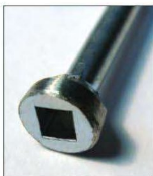
Figure 12: Grind the head of the #6 x 2 1/2" screw down to about 3/16" diameter.
