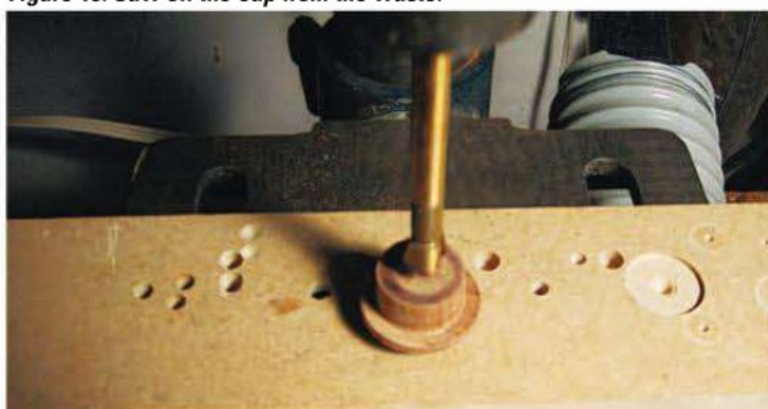
Figure 11: Drill a shallow hole on the underside of the cap for a magnet.
