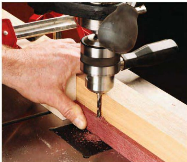
The purpleheart lattice is attached to the aprons with small dowels. Drill the holes, using a drill press for best results, while the stock is stuck-up rather than after it has been shaped on the band saw.
