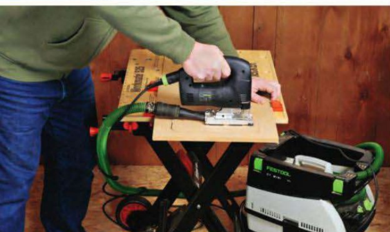
Some of the saws in this test allow tool-less footplate angle adjustments, while others require an Allen wrench (top photo). Chip extractor fittings (bottom photo) are provided as a standard feature only on the Metabo, Bosch and Festool — the most expensive tools in this review.
