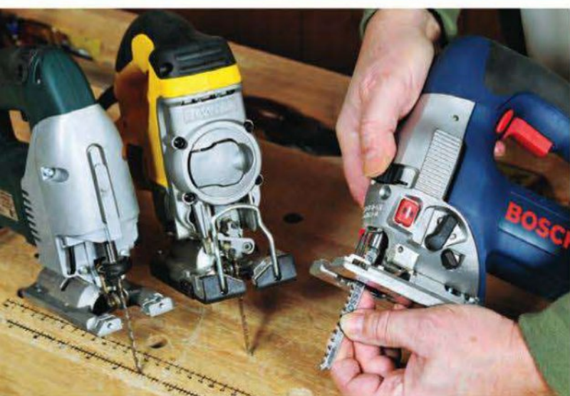
The Festool and Bosch saws (above) are the only models to feature blade guide systems, similar in concept to those on band saws. Below, tool-less blade change mechanisms are standard on all seven jigsaws.
