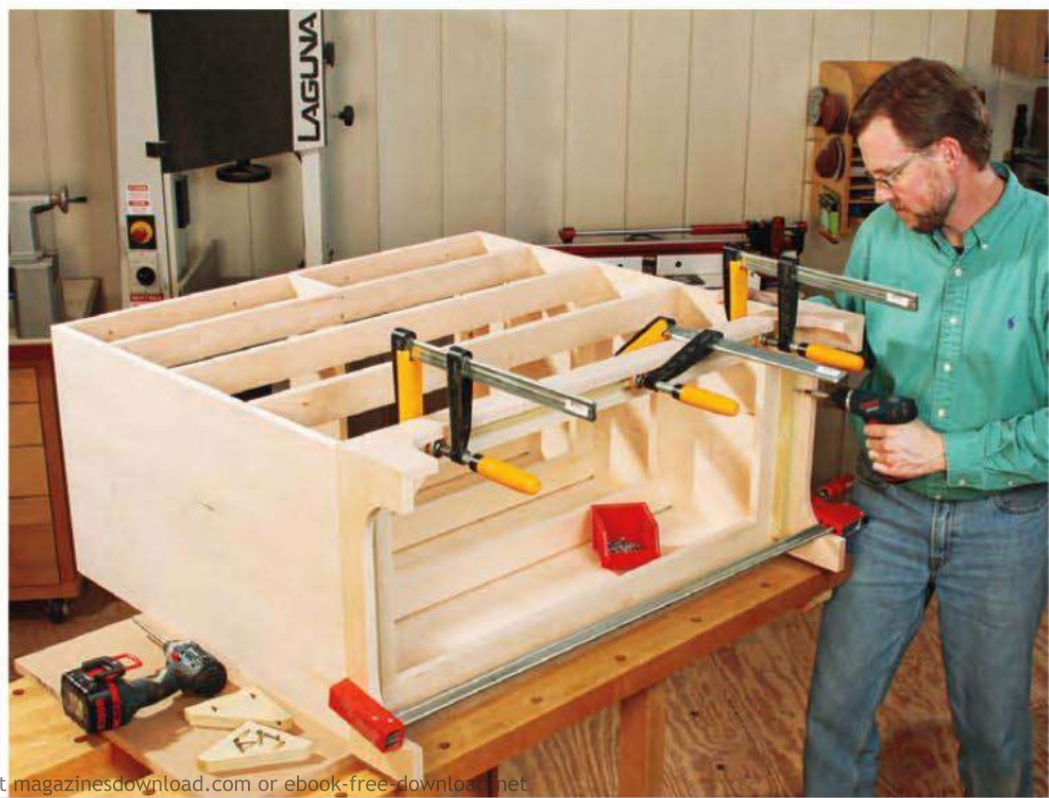
Once the cleats and glue blocks are in place, you can rout the cove profiles around the upper edges of the base at the router table (right). The assembly is tall, but it's still lightweight and easy to control. Fasten the base to the carcass by driving screws up through the base cleats (below), then add blocking to reinforce the back feet.
