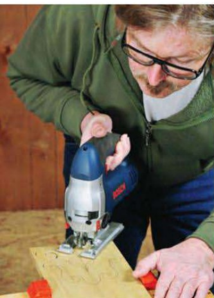
Good visibility is an important attribute of a jigsaw when cutting intricate scroll patterns.
