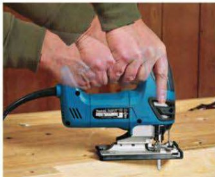
A longer handle allows for different grips suitable for a variety of cutting situations.
