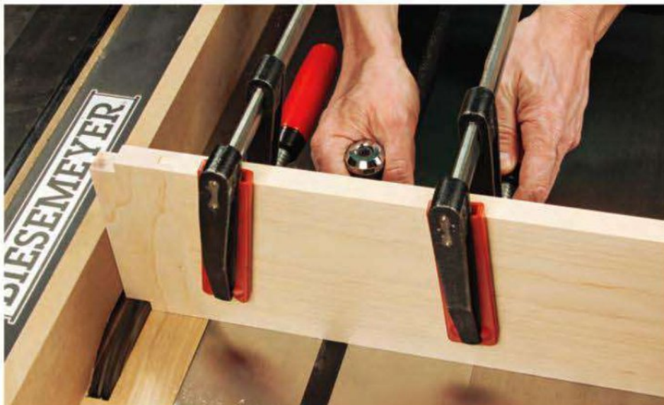
The two-piece drawer divider features a tongue and groove joint. After assembling it, you need to nibble away the front corners to fit this piece into and around the web frame dados.
