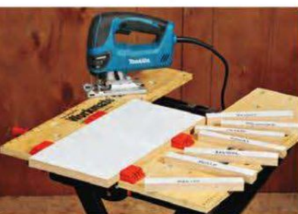
The author tested how well the saws cut melamine, a material that tends to chip easily.
