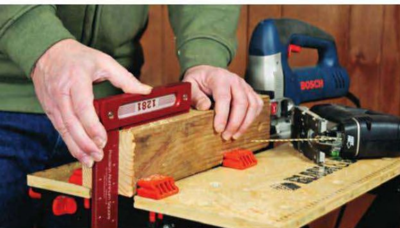
The blade guide systems on the Festool and Bosch helped keep their blades square and true when cutting thick wood.
