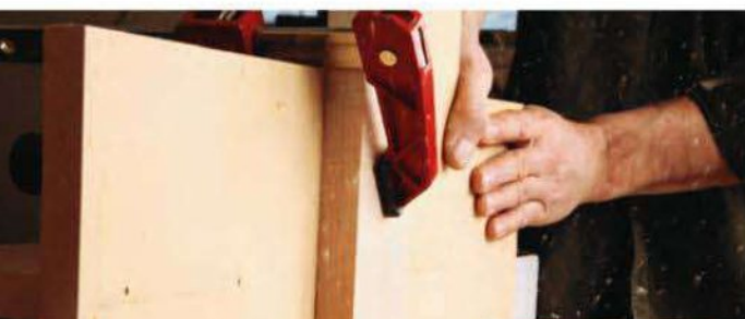
Using carpet (double-faced) tape to secure the leg blanks to the template, the author carefully shapes and smooths the curved faces of the legs with a pattern-routing bit.
