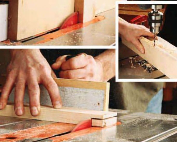
Bare-faced tenons join the aprons to the legs. With the tenons cut, the author bored a series of holes in the edges of the aprons for securing the lattice (inset).
