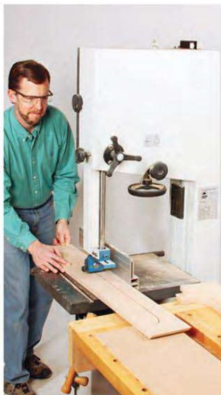
The author recommends miter-cutting the base sides and front piece first to perfect these joints, then marking and cutting the curved feet to shape (above left).
