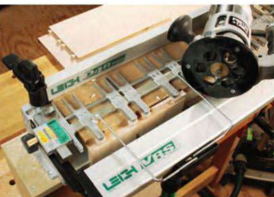
Leigh's D4R Pro Jig tackled this dresser's variable-spaced, half-blind dovetail layout on the drawers. The tail machining happens first.
