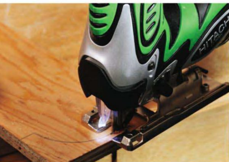
The Bosch saw has an On/Off switch for its dust blower — unique among the tools reviewed here. Only the three least expensive saws have an LED light to help illuminate the line of cut.
