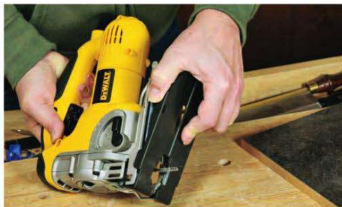
A useful accessory that comes with some jigsaws is a slick plastic cover that prevents its metal footplate from scratching the work.
