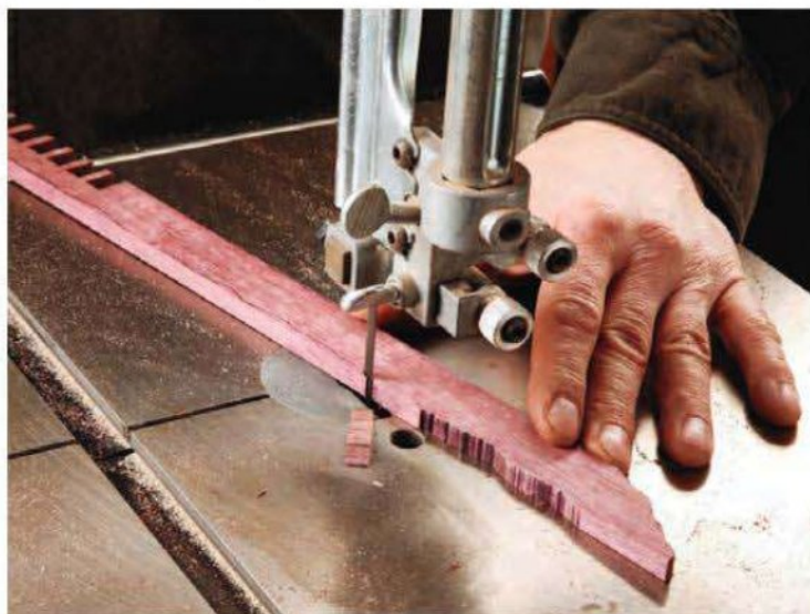
While it's not exactly a textbook use of the band saw, the author uses a 3/16" blade — cutting, scraping and carving the shape into the top edge of the lattice. Later, he smooths it some more with a cabinet card scraper.
