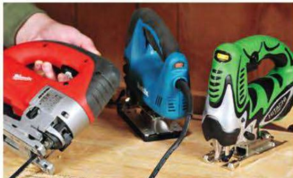
Variable-speed control is a feature common to all of the featured saws. Location of the speed dials varies.
