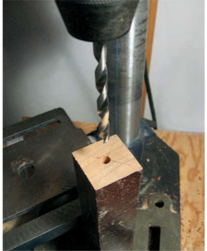
Figure 1: Drill a center hole to fit the bit holder shank.
