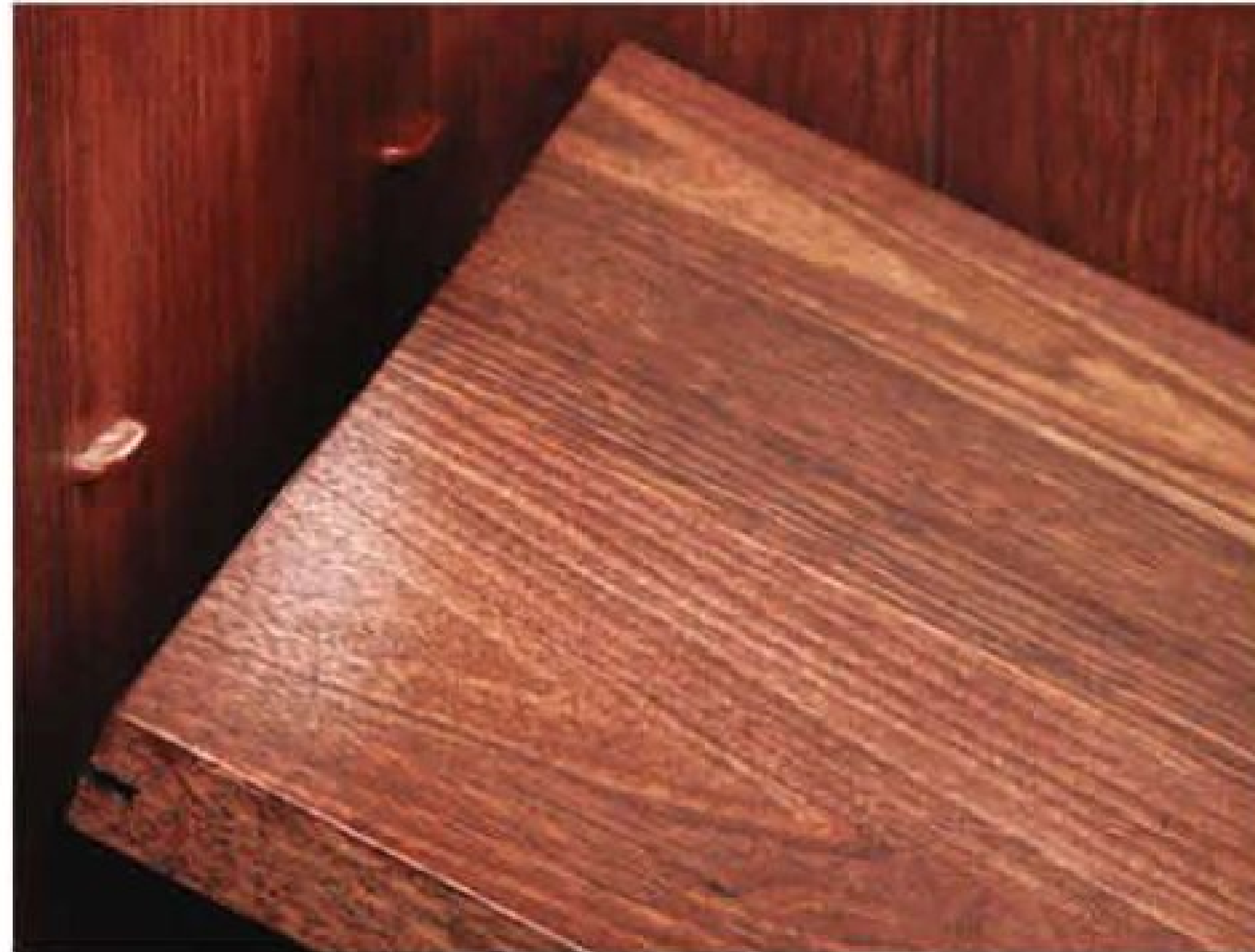
Red mahogany oil stain (left) added colorful highlights to the walnut lumber — popping the grain nicely. Above, the ends of the shelf (turned around so you can see the back) have a groove sliced into them that slides over the winged shelf pins.
