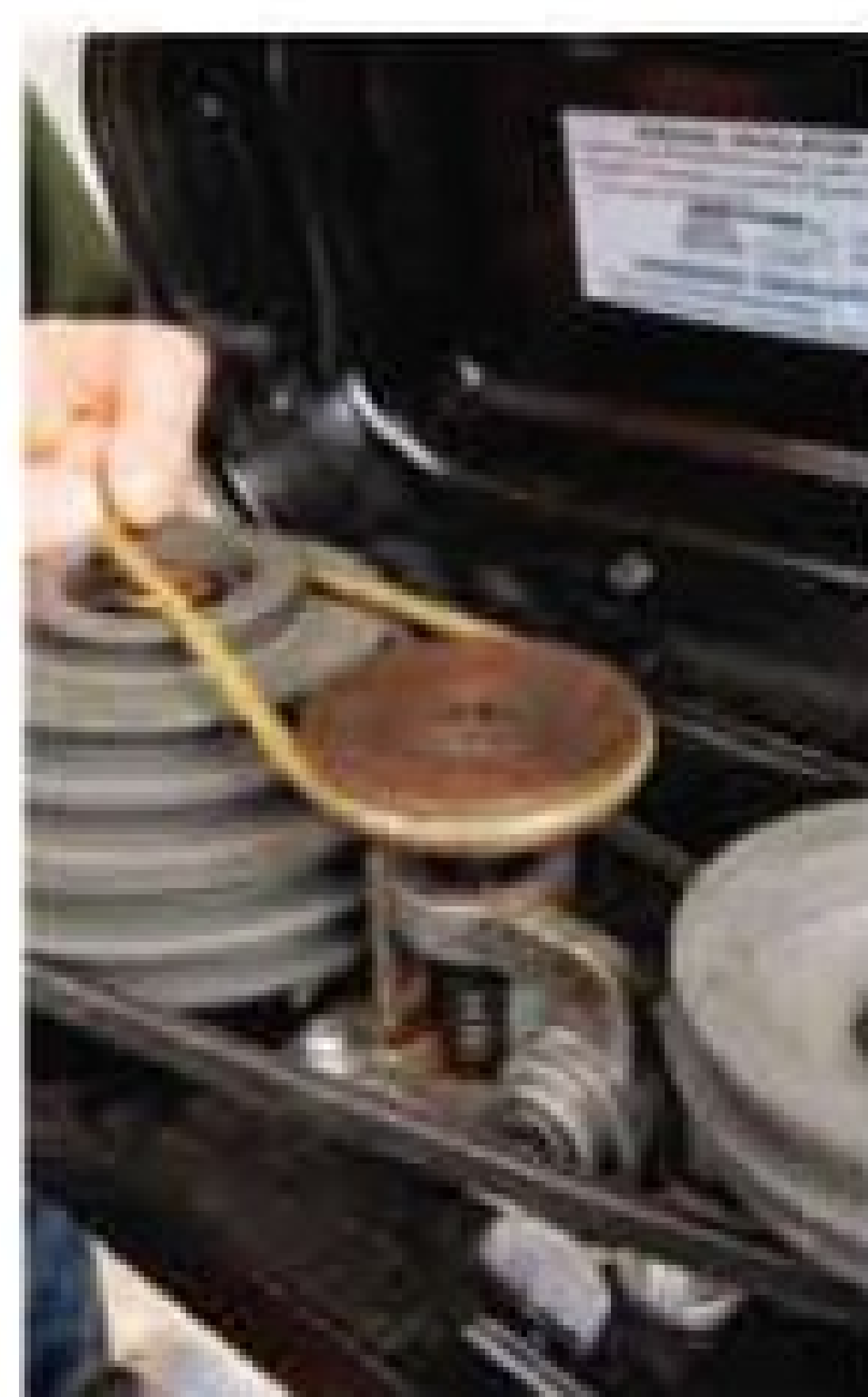
A third pulley and gear (left) changes the Shop Fox over from drilling to spindle sanding. The table has a through hole with interchangeable and variable sized insert rings for sanding drums (right).
