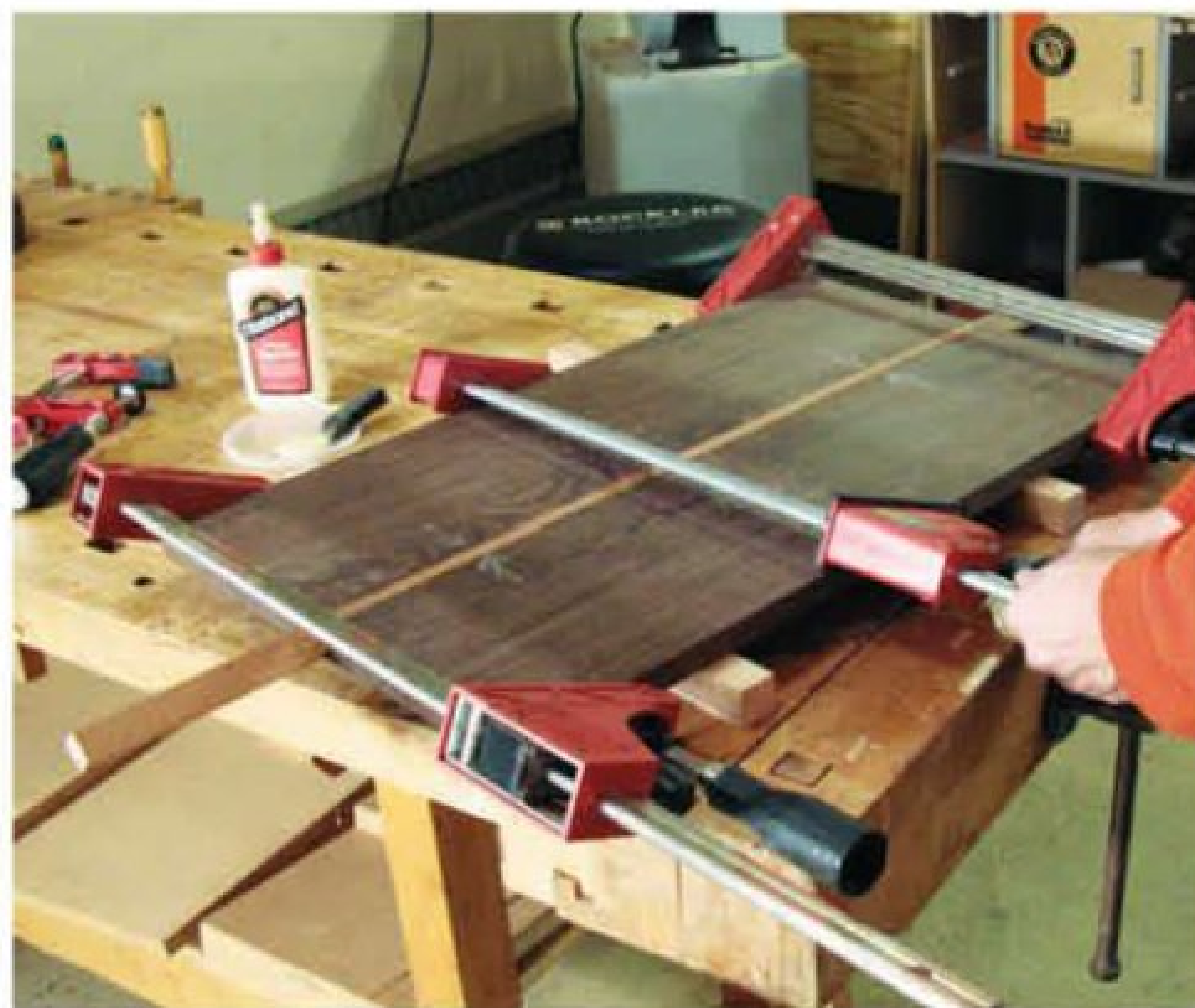
When gluing up the table top and the cherry inlay strip, it is important to keep the panels in alignment. After a test fitting, the author found that square-head clamps helped to achieve this goal.
