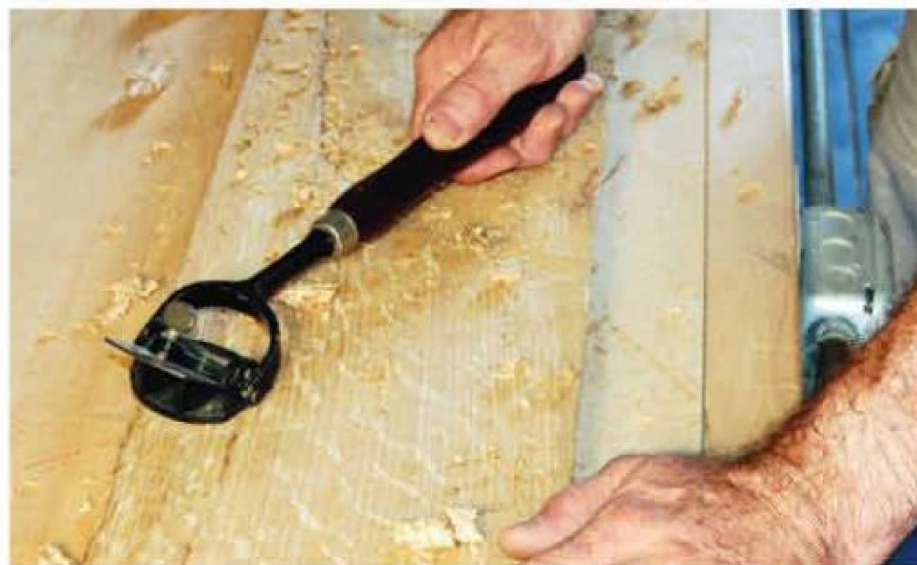
To select the best figured wood, the author used his Stanley #70 box scraper. A few pulls revealed the oak board's true color and grain.
