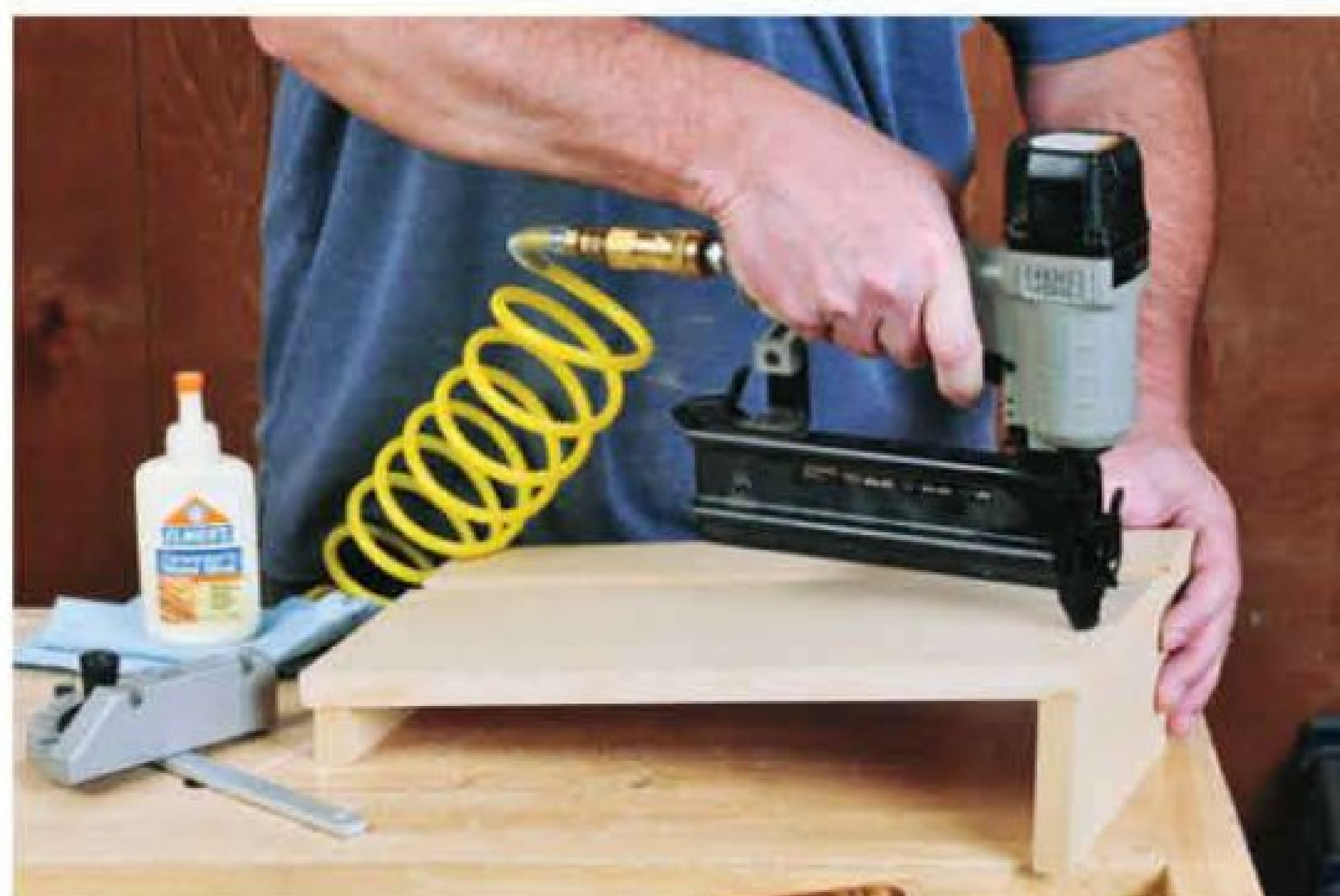
Reinforce the glued-up parts for the fixture's table together with a brad nailer. The angled table helps keep small parts put during sanding.
