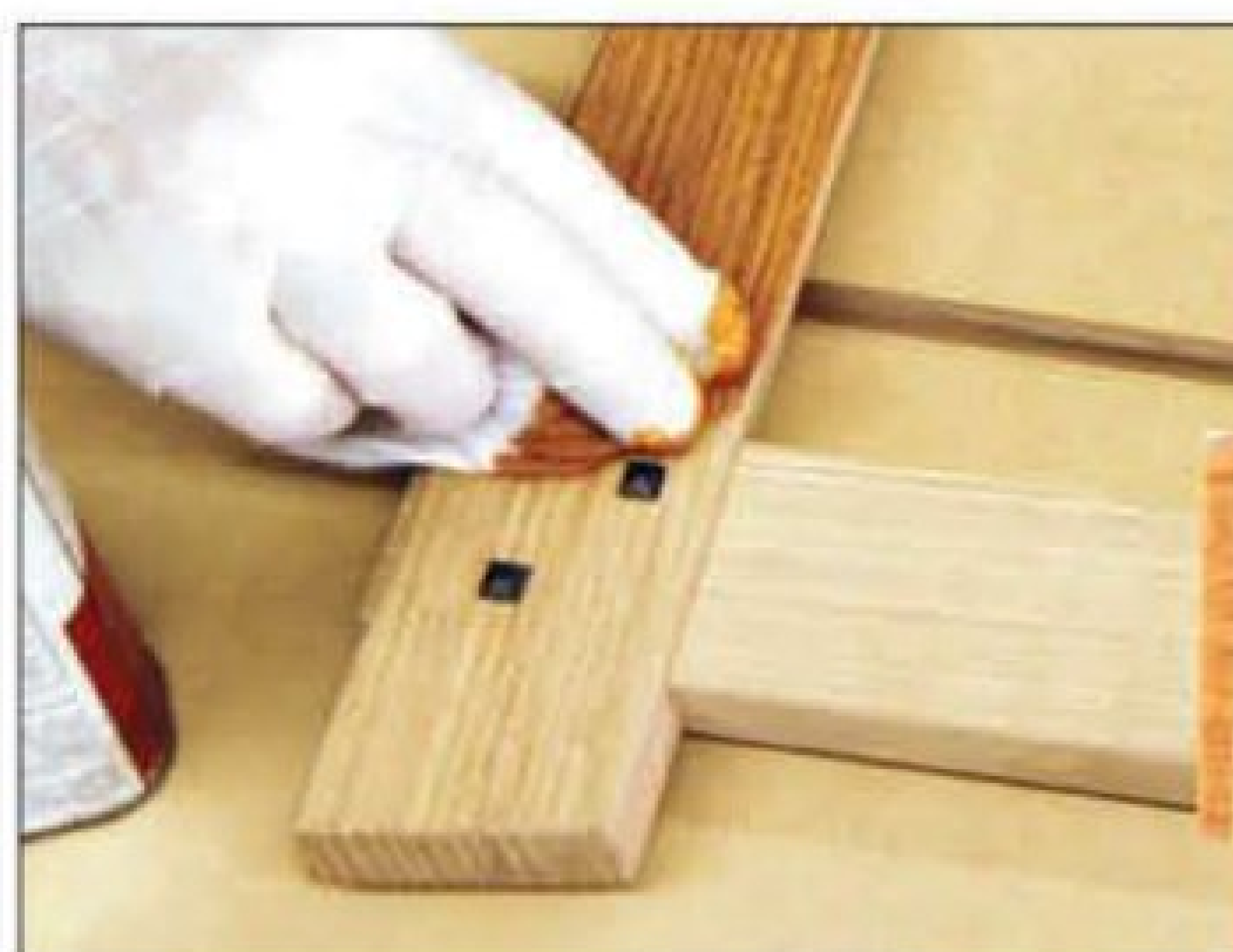
Oil stain was applied to the frame with a soft cloth, followed by lacquer topcoats.
