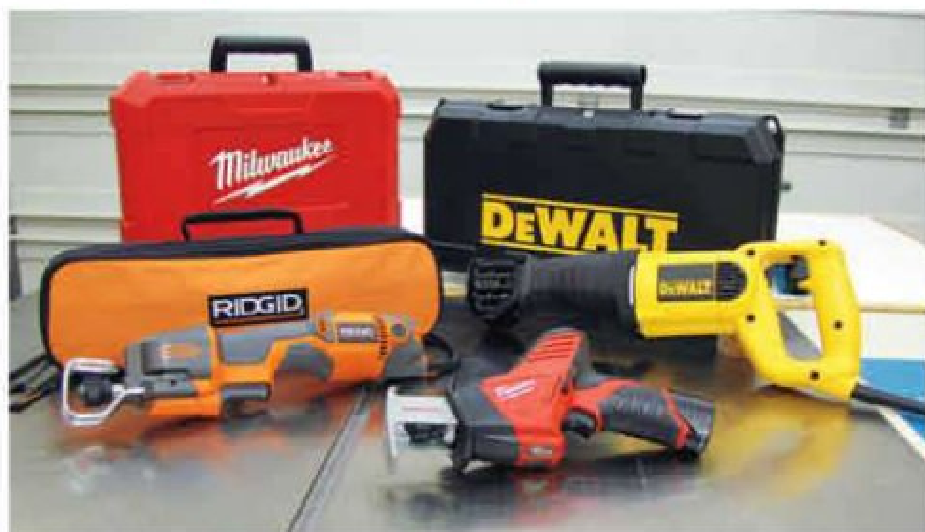
No matter what kind of job you have, there's a recip saw sized to match. Shown here are the full-size DeWALT, RIDGID Fuego compact and Milwaukee's Hackzall.
