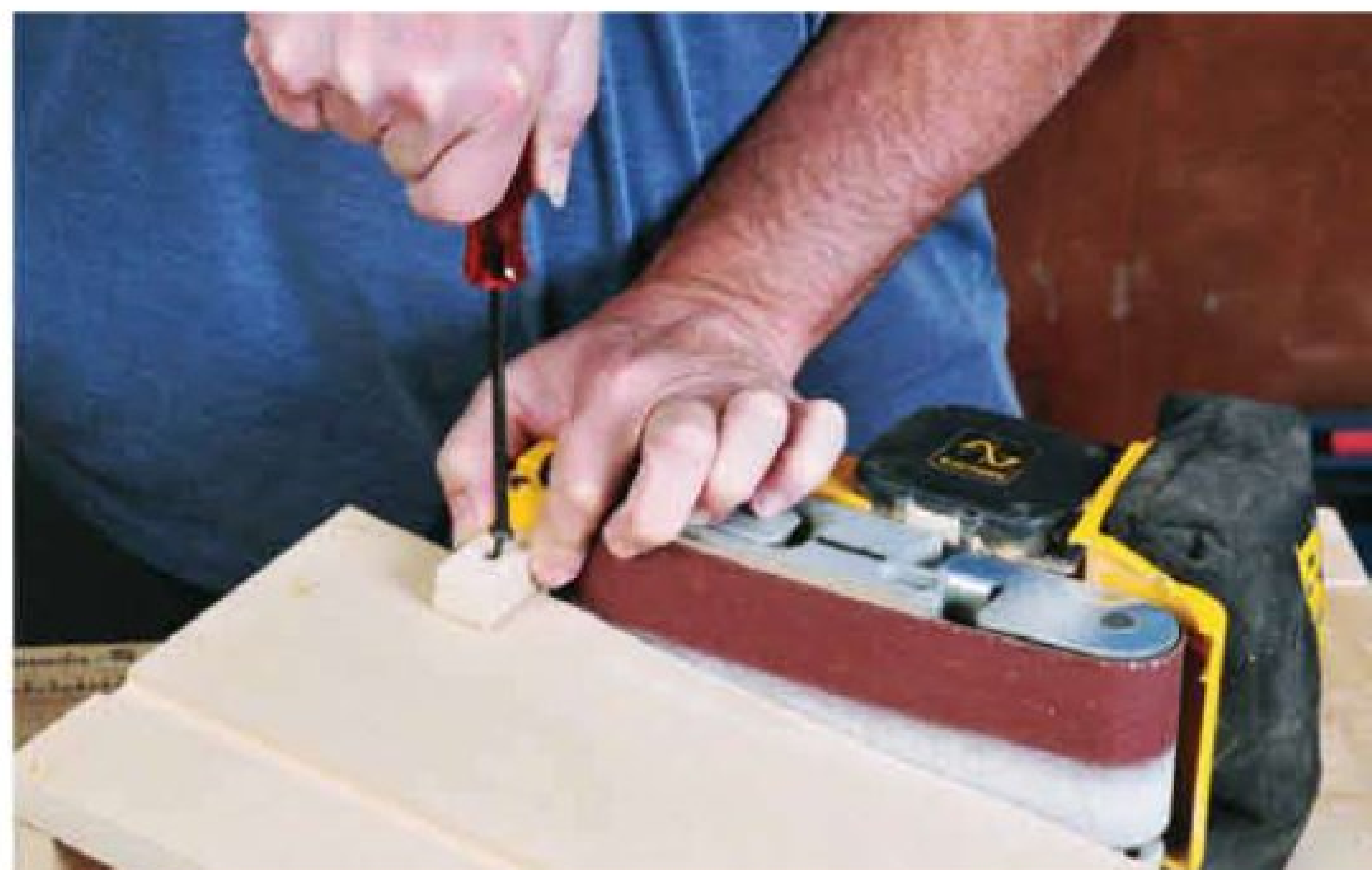
A small stop block screwed to the table top prevents workpieces from being thrown backwards by the force of the belt.
