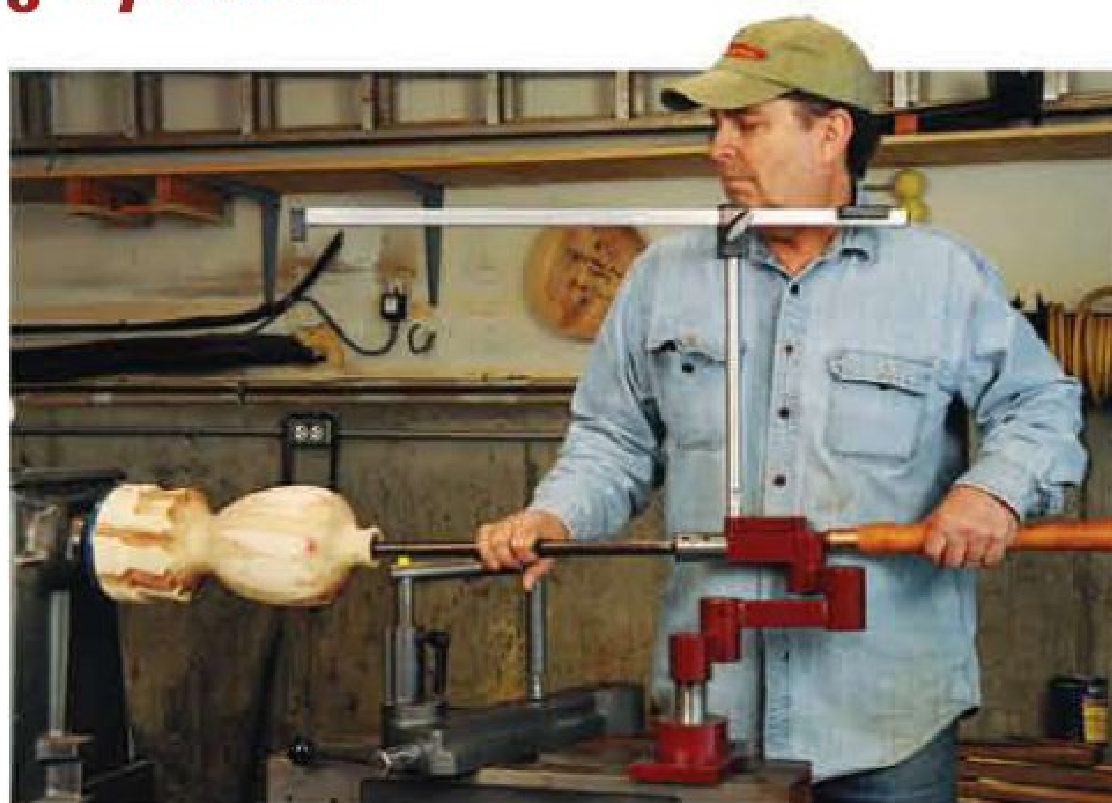
With a heavy-duty additional tool support and a laser that exactly locates where your cutter is, a captured hollowing system has its advantages. (Note ... the lathe is not turned on for this demo photo.)
