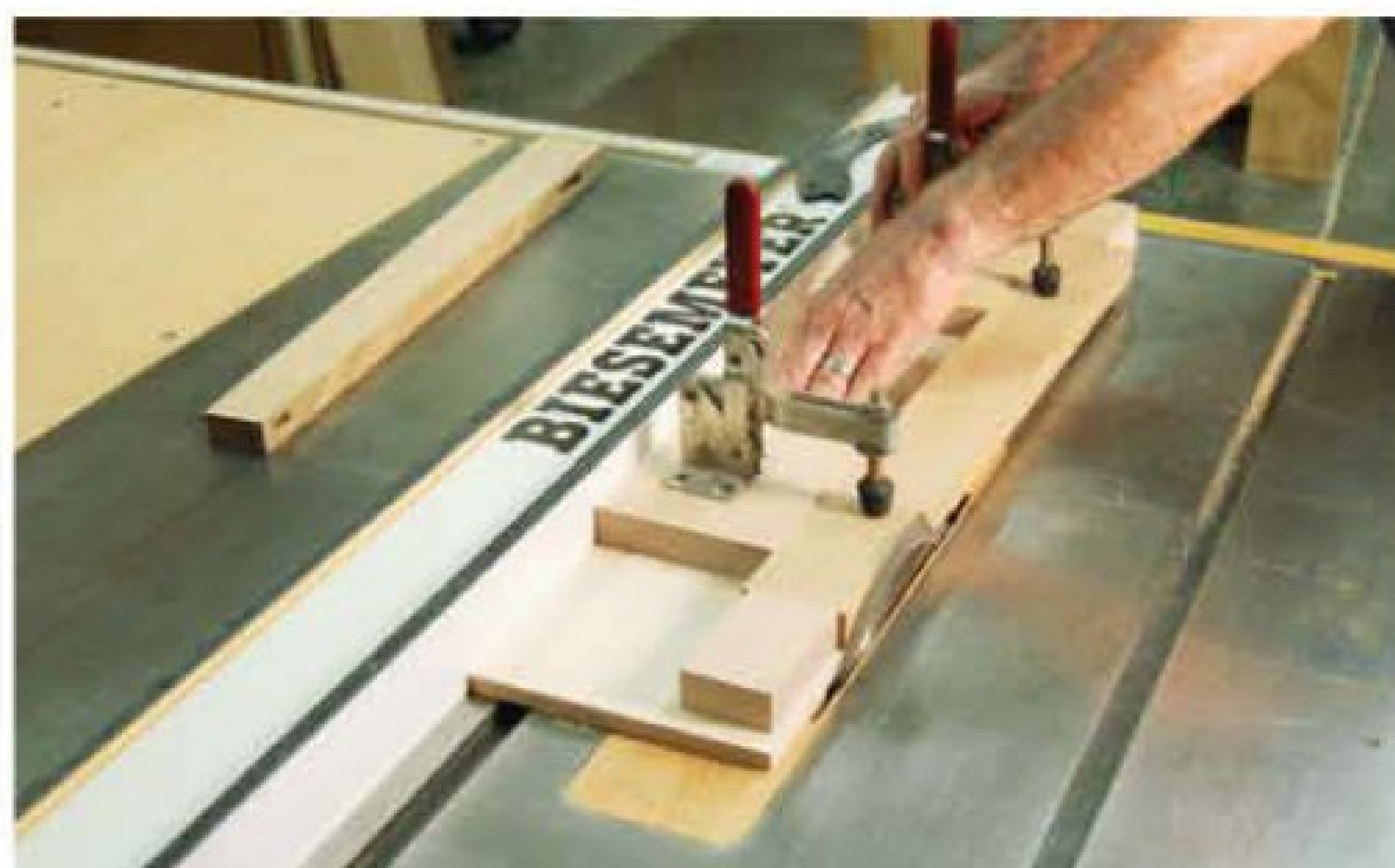
Here the author uses a shop-made tapering jig on his table saw to form the tapers on the outside edges of the two stiles.
