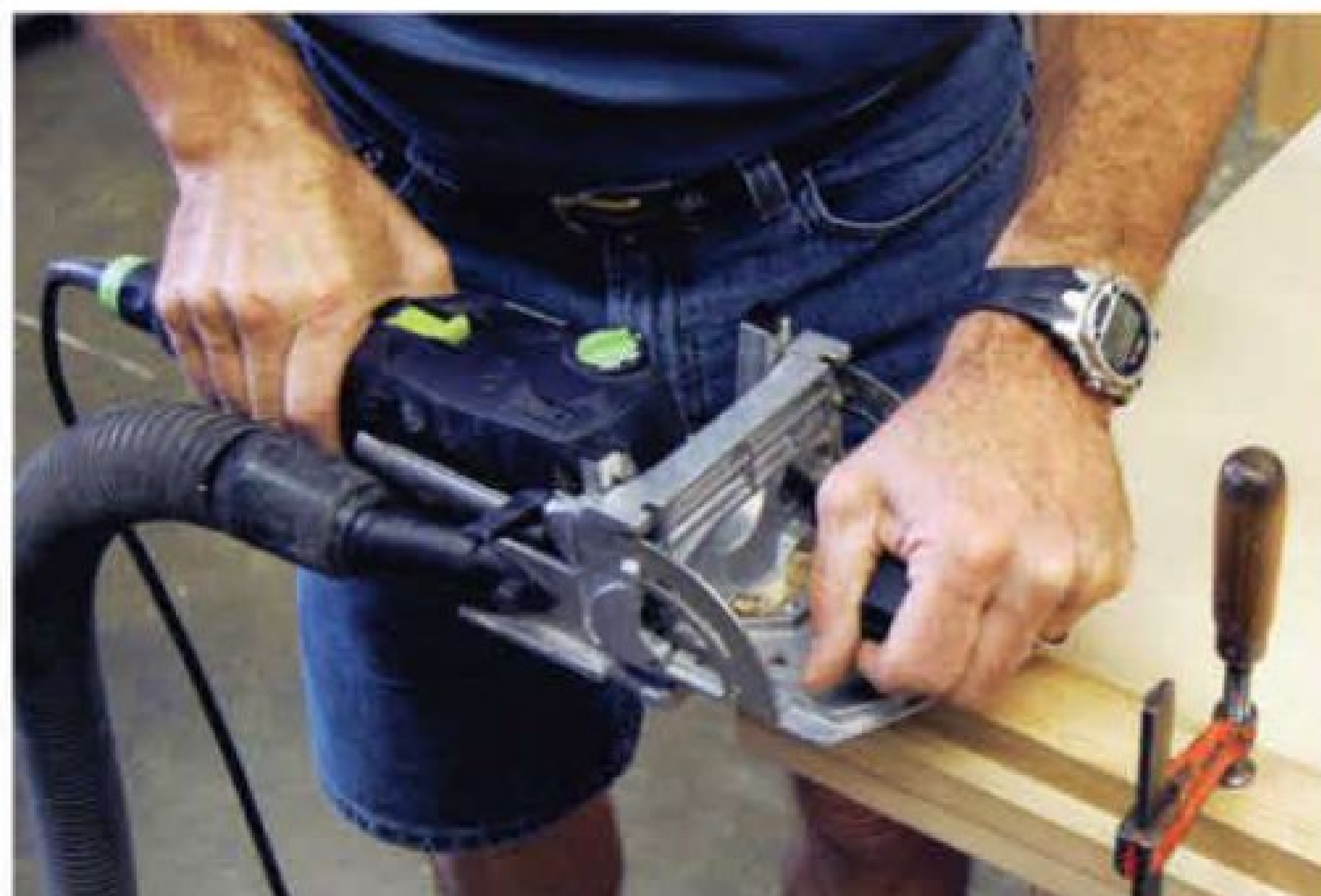
The author's Festool "Domino" tool was employed to create the four mortises for the loose tenons that hold the top rail in place.
