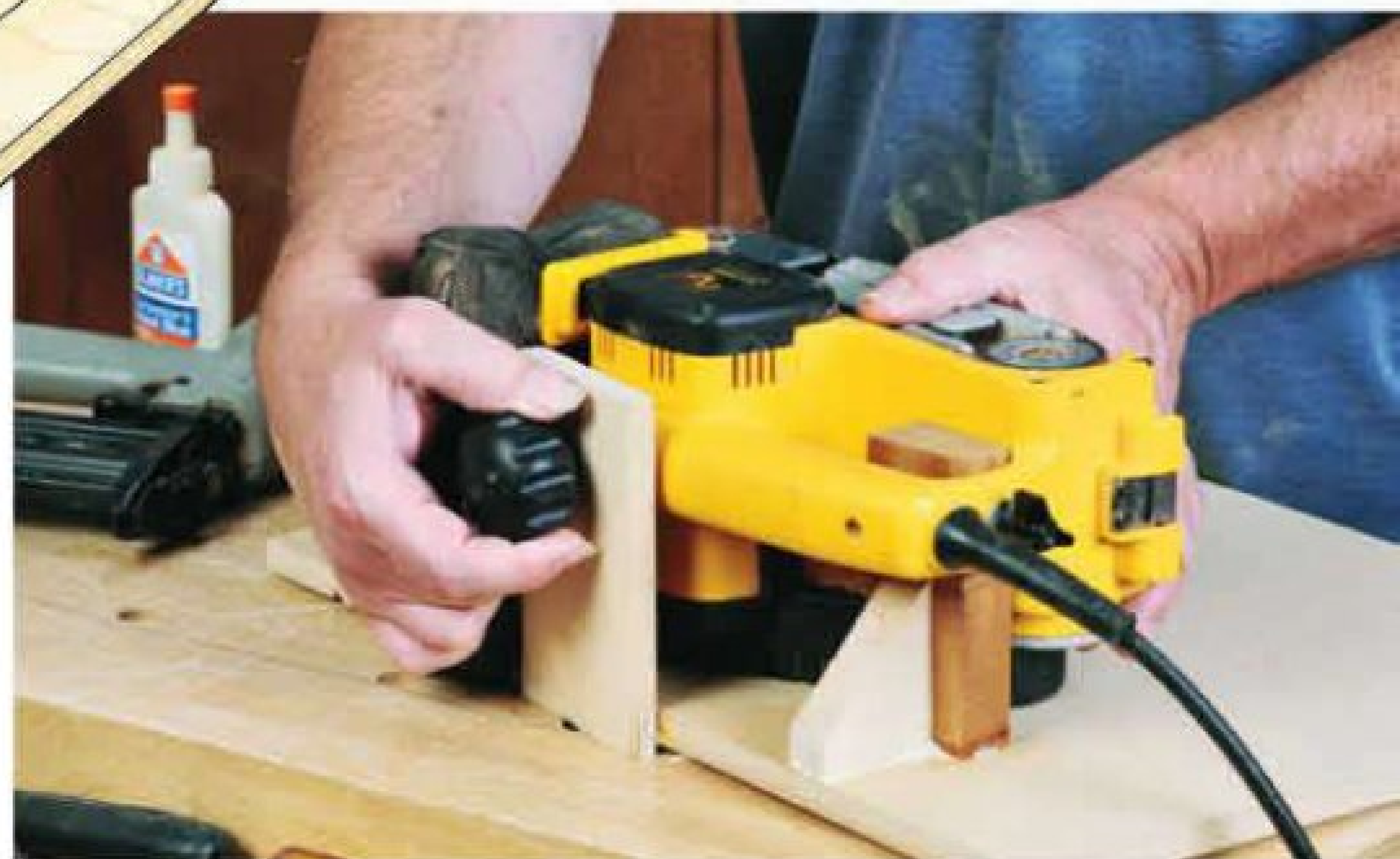
The removable top knob handle on this DeWALT belt sander is used here to fasten the tool to the base, via a mounting plate.
