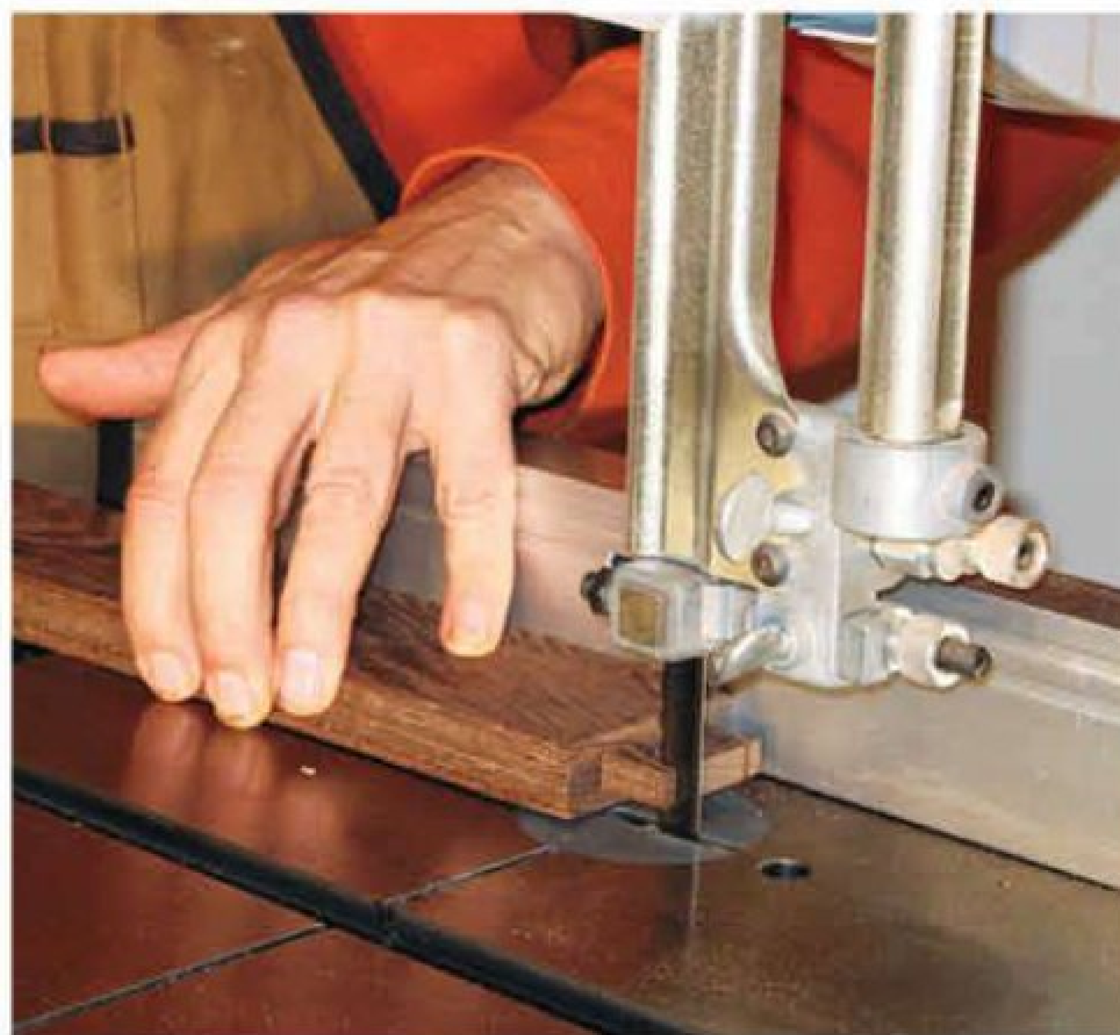
The author used the fence as a guide on the band saw when slicing the slots to accept the cherry tenon wedges. To work properly, the saw kerf must be slightly smaller in width than the wedges are thick.
