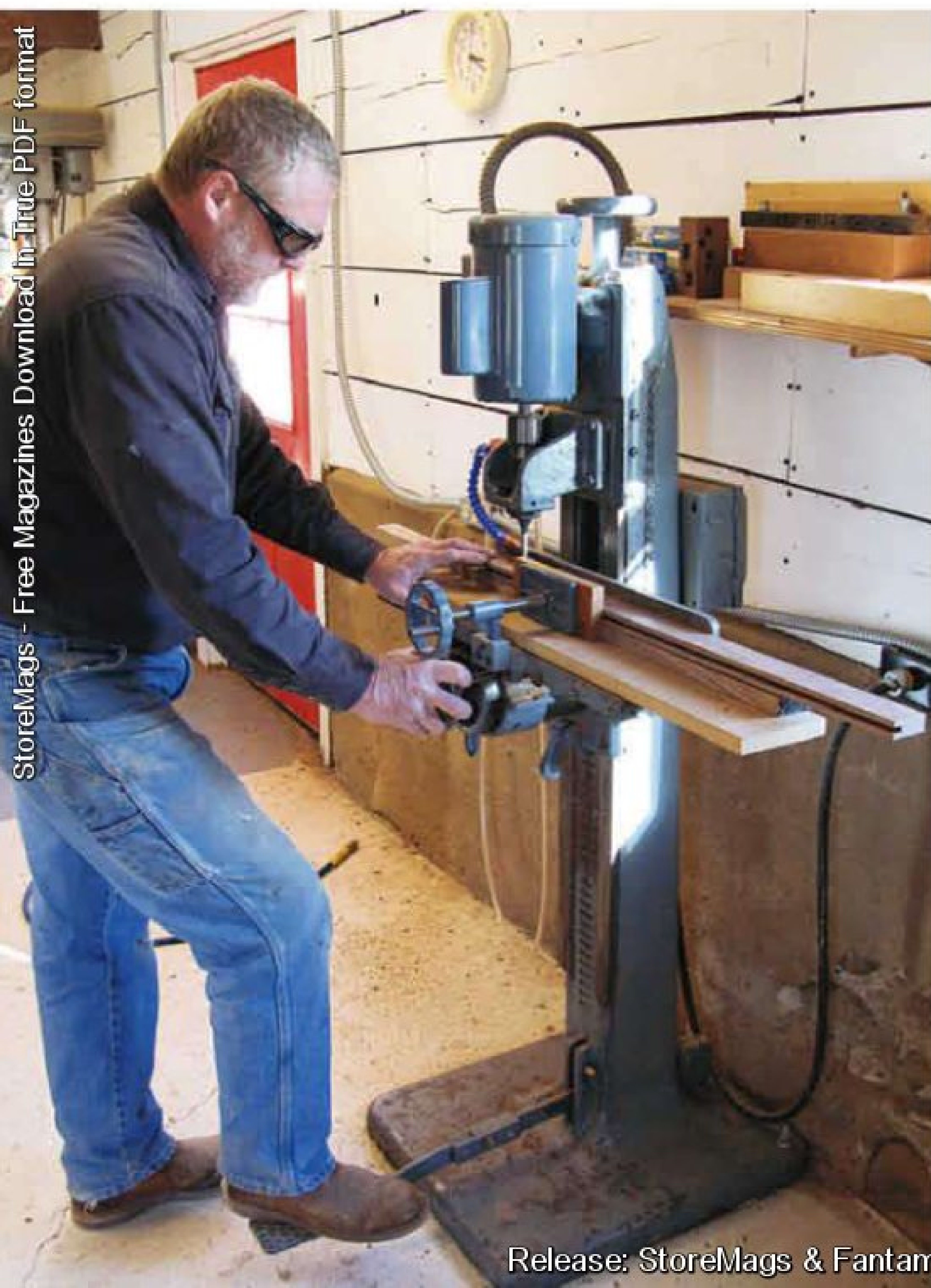
Chopping the mortises with his dedicated mortising machine, the author prefers to start with the innermost cut, working his way out. This helps to avoid bit deflection.
