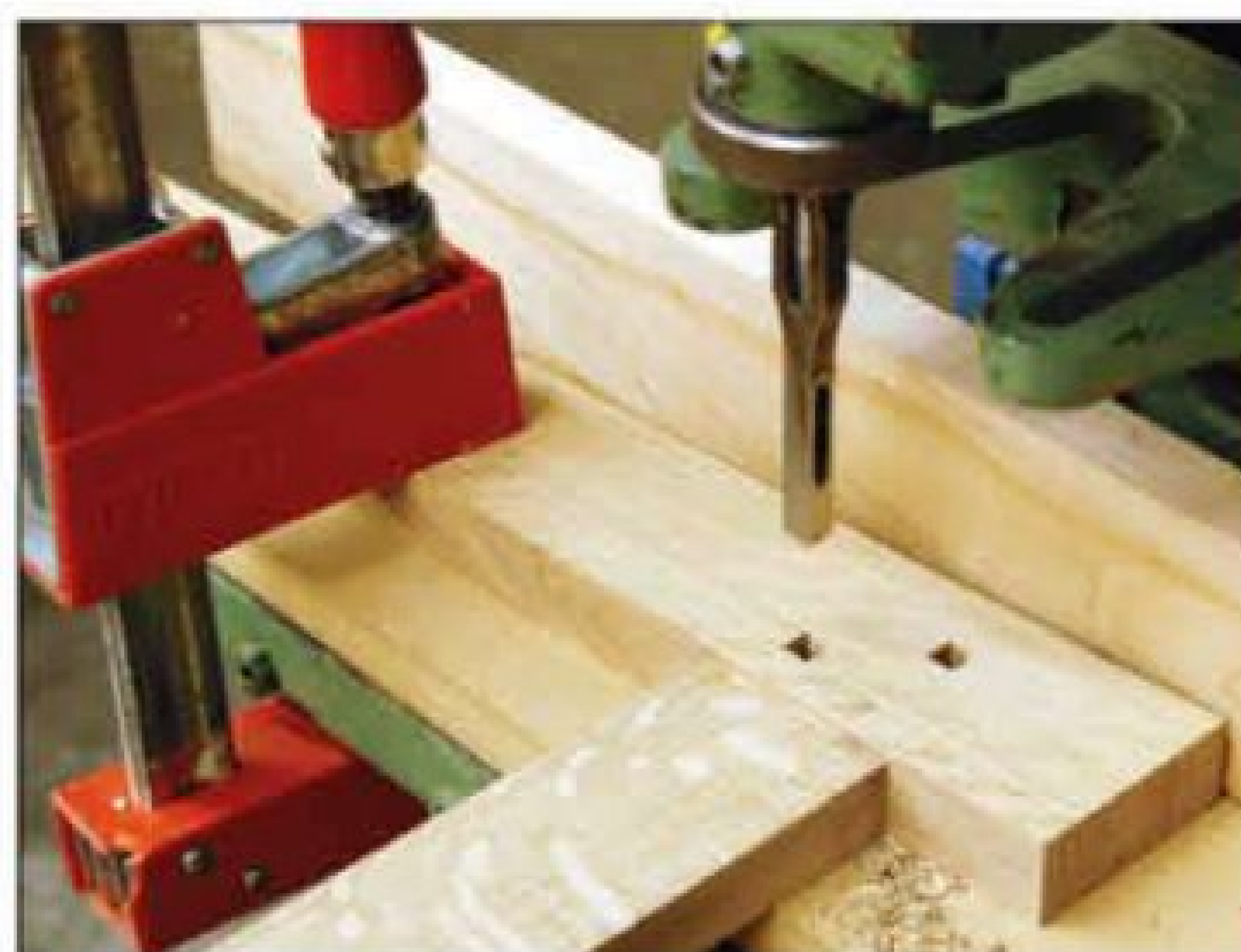
After dry-fitting the frame and positioning it on the Oliver, the author formed mortises for the ebony pins.
