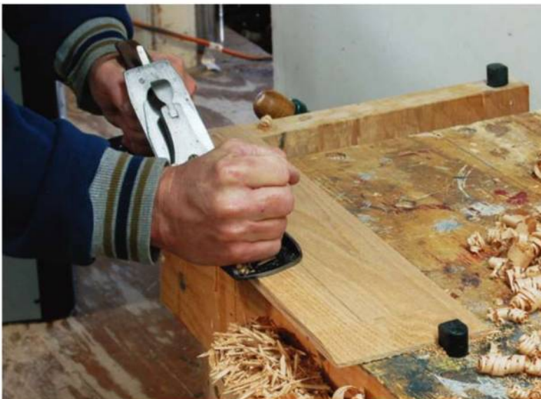
The back of the door panels were raised with a sharp jack plane: cut down to pencil lines running around the edges of each panel with pencil lines on the back surfaces.
