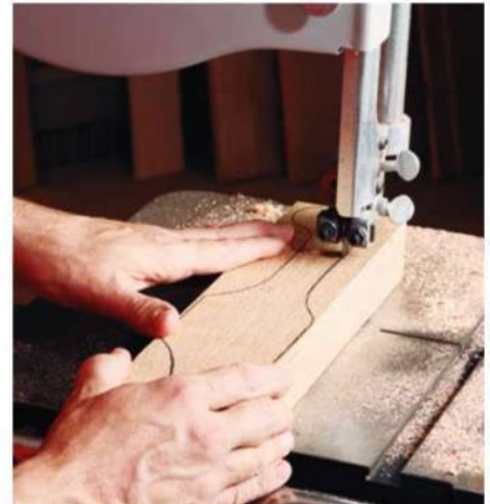
Begin by cutting out the tail section of the fuselage blank. Leave the front section squared up to assist with the jointing step.
