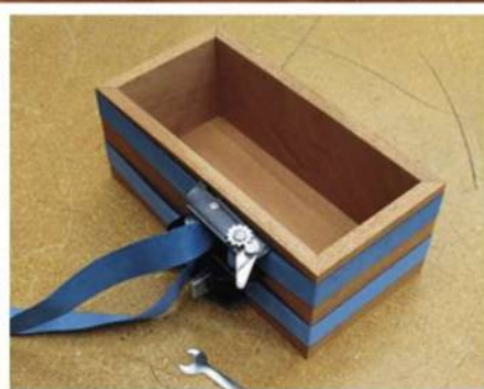
The sides and ends were ripped to width and then mitered to length. The author's miter saw was large enough to handle the miters (above). Band clamps held the box square as the glue cured.
