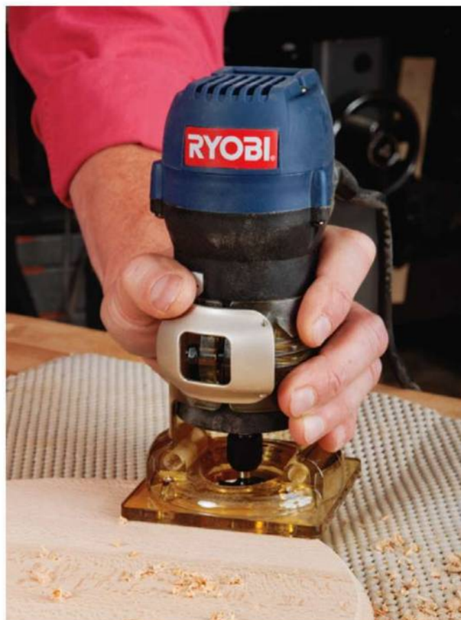
There's no reason to risk sanding through delicate face veneer when you can use a trim router to bring solid-wood lipping flush (above). Edge profiling (below) is well within a trim router's bag of tricks, provided you sneak up on the final cutting depth with several rounds of passes.
