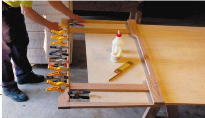
This photo shows a back view of the front assembly. Notice that the top rail is screwed to the back of the stiles (and the tapered stiles are temporarily attached to the top rail), rather than being tenoned.
