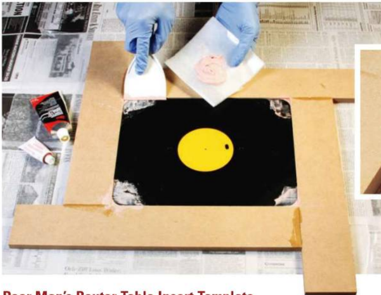
Scrap MDF and Bondo combine to create a perfect router insert template.
