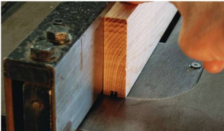
The author turned to his table saw to cut grooves in the rails and stiles for housing the floating door panels. It took a few quick passes per stile and rail.
