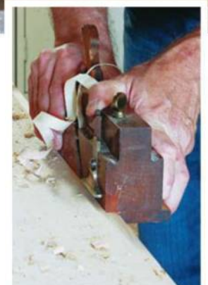
A solid oak cleat supports the front edge of the plywood plinth deck. The author cut the rabbet on the bottom front edge of the plinth deck using a moving filletster made in 1840 (shown at right). Cutting a single rabbet in this manner is not only quicker than it would be with a router or table saw (you don't have any cutters to change when you're using a moving filletster); it is also infinitely more pleasant to perform the work with a hand tool that saw its first use in a shop lit by candles or gas lamps.
