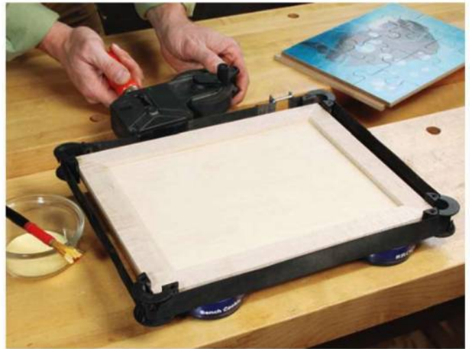
Miter-cut and dry-fit all four rails onto the frame base to make sure the joints will close properly during the gluing stage. A small band clamp like this one can provide even clamping pressure all around the frame.
