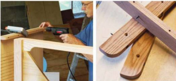
Cleats (left) create strong glue joints in plywood cases, but care must be taken so that their installation screws extend through the cleats no more than 5/8" when used with plywood that is nominally 3/4" thick. Glued and screwed cleats were applied to the inside top surfaces of the end panels, then to the underside of the top.
