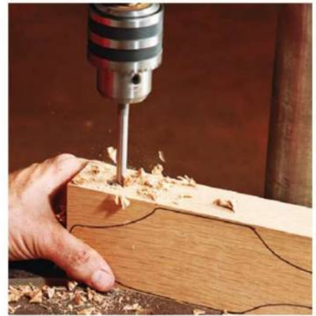
Bore the hole that will hold the pilot while the fuselage blank is still squared up. The author used a 7/8" Forstner bit in his drill press.
