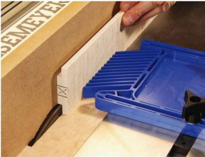
On stock this thin and narrow, one way to introduce more safety into the operation is to mill two rails at once from wider stock, then rip them free after the frame rabbets are cut. Control the stock with a featherboard.
