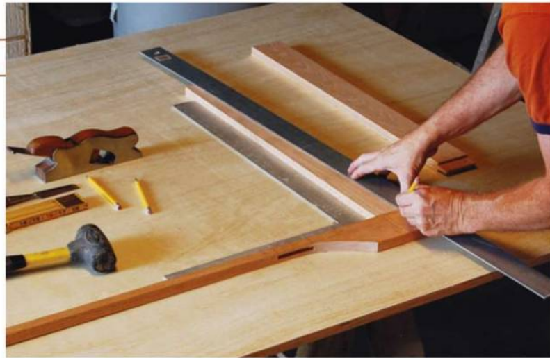
After cutting the mortise-and-tenon joints at the bottom of the front's rails and stiles, the author dry-assembled the joints, trued them with a framing square, and marked the angles on the tapered stiles.
