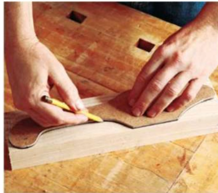
Mark out the shape of the airplane's fuselage with the aid of a template. A template will allow you to make several toys with ease.
