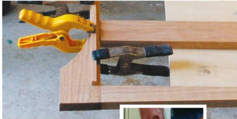
A solid oak cleat supports the front edge of the plywood plinth deck. The author cut the rabbet on the bottom front edge of the plinth deck using a moving filletster made in 1840 (shown at right). Cutting a single rabbet in this manner is not only quicker than it would be with a router or table saw (you don't have any cutters to change when you're using a moving filletster); it is also infinitely more pleasant to perform the work with a hand tool that saw its first use in a shop lit by candles or gas lamps.
