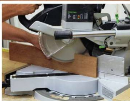
The sides and ends were ripped to width and then mitered to length. The author's miter saw was large enough to handle the miters (above). Band clamps held the box square as the glue cured.
