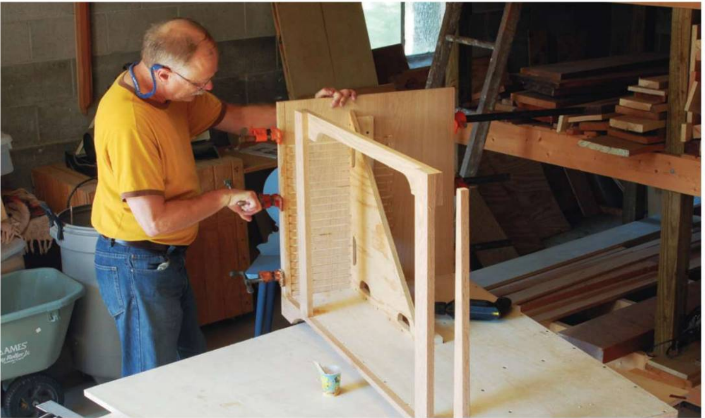
Plywood corner brackets, which stabilized the end panels during assembly, were temporarily screwed to the inside surfaces of the cabinet. Notice that the top rail of the front has been cut off and planed flat at this stage of the assembly.
