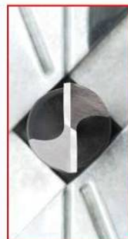
A perfectly sharpened bit.
