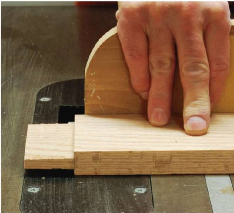
Door tenons were milled to rough size at the table saw using a stack of dado cutters, then fine-tuned with a shoulder plane to fit their mortises.
