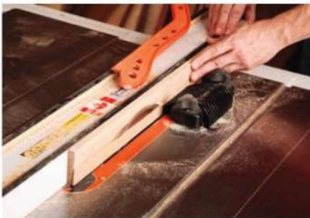
Here the author forms the 7° angle on an over-long piece of stock. He chose to make the piece long enough to easily make two wings.
