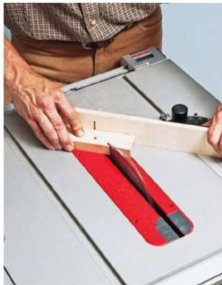
The frog is cut at 45° using a miter gauge equipped with an auxiliary fence. The 22.5° angle on the nose is formed in a similar way.
