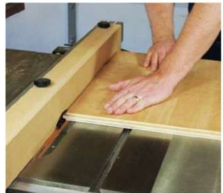
The sub-top is made from good quality plywood. The author forms a tongue around the edge of the sub-top using a dado head in his table saw.
