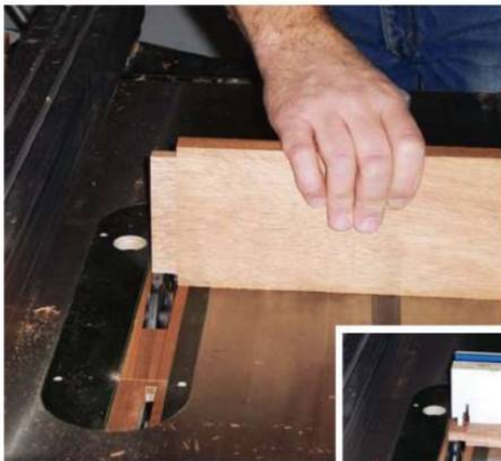
After the aprons and stretchers have been cut to length, the author raised tenons to match the mortises that had previously been chopped into the legs.
