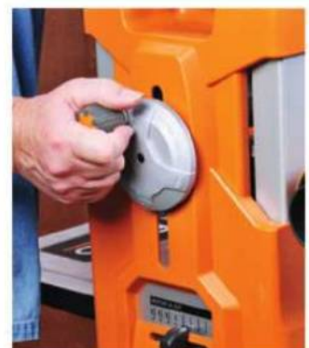
The RIDGID's unusual depth-setting wheel cranks vertically, instead of horizontally like the other planers, and it goes up and down with the motor/cutterhead.
