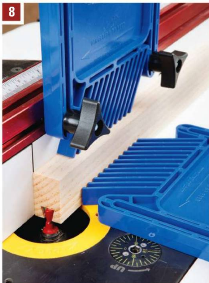
Want to mill an accurate sliding dovetail? The optimum setup should involve two featherboards, since this is a trapped bit technique.
