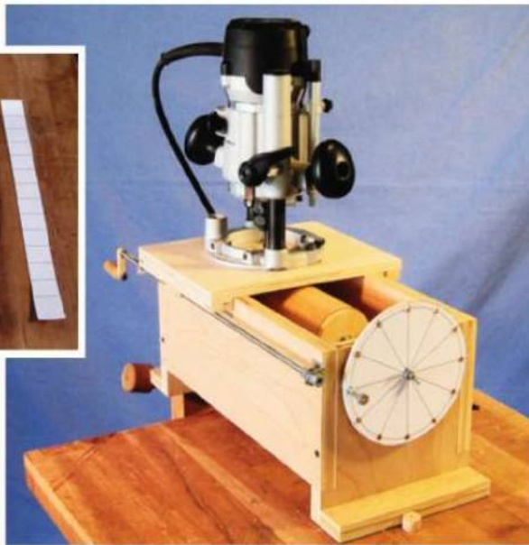
An index wheel (above left) locates flutes or grooves on a circular column when using a jig or lathe. The manual method (above right) transfers locations from a strip of paper.
