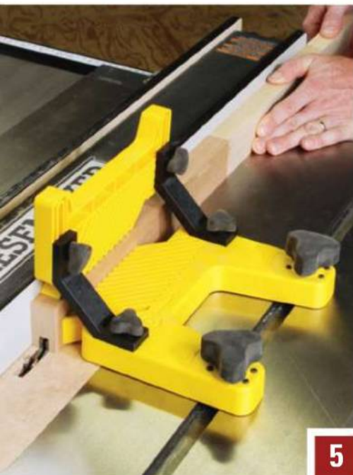
A combination of hold-in and hold-down restraint ensures safer operation and more accurate results with a dado blade.
