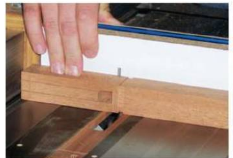
Plowing a shallow dado that extends all the way around the leg, the author prepares to miter and attach a decorative molding.
