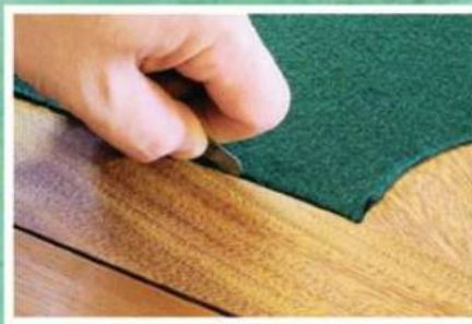
Tuck in the felt flap around the substrate using a thin wedge of some sort. The author used the rounded end of a small metal rule for the task.
