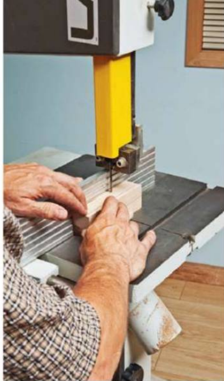
After calculating the frog and nose thickness from your plane iron, slice off the sides of the plane — a band saw is a good tool choice.
