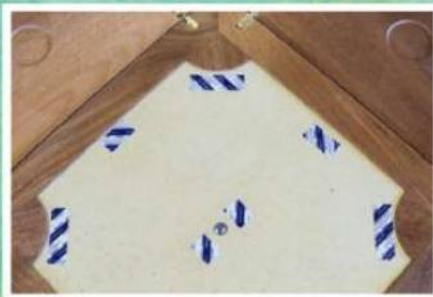
Double-sided carpet tape is used to secure the felt playing field to the frame subassembly. Use several pieces, as shown above.
