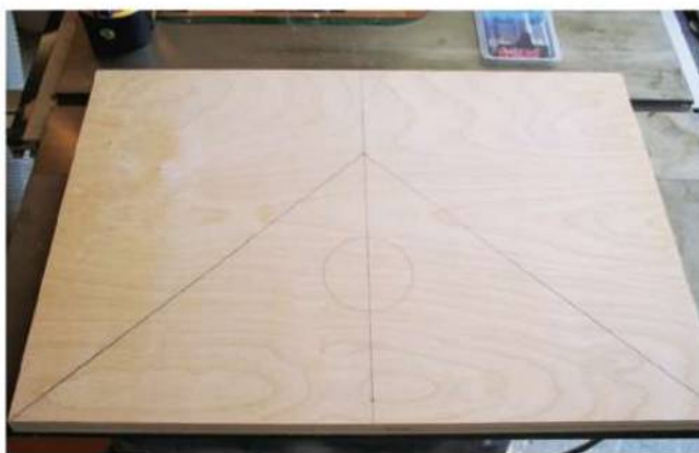
The key to perfectly fitting the leaves is creating an accurate leaf template. Test your template to be certain it is symmetrical.
