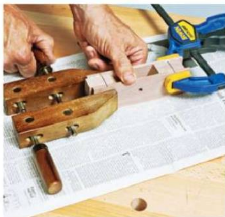
After dry-fitting the various components and adjusting the frog and nose positions, the final glue-up is pretty easy.
