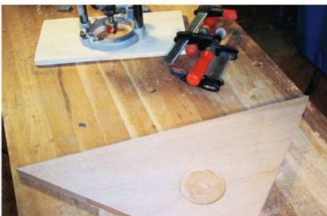
The chip depression is routed using a dish-carving or a bearing-guided core box bit inside a circular cutout in the template. The router has an auxiliary base attached to it to improve stability.
