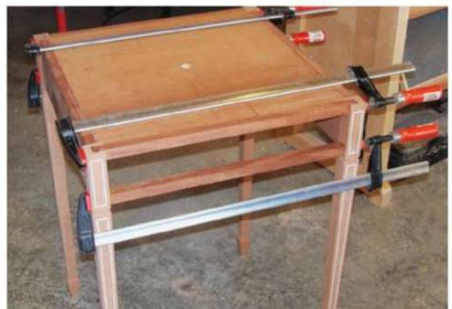
A final dry-fit of the joinery is essential before glue-up and assembly. You can't reverse the glue-and-clamp process once it's cured.
