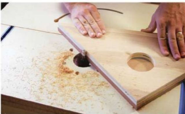
After rough-cutting the pieces to size (cut 1/16" from the line), attach your template with double-sided tape and cut the leaf to exact size.
