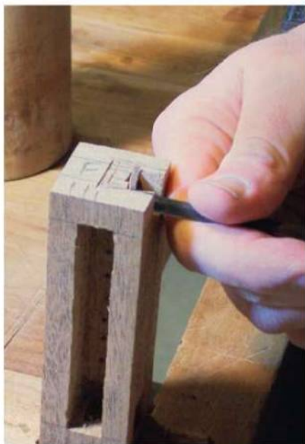
The top stretcher is joined to the leg using a dovetail rather than a mortise. The author formed the tail on the stretcher first, then transferred the shape to the top of the leg.
