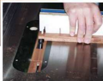
After the aprons and stretchers have been cut to length, the author raised tenons to match the mortises that had previously been chopped into the legs.
