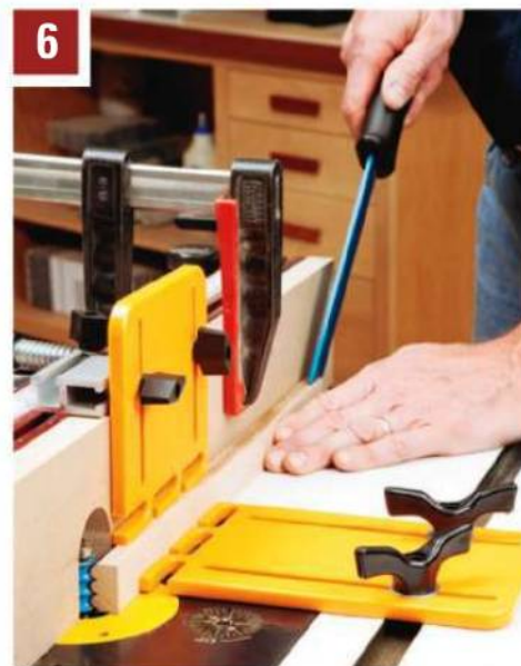
Push stick control is crucial when profiling narrow strips on the router table. Featherboards should not obstruct the push stick's path.
