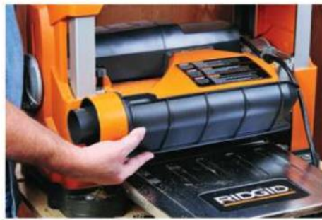
The RIDGID R4330 (below) has many impressive features, including a dust hood (left) that converts to a chip deflector (allowing you to use the planer without hooking up a vacuum) and a sliding depth preset (below left) that has eight different thickness settings.
