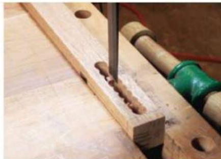
The author chopped mortises using a Forstner bit to remove the waste, followed up with a sharp bench chisel to pare the walls and ends.
