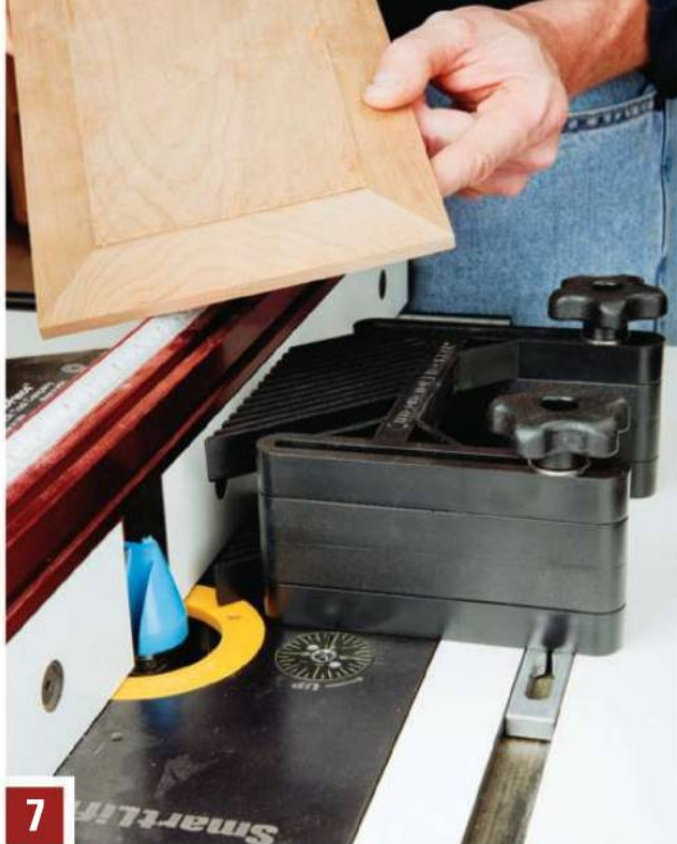
Rockler's Double Featherboard Kit creates a high-rise featherboard to keep panels planted against the fence during panel raising.
