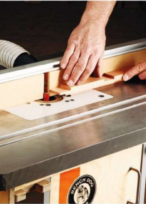
On the narrow stiles and rails, the author used a straight bit in his router table to form a rabbet that will later accept the art glass. Using the bit opening in the fence as a reference, the glass retaining rabbets were stopped. Later, after the door was assembled, they were completed.
