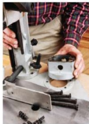
An included riser block (left) increases the stroke capacity of Craftsman's mortiser by 2 1/2". If you're a lefty, you'll also like the interchangeable feed handle (right) provisions here.
