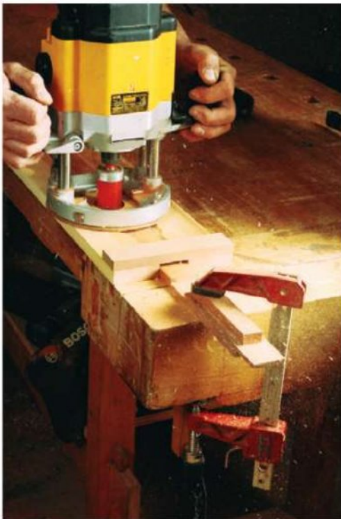
In addition to their half-lap joints, the middle section of the narrow stiles must be routed to about 1/2" thick. The author used a router and a basic jig to guide his machining.
