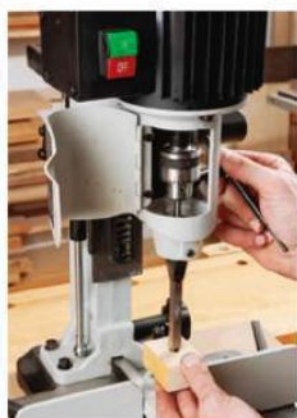
Fewer wrenches mean faster setups, and Delta speeds the process along with ratcheting handles (left). The headstock also offers excellent chuck access (right).
