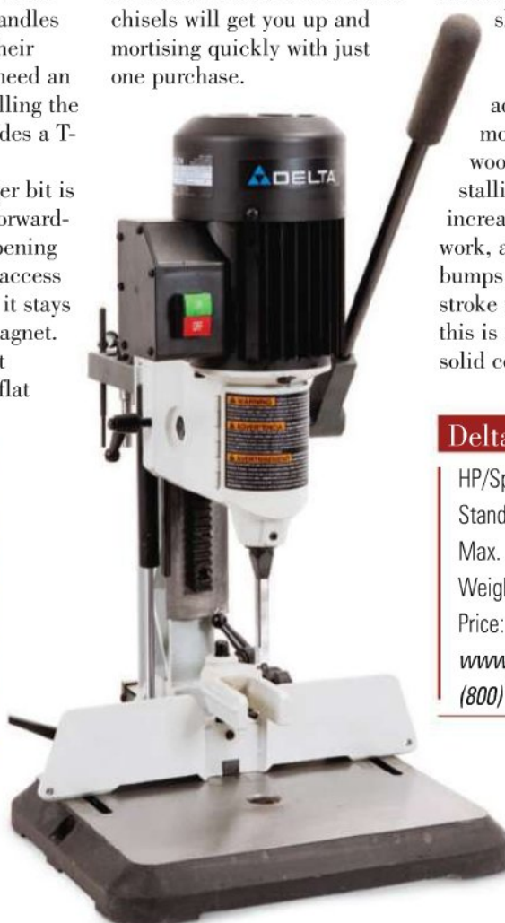
Fewer wrenches mean faster setups, and Delta speeds the process along with ratcheting handles (left). The headstock also offers excellent chuck access (right).
