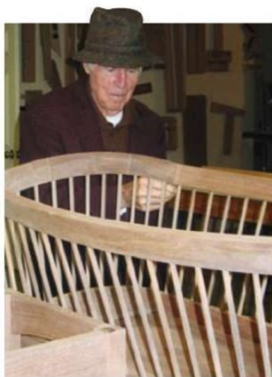
John McNany hand-sanded the cradle following assembly; wood filler repaired slight defects.
