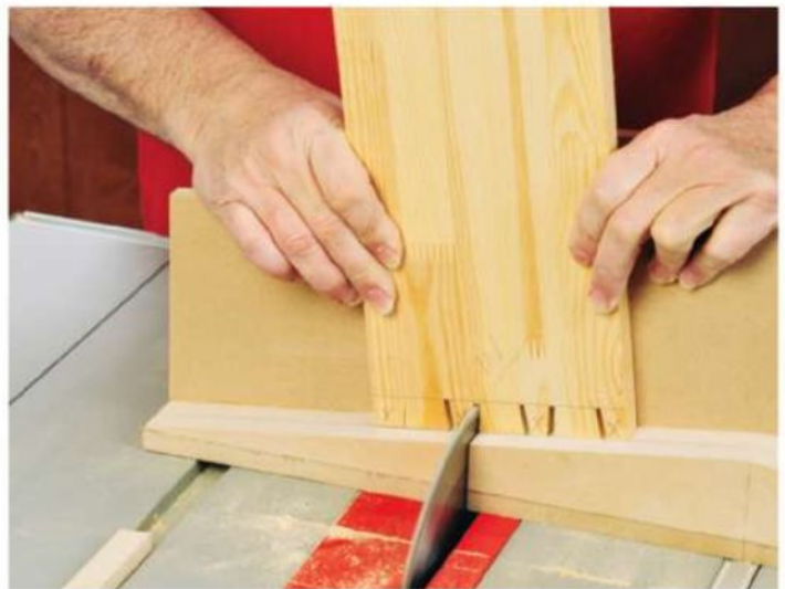
Figure 10: Spin the jig around front to back and cut the tails, using the ramps on each side of the jig to make the right- and left-hand cuts.
