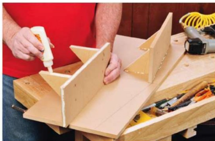
Figure 1: Attach the pin fences to the base at an 8° angle.
