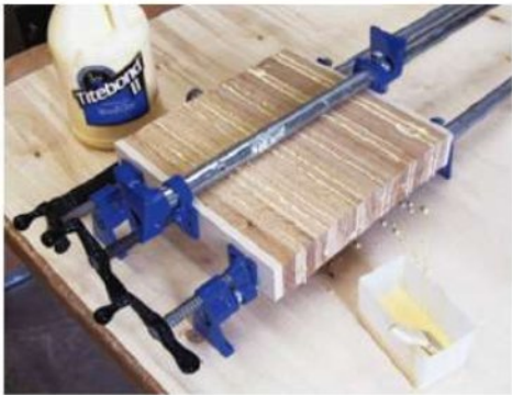
You can speed the process of laminating blanks for the casting pins and kubbs by gluing and clamping them all at once between several long bar or pipe clamps.
