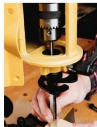
Powermatic ensures that workpieces will stay put by providing two knobs that set the hold-down, plus table feed rollers (left). Onboard spacers swing into place for setting chisel-to-bit clearance (right).
