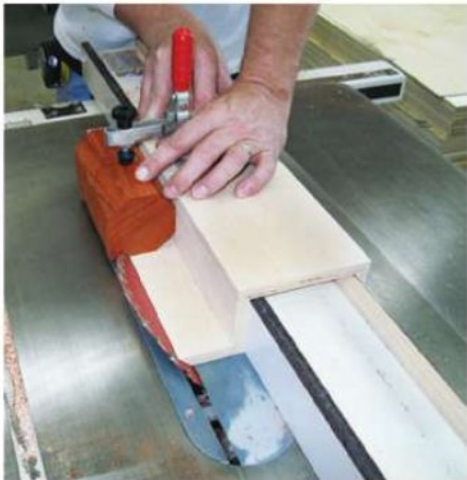
The same bevel-ripping jig and rip fence setting can form both the kubbs (left) and the casting pins (right). Set up the jig to cut the kubbs first. Four 45° rip cuts will turn them into octagons. Then slip a 11/32"-thick spacer next to the casting pin blanks before ripping them to shape.
