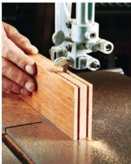
After the initial cuts on the table saw, the author stepped to the band saw to extend and complete the door's variously shaped tenons.
