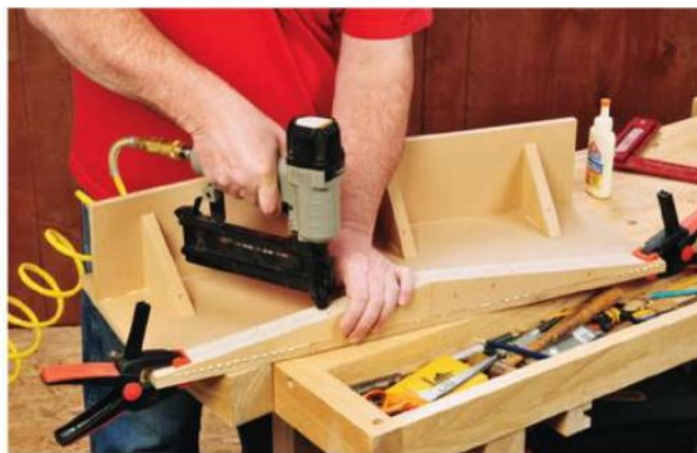
Figure 2: The 8° wedge ramp is formed from two 3/4" pieces.
