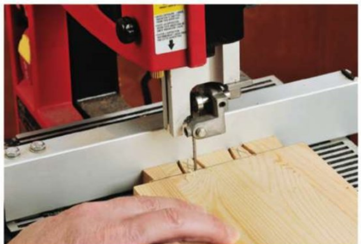
Figure 11: An efficient way to remove the waste between tails is to use your band saw equipped with a narrow saw blade. Set the fence to the proper distance and carefully saw away the waste.
