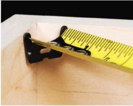
A tape measure's hook end has to be positioned in exactly the same way for each diagonal measurement — and a pinch rod's "chisel edge" must be at the same depth at each end.
