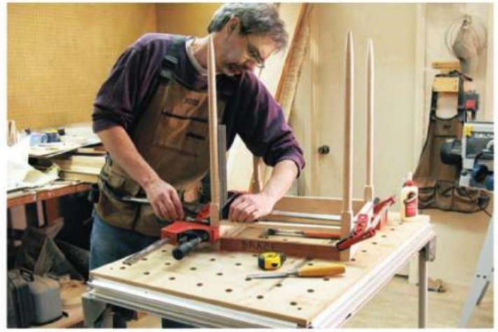
If all the parts are properly prepared, the table's assembly is very straightforward. As glue-up is a step that is nearly impossible to reverse, always check to see that your subassembly is square and true.
