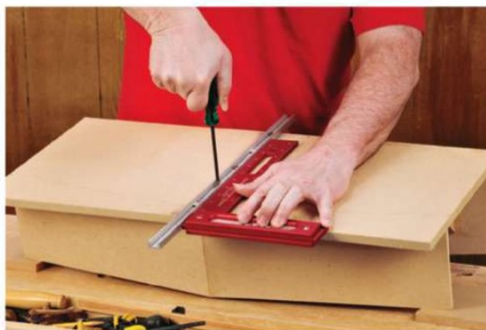
Figure 4: Attach an 18"-long miter bar to the bottom of the jig.
