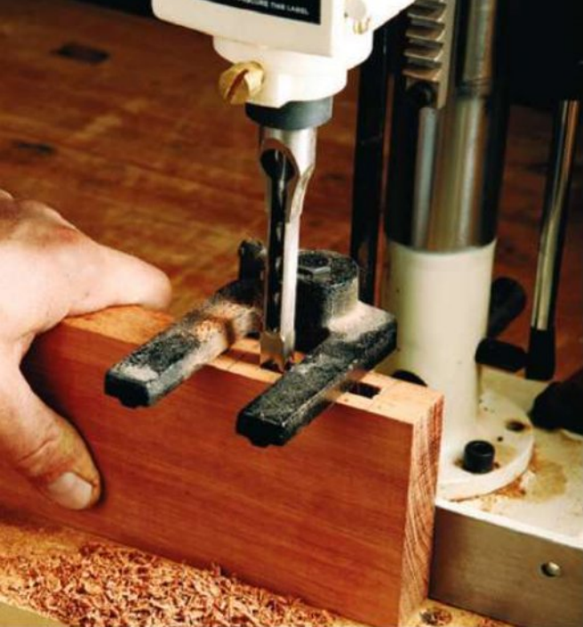
Lyptus is a dense hardwood that machines well. Our author found that a dedicated mortising machine was a real time and effort saver while making this screen door project.
