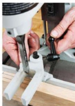
Fewer wrenches mean faster setups, and Delta speeds the process along with ratcheting handles (left). The headstock also offers excellent chuck access (right).
