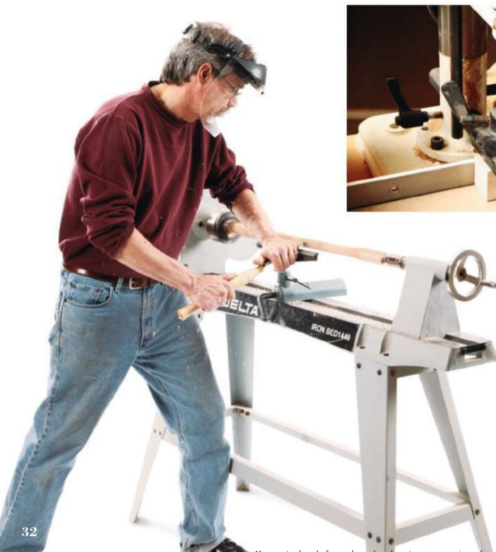
After turning the legs (at left), the next machining step was to chop their mortises (top photo). Once all the mortising was done, the author machine sanded all the legs clamped together.
