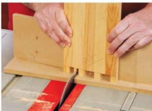
Figure 8: After establishing the left side of the pins, you can take multiple passes to remove the waste.
