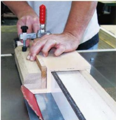
The same bevel-ripping jig and rip fence setting can form both the kubbs (left) and the casting pins (right). Set up the jig to cut the kubbs first. Four 45° rip cuts will turn them into octagons. Then slip a 11/32"-thick spacer next to the casting pin blanks before ripping them to shape.
