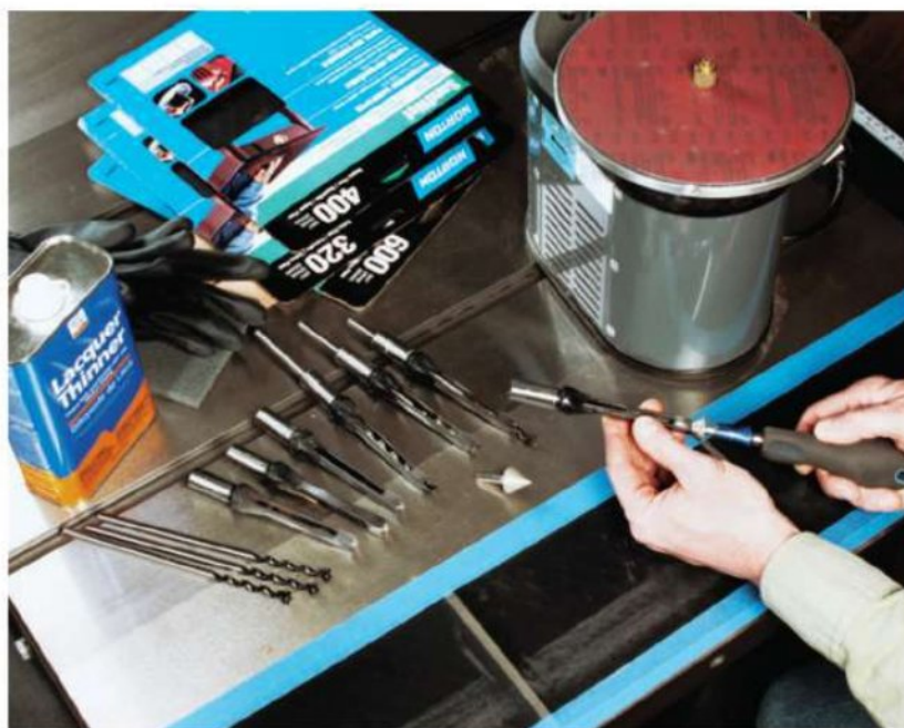
Our author used a procedure similar to sharpening a bench chisel to clean and lap the new hollow-chisel bits before beginning his cutting test. The effort seems to have helped. Generally, clogging was minimal, and the bits cut cleanly without laboring the machines. Lapping the chisel backs may also have reduced friction during use, which leads to heat buildup, bluing and eventually dulled edges.
