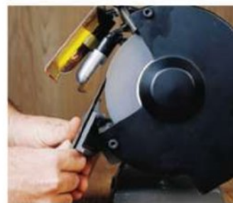
Grinding to repair the edge
