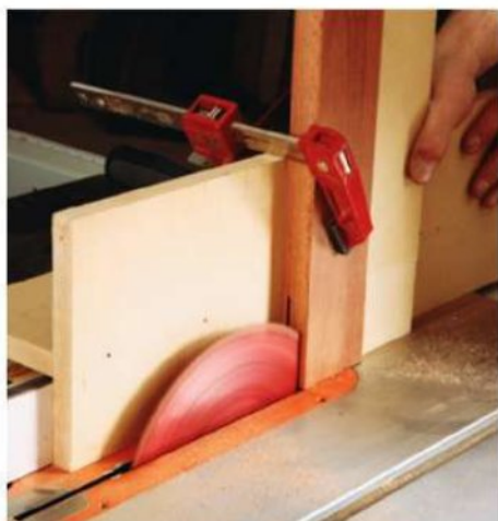
The author formed the large tenons for this project using a shop-made jig for the table saw. Test fit the tenons to the mortises.
