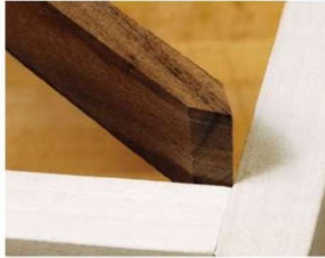
A tape measure's hook end has to be positioned in exactly the same way for each diagonal measurement — and a pinch rod's "chisel edge" must be at the same depth at each end.
