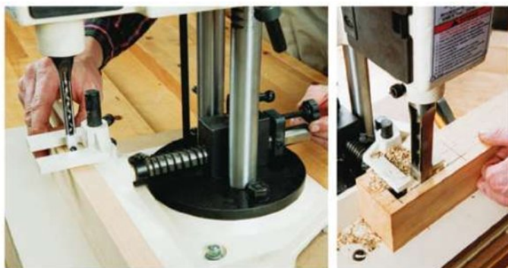
You can adjust Shop Fox's fence incrementally using the threaded micro-adjuster in back (left). A larger motor than most other machines in this category enabled the W1671 to tackle big, tough mortising in ash (right).
