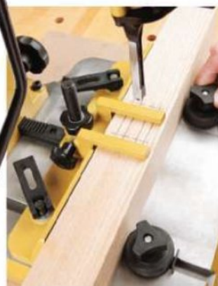
Powermatic ensures that workpieces will stay put by providing two knobs that set the hold-down, plus table feed rollers (left). Onboard spacers swing into place for setting chisel-to-bit clearance (right).
