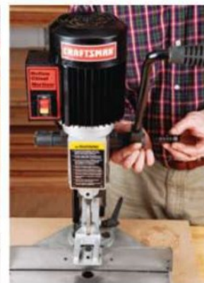
An included riser block (left) increases the stroke capacity of Craftsman's mortiser by 2 1/2". If you're a lefty, you'll also like the interchangeable feed handle (right) provisions here.
