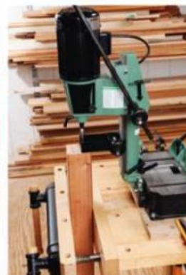
General International expands the range of mortising possibilities by outfitting the 75-050T M1 with a tilting column (left) and a convenient means of rotating the headstock for off-the-table applications (right).
