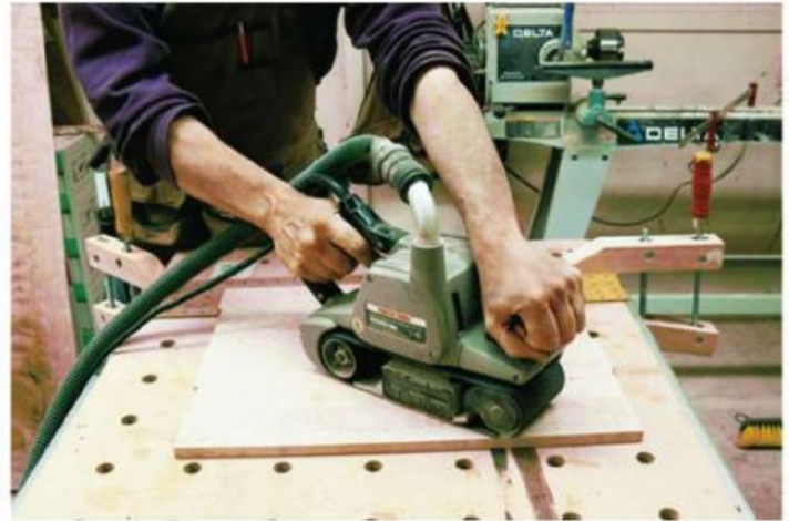
Once the slightly oversized tabletop blanks were removed from their clamps, the author used a 4 x 24 belt sander, working on the diagonal, to flatten and smooth the tops. When flat, the tops were cut to size.
