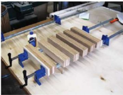
You can speed the process of laminating blanks for the casting pins and kubbs by gluing and clamping them all at once between several long bar or pipe clamps.
