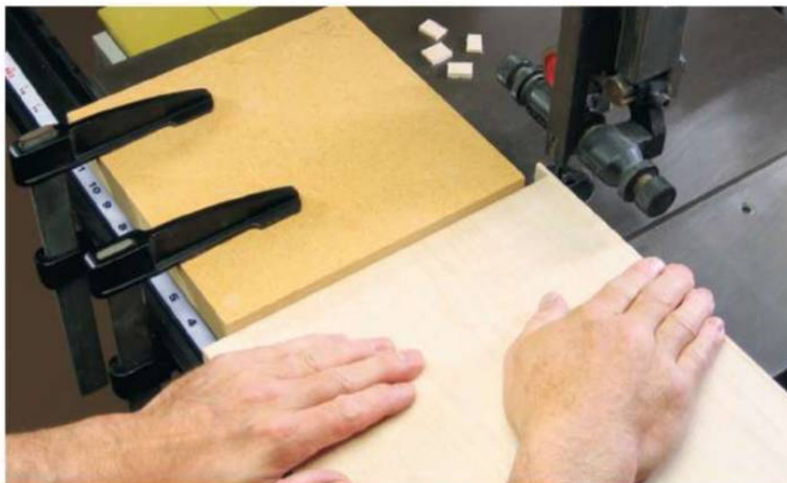
Once the glue sets, try this simple band saw fence setup. It makes quick work of trimming the edging ends. The right side of the clamped-on fence is aligned parallel and just slightly right of the saw blade.
