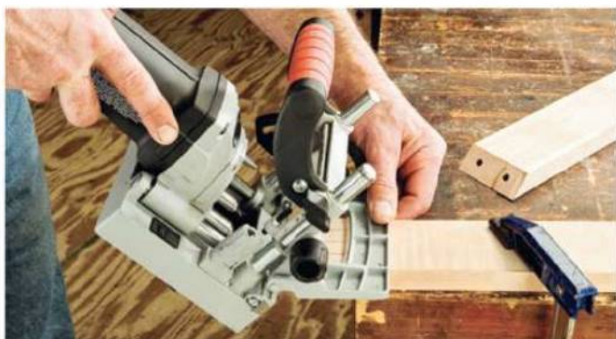
The Freud FDW710K, Domino and biscuit joiners can be used to add loose tenons to an angled surface, like this miter.
