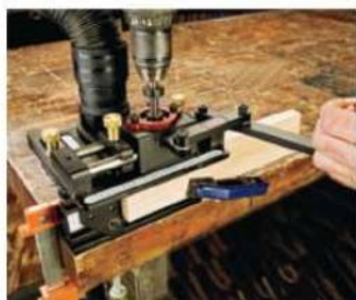
Run the drill, press down lightly, and move the handle back and forth to make a mortise with the JessEm Zip Slot Mills.
