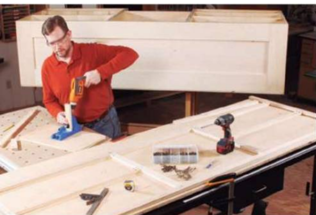
Attach thick edging strips to the long top and back panels with #20 biscuits (top photo). The author constructed the carcass as two subassemblies of shelf banks, building one side at a time (above).
