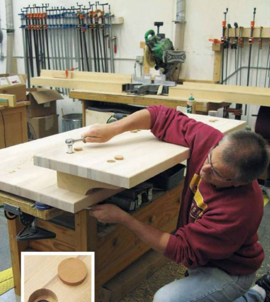
A set of ratchet wrenches are used to keep the bolt assembly buried in the counter and top, as shown at left. Two long wood screws will ensure a tight fit between the outer supports and the top (top photo). Once the top was completed, the author moved on to the casework, which was kept very simple.
