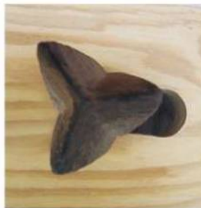
Our February mystery tool's end was designed to create splits in wooden baskets and barrels.
