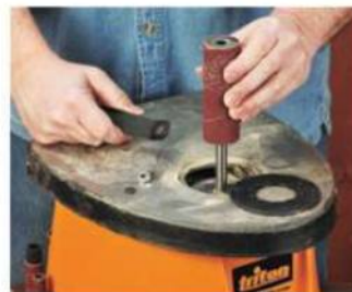
An oscillating spindle sander’s interchangeable drums let you set up the machine to effectively sand concave curved edges of different diameters.
