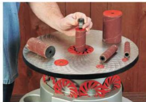
A rubberized knob locks a sanding drum on the Craftsman's spindle, allowing quick, tool-less changes from one drum diameter to another.
