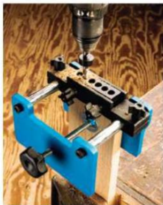
The beadLOCK system relies on a movable drill guide, which allows you to drill five overlapping 3/8" holes by using the guide in two positions.
