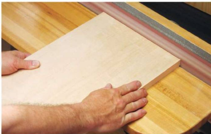
With everything trimmed up, sand the edging ends flush using an edge sander. If you don't own this machine you can sand by hand, but be sure to use a hard sanding block.
