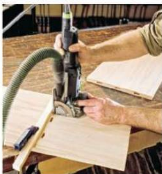
Case joinery requires mortises in the middle of a piece, and in an edge. This can be done with biscuit joiners, the Freud FDW710K machine or with the Festool Domino, but not with the others.
