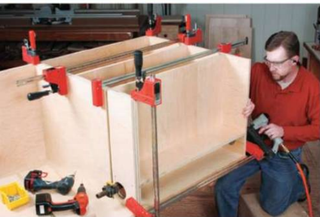
Attach thick edging strips to the long top and back panels with #20 biscuits (top photo). The author constructed the carcass as two subassemblies of shelf banks, building one side at a time (above).
