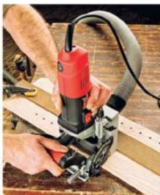
Two boring bits on Freud's FDW710K Doweling Joiner make quick work of drilling equally spaced shelf pin holes.
