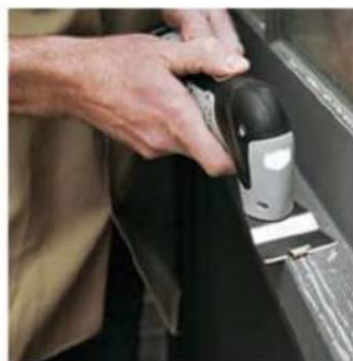
SCRAPING: Side-to-side oscillation also functions for scraping tasks, such as paint removal, with a scraper blade.
