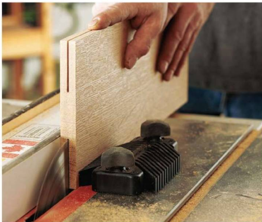
The author uses a thin kerf saw blade to start the resawing process. After both saw kerfs have been formed in the board, the author switches to a band saw to complete the resawing effort. The two existing saw kerfs help keep the band saw blade aligned during the cut.
