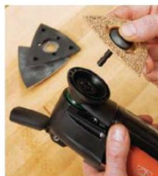
The QuickIN lever system on Fein's FMM250Q and SuperCut enables tool-free attachment changes.
