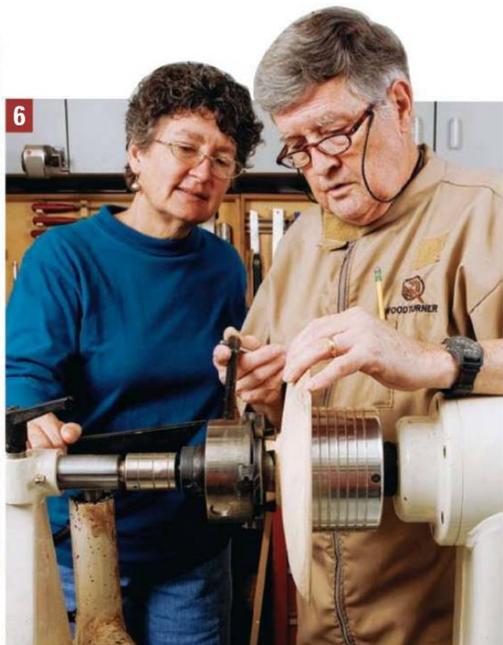
Once the bowl is properly centered onto the vacuum chuck, the next step is to engage the vacuum pump and then release the original chuck — the bowl is now ready to have its base completed.
