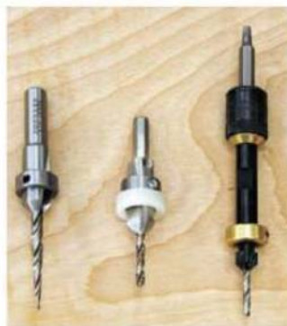
Here are three typical styles of piloted countersinks. Each can be adjusted to create a pilot hole of exact depth, along with its countersink, simultaneously. The stop collar on each sets the optimal depth for countersink.
