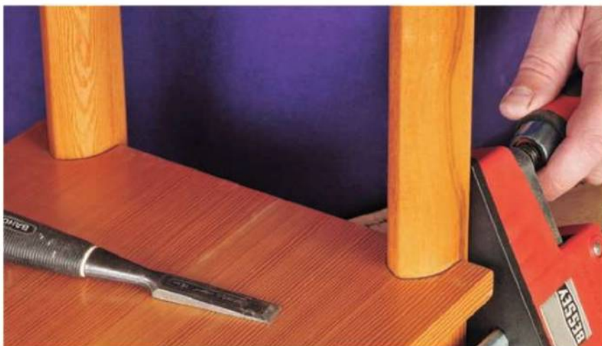
The reveals that surround these parabolic shaped legs add drama to the look of the table. The legs look as if they are piercing the shelf. The author added the reveal after fitting the legs, carving the gap with a sharp chisel.
