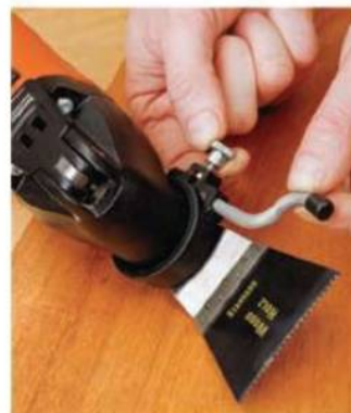
Fein's SuperCut multi-tool includes an adjustable depth stop for controlling plunge cuts.
