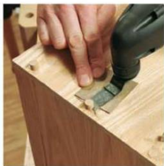
CUTTING: Offset end-cutting blades enable a multi-tool to make plunge and flush cuts without the risk of kickback.
