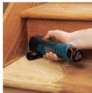
SANDING: Install a triangular or teardrop-shaped sanding pad on a multi-tool, and it becomes a detail sander for many applications.
