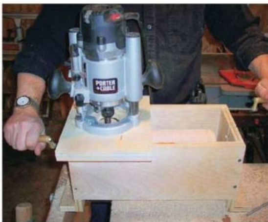
Shaping each sleeve into a cylinder is a process of slowly moving the router slide across the jig while simultaneously turning the sleeve. It's a two-crank operation.
