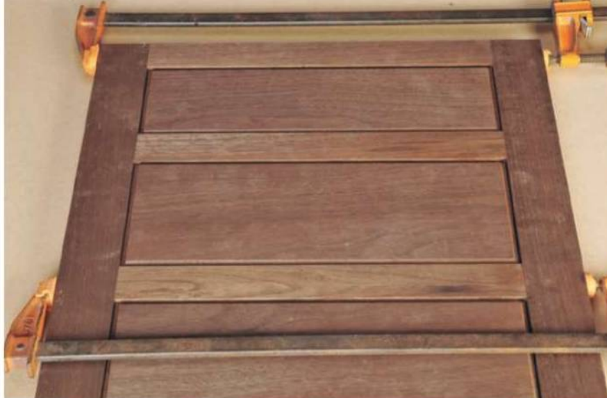
In this frame and panel assembly, the author created a predetermined space around the perimeter of the panels. Although the panels are in the same plane as the frame, their reveals set them apart and add an attractive pattern to the piece.
