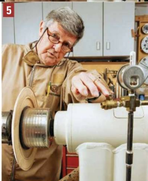
Once the bowl is properly centered onto the vacuum chuck, the next step is to engage the vacuum pump and then release the original chuck — the bowl is now ready to have its base completed.
