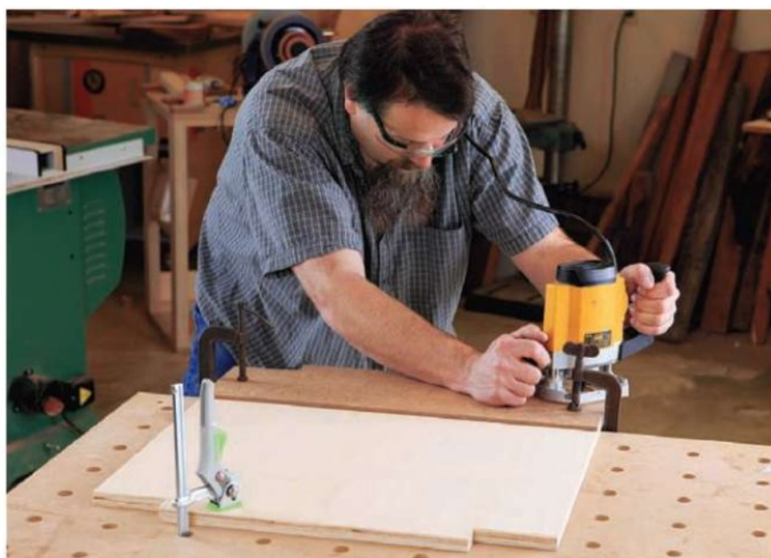
After roughing out the notches on the inner panels, the author pattern-routed the final shape with a 1/2"-diameter pattern routing bit. Its radius perfectly matched the 1/4" roundover bit used on the legs.
