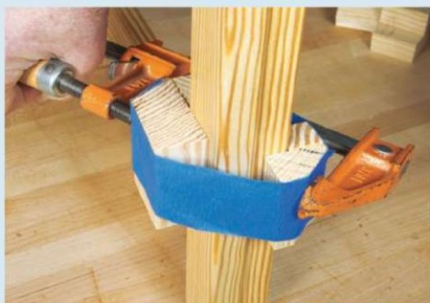
Modified cut-offs from the bench and table legs were used as clamping blocks to aid the process of gluing and clamping the leg inserts securely. The tape holds them in place to aid clamping.
