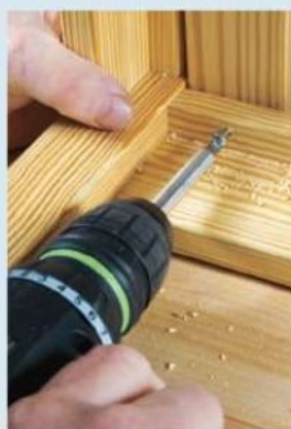
The seat slats are attached from below through a cleat. Come from each end to the middle, using a spacer to keep the gap between slats equal.
