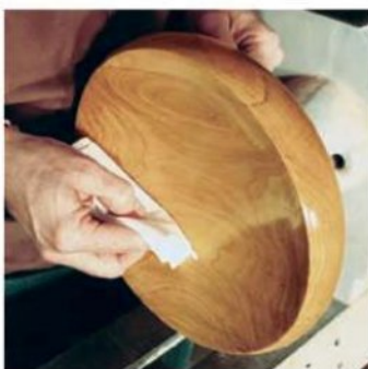
The author applies his liquid friction polish to a spinning maple bowl. As the friction spreads and polishes the product, a smooth, shiny finish begins to appear.
