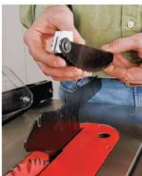
JET's spreader-type riving knife has quick-release provisions for the guard and kickback pawls (left). A bottom storage drawer (right) holds lots of accessories.
