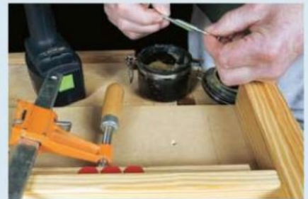
A jig is required to locate and control the bench parts during assembly. After the pieces are clamped in place, pilot holes are drilled and the beeswax coated screws are driven home.
