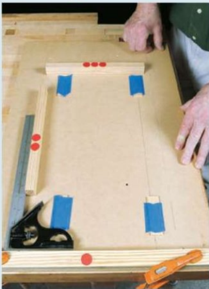
A jig is required to locate and control the bench parts during assembly. After the pieces are clamped in place, pilot holes are drilled and the beeswax coated screws are driven home.
