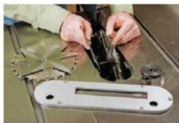
Rikon offers a sliding table accessory for this right-tilting saw (right). A second throatplate insert for dadoing (left) is a convenient standard feature.
