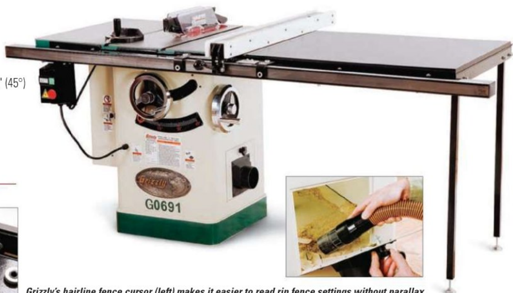
Grizzly's hairline fence cursor (left) makes it easier to read rip fence settings without parallax discrepancies. A handy cleanout door around the dust port (inset) simplifies cleanout chores.
