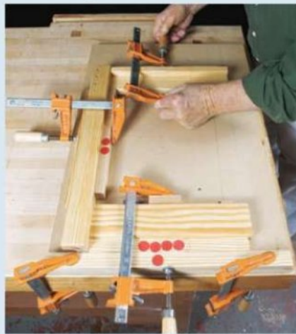
A jig is required to locate and control the bench parts during assembly. After the pieces are clamped in place, pilot holes are drilled and the beeswax coated screws are driven home.
