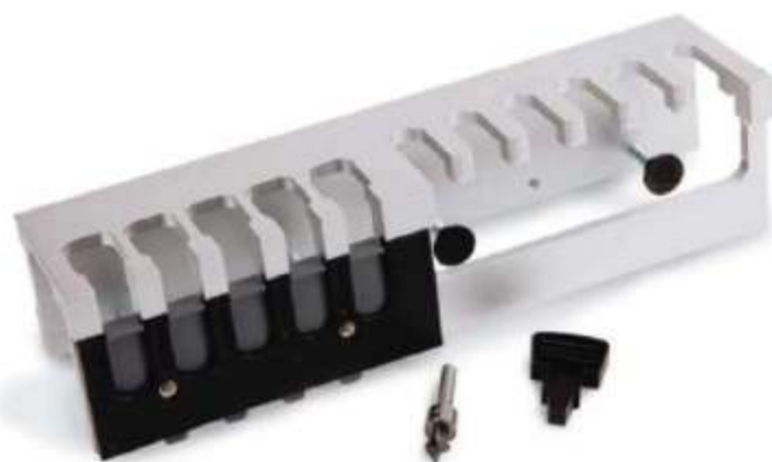
Teeth on the Dovetailer's gray adjuster plate help you register the tailboard for routing using the pin board as a guide. This ensures that the board edges will line up on the finished joint.
