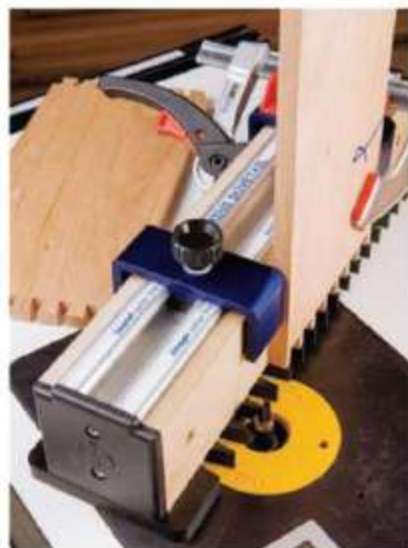
Gifkins's one-piece pin/tail template and wraparound stops (right photo) form a solid platform for routing perfect through dovetails. The author's first test cuts created the box in the left photo.
