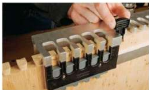
Long runs of dovetails are possible with this jig by snapping in an aligning tool to index the jig for each new set of cuts. Blanket chests or deep drawers are fair game.
