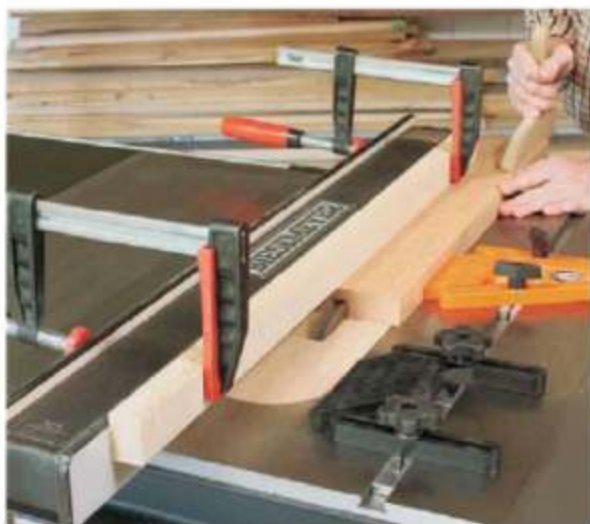
Cut a deep groove into your frame stock for the dentil with a dado blade. A scrap hold-down clamped to the rip fence and featherboards on the table will ensure consistent, safe cutting.
