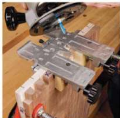
A tab under the pin and tail inserts locks positively into saw kerfs you cut in your custom template. They index the router cuts.
