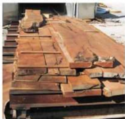
Stacked and staked rough-cut lumber ready to go into the kiln for processing.
