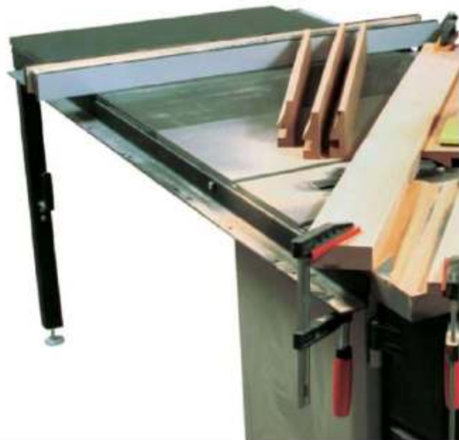
Cut a deep groove into your frame stock for the dentil with a dado blade. A scrap hold-down clamped to the rip fence and featherboards on the table will ensure consistent, safe cutting.
