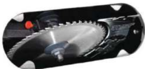
Cut a deep groove into your frame stock for the dentil with a dado blade. A scrap hold-down clamped to the rip fence and featherboards on the table will ensure consistent, safe cutting.
