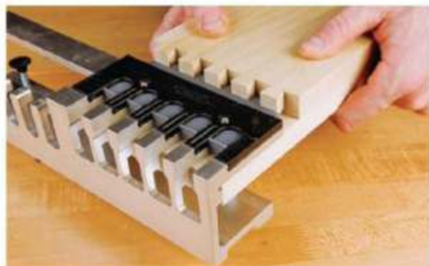
Teeth on the Dovetailer's gray adjuster plate help you register the tailboard for routing using the pin board as a guide. This ensures that the board edges will line up on the finished joint.
