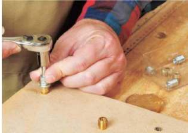
After temporarily screwing a bolt into the threaded insert, a socket and ratchet wrench drives the insert into the hole in the side of the horizontal router table's base.
