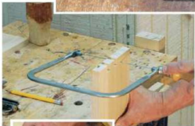
After defining the sides of the tails with a backsaw, the author removed most of the waste with a coping saw before finishing the opening by paring the cut to the baseline. After cutting the tails, the author holds the drawer side in place and marks the pins.
