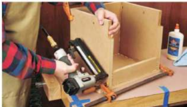
A pneumatic nail gun makes quick work of assembling the router table's MDF base, keeping the glued parts aligned and together while clamps are put into place.
