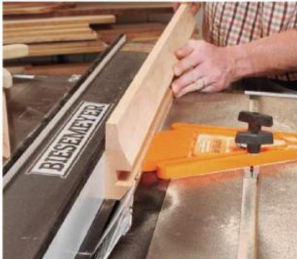
Rip a bevel to form a pleasing transition between the dentil groove and the inside edges of the frame. It's a really good idea to use a featherboard to help control these on-edge cuts.
