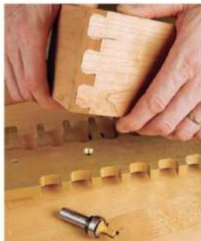
An optional template and special "organic" bit form these unique, radiused half-blind joints.
