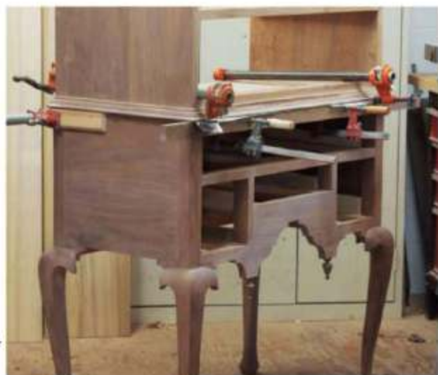
The author first glued and nailed in place the two side sections of molding, resting them on the blocks he'd clamped to the case (process described in the story's text). He then glued the front section into place, clamping it as shown here.
