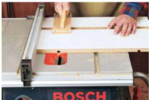
Cut a pair of grooves into the bottom of the router's tilting table top using a dado blade in the table saw (top photo). These house the plywood compasses. To mount the top to the table's base, studded hand screws are installed through the curved slots and screwed into the threaded inserts you installed earlier.
