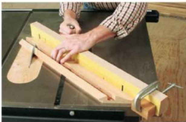
You'll better your chances for perfect-fitting miter joints if you tune up your miter gauge and use a long, stiff, auxiliary fence. Add a sandpaper facing and use a stop block for even more precision.
