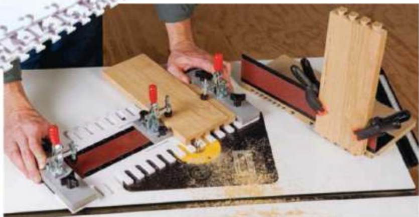
A wide jig base faced with sandpaper and three supplied toggle clamps hold workpieces securely for router table use. A right-angle fence mounts on the jig to rout pin boards vertically.
