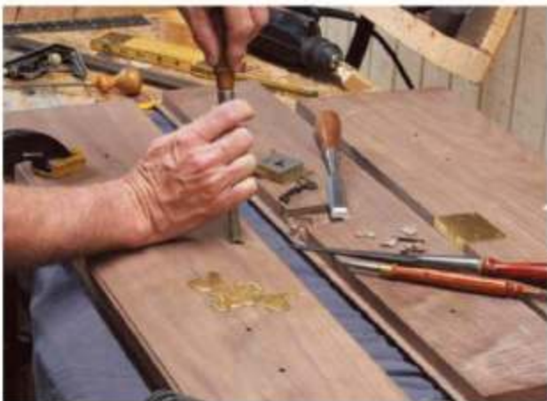
It's easier to cut the mortises for the lock hardware before the drawer components are dovetailed and assembled. Here, the author is cutting the notch for the key's tooth with a chisel.
