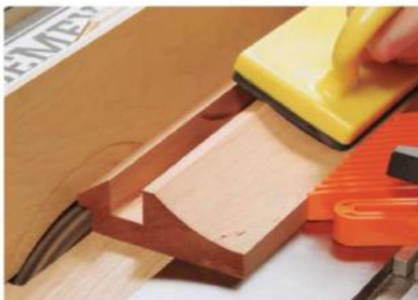
Cut a rabbet along the beveled edge of the rail and stile blanks using your dado blade buried in a sacrificial fence. This rabbet will house the picture frame's photo or print, glass and backer board.
