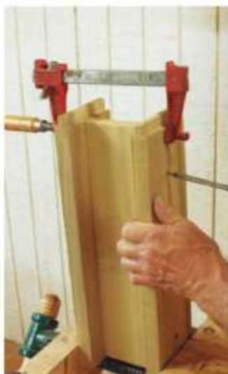
Solid wood case sides expand and contract in response to seasonal changes, so the drawer runners must be fastened in a way that permits movement. The front end of each runner's tongue fits a groove milled into the drawer rail. The back end of the runner is secured with a single fat woodscrew turned into the side of the case. The piece of 3/8"-thick scrap holds the runner back as you set the screw (middle photo).
