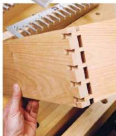
Keller jigs have proven themselves in pro shops for more than 30 years. Once they're set, you'll rout crisp dovetails with little fuss.
