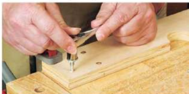
A socket and ratchet wrench, set onto a pair of nuts, drive the hanger bolts into place. These hanger bolts attach the router plate to the crossmember on the base.
