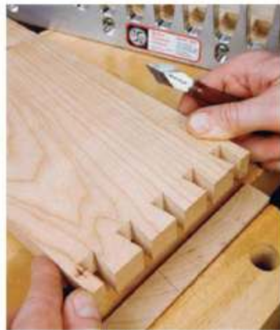
Registering the pin board for accurate joint alignment is as easy as holding the boards together and knifing a pair of tail lines onto it.
