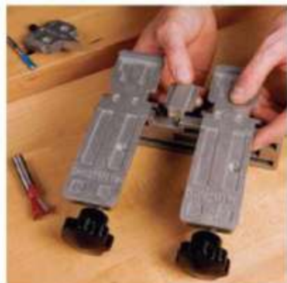
Changing over the ChestMate between pin and tail cuts is easy: loosen the jig wings and slip in the appropriate pin or tail insert.
