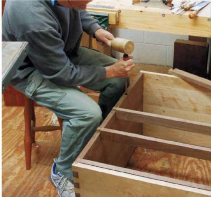
Each of the 2"-wide drawer rails on the upper case is held in place with a 1"-deep dovetail. The author cut the tails by hand with a backsaw, then marked the tails onto the front edge of the case sides and cut the dovetail sockets with a chisel.
