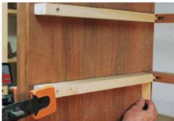
Solid wood case sides expand and contract in response to seasonal changes, so the drawer runners must be fastened in a way that permits movement. The front end of each runner's tongue fits a groove milled into the drawer rail. The back end of the runner is secured with a single fat woodscrew turned into the side of the case. The piece of 3/8"-thick scrap holds the runner back as you set the screw (middle photo).
