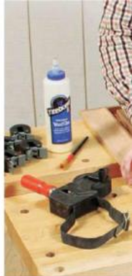
The author reinforced the miter joints on the outside edges of the frame by pulling them tight with a band clamp.
