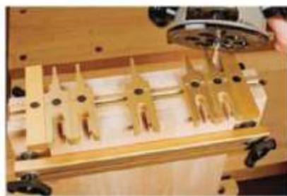
Adjustable tuning forks guide Sommerfeld's piloted bits to create variable-spaced dovetails. The forks set both pin and tail cuts.
