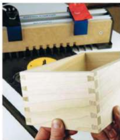
Gifkins's one-piece pin/tail template and wraparound stops (right photo) form a solid platform for routing perfect through dovetails. The author's first test cuts created the box in the left photo.
