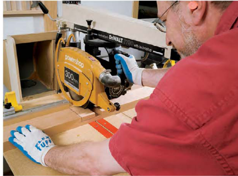
Half-lap joints are used where the base's foot-end cantilevers overlap. I cut these using my radial arm saw and a dado blade. A similar table saw setup would work fine.
