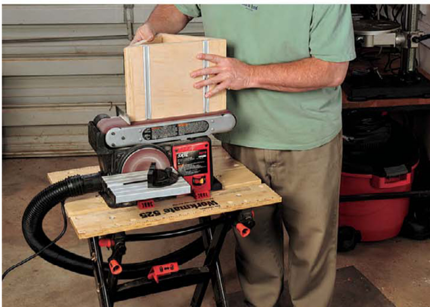
The author recommends a combination belt and disk sander as an essential benchtop tool for a small woodworking shop. Few projects will leave your shop without touching a power sander.
