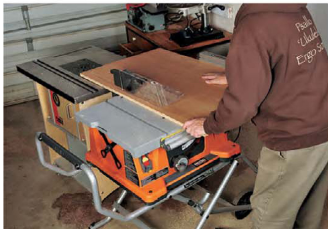
A cabinet-style router table can be used for storage, a work table and also as an outfeed table for your table saw. Small-shop owners need to allocate their floor space carefully as they outfit their shops.
