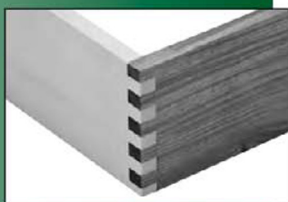
Finger and Lap Joints
