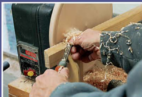
Use the point of your skew to push thin layers of material across the outside diameter of the candlestand top, working from right to left (top photo). This passive style of turning simplifies — and makes safer — the process of working a surface spinning past a tool at high rim speed. The author uses a spindle gouge reground with a long tip to hollow out the excavation inside the lip that surrounds the top (bottom photo).
