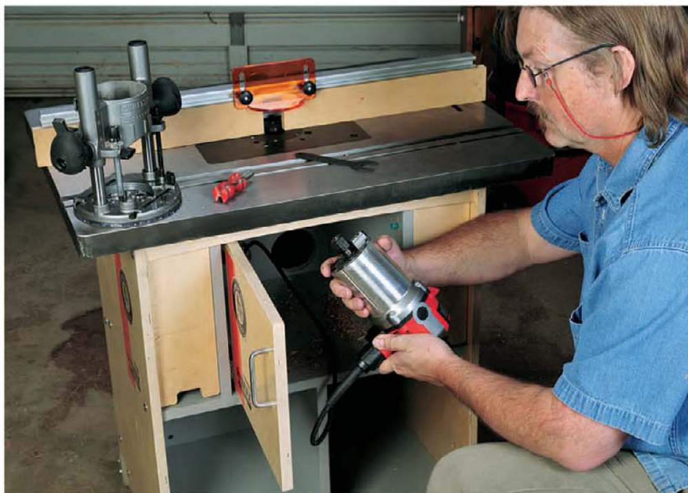
Bench Dog's cast-iron topped router table is the top of the line when it comes to under-the-table mounted router woodworking. Or remove the router to do a variety of tasks as a handheld tool.
