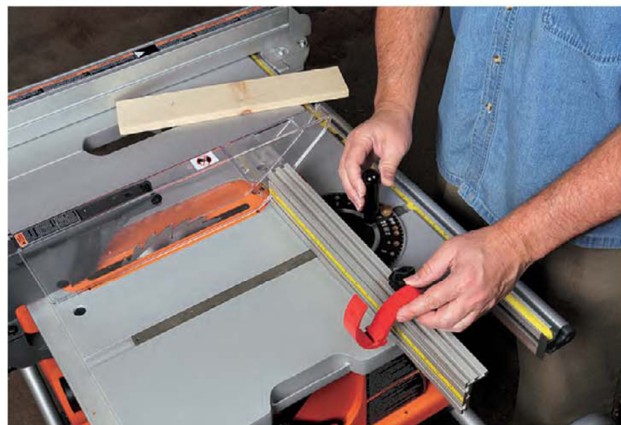
For accurate mitering and crosscutting, the author recommends upgrading your saw with an aftermarket miter gauge with long fence and flip-down stops.
