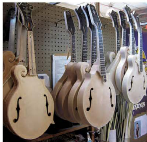
Specialized hand work, like the installation of bracing (top) is performed by individual luthiers. Mandolins at various stages of construction (above) await the next step toward completion (left).
