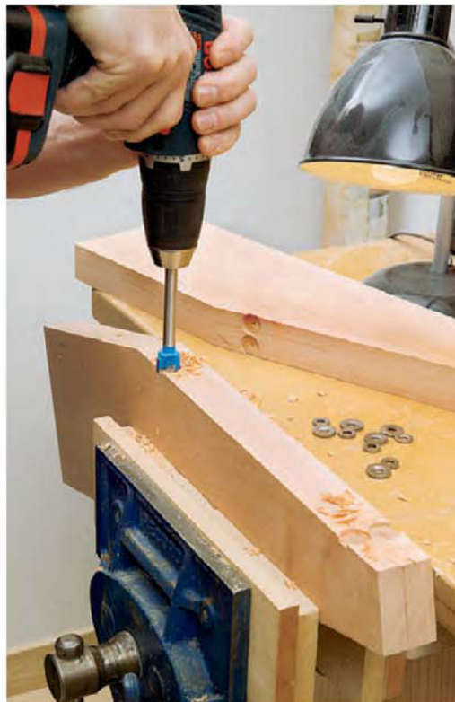
Drill the counterbore holes for the desktop fasteners in the headboard supports. A 3/4"-diameter Forstner bit works well for this task. Drill the hole depths so the fasteners seat flush.
