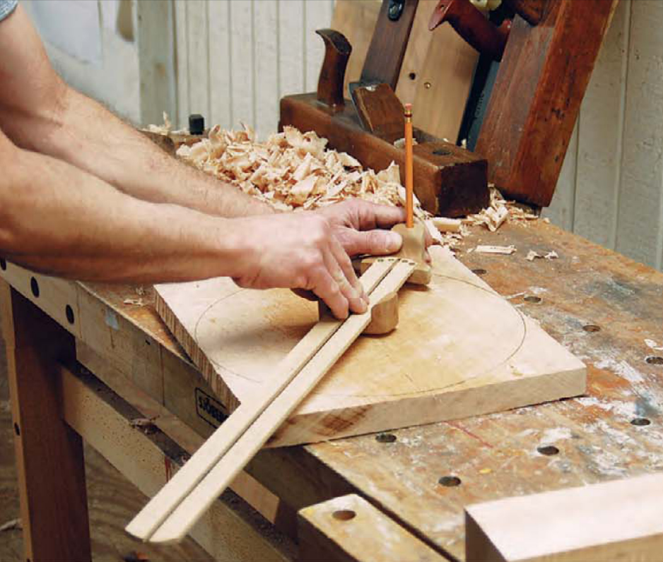
The author uses a shop-made beam compass to draw the outside diameter of the candlestand top. Instead of bringing this blank to final thickness right away, he recommends planing and flattening the top in stages to help minimize warping.
