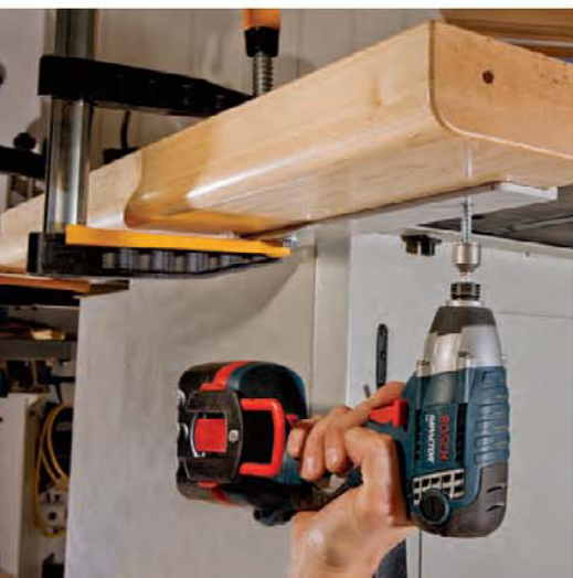
Clamp and then bolt the mounting plate to the saw's fence rail with five 2" lag screws and washers. Keep these fasteners well clear of the miter slots you'll need to rout later.
