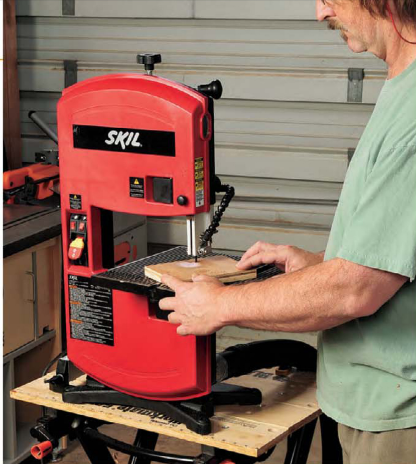
Sometimes you just don't want to cut a straight line. Here, the author uses a benchtop band saw that can cut delicate scroll work or slice through 3½" stock — and many tasks in between. While it can't handle really heavy-duty work, it can be a small-shop workhorse.
