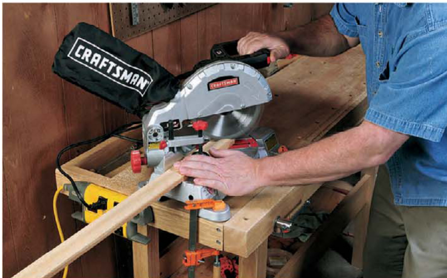
A power miter saw, also known as a chop saw, makes quick work of cutting long stock down to size, forming accurate miters and making repetitive cuts. While a table saw can cut miters, this saw can be set up for specific tasks and be a timesaving addition to a small shop.
