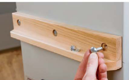
The leg stops here: it's simply a wooden ledge fastened to the saw cabinet with three short carriage bolts set into counterbored holes.
