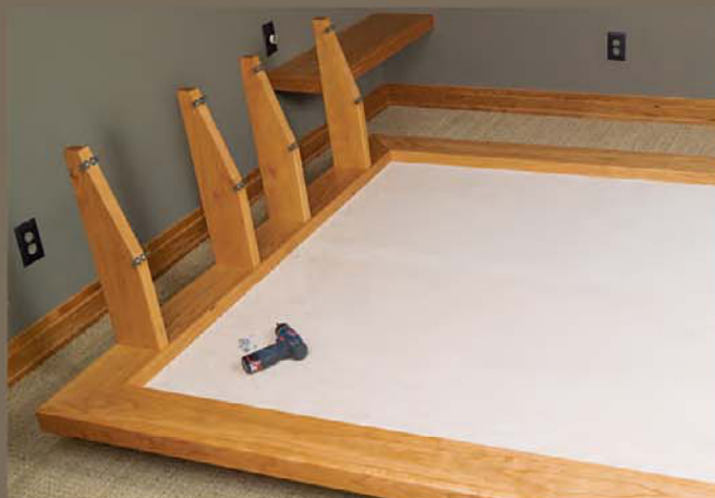
Set the platform on the base so initially it overhangs the head end of the base about 8 inches. Align and attach the headboard supports. Align and screw the platform to the base, and then attach the headboards.
