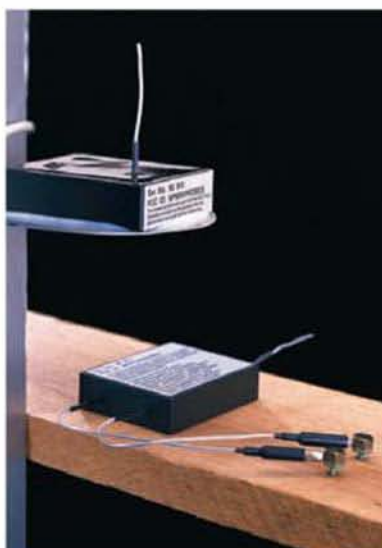
Computer technology is central to Lignomat meter systems. Shown here, a wireless transmitter with probes passes MC readings onto a receiver connected to a personal computer that displays the data. Wireless probes can also measure temperature and EMC values.
