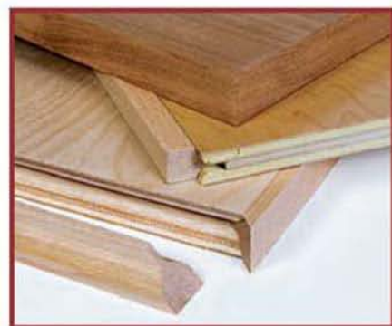
Edge-band bits that mill both the plywood and the edging produce stronger-than-the-glue joints that align positively. Easy and effective.
