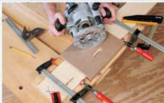
The author used a slotting jig, rub collar and straight bit to mill four slots in the fence back for the through bolts. Two rails under the jig made for easy alignment and clamping.
