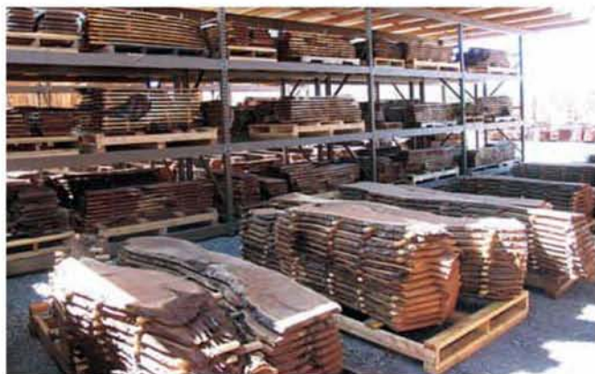
Each tree of velvet mesquite — shown stuck up in flitches in the Arizona sunshine — produces beautiful one-of-a-kind lumber. You would do well to keep individual stock pieces' shape in mind during a project.
