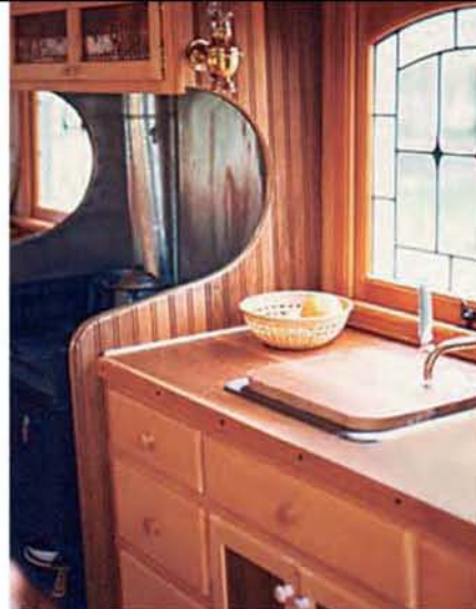
The author uses marine woods (spruce, cedar, fir) in his wagon interiors for durability and longevity.
