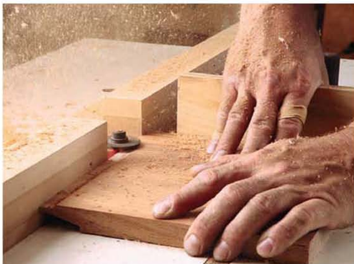
The chips flew during the panel-raising process. The author anchored a shop-made fence to the router table with screws. The large diameter panel-raising bit had a back cutter that formed a clean shadow line around the face of the panels.
