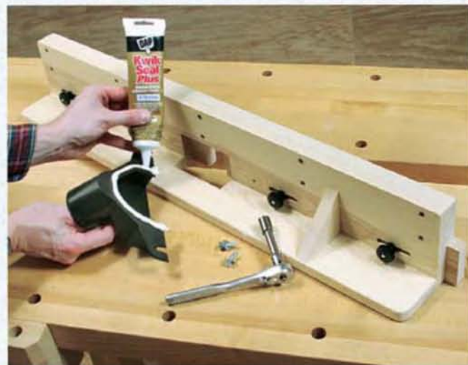
Squirt a bead of caulk around the contact surfaces of the dust port before mounting it to the fence back with short lag screws.
