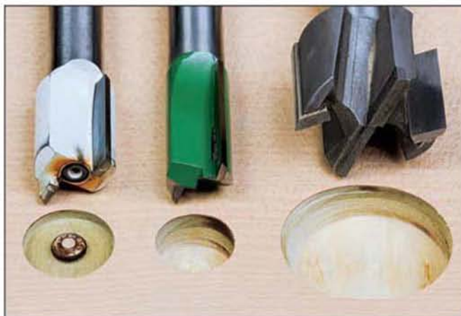
Not all straight bits are created equal, at least when it comes to plunge cutting. Bill Hylton helps us identify proper plunge-cutting bits.
