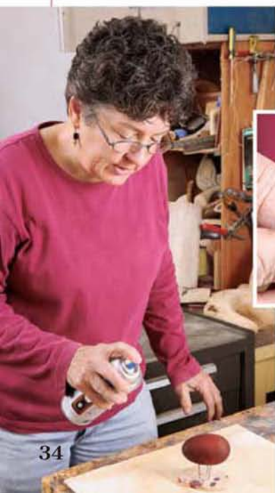
Spray finish seals the wood but leaves pores open. If the finish runs in one spot, use a pin to prick open the pore holes. Sand with steel wool after finish dries.
