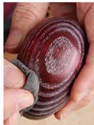
The author wears gloves to apply liming wax, a petroleum-based product that can penetrate the skin. Steel wool removes wax residue.
