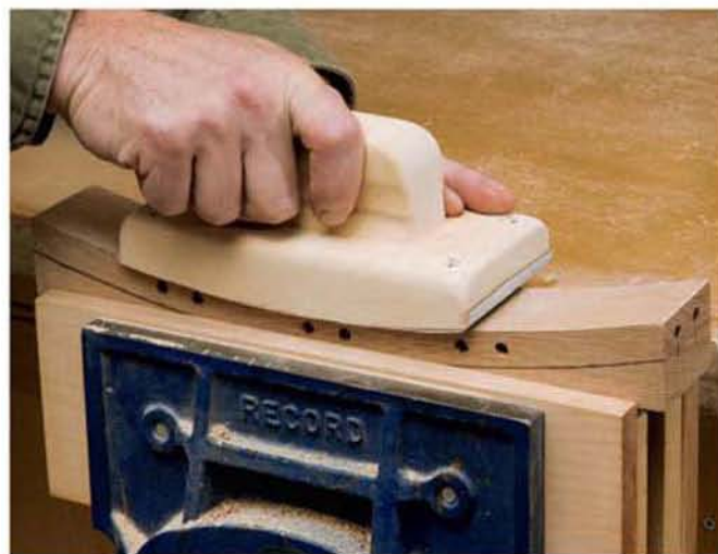
Sand the inside faces of the crest and seat back rail with a curved wooden sanding block.
