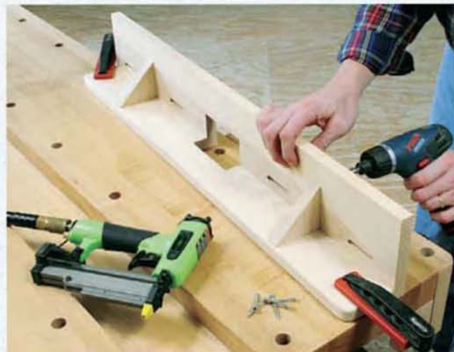
Use glue and pin nails or brads to assemble the fence back, base and braces. Check to make sure the back and base form a 90° angle, then reinforce the glue joints with countersunk screws.
