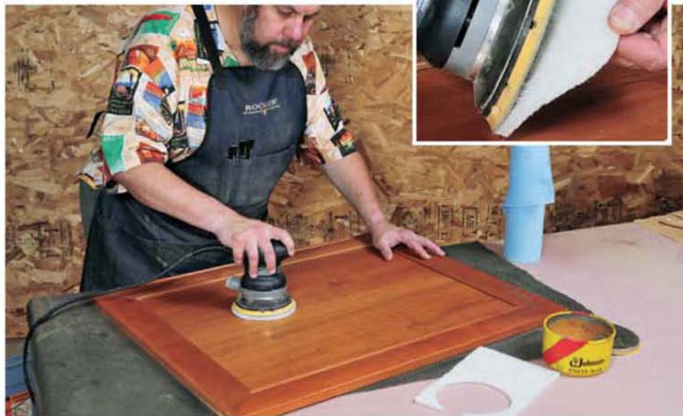
A white nylon abrasive pad, paste wax and paper shop towels are key components in what Michael Dresdner likes to call power waxing. It works no matter what choice of topcoat or application method you use.
