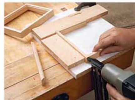
The shelf frames were pinned together at their mitered corners. Then, the plywood tops and bottoms were cut to fit the frames.
