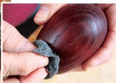
Spray finish seals the wood but leaves pores open. If the finish runs in one spot, use a pin to prick open the pore holes. Sand with steel wool after finish dries.
