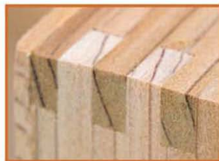
Close-up of box joint in a small cedar box.
