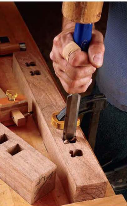
Nothing beats a sharp chisel when it comes to cleaning up and paring a mortise square. Form the mortises first, then the tenons.
