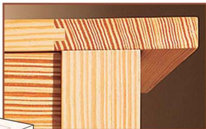
This photo shows the back view of the illustrated joint at left. The top's stub tenon is clearly shown.
