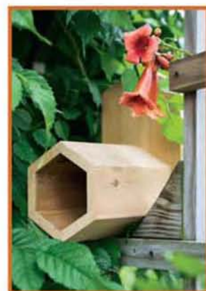
Western red cedar wren house made with a bird's-mouth bit.
