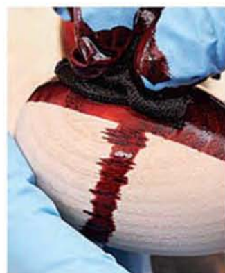
Saturate your project's wood with a dye for a deep color. Let the piece dry several hours — the author usually lets hers sit overnight.
