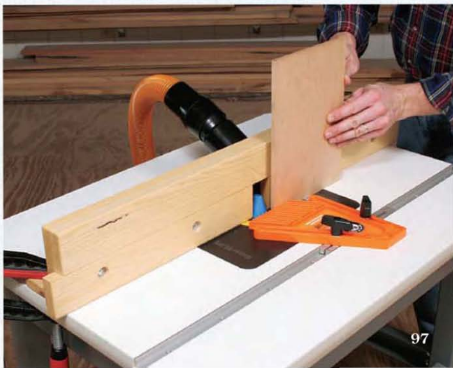
Squirt a bead of caulk around the contact surfaces of the dust port before mounting it to the fence back with short lag screws.
