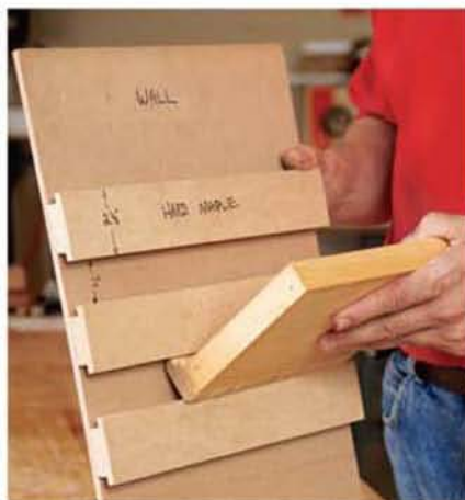
The wall shelf system project began with a mock-up to establish the proper dimensional relationships between the various moldings.
