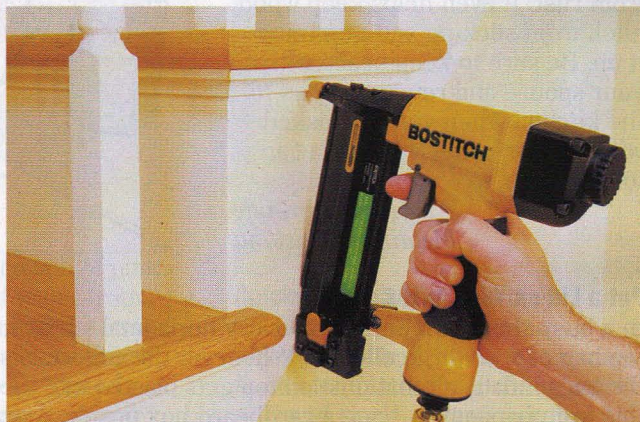
Nailer depth setting vs. the thickness of your wood: A good rule of thumb is to use fasteners three times the thickness of your wood.
