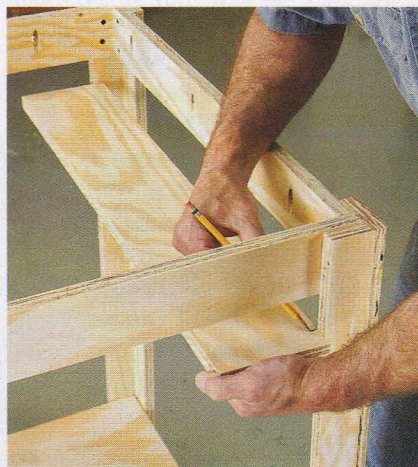
Mark, don't measure, to ensure a perfect fit of the drawer rails between the leg posts.
