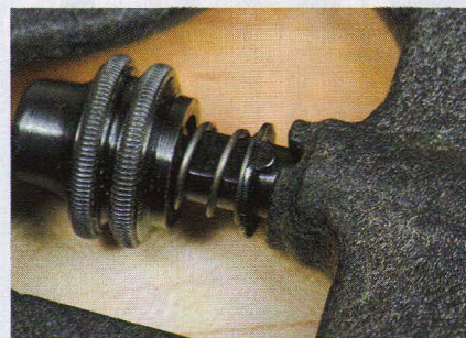
A lock bolt with a tabbed washer that slides onto flats ground onto the bolt and locks into the head is easiest to use. When the blade is removed, the bolt assembly drops — it won't fall completely out — and frees the tabs from the head, allowing the bolt to be rotated. You can do it without really looking. Lock bolts are used on Starrett and Rockler squares.
