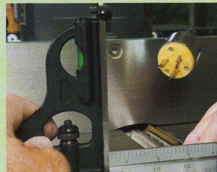
Verify the set of your jointer knives and the infeed and outfeed table alignment. Often overlooked, this task improves results.
