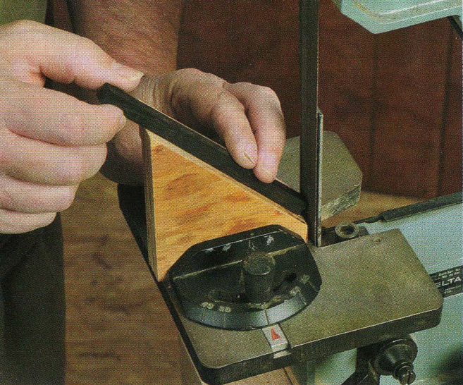
Using a plywood jig screwed to a miter gauge, the author uses a strip sander to chamfer both ends of a square "log" before cutting off short square plugs from each end.
