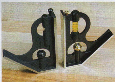
A cast-iron head is essential for long-term accuracy, but it's more expensive to produce. The die-cast zinc head from a trade/consumer-grade square (right) is lighter weight and softer.
