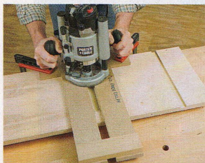
Plowing stopped and through dados in the cabinet sides was easy work, using a slotted router jig to guide a 1" O.D. rub collar and undersized 23/32" plywood-cutting bit.
