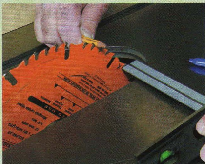
You can check your table saw's table and blade alignment with a combination square. It's a two-step process.
