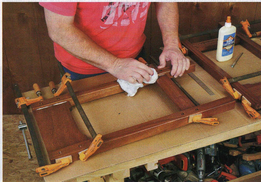
As with the original two pieces of this set, all the table parts are stained and finished first, prior to assembly. Glue-up is done in two stages: First, each pair of side aprons and stretchers is glued up with a pair of front and rear legs into a subassembly, as shown here. The subassemblies are then glued together.
