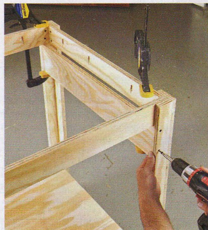
Glue and screw the drawer rails in place, holding them tightly to the bottom of the upper frame.
