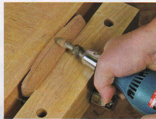
A rotary rasp chucked in a die grinder makes quick work of sculpting the curved sides of the table's drawer pull.
