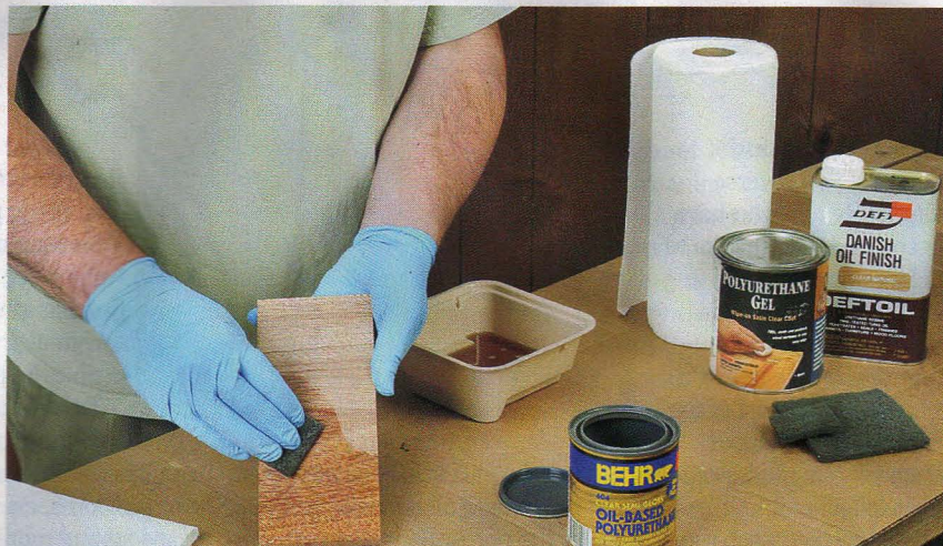
Polyurethane gel, Danish oil and wipe-on poly, as well as standard oil-based polyurethane used unreduced and straight from the can, all work great as wipe-“off” finishes.
