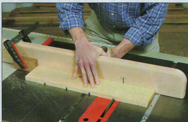
The author used a simple crosscutting jig made from two miter gauges and a long fence to cut the shelf dados. A stop block sets each dado position. Cut the dados on both side panels before resetting the block.
