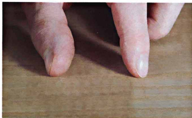
The area between the fingers is a "snipe." You can see in the right foreground where mill marks have been removed by the handplane.
