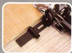
Automatic indexing without measuring
