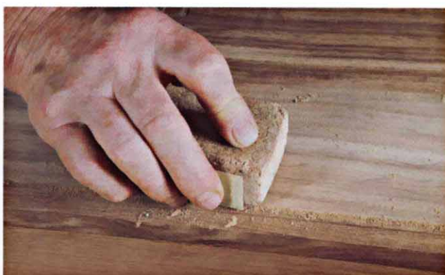
When using a sanding block (the author prefers cork), hold the block flat with constant pressure. Don't let more than half of it overhang an edge.
