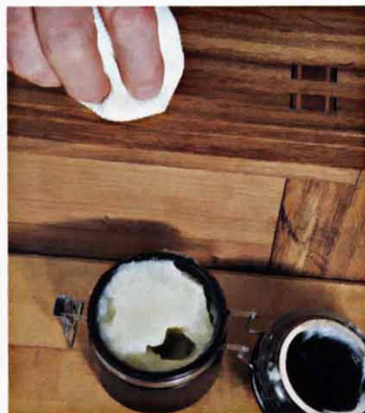
A variety of waxes are widely available. My preferred, and homemade, version is made from a pure bleached granulated beeswax dissolved in pure turpentine and made as soft as summer butter.
