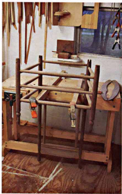
Cutting the rocker notches requires a combination of cleats and clamps to hold the chair secure as the notches are formed.
