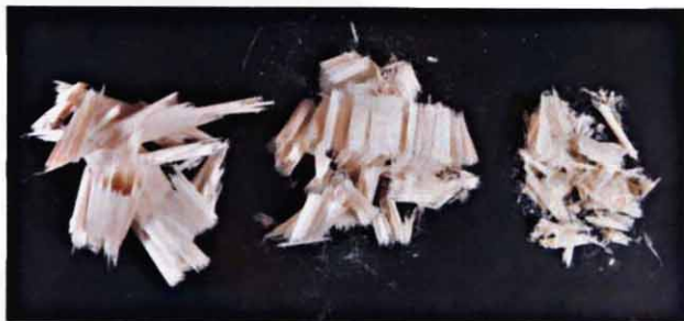
Three types of shaving are made as you refine the surface by planing across the grain: first shavings (left), feathers (middle) and finally, down (right).
