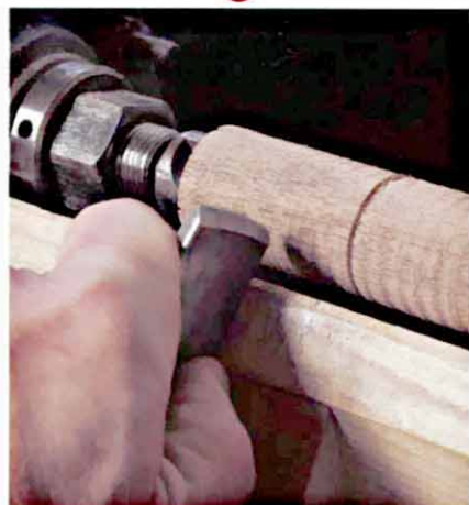
The author transfers the lengths of the rungs from the story sticks directly onto his wooden tool-rests, then to the work with a skew chisel.
