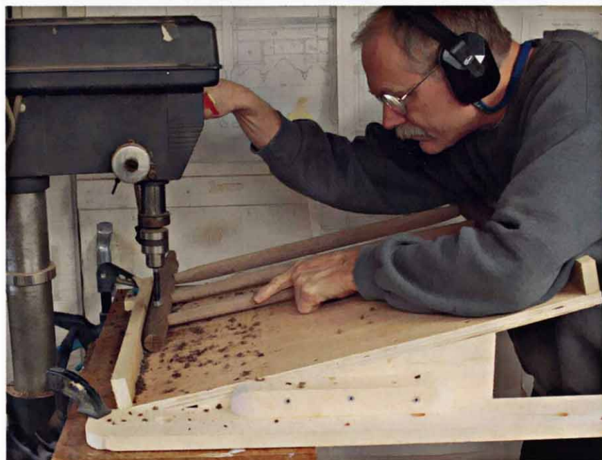
After you've glued your front ladder together, set up the side-rung-mortise jig (SRMJ) as shown so that it will bore a 15/16"-deep mortise in the center of the posts. Then drill the three side-rung mortises in one post, turn the ladder around, and drill the three side-rung mortises in the other post. Next, rotate the jig 180 degrees on your drill press table and drill the side-rung mortises in the back ladder.
