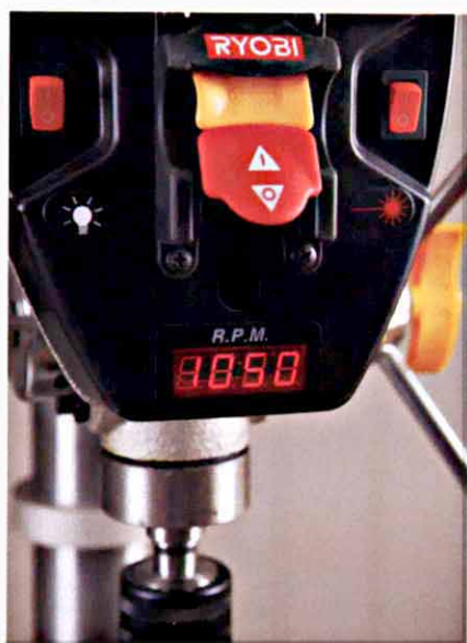
Digital readout makes variable speed even better. Now you'll know the exact chuck speed so you can adjust it as needed.
