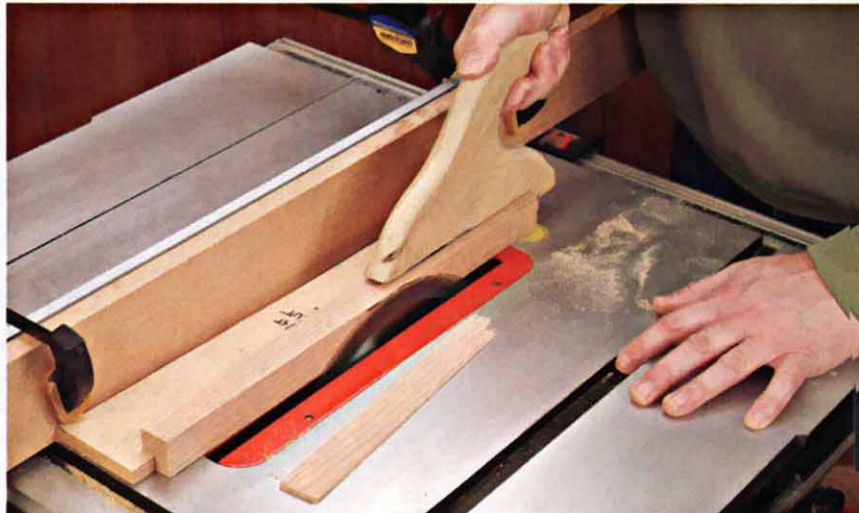
To make a tapered leg, make the first taper cuts using the shallow notch of the jig to taper adjacent sides. The clamped-on auxiliary fence shown here extends the length of this table saw's short rip fence to support the entire length of the cut.
