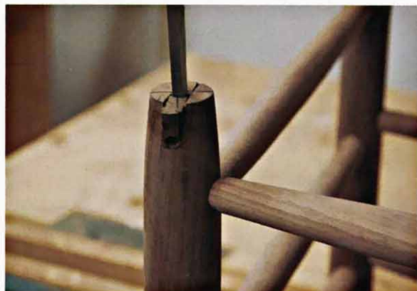
To form the rocker notches, first define the sides of each notch with a thin backsaw. Then drill through the posts with a 3/8"-diameter bit at a position that will become the bottom of the notch. Finish by splitting out the waste with a chisel and paring the walls as needed.
