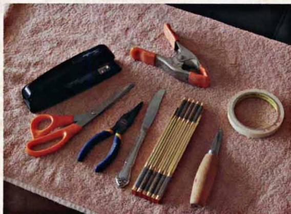
The tools you'll need for weaving include a desk stapler, scissors, needle-nose pliers, spring clamp, measuring tape or folding rule, sharp knife, butter knife and masking tape.
