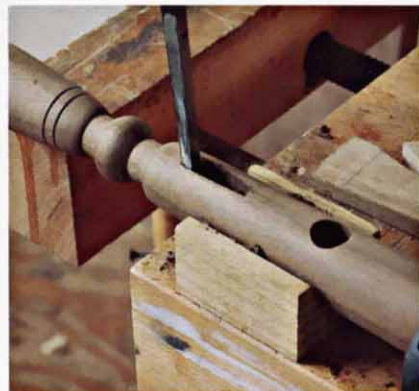
Chop out the crest rail mortises in the back posts with a 1/4" mortising chisel. Make the mortises 9/16" deep and 1 1/2" long. Use a curved support to brace the post from below and to keep it from twisting.
