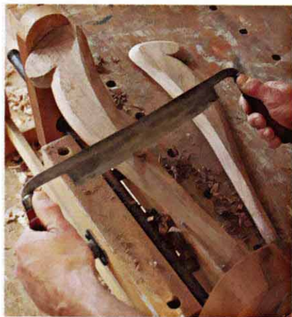
The author turns to a drawknife, rasps and sanding to shape the edges of the arms. Pencil lines establish the transition areas.
