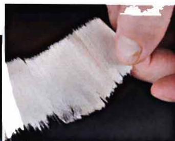
A typical cross grain shaving (above), showing the slightly curved blade.
