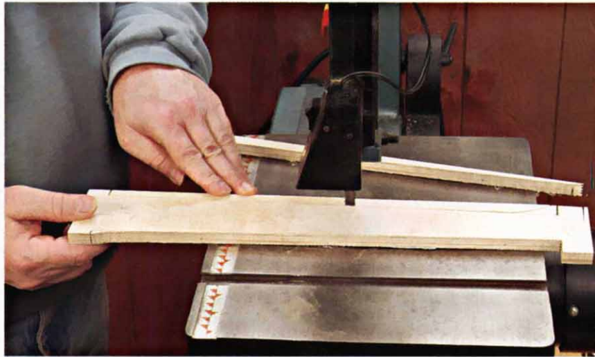
Making the multi-sided tapering jig requires two differently sized notches; the second notch is deeper than the first to ensure that the taper cut on the opposite edge is cut correctly. Always test your jig on scrap lumber to be certain of its accuracy.
