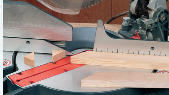
Rip two fence strips to width from straight-grained stock, then miter cut one end of each to 45°.
