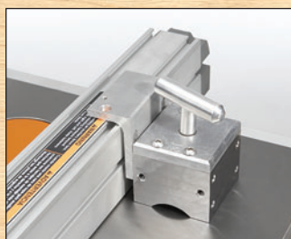
A MagSquare used to attach a bracket to a support fence.
