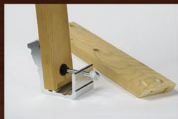
Clamp wood in jig
