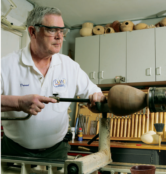
Dave Morrical demonstrates how to end-grain hollow a vessel. Depending on how narrow the vessel's opening is, much of this work is done "blindly" and by feel. It's a skill that can only be honed by many hours of practice.
