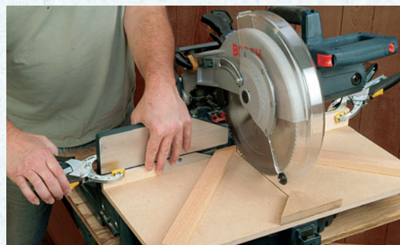
To prepare the the jig for use, lower the blade into the kerf slot to register position. Then you can clamp the cleats to the saw fence.
