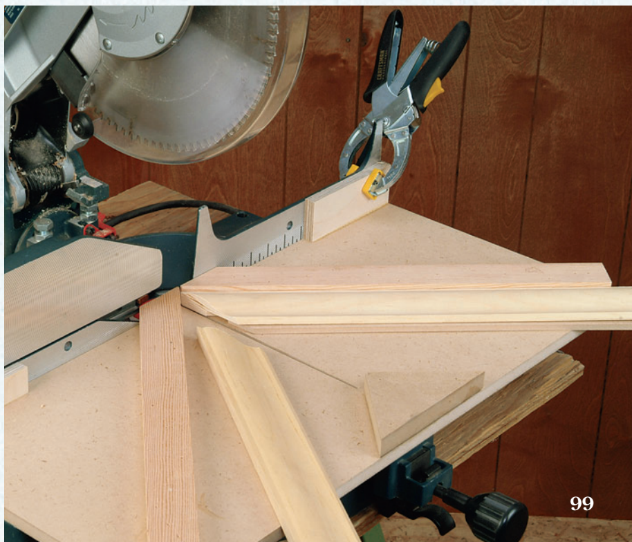
To prepare the the jig for use, lower the blade into the kerf slot to register position. Then you can clamp the cleats to the saw fence.
