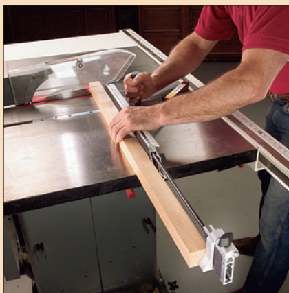
An extendable fence provides support when you're cutting long pieces. It allows you to use the stop to cut multiple pieces to the same length.
