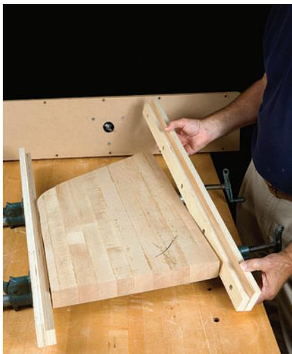
**Make up a pair of support tracks and fasten or clamp them on either side of the blank. Attach a narrower ledge to the inner face of each track to provide clearance so you can mill to the blank's edges without hitting the tracks.**
