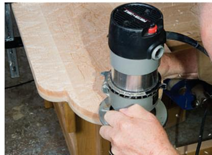
The Freud spiral bit left a very smooth edge. With a shank-bearing bit and an end-bearing bit, you can shape the top in fine style.
