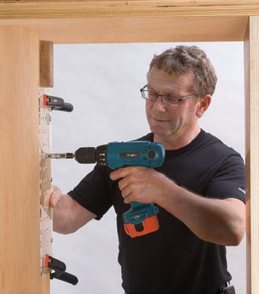
**There's no way around it: shelf-pin holes are tedious to drill. A drilling jig at least ensures they'll all be evenly spaced when you're done.**
