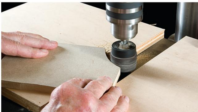
The templates, after they have been shaped by a band saw or its like, must have their shapes refined (here with a drum sander) to the marked lines.
