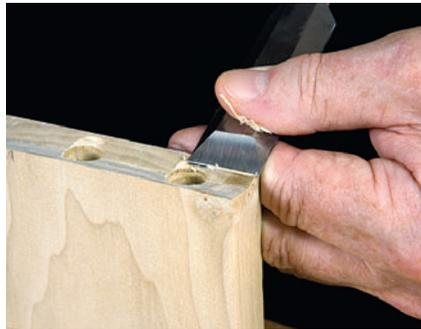
With the V formed, get to the desired angle by chiseling from the face of the rail down the slope of the V.
