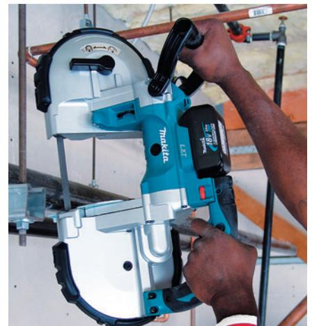
The higher power and lower weight afforded by Li batteries have led to some tools you may never have seen before. At left is DeWalt's cordless circular saw featuring an industry-first 7/8" blade; at right is Makita's 18-volt cordless band saw.
