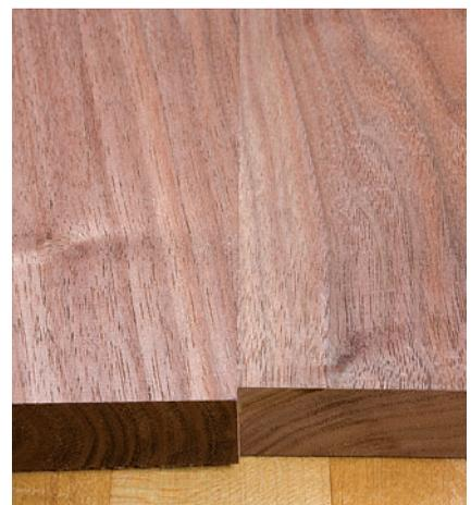
These router-jointed edges are as square, smooth and chip-free as you could make on a jointer. As you can see, the glued joint is virtually invisible.
