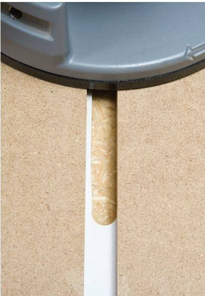
As you guide the router along one fence, the cut is immediately adjacent to that fence's base. The cut is completed to the full desired width on the return pass.
