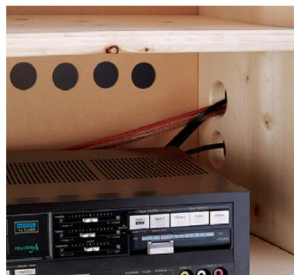
Pass-through holes are the easiest way to keep wires organized and tangle-free. Drill holes large enough to fit the cord plugs. You'll also need to drill ventilation holes through the back to keep components from overheating.
