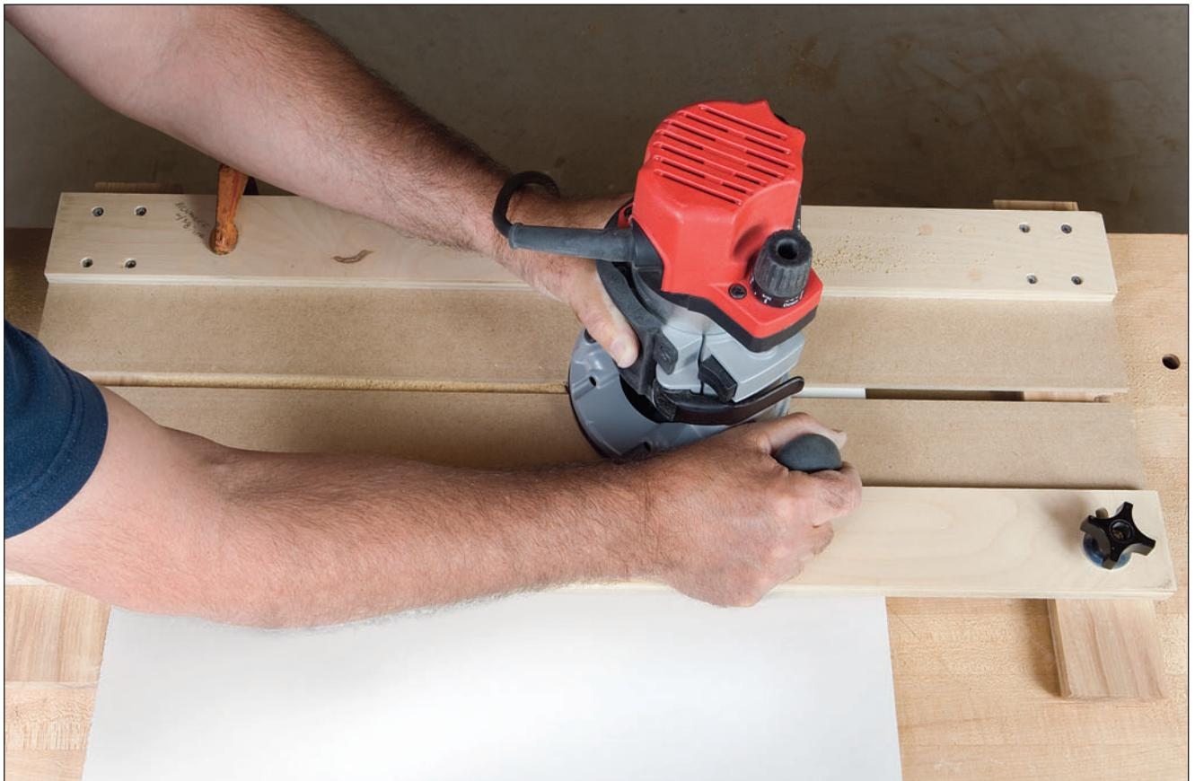
Set the router on the jig with the bit in the gap and clear of the work. Pull the router along one fence, then push it back along the other to mill the dado. The fences keep the router from wandering off course so it cuts the dado to the exact width you require. It doesn't get much easier.
