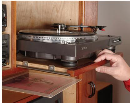
The author keeps his prehistoric turntable on a pull-out shelf mounted on full-extension slides (above). Adjustable shelves (below) allow you to change components without building a new cabinet.
