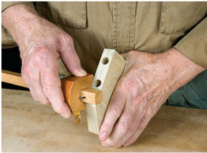
Start the process by marking the end of the rail with a center line, using a marking gauge.
