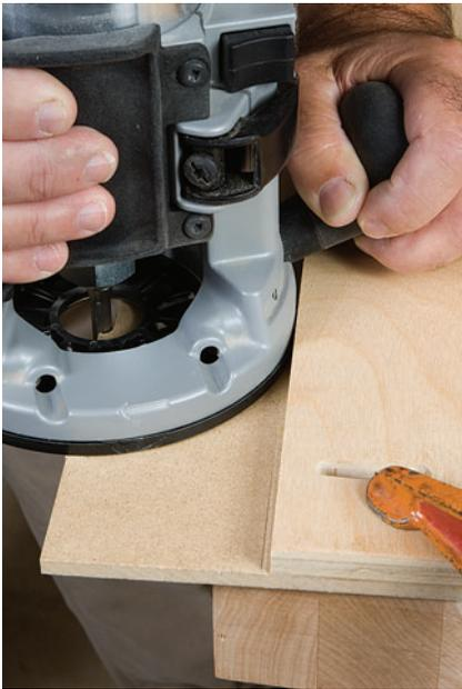
The critical step to building the jig is trimming the fence bases with the router and bit you'll always use with the assembled jig.
