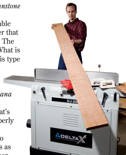
**When face jointing a board, the cutterhead of the jointer must be at least as wide as the board you are flattening.**
