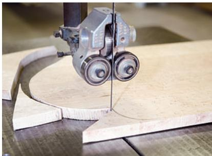
Saw close to the layout to line to help prevent chipout or tearout when you template rout to the line. Get within 1/16" or less.
