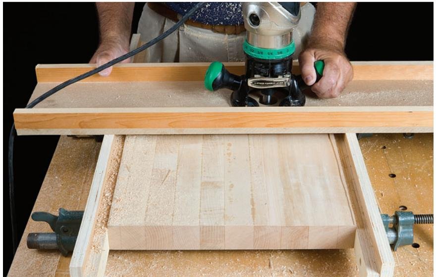
**Router surfacing will require a sled that's more than twice as long as the workpiece is wide so there's plenty of overhang on the tracks. Milling the surface involves moving the router and sled back and forth along the tracks, methodically widening the surfaced area.**
