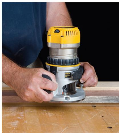
Guide the router along the fence, in the correct left-to-right direction, to mill it clean, square and straight.
