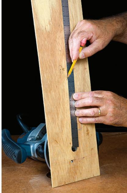
Measure from the bit and mark the pivot point. Drill a hole at the spot for a pivot nail or screw. The bit is outside the radius if you want a disk, inside it if you want a hole.
