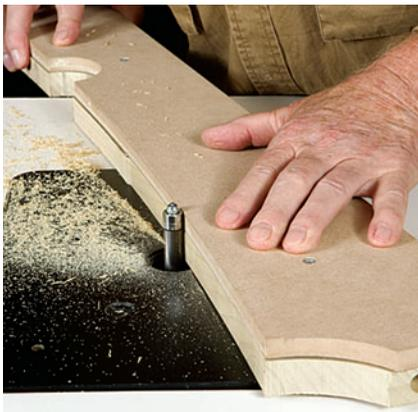
**Using an upcut spiral bit, the author was able to remove the excess as shavings, leaving a smooth, clean-cut top rail.**
