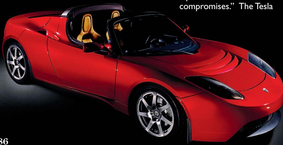
roadster (launch date: mid-2007) will be powered by a 3-phase, 4-pole AC induction motor that can deliver up to 248HP — charged by 6,831 small (AA-sized) lithium-ion cells. A home-based charging system is included with the vehicle and is installed in the garage of the purchaser by a qualified electrical technician. For info, visit [www.teslamotors.com](http://www.teslamotors.com).
