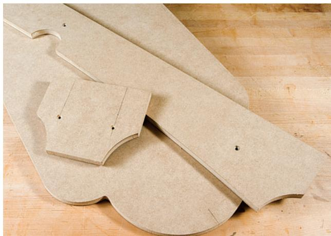
All the required templates are made and refined. In addition to providing accuracy as you shape your stock, these patterns can be used repeatedly.
