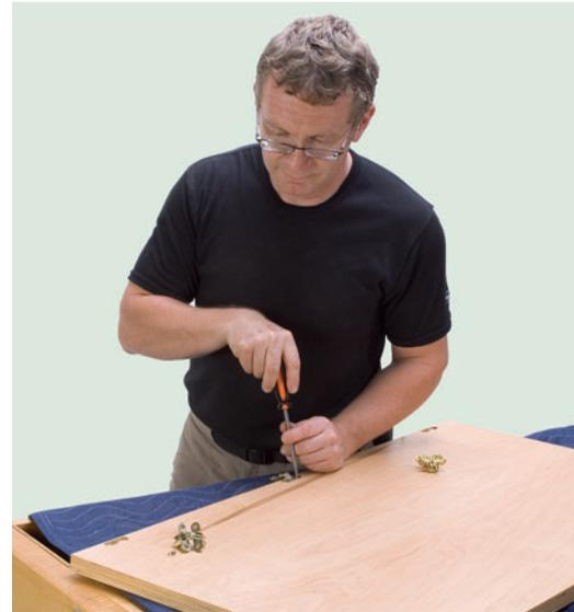
Soss hinges. Installing the Euro hinges on the center doors was a simple matter of drilling the appropriate holes and mounting the hinges. Installing the Soss hinges was quite another matter. You can buy templates for routing Soss hinges. I prefer to use my own shop-built jig. In any case, be extremely careful as you rout out the mortises for these hinges. You basically have one shot to do it right ... practice on some scrape wood!
