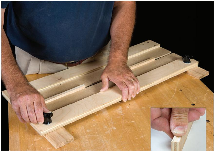
Slip a couple of scraps as thick as the dado you want to cut between the fences. Squeeze the fences tight, then tighten the knobs on the adjustable fence. You'll get a perfect, snug fit.
