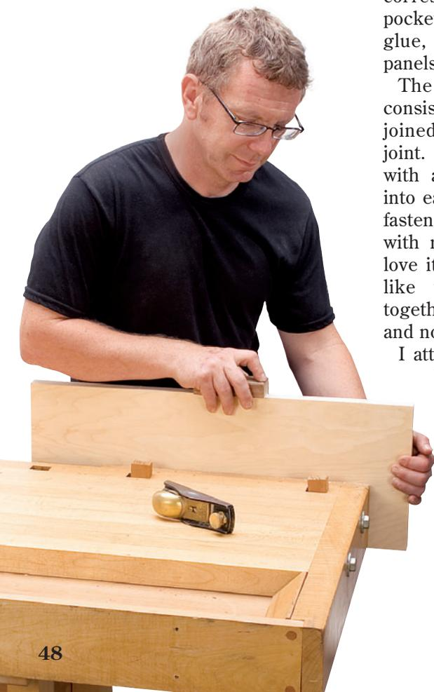
**Use a sharp block plane, followed by careful sanding, to clean up saw marks on the exposed plywood edges.**
