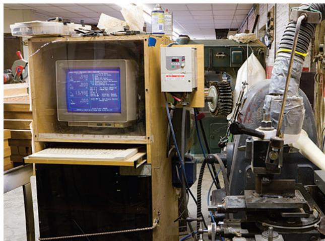
**This converted Wadkins lathe has a lead screw and a stepper motor. This means that if you can electronically tell the cutter where to move in space, it will cut (turn) a leg for you — the power of CNC!**
