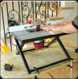
Motor transitions easily to the fixed base for table mounted applications.
