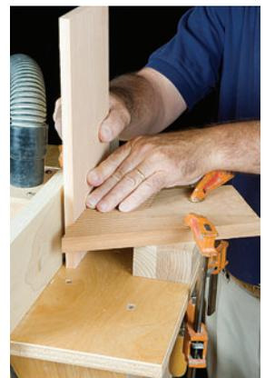
A router table will cut dadoes and grooves (left), shape edge profiles (center) and even raise panels for cabinet doors with a vertical panel-raising bit. All it takes is a little plywood, a couple of hours' time and Bill's "Po' Boy" plan.
