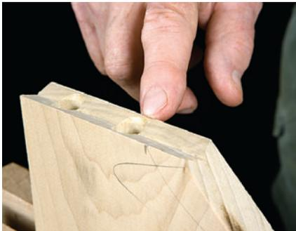
Leave the smallest of flats on the edges of the V-groove — say, 1/32". Refine the angle as shown in the photo at right.
