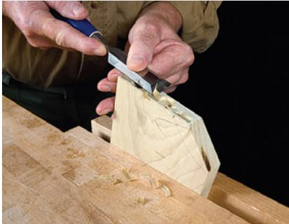
Using a wide chisel and horizontal paring, cut the V to within 1/16" of the edge of the wood. The poplar cuts easily.
