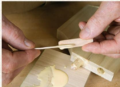
**Next, wet half the dowel before inserting it in the hole. But don't apply excessive amounts of glue. "Wet" does not mean "dripping."**
