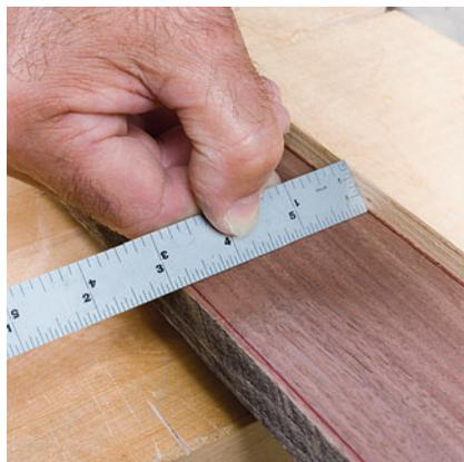
Determine where to clamp the straightedge by measuring from its edge to a reference line drawn on the workpiece.
