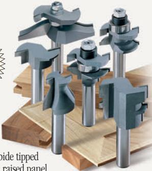
1/2" shank carbide tipped bits for making raised panel doors, table tops and drawer assembly. For stock up to 3/4". Includes Ogee Raised Panel with Undercutter, Matched Rail & Stile, Glue Joint, Drawer Lock, and Door Lip bits.
