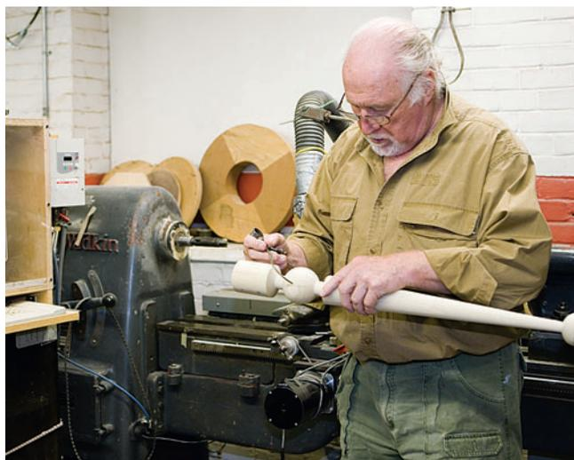
**Regardless whether you turn by hand and compare your leg's shape to a template or shadow drawing, or use a manual duplicator, you are making methodology and technology choices. Here, the author checks the tolerance of the leg blank as it comes off his CNC lathe.**
