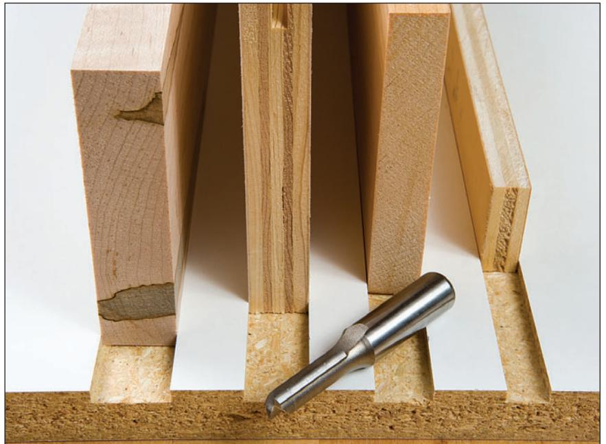
Regardless of stock thickness, you can produce perfectly fitted dados. Here are dados fitted to 7/8" solid wood, 3/4" plywood, 5/8" solid wood and 1/2" plywood, all cut with a 3/8" straight bit.
