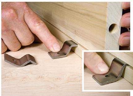
Because the kerf and screw arms of the clip are not parallel, the clip levers off the back of the screw plate. When the screw is driven home, it pulls the top and base together tightly.
