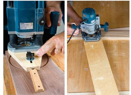
Power up, plunge the bit, and swing the router counterclockwise around the trammel’s pivot. (The shop-made trammel shown above left is adjustable.) Plunge a little deeper with the next and additional passes until the bit cuts all the way through. You can use a plywood scrap to make a trammel that pivots on a screw (right) to cut large arcs or circles.
