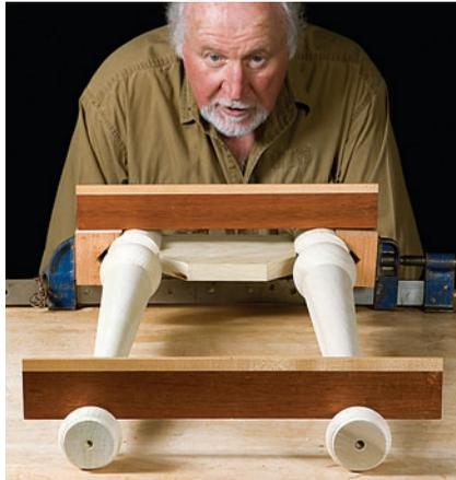
**Check for twist with winding strips, the same way as you would for a square stock assembly.**
