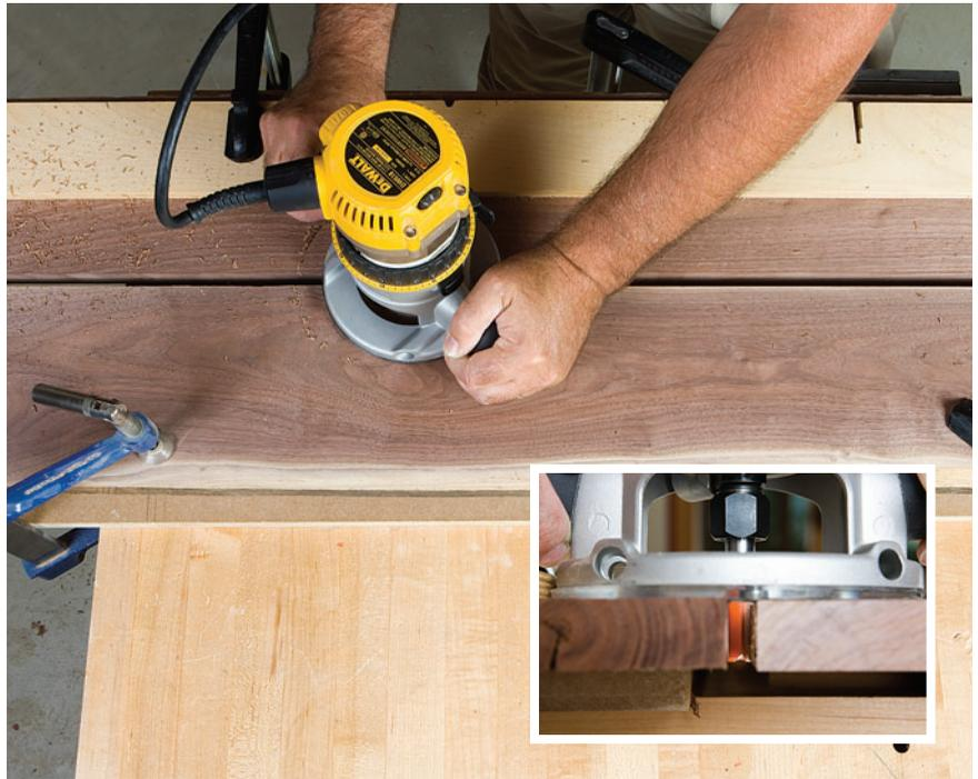
Here's a simple setup that converts your router and straight bit into a "jointer." With a couple pieces of plywood and two straightedges, you can create a tight glue joint in jiffy.
