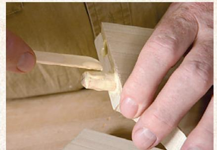
**Insert the dowel and then wet the other half of the dowel. The author uses a paddle as the applicator for the glue. A 1/4" dowel works as well.**
