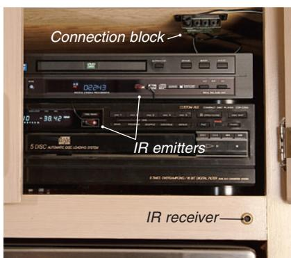
Mounting an IR receiver on the cabinet face allows infrared receivers to operate when the cabinet doors are closed.
