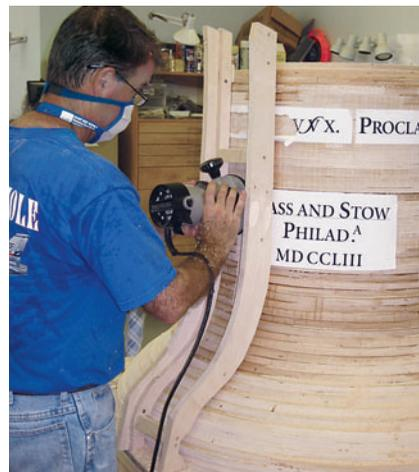
**The bell was so heavy that Carr used a router on a moveable jig to form the shape, keeping the bell stationary as he worked around it.**
