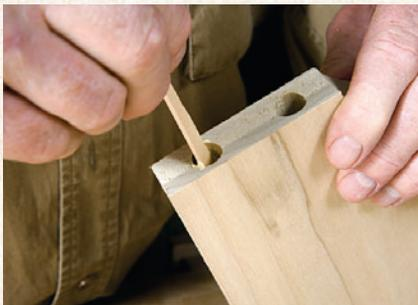
**Thoroughly wet the dowel hole. A splurt of glue randomly squirted into the dowel hole will result in dry areas, causing a weaker joint.**
