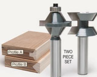
1/2" shank with carbide cutters. Locked in joint - easy alignment. Add an attractive edge to cabinet doors and shelves. Use with plywood MDF panels or shelves from 1/2" to 1" thick. Large glue surface.
