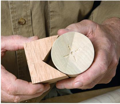
**A V-shaped clamping block prevents damage to the cylindrical leg and allows you to apply pressure where needed.**
