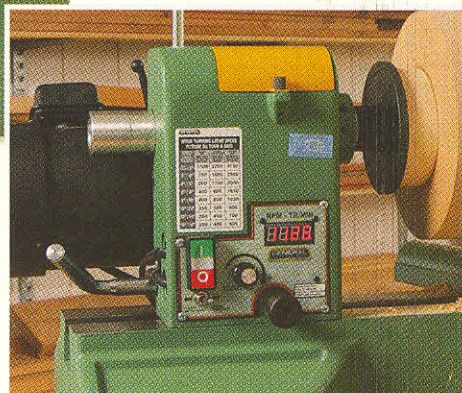
General provides digital readout and a helpful speed chart to dial in the variable speed (right). The 25-650 also comes with a magnetic "panic" button (above) that can mount anywhere you want it to be.
