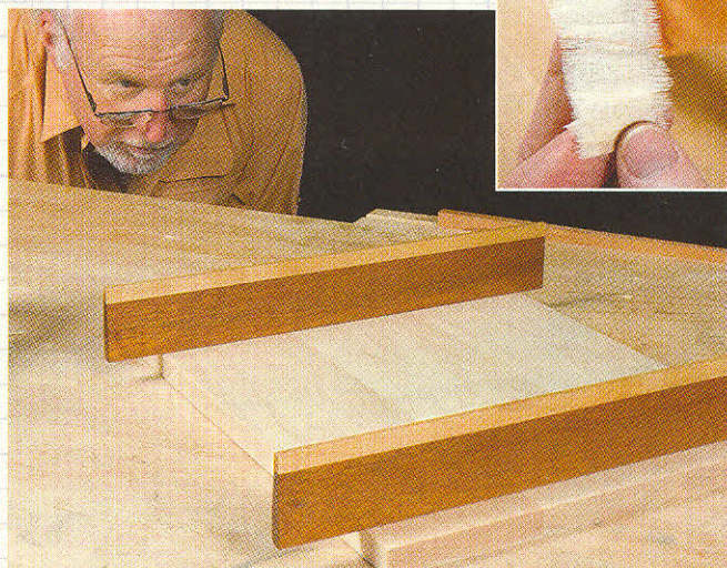
Periodically check for twist by sighting across the top of a pair of winding sticks.
