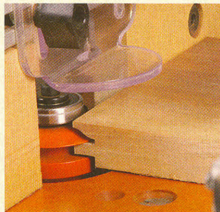
Mill the cope and stick joints for the door frame starting with the rails. First mill the cope profile across the ends of a 6"- to 8"-wide workpiece, using a guard to shroud the bit.
