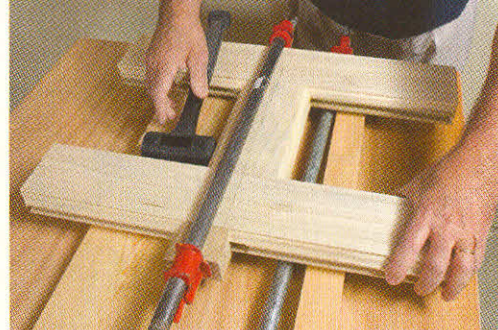
Start your dry or final assembly of the mullions and rails by working from the top of the door down or the bottom up. Insert the loose tenons and install clamps above and below the assembly to close the joints.
