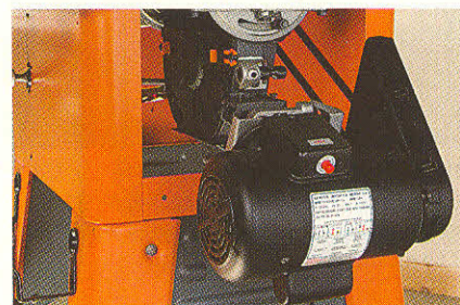
With the motor hanging off the back and even smaller trunnions and gearing, the end of the contractor's saw may be drawing near.
