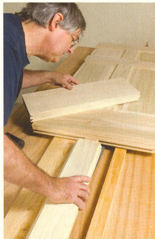
Continue the assembly process, slipping panels into their grooves to help hold the rails and mullions in position. Make sure the mortise layout marks are aligned. Then finish up by installing the stiles.
