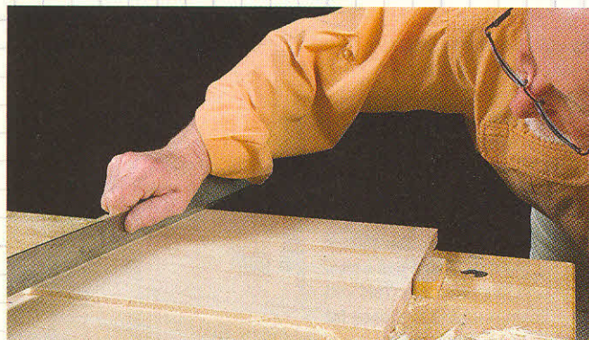
Check for flat in length and width as you proceed, using a straightedge. Continue planing until you see no light underneath.
