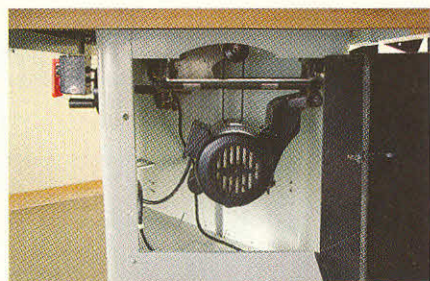
The hybrid cabinet is a great help in controlling sawdust. It also contains the motor, which makes it a bit quieter than a contractor's saw.
