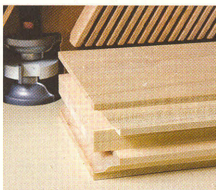
Minimize chipping by staging the sticking cuts. Follow a shallow first pass with a not-quite-full-depth cut. A final cleanup pass leaves you with a virtually chip-free finish.
