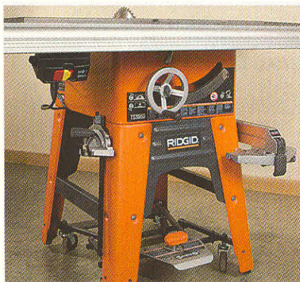
An open base is less expensive to manufacture but much messier in the shop. Many folks are concerned about dust collection these days.
