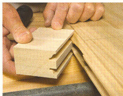
Seat the lock-rail to the middle mullion joint by applying a clamp momentarily. A coped scrap is valuable as a clamp block to protect the stuck edge of the lock rail.
