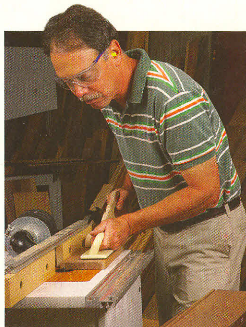
Route the back panel grooves along the four case parts at the router table with a 1/4" straight bit chucked in your router.
