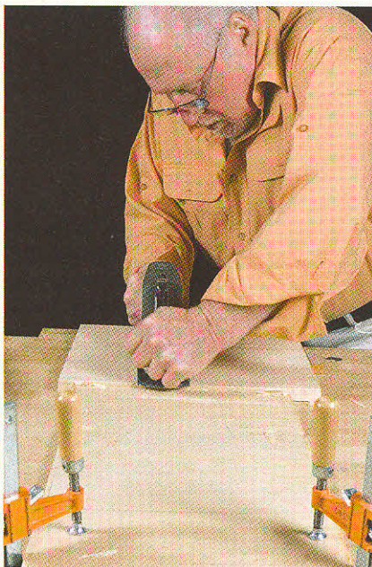
To facilitate cross-grain planing, trap the workpiece firmly on three sides: the bench stop, a board clamped in the vise and a board clamped to the bench.
