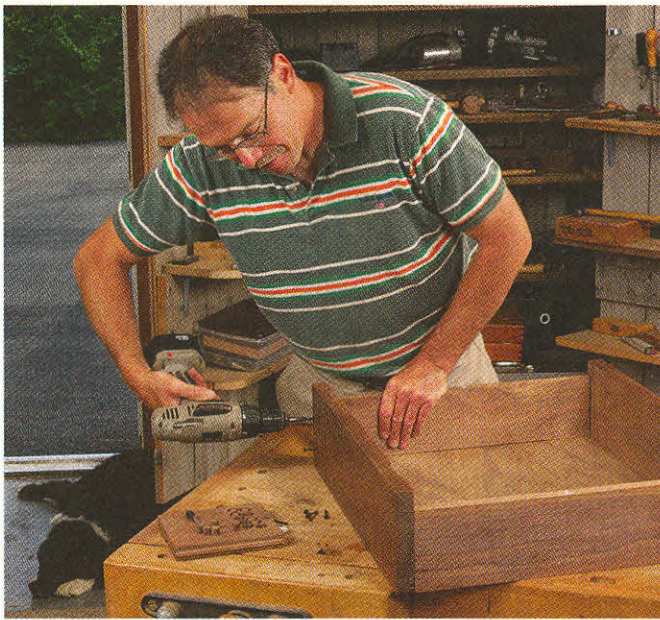
There's no fancy finery to the case's corner joints (left); they're just screwed and plugged butt joints at all four corners. The author even chose to use screws to secure the cope and stick joints on the door (right). The rails and stiles are machined and test-fitted prior to assembly.
