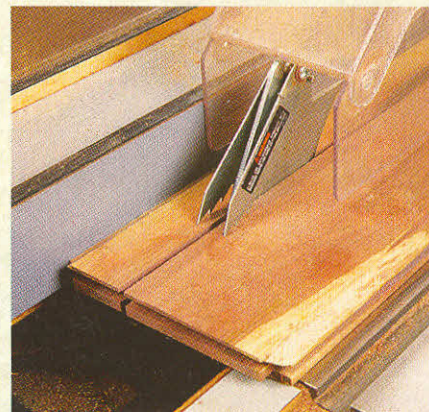
Once the cope and stick joints are routed, turn to your table saw to rip the rails and stiles free. The combined rail workpiece is shown here.
