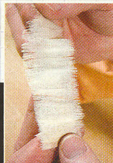
Here's a shaving from a slightly curved blade when planing across the grain: thick in the middle, thin on the outside edges.
