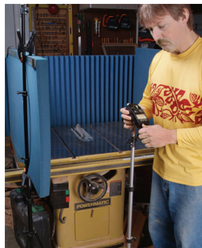
To explore advertisers' claims about noise reduction, the author used acoustic foam panels to set up a three-sided baffle and then used a sound level meter to compare the noise output of the various saw blades.
