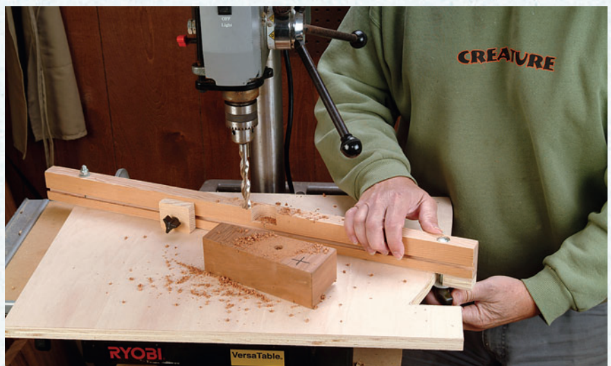
Figure 3: Add a small plywood lock block to the fence (see Drawings ), place a fender washer on the bolt, and follow with a threaded knob.
