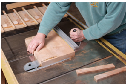
Cutting test: crosscutting red birch plank using Woodhaven's miter gauge, with the cut test strips in the foreground and background.
