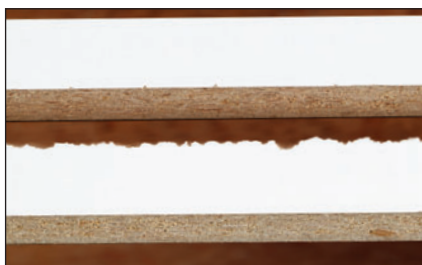
Two melamine test cut strips, with their bottom cut edges facing each other. The lower strip rated "Poor," the upper strip "Excellent."
