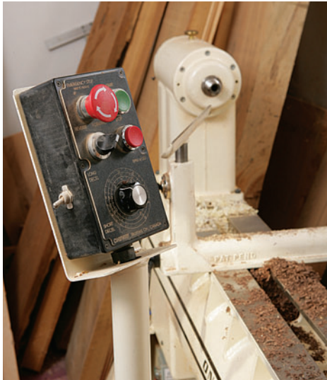
The location of the controls is one consideration to keep in mind. Some lathes, like the author's, have a moveable control panel.
