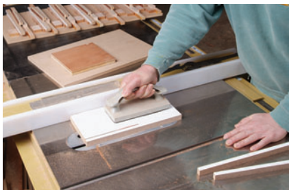
Cutting test: sawing test cut strips from melamine panels using table saw rip fence.
