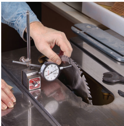
The author measured runout of the test saw blade plates with a dial indicator.
