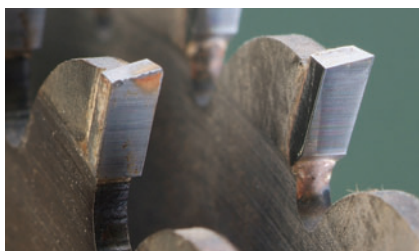
Closeup of saw blade teeth on two identical model (Forrest Woodworker II thin-kerf) blades: tooth on right is brand-new; tooth on left is chipped and dull.
