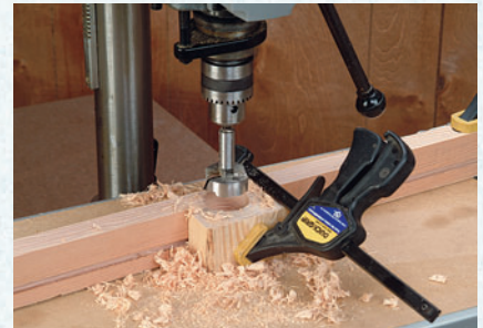
Figure 2: Form a “half hole” on the face of your fence in order to provide clearance for the chuck when drilling close to the jig surface.
