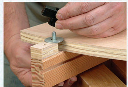
Figure 3: Add a small plywood lock block to the fence (see Drawings ), place a fender washer on the bolt, and follow with a threaded knob.
