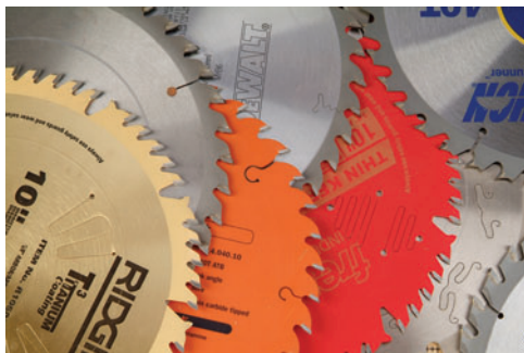
A montage of the different styles of expansion slots and anti-vibration cutouts in plates.
