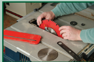
Fitting stabilizing washers on either side of a thin-kerf blade can help reduce deflection during heavier cutting.
