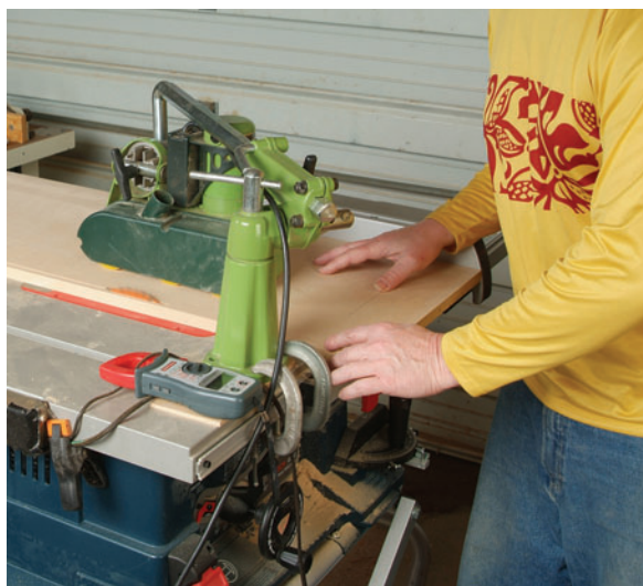
The author compared feed pressures of various blades by cutting 3/4" MDF panel, using a power-feed set up on a Bosch portable table saw and an ammeter to measure the amperage draw from the saw.
