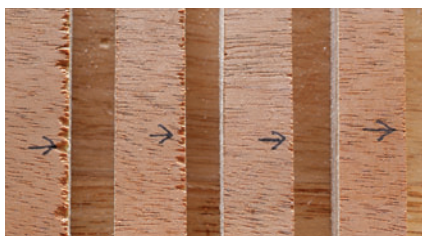
Four mahogany plywood test cut strips, showing the lower edge of cut (arrows indicate test edges). They are rated, left to right: "Poor," "Fair," "Good" and "Excellent."
