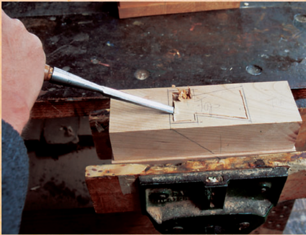
Figure 4: After laying out the plane's mortise, secure the blank in your vise. Carefully begin chopping out the waste, cutting only the portion of the bedding slope between the abutment cheeks.
