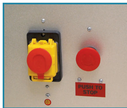
Craftsman switch setup is excellent. The author likes the easily accessible stop switch.
