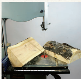
Heavy-duty jobs: The 1/2" blade has roughly four times as much beam strength as a 1/4" blade. In this sequence, the author uses a 1/2" bi-blade with three teeth per inch (TPI) to first cut a cherry log in half, then in half again, and then (using a high fence) to form small boards.
