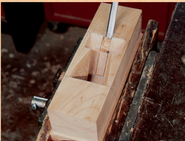
Figure 9: After getting the bedding slope as flat as you can with a wide paring chisel or a float, mark and cut the groove for the head of the machine screw which attaches the cap iron to the iron.
