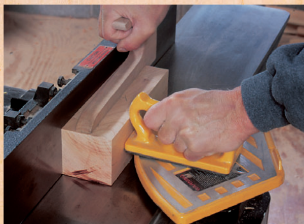
Figure 1: Prepare the plane blank by first cutting it to length. Use your jointer to mill the blank so that all six of its faces are 90^\circ to their adjacent faces. A precision tool must be precisely made.
