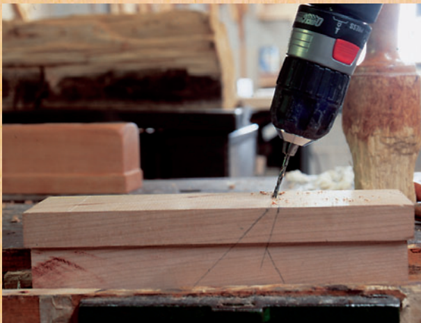
Figure 5: To begin the mouth, the author drills two holes in the center of its width with a 3/16" bit. These act as references as he chops a hole on top of the blank which will become the mouth on the bottom of the plane.
