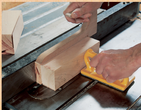
Figure 3: Complete the stylish and practical step-out with a 1/8 " deep cut that is 3/4 " from the table saw’s fence. In every step shown above, take note of the prudent use of push sticks and pads.
