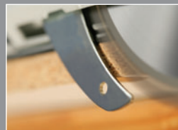
Spring-loaded riving knife
