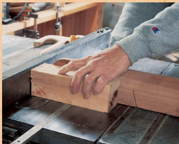
Figure 2: Use a smooth-cutting table saw blade, such as the author’s planer blade, to begin forming the plane’s distinctive step-out shoulder. A carbide-tipped 60- or 80-toothed blade is an acceptable alternative.
