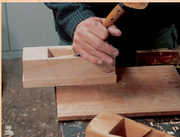
Figure 7: Position the mouth just over the edge of the benchtop to support the sole behind it when you're chopping the bottom section of the throat. Otherwise, you risk chopping out sections of the sole.
