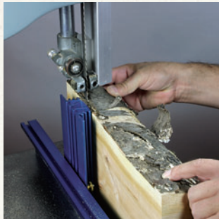
Heavy-duty jobs: The 1/2" blade has roughly four times as much beam strength as a 1/4" blade. In this sequence, the author uses a 1/2" bi-blade with three teeth per inch (TPI) to first cut a cherry log in half, then in half again, and then (using a high fence) to form small boards.
