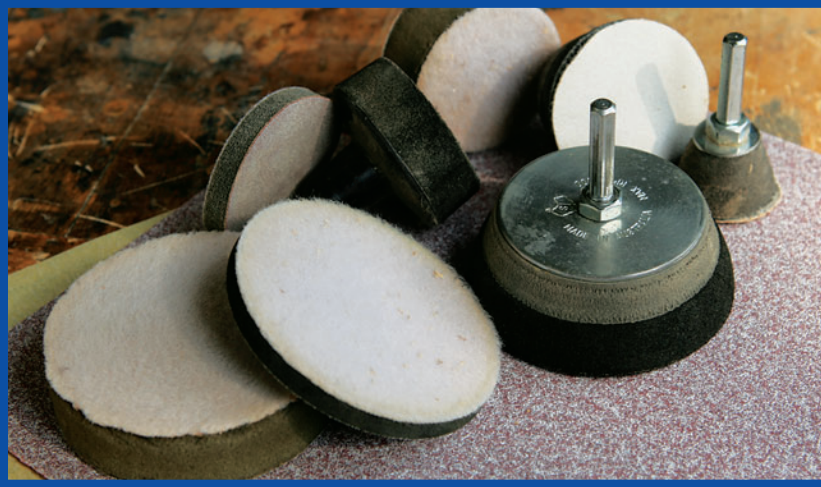
Sanding discs and interface pads come in a wide variety of sizes and types, including foam-backed and wave-type. Interface backing pads are inexpensive and help to extend the life of the more expensive sanding disc holders.
