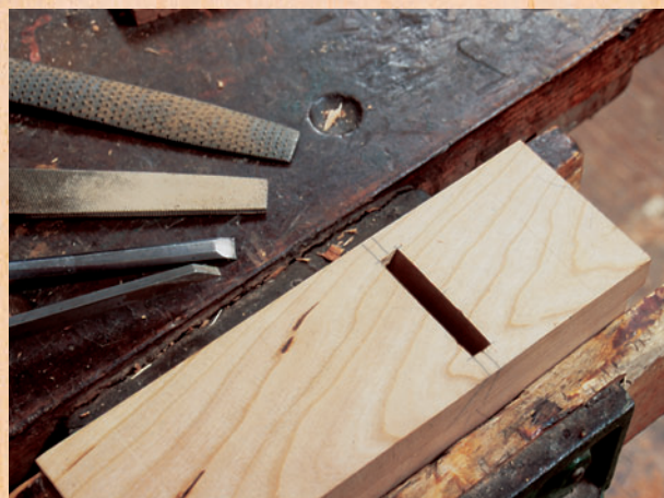
Figure 10: The scorings that can be seen in this photo mark possible locations of the mouth's front edge. The author adjusts the location after loading the iron, moving the front edge of the mouth forward a bit at a time until it's correctly placed.
