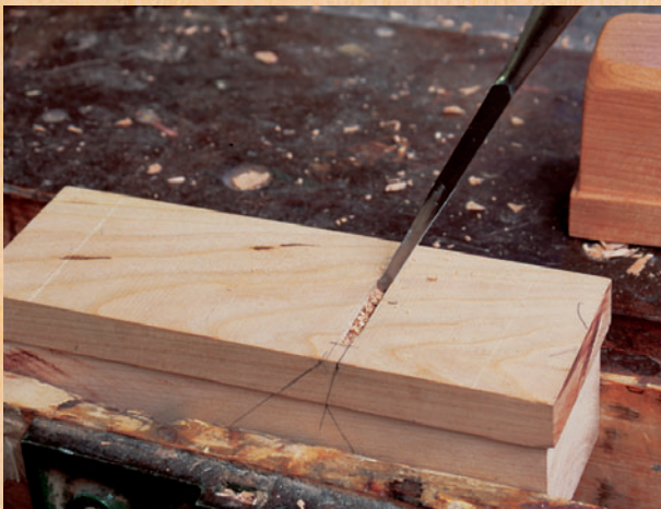
Figure 6: Use a 3/16" chisel to form the mouth of the plane. The holes you drilled in the previous step serve as guides for this process.
