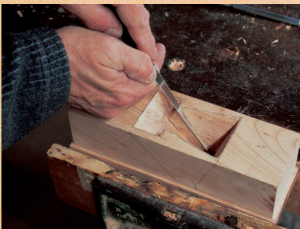
Figure 8: The detail saw used here to cut the top of a wedge slot can also be used to cut the floor of each wedge. Be careful not to cut too deep and go through the 1/4" sidewall of the wedge: it's the only thing holding the plane body together at this point.
