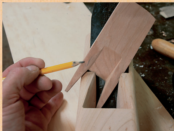
Figure 11: The author cuts a 5/8", two-pronged wedge, creating its slope on the band saw. He rubs pencil lead on top of the wedge slots, taps the two-pronged wedge into place on the assembly, then removes it.
