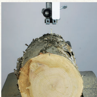
Heavy-duty jobs: The 1/2" blade has roughly four times as much beam strength as a 1/4" blade. In this sequence, the author uses a 1/2" bi-blade with three teeth per inch (TPI) to first cut a cherry log in half, then in half again, and then (using a high fence) to form small boards.
