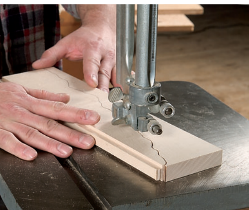
On the band saw, the author scrolls the edge of the brace. After he is done, he will scrape the edge until it's pleasing to the eye and "uniformly textured."
