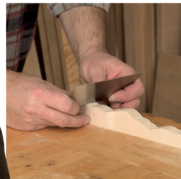
One of the distinct textures on the podium is the scraped edges of the organically shaped supports.
