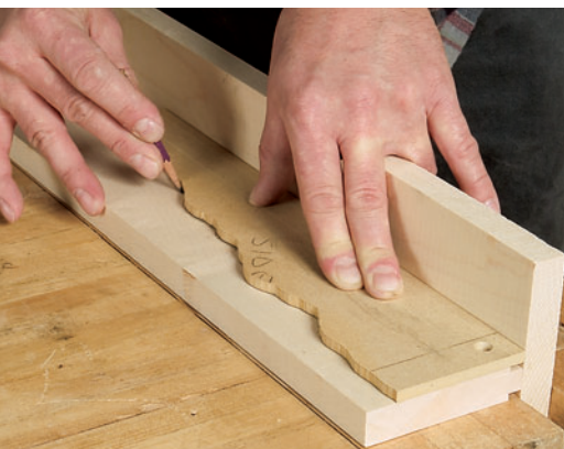
With a straight edge clamped into his tail vise, the author uses a template to trace the organic shape of the brace. This creates uniformity even with the free-formed edge.
