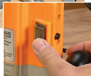
One of the “cons” of this router: an awkward on/off switch that was more difficult to lock on than to turn off.
