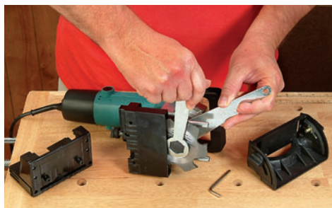
You take the good with the bad: the biscuit joiner's blade was loose on its arbor during a (powerless) dry run, but the kit had wrenches to fix the problem.
