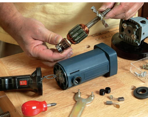
Rows of shallow holes drilled by an automated balancing machine indicate a dynamically balanced motor fan and armature on the right-angle grinder: a surprise on a "cheap" tool.
