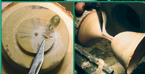
Mount a 10" segment of tree limb or trunk between centers. Mount it off-center to avoid making the weaker pith part of your stem. Remember to raise a round nub to grab later in a chuck. Hidden knots or defects can create a problem as you turn.
