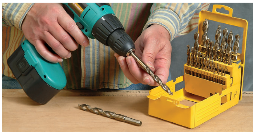
The Feida — and the other two drills in this article — required the author to switch to drill bits with flattened shanks (three flat areas on the shank, to provide a better grip for the chuck). The keyless chucks kept slipping on smooth-shanked bits.
