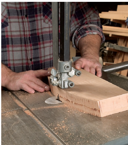
With the saw's table angle to 10°, the author begins to create the chamfer on the podium foot.
