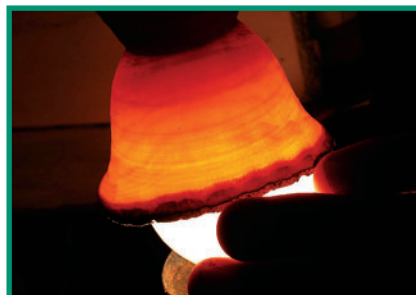
The water-saturated wood transmits light quite well. You can use this fact to help judge the thickness of your goblet walls.
