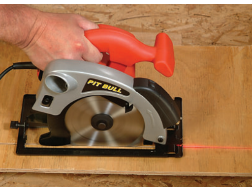
The Pit Bull circular saw sported a battery-powered laser that projected a red stripe to show the blade's line of cut — a very useful feature.
