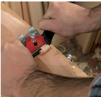
Finally, the author cleans up edges of the chamfer with a spokeshave. The large feet provide a solid base and the chamfer helps to minimize the visual impact of the feet.
