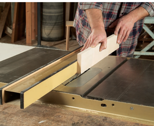
When machining the decorative maple braces, the author begins the process while they are still stuck up. He forms the tongues on the back edge of the braces first.
