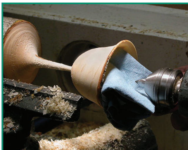
With the stem and the bowl of the goblet shaped, you can remove the live center (and its padding that prevented scratches). This goblet is almost ready to be parted from the remaining piece of limb.
