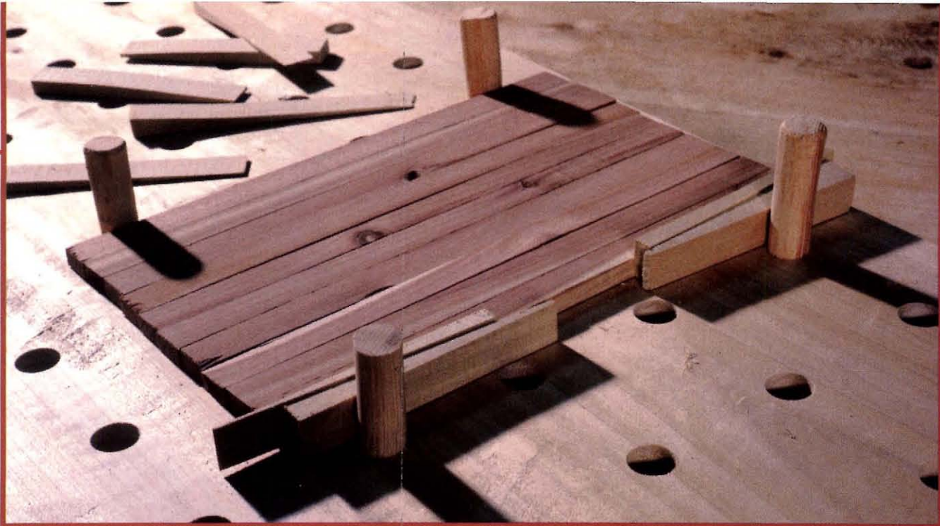
When used in pairs, wedges provide an elegant way to apply direct, parallel clamping pressure without clamps.
