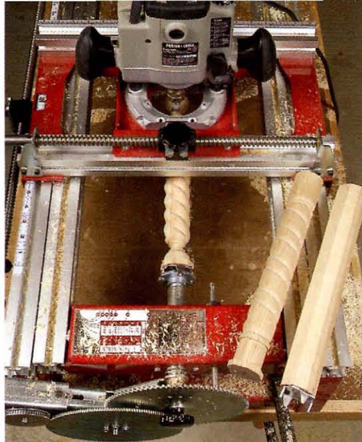
A large router isn't really required for milling stock, routing turnings and spirals, cutting flutes and beads. The 2HP model 1 used worked fine.
