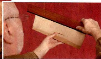
Checking straightness on the face edge of a board with a wooden straightedge.
