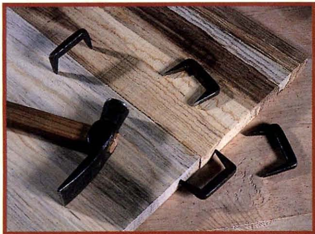
These iron joiner's dogs (pinch dogs) have tapered legs that pull boards together when driven into end grain.
