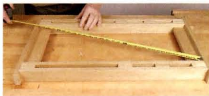
Checking squareness of an assembly with a tape measure.
