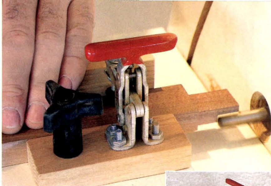
Figure 6: A hold-down clamp, secured by a T-bolt and star knob, keeps the workpiece tight against the fence of the Y-table, while a straight bit mills a tenon on the end of a cabinet rail.
