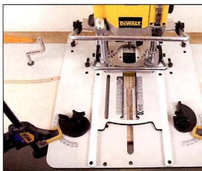
To dado with the 'Rat, you tuck the workpiece up under the mounting plate and use "the brush" to hold it. Once the piece is aligned for the cut, apply a clamp to secure it to the plate.
