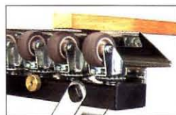
Ramp raised to support narrow workpieces.
