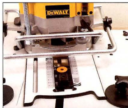
The spirals flanking the router plate control the angle. Twist the router against the spiral and slide it forward, then back to make a cut.
