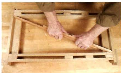
Pinch rods are sharpened so they will fit into the corners. Sight and touch make the measurement.
