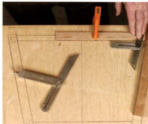
An angled shoulder line on a tenon is made by first setting the bevel to pieces of wood clamped in place on the drawing.
