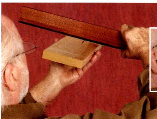
Checking straightness of the face side of a board with a wooden straightedge.
