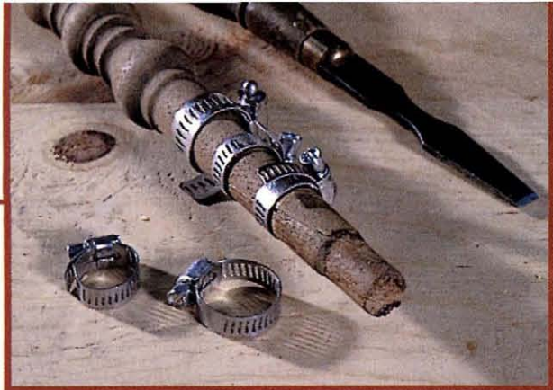
Hose clamps of various sizes are indispensable for repairing small round parts such as chair tenons.
