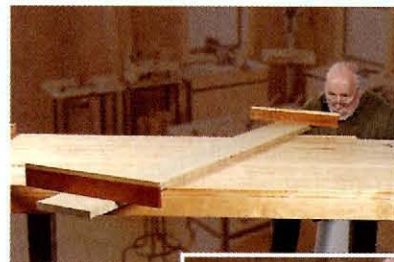
Check for twist by putting winding strips at each end (at right angles to the board) and align your eyes with the center marks. Half the board may be flat, the other half in twist. Complete the survey by moving the winding strips.
