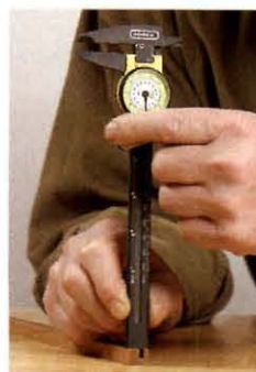
The author gauging depth with a dial caliper. Linear dimension requires measuring tools with graduated scales.
