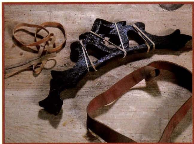
Rubber bands are particularly useful where band clamps are too big or bulky to do the job.
