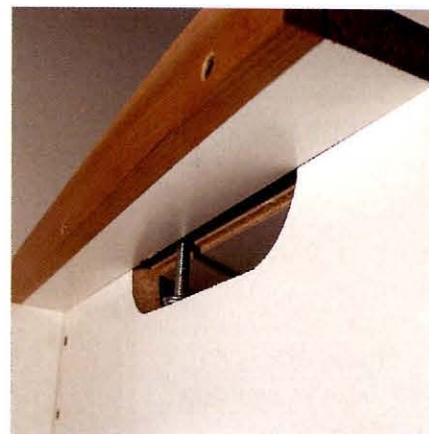
Figure 4: A pair of 3/4" grooves in the bottom of the runway accommodate both the heads of the T-bolts and the tops of the runway sides.
