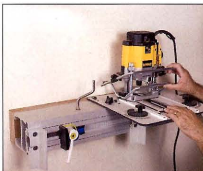
The plunge router, mounted on the router plate and equipped with the PlungeBar accessory, sits on the base plate. It can slide fore and aft, pivot or be locked down.
