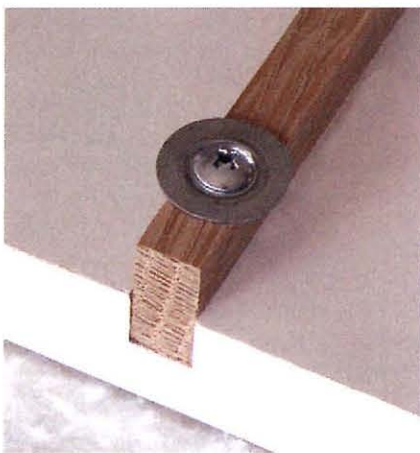
Figure 5: In the underside of the Y-table, a screw and washer in the hardwood guide run in the T-slot of the X-table to control lifting.
