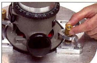
Quick-release clamps hold router in place.
