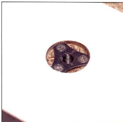
Figure 2: Three T-nuts embedded in the tabletop add versatility to the machine by allowing for the easy addition of jigs and hold-downs.
