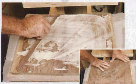
The author attached highly figured, shop-made, veneer to plain sawn walnut panels. Apply glue to the panel only. Note that the panel is sitting on a plywood caul protected by wax paper.
