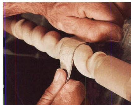
As with most woodworking endeavors, sanding is one of the final steps before finishing. Strips of sanding belts can be folded and used for this purpose.
