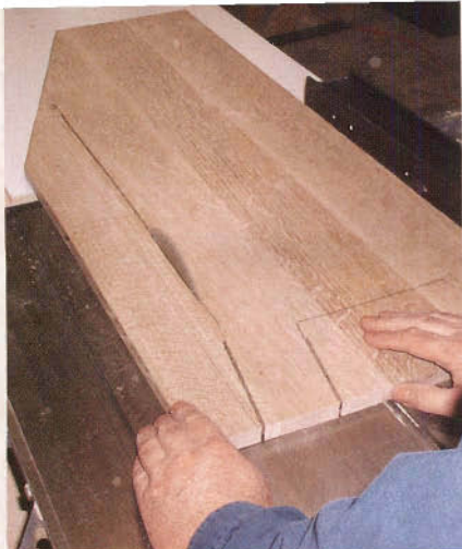
Figure 1: The cuts which reveal the desk sides are made on the table saw to keep them straight, and then finished with a saber saw.
