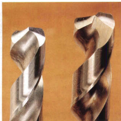
Standard pointed bits (left) are ground at 118°, while split-point (right) have faces ground at 135°. The author considers the split-point bits a better all-around choice.
