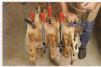
Use plenty of clamps to ensure that sufficient pressure is applied across the clamping cauls. Allow plenty of time for the glue to cure: at a minimum, overnight.
