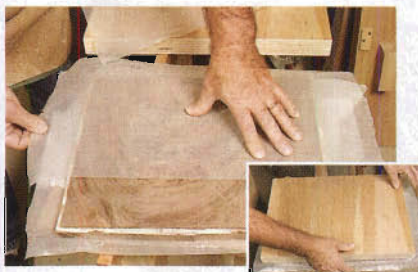
Put the veneer onto the glued panel and prepare to clamp it up between a sandwich of plywood cauls protected from the excess glue by layers of wax paper.
