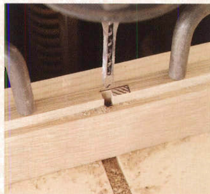
Figure 15: The small mortises for the muntins in the bookcase doors are chopped with a 1/4" chisel chucked in the mortising machine.
