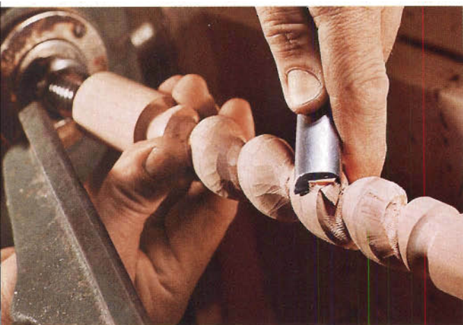
After a sufficient quantity of stock has been pared away, switch to a sweep or concave chisel. Invert it and continue to remove wood. It begins to shape the rounded upper edge of the spiral.
