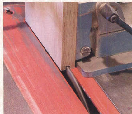
Figure 4: The vertical grain on the ends of the drawer supports is a T-molding ripped from the edge of a board and glued into a dado.
