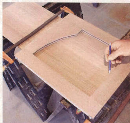
Figure 11: Dry clamp the doors together and use them as templates to mark the shape of the panel. Add 5/16" all round for the groove.
