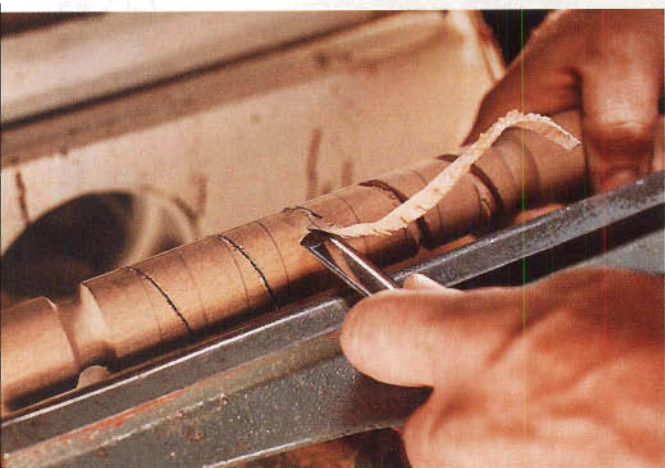
Once the spiral or twist has been incised with the dovetail saw, break the cut open with a flat chisel. The author uses a variety of carving chisels and gouges to pare the waste from the twist.
