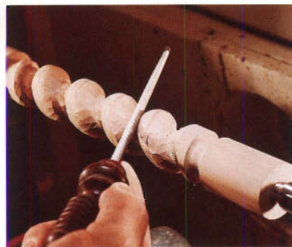
For fluted spirals, you can also use a rasp to remove wood and shape the bottom of the cut.
