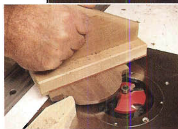
The tombstone panels (and the rail that receives them) require some template routing. When raising the curved ends of the panel, use a safety block to apply downward pressure.
