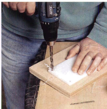
To get a nice, clean, large hole, use a two-step process. First, drill a small pilot hole. Next, use a stepped-point bit to bore the desired hole diameter, using the pilot hole to keep the bit centered as you drill.
