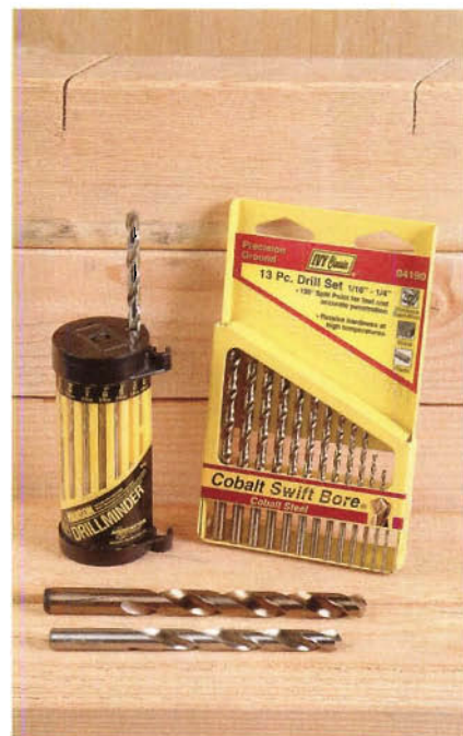
Cobalt drill bits (the dull gold bit above) are heat-treated and generally last longer than regular HSS bits (shown below the cobalt bit).
