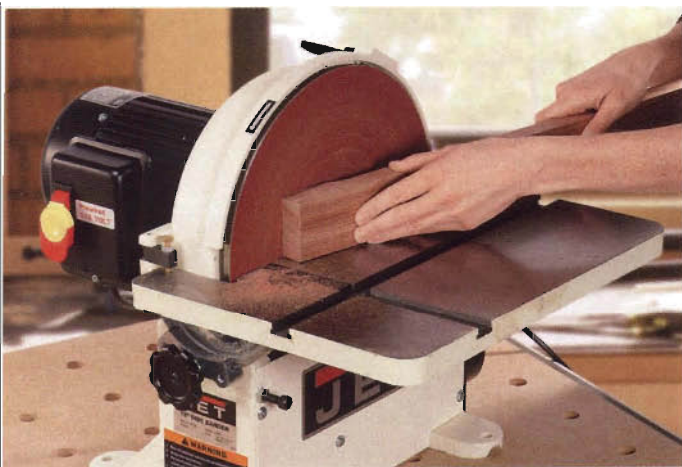
First, the author uses a one-cut jointer trick to do the majority of the machining on the legs (below). It's a simple but sophisticated technique. Next, shape the feet by sanding an angle on the remaining lower leg stock (above).
