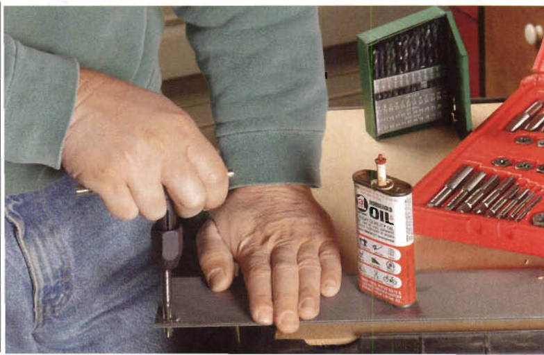
To make easy work of tapping holes (1/4" or smaller) in either metal or plastic, a set of large-numbered wire gauge bits is just the ticket.
