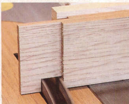
Figure 14: Trim the shoulders on the bookcase door rail mortises to size using a dado head in the table saw.
