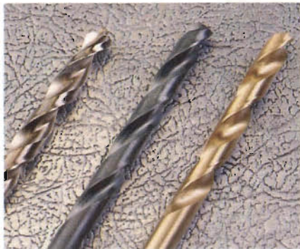
Ferrous oxide (left), black oxide (center) and titanium nitride (right) are all coatings for HSS steel bits. The coatings reduce heat buildup and help resist rust.
