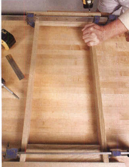
Figure 3. Clamp the shoulders tight to the cap and shoulder rail assembly with the inside legs in place.
