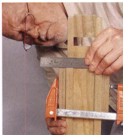
Figure 15. Glue and clamp the short shoulder rail flush to the shoulder rail.
