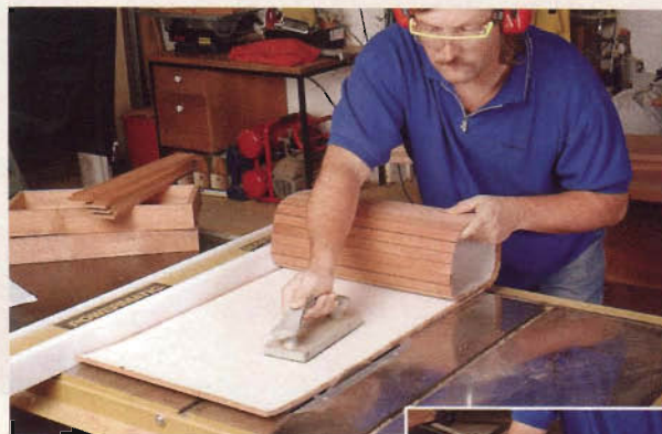
Roll out the tambour as you trim it on the table saw. Then create "tongues" on the ends of the slat by forming a rabbet with a dado blade (inset).
