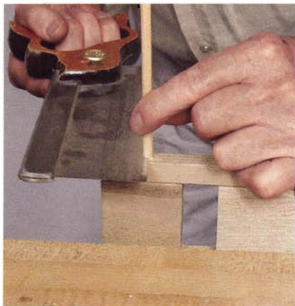
Figure 13. Saw off the excess length of dowel before cleaning flush with a chisel.
