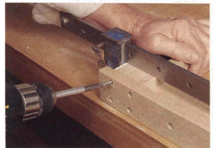
Figure 7. Glue and clamp outer legs to the leg blocks, then screw them through the cap rail.
