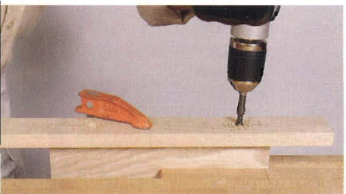
Figure 2. Clamp, drill, and screw the parts together dry to assist with positioning them once the glue is applied.
