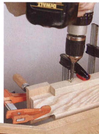
Figure 12 (right). Position the second shoulder rail with the aid of a block clamped tight and square to the first shoulder rail.
