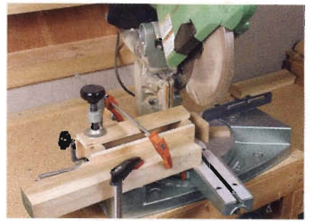
Figure 19. Clamp the jig tight to the bed and fence of the chop saw. To hold by hand is neither safe nor accurate.
