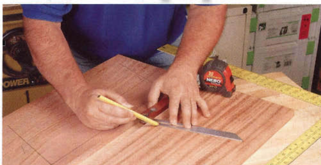
Use a sharp carpenter's pencil and an angle gauge set to 70° to mark out where the tray bottoms meet the cabinet sides.
