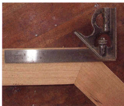
Two 22½° miters will add up to 45°. The author used his try square to check the accuracy of the frame's miters.
