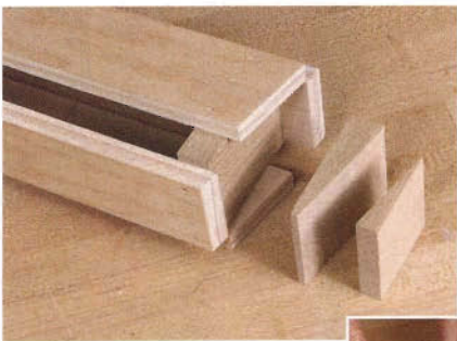
Figure 17. Make the wedge jig using two wedge blanks and strips of 1/2" plywood.
