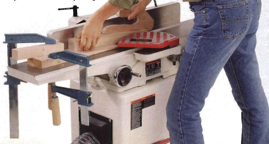
Step 2: Using your push stick, first lower your stock down to the level of the infeed table and then push it up the ramp. You can clamp a stop block to the back of your ramp to create a foot on your leg.
