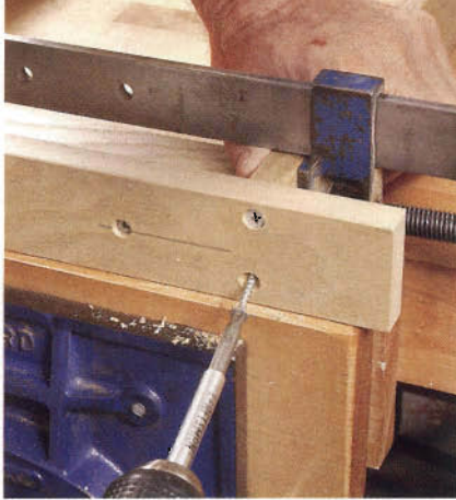
Figure 4. Screw through the cap rail into the end grain of the inside leg. Screws are angled towards one another for extra strength.
