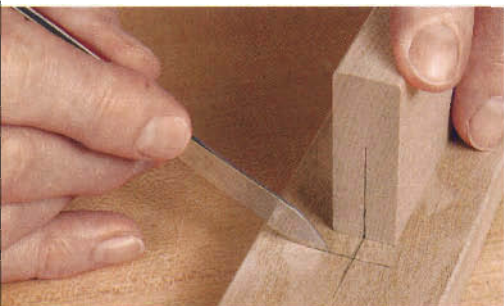
Figure 1. To accurately position the shoulder rails on the cap rails, mark their centers with a marking gauge.
