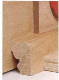
Running molding strips. To get consistent results, it's essential to run the molding through a "tunnel" of hold-downs to keep the workpiece tight to the table and the fence. Use a push stick to complete the cut.
