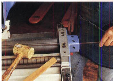
The Torsa system makes removing and installing planer/jointer knives a breeze.
