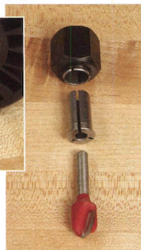
The lack of a 1/4" collet for some models requires you to use a sleeve on 1/4" shank bits.
