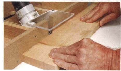
Straightening an edge. The photo clearly shows the correct way to joint an edge by pressing the workpiece against the outfeed table after two or three inches of the cut have been completed.
