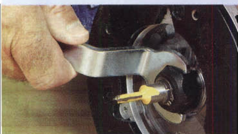
The bent wrench supplied with the Porter-Cable 8529 allows you to change bits through the base, ideal when the router is mounted in a router table.
