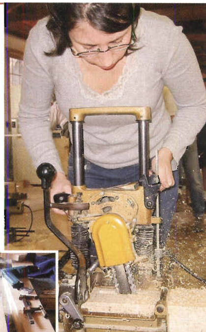
LiLi Jackson put a chain mortiser to use in making her workbench — pieces of which are shown at left.
