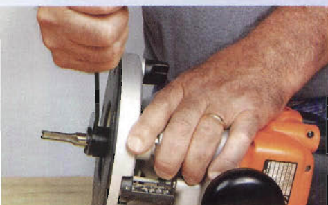
To change bits in the Triton, you wind the motor all the way to the base. The collet extends through it, and the spindle and the switch are automatically locked. Hold the router with one hand and work the wrench with the other.
