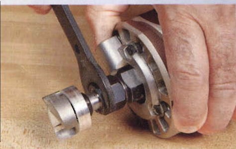
Changing a bit in a fixed-base router (DeWalt's DW618) that has a spindle lock requires only one wrench.
