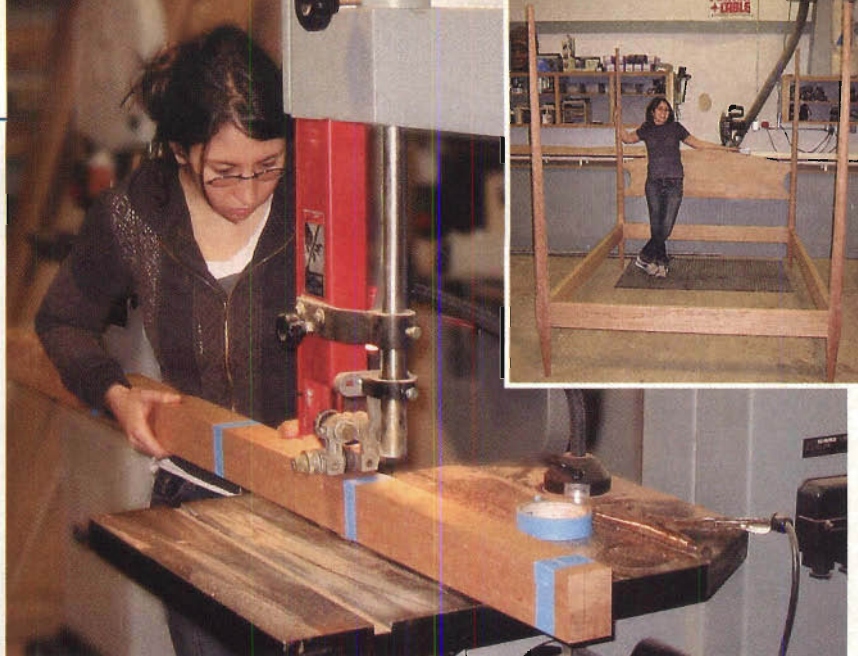
LiLi Jackson used the band saw in her pencil post bed class. After rough shaping, she used a hand plane to do most of the shaping on the pencil posts.
