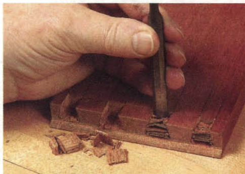
Return the work to the bench and chop carefully into the corner of the socket to clean out the bulk waste.
