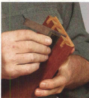
Check the back wall cut for parallel: press a chisel against the wall and check against a straightedge.
