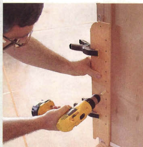
A shop-built jig and a stop on the drill bit control the location, frequency and depth of the shelf support holes.
