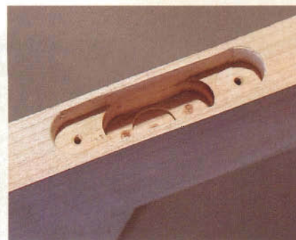
The Soss brand hinges, which attach the doors to the operable stiles, come complete with templates (above). After marking several hole locations, drill out most of the two-step mortises with a 1/2" Forstner bit (inset). Then clean up the mortises with a chisel, or use a rotary tool equipped with a 1/2" coarse grit drum sander to get the final mortise (right).
