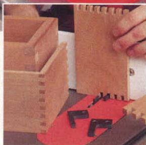
Eagle America's Mitey-Sled™ (above) and Mitey-Jig™ (left) let you make 1/4", 3/8" or 1/2" box joints on your table saw. Simply select the proper size of joint index template, fasten it to the jig, set the spacing for the first cut, and you're ready to go.
