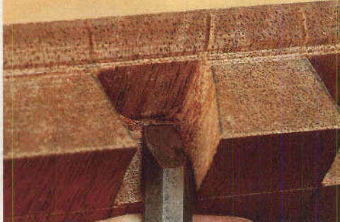
Clamp the pin piece in the vise and sever the corner end grain fibers with a skew chisel.
