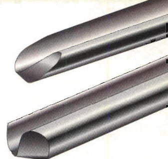
The two illustrations above represent the difference between an Irish, or Celtic, grind (top) and a conventional bowl gouge grind (bottom).
