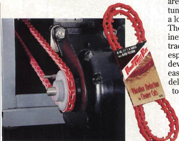
Cut blade vibration down to size while improving power transfer on your contractor's saw by slipping on a link belt. Buy these belts by the foot or in a 4' loop. You'll get positive results right off the bat.
