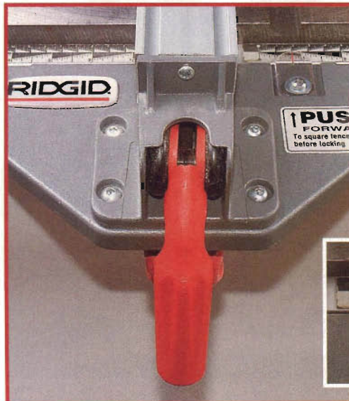
The TS2424 rear trunnion assembly offers easy access for quicker adjustments.
