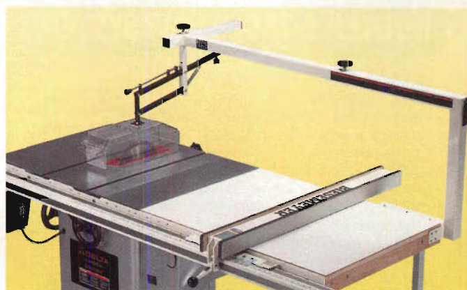
Biesemeyer Blade Guards mount to any 10" table saw with a 30" or 50" side extension table and T-square style rip fence. The blade shroud raises and lowers by way of a pair of counterbalanced springs.
