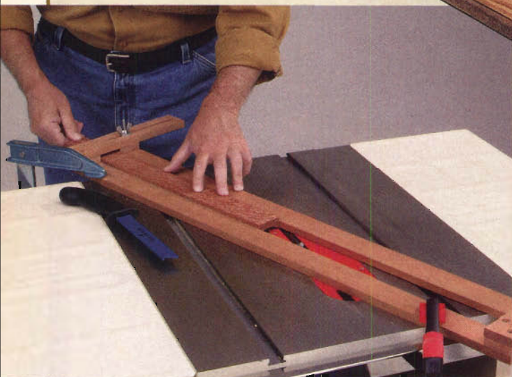
After many test cuts on pine, the author used his shop-made jig to form the coves in the lacewood staves. The adjustable jig accommodated both widths of door staves.
