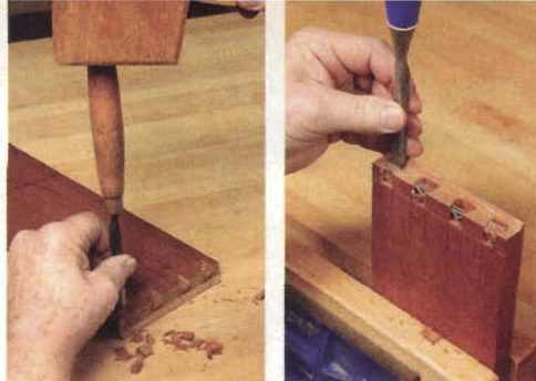
Left, chop across the grain up to 1/16 " of shoulder line to remove what comes easily. Then (right), chop slivers down the grain to 1/16 " of the rabbet line — no fallout.
