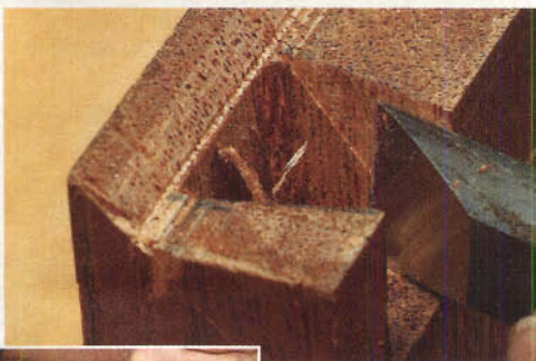
Continue the socket cleanup with a chisel narrower than the height of the pin so you can see the sawn pin face that guides your cut. Clean up the end wall by vertical paring, using the rabbet as a guide.
