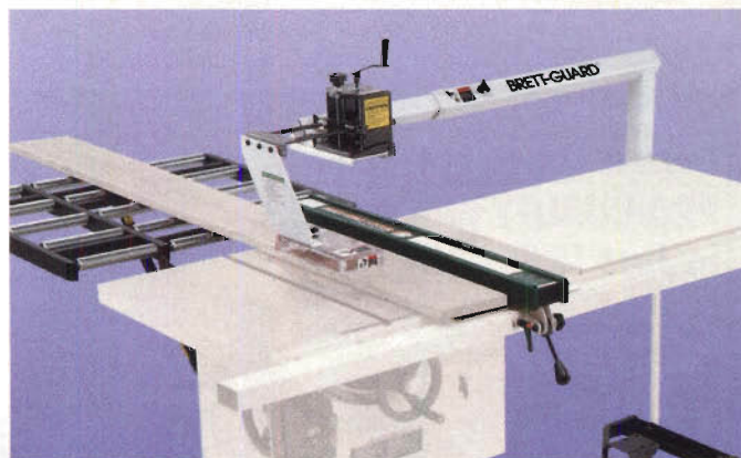
HTC's Brett-Guard Sawguard has a thick box-style blade shield that cranks up and down to adjust for different stock thicknesses. It doesn't ride up and over workpieces like other guard styles that act on gravity, so it provides "fixed" protection from the blade.
