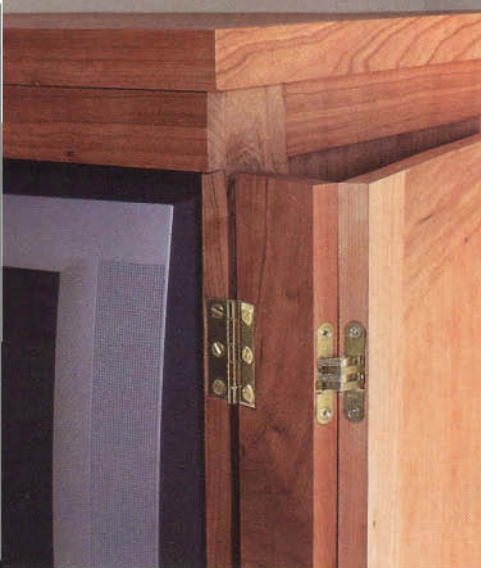
The Soss brand hinges, which attach the doors to the operable stiles, come complete with templates (above). After marking several hole locations, drill out most of the two-step mortises with a 1/2" Forstner bit (inset). Then clean up the mortises with a chisel, or use a rotary tool equipped with a 1/2" coarse grit drum sander to get the final mortise (right).
