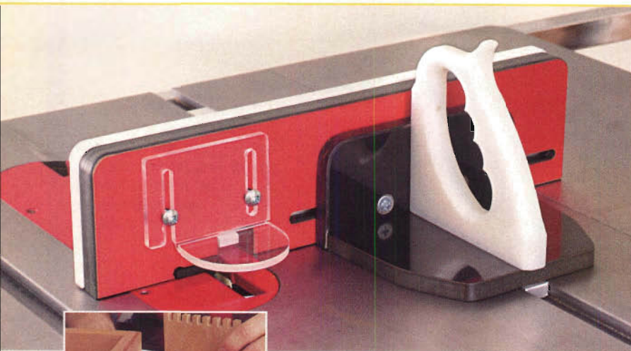
Eagle America's Mitey-Sled™ (above) and Mitey-Jig™ (left) let you make 1/4", 3/8" or 1/2" box joints on your table saw. Simply select the proper size of joint index template, fasten it to the jig, set the spacing for the first cut, and you're ready to go.
