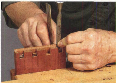
Check the back wall cut for parallel: press a chisel against the wall and check against a straightedge.
