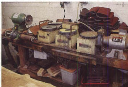
Steve's four sharpening wheels are the most specialized equipment his shop holds for his plane making pursuit.
