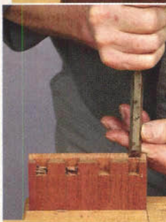
Continue the socket cleanup with a chisel narrower than the height of the pin so you can see the sawn pin face that guides your cut. Clean up the end wall by vertical paring, using the rabbet as a guide.
