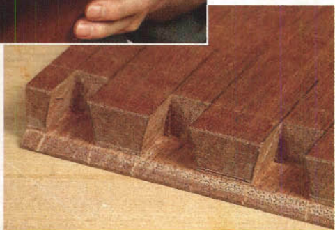
Check bottom of socket (left) for square. Tail sockets (below), cleaned out by careful chisel work, are ready to mark out the tails.
