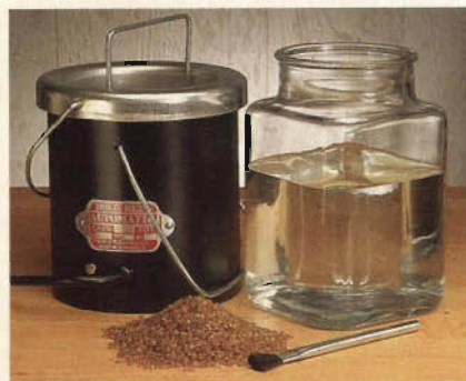
An electric glue pot can be used to heat hot hide glue, and a bristle brush to apply it. Granules and water are mixed to create a gel.
