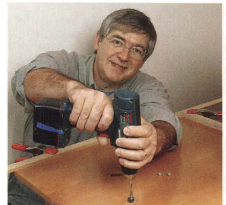
One of the last tasks is to drill for the dowels that secure the gallery to the desktop. It must be done with considerable care.
