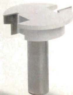
A drawer lock bit (below) and compression bit are two of the three special cutters the author used for this project.
