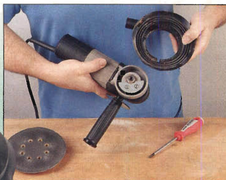
A dust collection kit with an easy mounting shroud and eight-hole backing pad is an added option for the Porter-Cable 7336.
