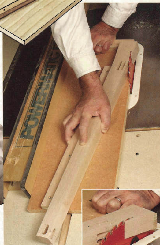
Saw the inside foot taper to avoid major tearout problems. Attach a couple of fences to a scrap panel to make the jig quickly. Recycle the screws and panel after the legs are cut.
