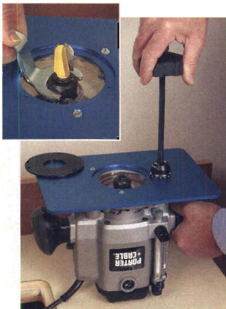
Porter-Cable's 8529 plunge router is designed to be adjusted in or out of the table. The optional adjuster drops through a hole you drill in the mounting plate and mates with the router's height adjustment screw. The bent wrench Porter-Cable supplies (see inset) easily changes bits from above the table. It can access the collet, even when it's slightly below the table surface.
