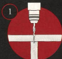
(1) Drill stepped pilot hole
