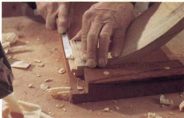
The author used a backsaw to cut the tenons for this table. Then he turned to his chisels to pare the tenons, creating a slight angle to accommodate the curved aprons.
