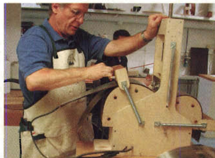
Charles Fox, above, is the inventor of the sidebender machine, now used to form the bouts of nearly every guitar manufactured.
