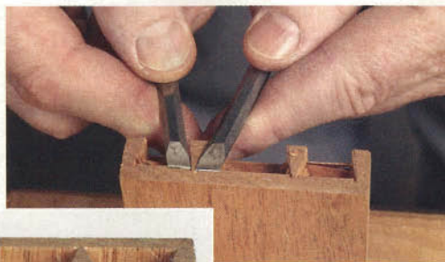
The corner waste is removed by first severing the end grain with a pair of purpose-made 1/4" skew chisels. The goal is pins and sockets that are clean as a whistle.
