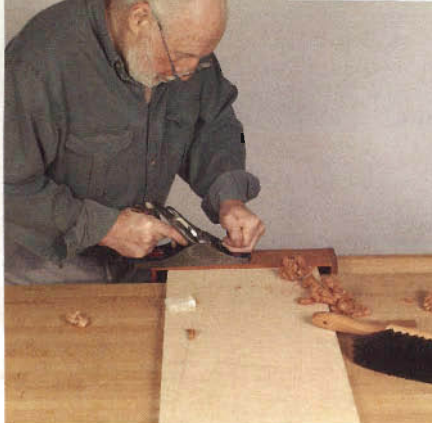
Plane both drawer sides down to match the end grain of the dovetail pins.
