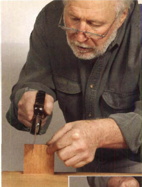
Cutting the tails for a single-lap dovetail is the same as cutting the tails for a through dovetail. After cutting the tail slopes with a dovetail saw, remove the bulk of the waste with a coping saw. Your next step is to clean up to the lines by vertical and horizontal paring.
