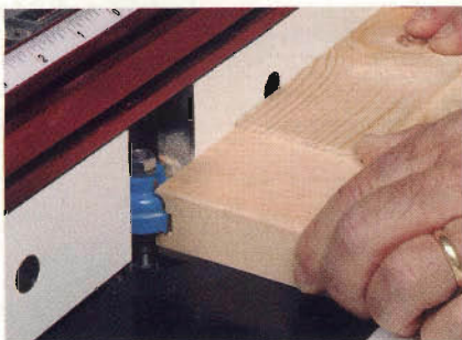
Cope the rail ends first. A push block helps keep the rail square to the fence and backs up the cut to prevent tearout.
