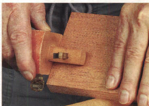
Knife a line around the workpiece, pressing the fence firmly against the squared off end.
