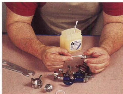
Use a Q-tip® to apply a small amount of petroleum jelly to all the threaded parts of the gun before you reassemble. This keeps them moving freely and easy to disassemble next time you clean.
