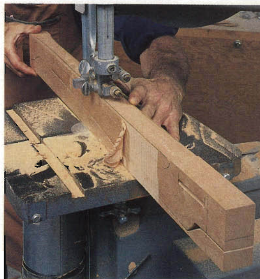
Reattach the offcuts to the front and back of the leg with hot-melt glue, then band saw the side profiles to within 1/16" of the cutlines.
