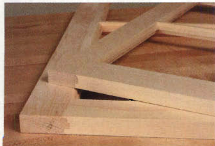
No one cutter set can do it all. Architectural sashes (bottom) are beyond the capacity of bit sets designed for cabinetry (top). Select the set best suitable for your job.
