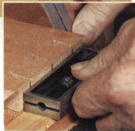
Butt the fence of your try square firmly against the protruding pin piece. Register the tail piece to the try square fence and align the edges with the try square blade (right).
