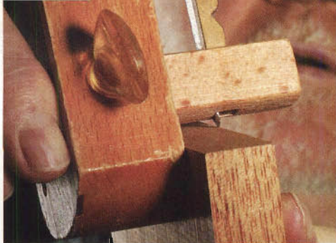
Practice cuts: Set your cutting gauge 1/32 " less than the thickness of the workpiece.
