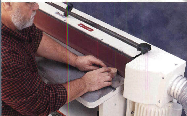
Use a stationary belt sander to complete the shape of the top caps.
