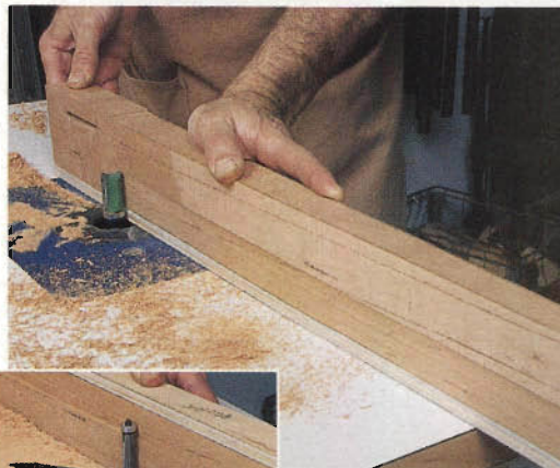
The first step in routing the side profile is to use a flush-trim bit with
