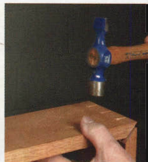
Close the joint with a hammer blow to each tail in turn. A change in tone tells you which tail is too tight.
