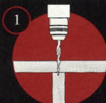
(1) Drill stepped pilot hole
