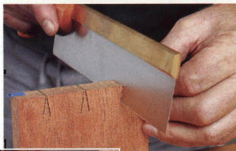
With the saw teeth held horizontal, cut the slopes of the tails down to the knifed shoulder line on both sides. Saw the outer edge end slopes (left), starting from the near corner.
