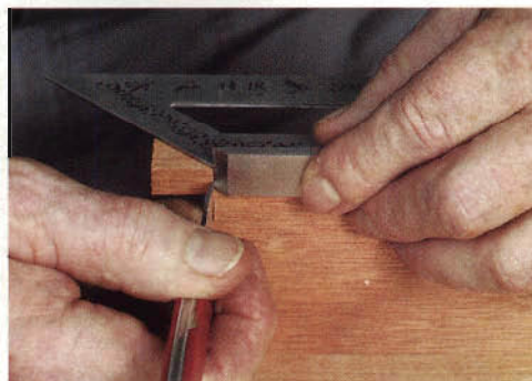
Slide the miter square to the point of the knife which is located in the shoulder line.
