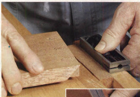
Butt the fence of your try square firmly against the protruding pin piece. Register the tail piece to the try square fence and align the edges with the try square blade (right).
