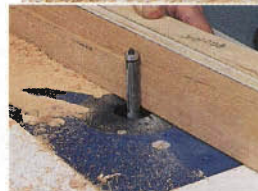
The first step in routing the side profile is to use a flush-trim bit with
