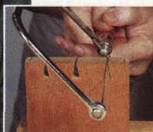
Remove the waste with a coping saw. The key is to keep sawing in the same place while turning the blade from vertical to horizontal.
