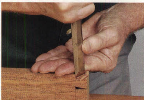
Clean up the mitered face by careful vertical paring.
