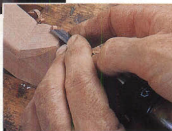
Turn to your chisels to complete the shaping of the legs. After undercutting the toe, carve from the foot toward the ankle to shape what your block plane couldn't reach. Then (inset) move up to the knee and use a straight chisel to pare opposing facets, starting 3/16" from its centerline.
