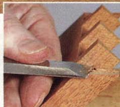
Establish the miter face by vertical paring for about 1/16", then set the pin piece in the vise at 45° and complete the miter using the small land as a guide.
