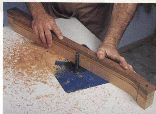
After band sawing the front and back profiles to within 1/16" of the cutline, attach the side template and rout to the cutline using a flush-trim bit.
