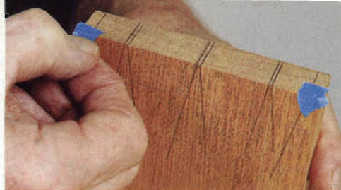
Masking tape tabs remind you to treat the end cuts differently because they are to be mitered.
