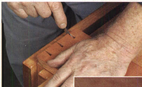
Hold the tail piece firmly in place with the heel of your hand as you knife the pins. The knife lines clearly show where you have to cut to make a tight interface.
