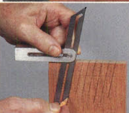
Square a series of pencil lines 3/8 " apart across the end grain (above). On one side mark long sloping tail lines (left) from the end grain lines.
