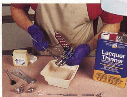
Remove and soak, from left to right, the air cap, fluid tip, gasket ring, fluid needle, spring, and control knob. Scrub the fluid passageways of the gun with solvent and a bottle brush.
