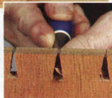
Establish the shoulder lines by vertical paring with a 1/4" bevel-edge chisel. Flatten the pin sockets (right) by horizontal paring, using the shoulder lines as your guide.
