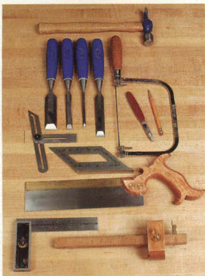
Tools for dovetailing (starting at bottom right): cutting gauge, try square, dovetail saw, Japanese miter gauge, sliding bevel, bevel-edge chisels, Warrington hammer, coping saw, pencil, marking knife.
