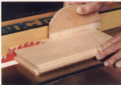
Narrow sash bars are ripped from a wide blank. Cut it to length, cope the ends, and stick the long edges. Then rip a sash bar from each edge.
