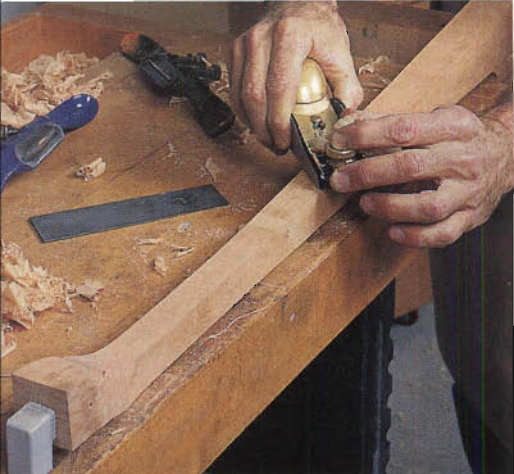
A block plane held sharply skewed will smooth away most of the router marks. Use spokeshaves, scrapers, or files on tighter curves near the foot.
