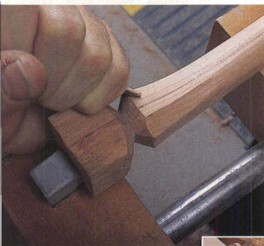
Turn to your chisels to complete the shaping of the legs. After undercutting the toe, carve from the foot toward the ankle to shape what your block plane couldn't reach. Then (inset) move up to the knee and use a straight chisel to pare opposing facets, starting 3/16" from its centerline.
