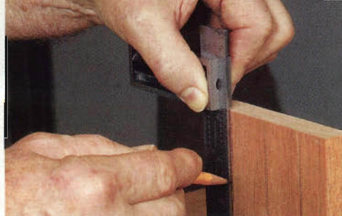
Square pencil guidelines down from the knife lines to guide your saw cuts.
