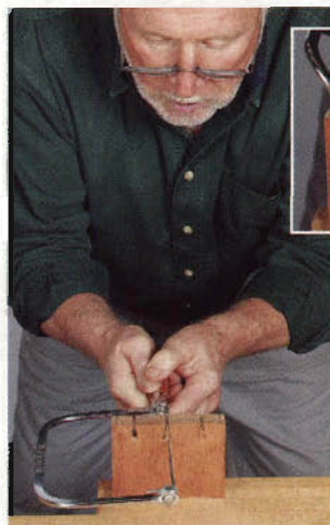
Remove the waste with a coping saw. The key is to keep sawing in the same place while turning the blade from vertical to horizontal.
