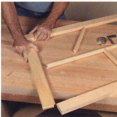
Assembly is very simple. To eliminate glue-up frustration, mark alignment points on rails, stiles and the mullions and muntins. A practice run, done without glue, is the right time to do this.
