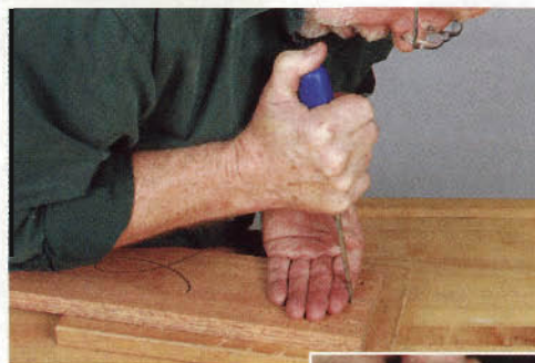
Establish the shoulder lines by vertical paring with a 1/4" bevel-edge chisel. Flatten the pin sockets (right) by horizontal paring, using the shoulder lines as your guide.
