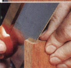
With the saw teeth held horizontal, cut the slopes of the tails down to the knifed shoulder line on both sides. Saw the outer edge end slopes (left), starting from the near corner.
