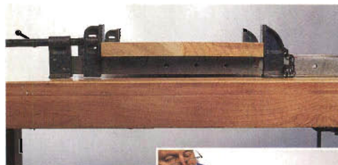
Too much pressure can bow a flat panel. Use a straightedge to check for flatness (inset). If it is bowed, reduce pressure and alternate clamps top and bottom.
