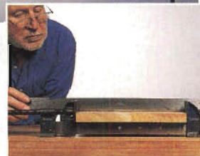
Too much pressure can bow a flat panel. Use a straightedge to check for flatness (inset). If it is bowed, reduce pressure and alternate clamps top and bottom.
