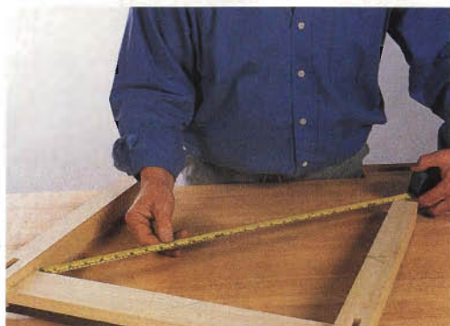
Next, confirm that the diagonals are also equal.
