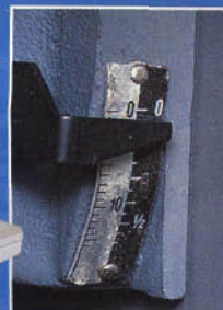
A scale on the back of the DJ-20's center-mounted fence measures the angle set. It's exceptionally sturdy.
