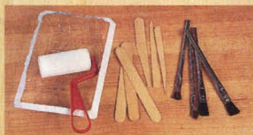
Three types of glue applicators that will cover most gluing requirements: roller, paddle, and brush.
