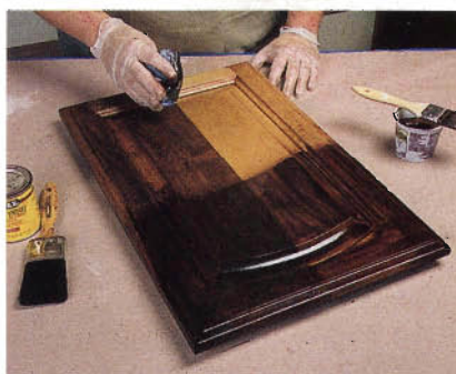
The left half of this door is raw wood while the right side is sealed. Stain has been applied to both sides, but wipes cleanly off the sealed side while permanently coloring the raw wood.
