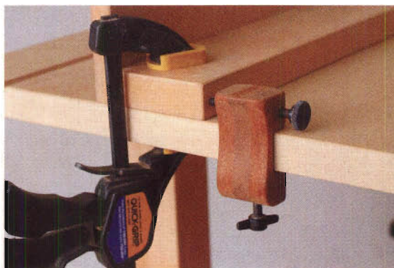
Turning the knurled bolt in or out on these micro-adjusters makes it easy to move the fence in fractions of an inch or to locate an exact fence position again if needed.
