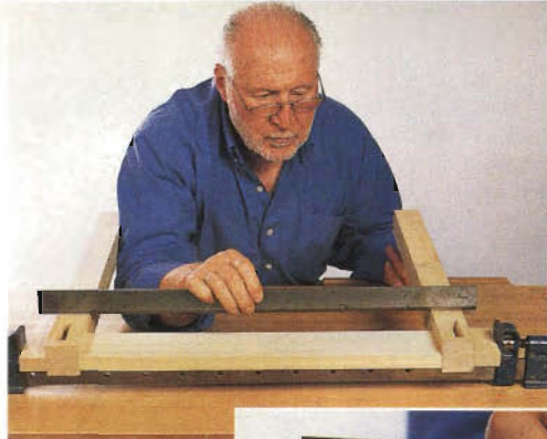
Confirm by straightedge that the faces of the legs are aligned. An incorrectly placed block (inset) causes misalignment.
