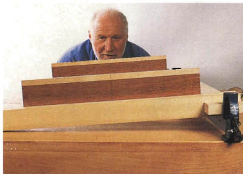
Finally, confirm that the assembly isn't twisted. The author uses a pair of shop-made winding sticks for this process.
