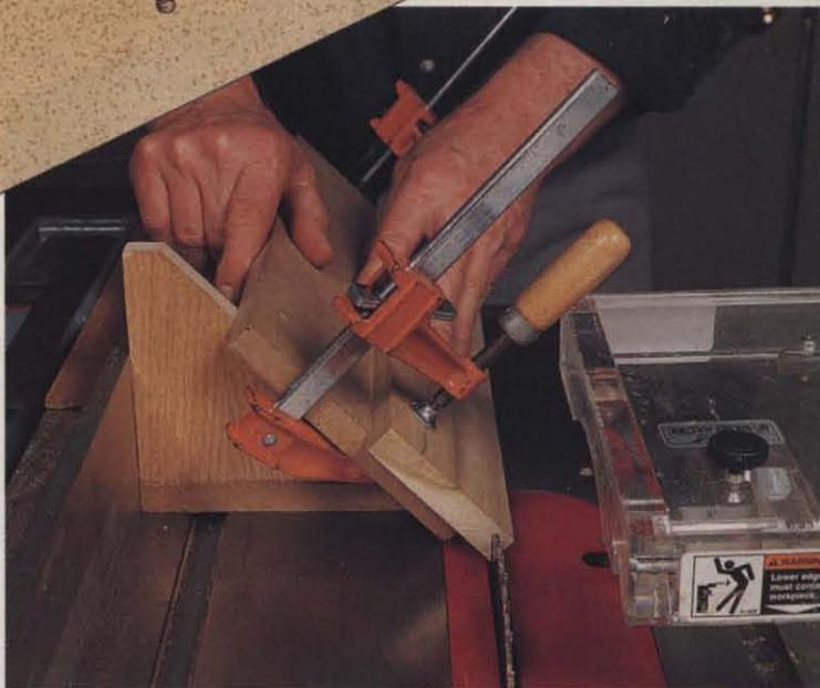
With the workpiece clamped to the jig's fence (above), advance the jig past the saw blade as in a normal ripping operation. Keep your hands safely away from the blade. The proof of the jig's accuracy is in the resulting tightly fitting miters (right).
