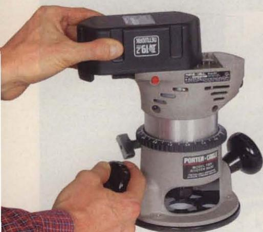
Slip the 19.2-volt battery onto Porter-Cable's 9290 cordless router, and you're ready to rout — in the middle of a field if need be. No need for an outlet here until recharge time.
