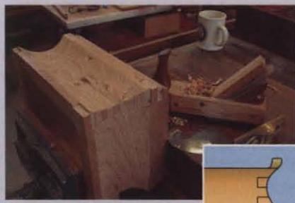
The lower bout of the S curve is started by slicing an angled cut at the bottom edge of the box, as shown in the inset.
