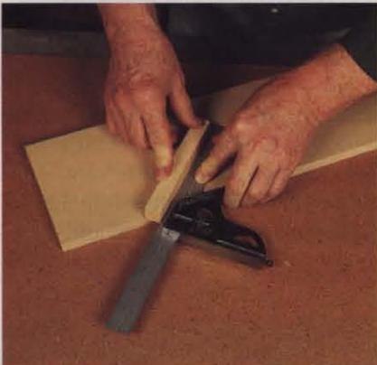
This pattern sawing jig (*above*) was used to make the buttresses for the 45° bevel jig (*above, right*). To complete your jig, use a combination square (*left*) to position the first stop at 45° to the edge of the baseplate of the pattern sawing jig.
