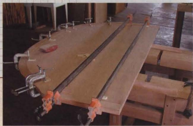
Clamping the rim to the tabletop is a significant task. Affixed with epoxy and located horizontally with the aid of multiple small splines, this is the most visible joint on the entire table project.
