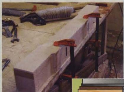
The first cut, using a template as a guide, allows you to shape more than half the thickness of the foot accurately.
