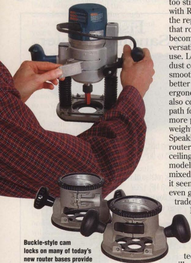
Buckle-style cam locks on many of today's new router bases provide more positive locking pressure around the motor than the old thumbscrew tighteners. One flip is all it takes to lock or release the motor.
