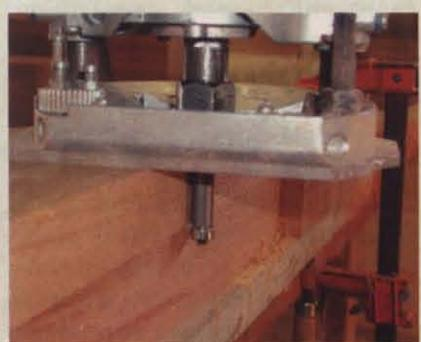
Flip the foot over and switch to a flush trimming bit, and you can complete the shape of the foot using your previously routed profile to guide the router bit.
