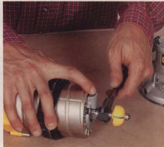
Spindle locks turn bit changes into a convenient one-wrench operation. Typically the lock engages by pushing a button.
