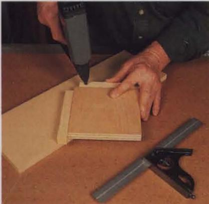
Next, use a square buttress blank to position the second stop. Screws are fine, but in this example, an air nailer makes fixing parts quick and easy.
