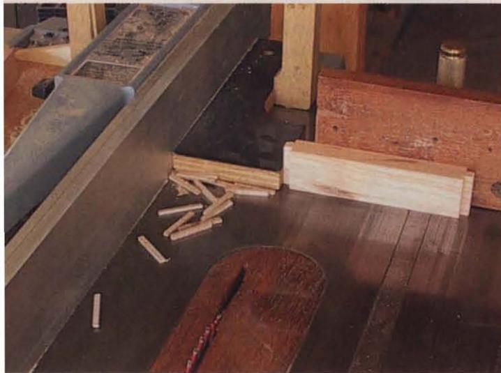
Using a stand-off block to register the cut and his miter gauge for safety, the author machined tenons onto the ends of the muntins.
