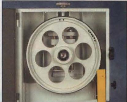
This band saw's well-balanced and very heavy flywheel obscures its powerful tensioning system.
