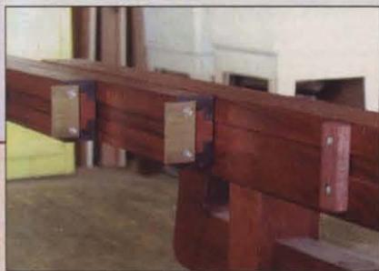
Brass closing plates are mounted as shown above. Also note the T-shaped stop blocks (pieces 12) secured with screws in the T-slots next to the closing block.
