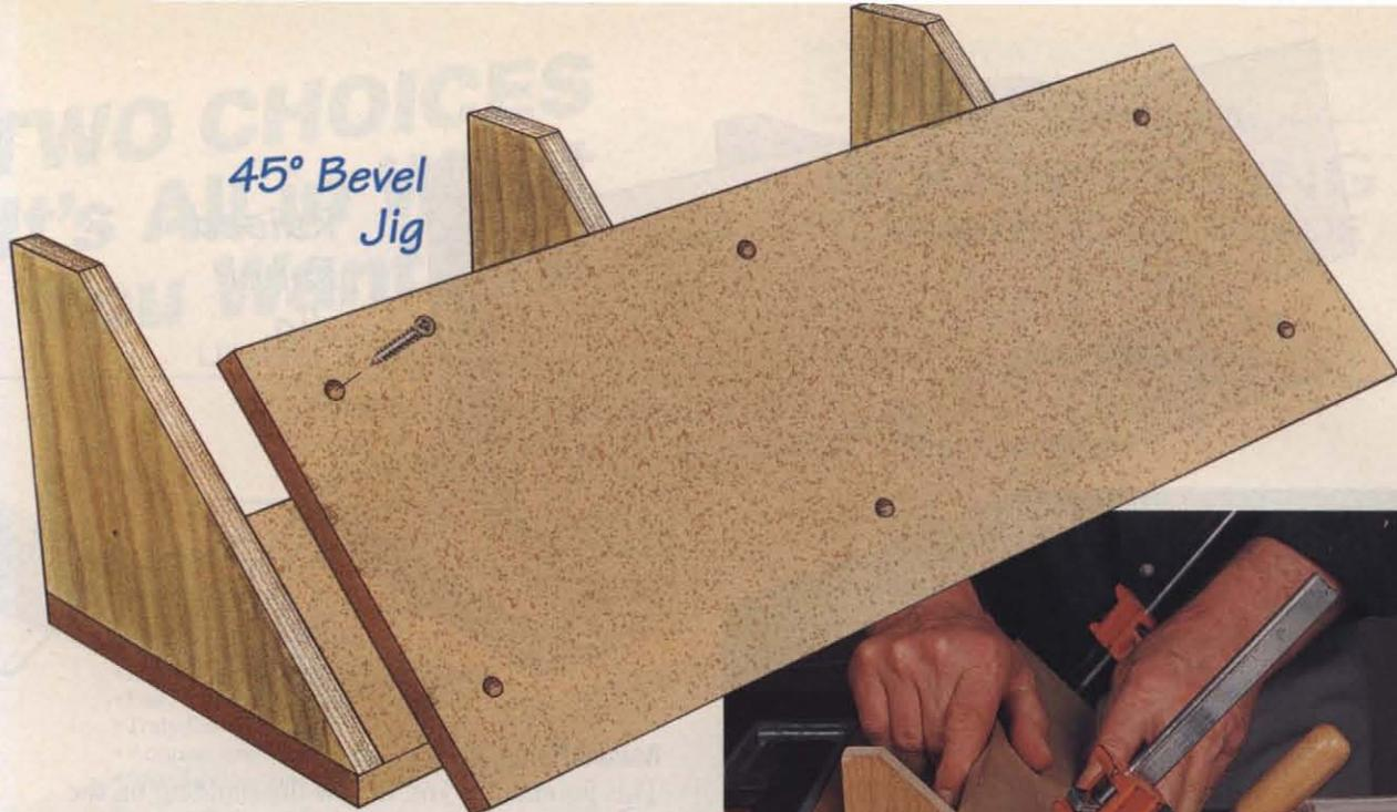
clearance holes through the baseplate on the layout lines and countersink both sides to create flat mating surfaces.
