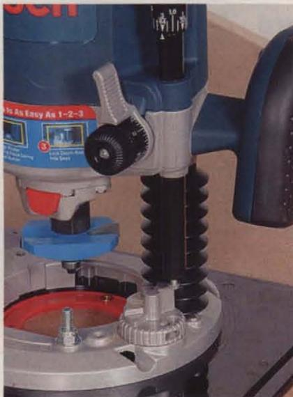
The depth stop rod on Bosch's 1619EVS doubles as a height control for router table use when it's locked into a keyhole slot in the depth turret. With these parts engaged, the rod raises and lowers the router using the fine-adjustment knob.
