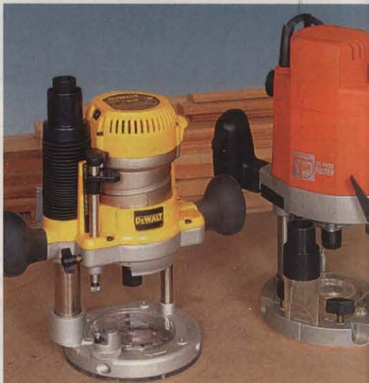
There's no need to choke on chips and dust if you buy a router outfitted with dust collection. DeWalt's DW618 plunge base draws debris up through an oversized plunge column. The Fein RT-1800 comes with a clear plastic extraction hood that screws to the base. Both dust collection styles have fittings that connect to a vac hose.
