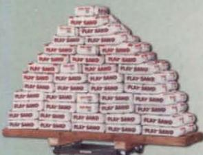
D2058 shown holding up 5,000 lbs. during testing!
