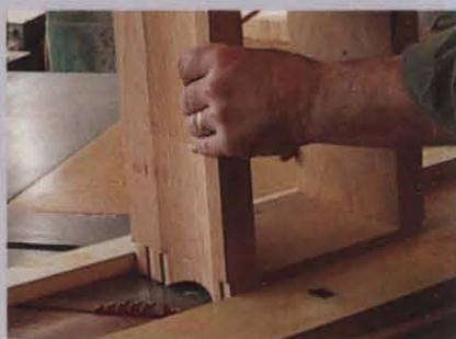
With the angle established, raise the blade 1/16" with each successive pass. Continue until you have the desired curve on all four faces.
