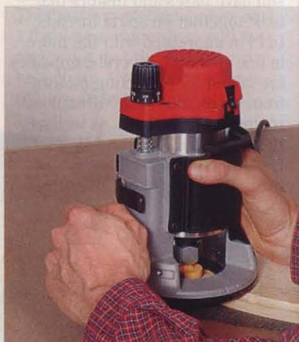
Milwaukee's tactile grip on the 5615 came straight from the suggestion box of professional users. A direct grip on the motor column seems to lend more control than grabbing both smaller handles, and your hand stays put with a hook-and-loop strap.
