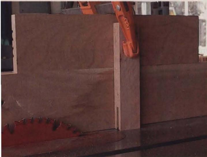
The author used a low-tech mortising jig to make his open mortise joints. This is a basic approach that is accessible to any woodworker.
