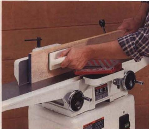
Before laminating the top, establish straight, square edges by jointing the hard maple stock.
