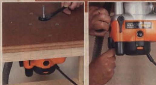
The Triton is a winning table-mounted unit. At left, one-wrench, above-the-table bit changing and at right, a winder-operated, rack-and-pinion system for setting depth-of-cut.
