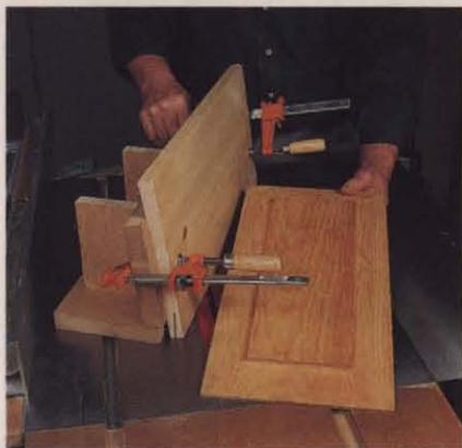
Make the tapered buttress by setting a square blank on the baseplate of a pattern sawing jig. Position the blank with a fence and two end stops, and hold with a toggle clamp. Guard the blade and advance the jig with a push stick.
