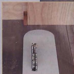
Using a registration pin mounted in a backer board, the author made a "one-time" finger joint jig for his table saw.
