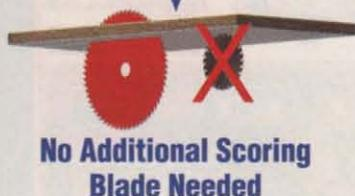
In the past, the best way to make clean, chip-free cuts in double sided laminate was to use an expensive panel saw with a separate scoring blade.
