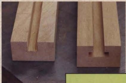
After plowing a simple groove into the slide member, expand the T-slot with a router bit. (An Amana 45662.)
