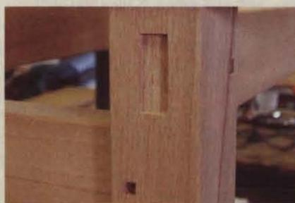
To rout these mortises, use a solid carbide 1/4", downspiral bit with a 5/16" (3/8" o.d.) rub collar. Like the other plug holes, I cut them 3/16" deep and cleaned up the corners with a chisel.
