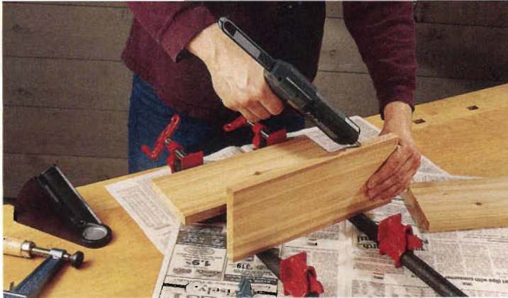
The author used Franklin's new waterproof hot melt polyurethane for his bat house, but any water-resistant glue should work fine.
