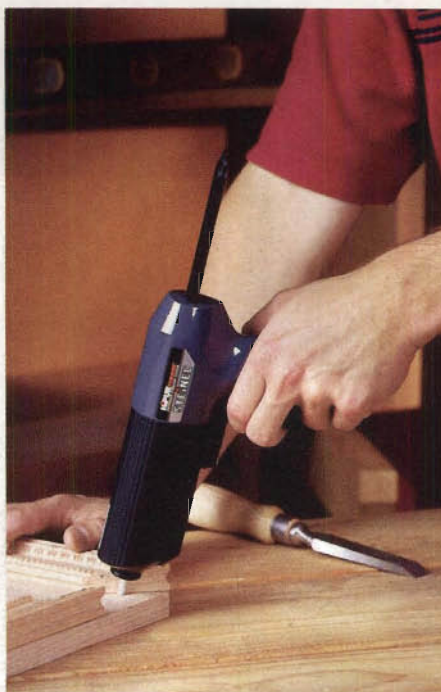
Franklin's HiPURformer is a moisture-cured urethane which forms a final bond like polyurethanes, but it's a hot melt.
