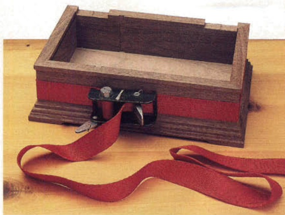
Band clamps come in many guises, from exceptionally light duty ones rigged with nothing more than a piece of string, to more robust models like the strap-fitted one shown here. They are indispensable when it comes to mitered frames, octagonal forms and round projects.
