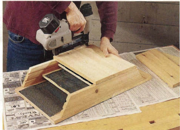
Finish nails secure the front of the bat house. All the internal surfaces have mesh stapled firmly in place.
