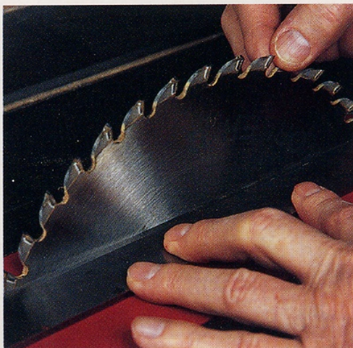
The first step in checking the alignment of the blade with the miter slots is to lay a straightedge tight to the blade. Avoid contact with the teeth.
