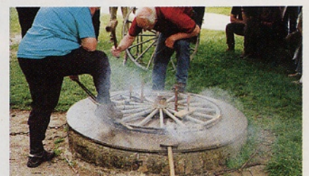
The blacksmith forges a metal tire to fit the wheel. A circular fire matches the wheel size.
