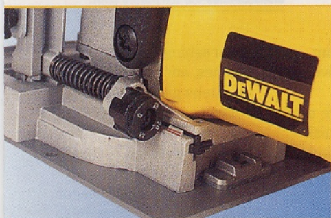
An easy to use control knob sets the depth for different size biscuits. In front of the knob is the single heavy-duty return spring.
