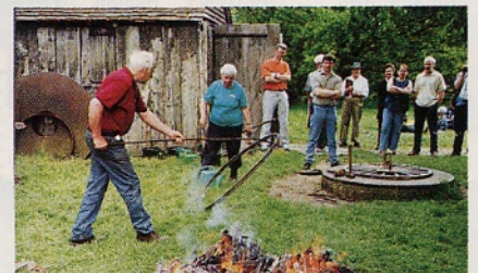
The blacksmith forges a metal tire to fit the wheel. A circular fire matches the wheel size.
