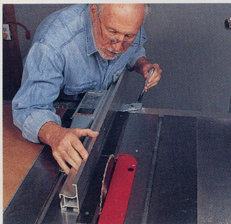
The author does not recommend "toe-out" at the back end of the fence. Lay a straightedge tight to the blade and adjust the fence until it is parallel.
