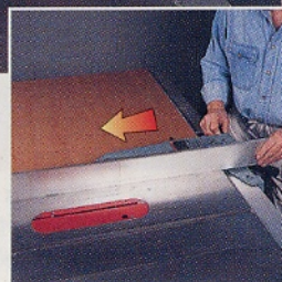
Being able to adjust the fence fore and aft is a major advantage when ripping solid wood. If your fence is fixed, attach a wooden auxiliary fence.
