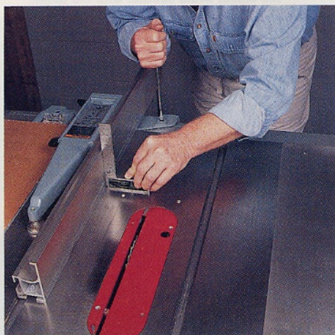
Using a try square, adjust the fence so that it is at right angles to the table surface. Both adjustments are especially easy on a Delta Unifence.
