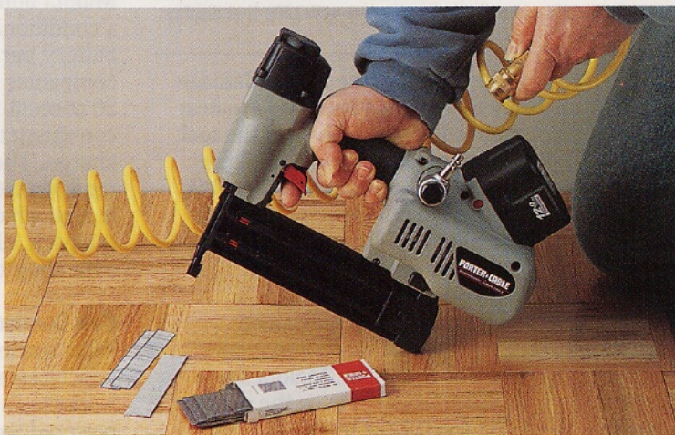
Porter-Cable's model BN200V12 brad nailer heralds an interesting variation: The tool runs on either a 12-volt battery, which powers a small internal air compressor, or via an air hose fed by a portable compressor.
