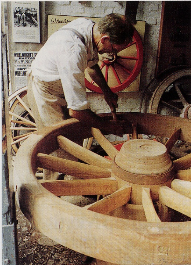
British wheelwright Mike Wright works on chamfering a wooden farm wagon wheel. In making his wheels, he employs skills that reach far back into history.
