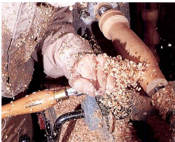
Stay with your large gouge to turn the outside profile of the vase until you begin to reveal the openings or "windows," then switch to a smaller gouge for further shaping.
