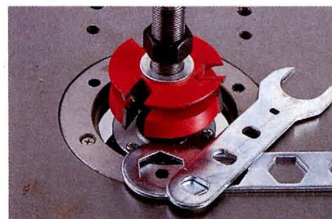
Shaper cutters are exceptionally easy to install, since the spindle is right up in front of the user. Height adjustments are just as easy.
