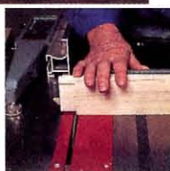
Saw all four shoulders with the miter fence. Note that the fence is well behind the workpiece so the falling piece can't get trapped between the blade and the fence.
