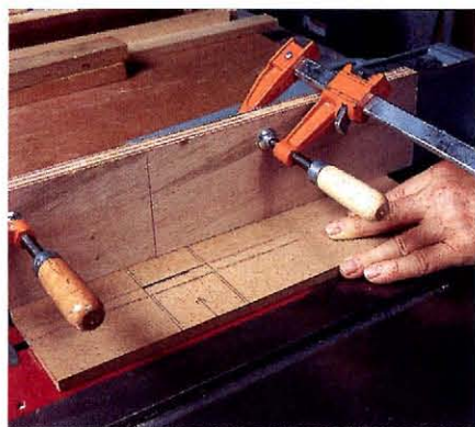
Raise the saw blade through the baseplate (securely fastened by a hold-down clamped to the fence). The center line across the width of the aperture is aligned with the vertical line on the fence.
