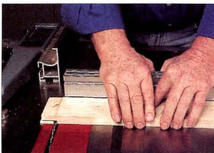
Saw all four shoulders with the miter fence. Note that the fence is well behind the workpiece so the falling piece can't get trapped between the blade and the fence.
