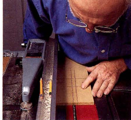
Set the first cut on the baseplate of your jig by aligning the outside of the saw blade with the aperture guideline.
