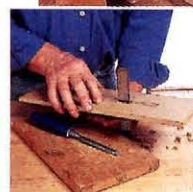
Remove the waste at each end of the aperture by vertical paring with a bench chisel. Now check for square.
