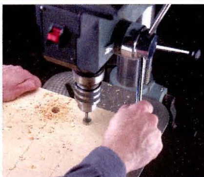
After a little experimentation, the author arrived at the perfect number of holes for the draft vent top, see the layout detail above left.
