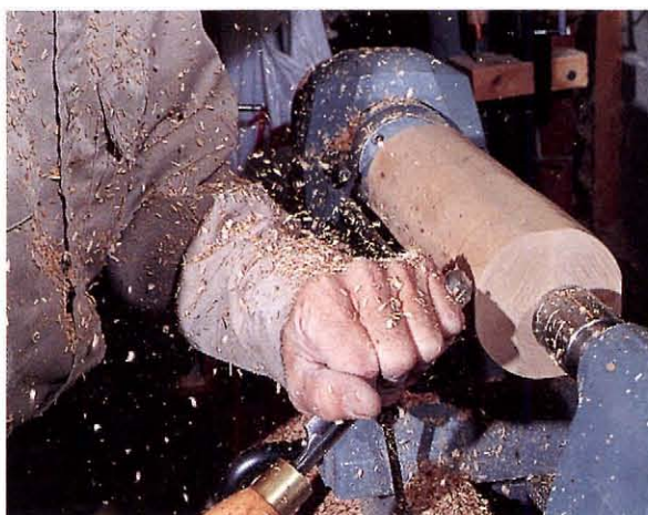
With the billets glued together in their final orientation and remounted in the lathe, reduce the blank to a cylinder using a large gouge.
