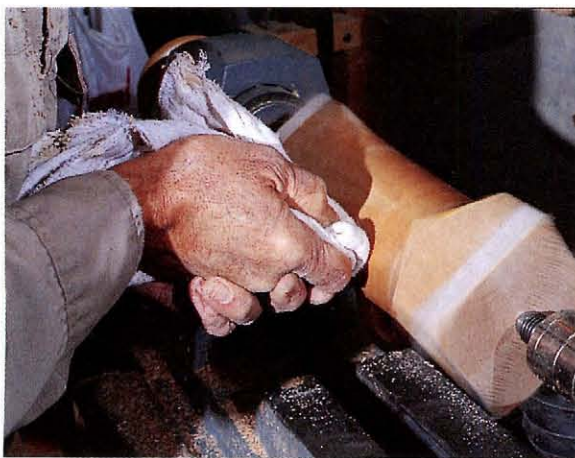
Before removing the project from the lathe apply a finish to the inside curve (the author prefers beeswax). Then polish the beeswax to a smooth, glossy finish with a lint-free cloth.
