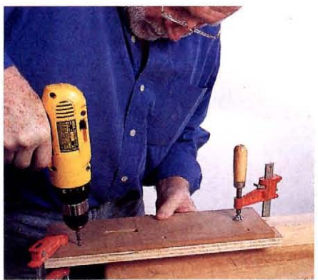
With the baseplate opening milled, attach the first base block and then add the second, using the leg as a spacer.
