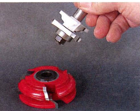
These two bits do the same task, cutting stile and rail joints. Note the difference in size: the router bit (top) is much smaller.
