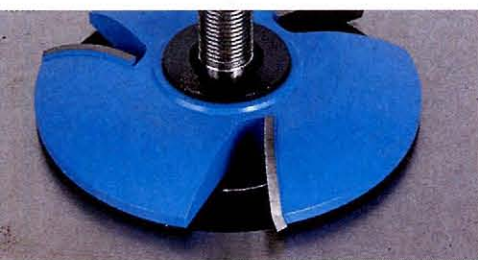
Shaper cutters come in a remarkable variety of sizes and shapes. This Amana panel raising bit is a very large cutter. In fact, it's just a bit too large for this setup, complicating your choice.
