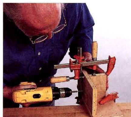
Step 3: Attach the buttress to the middle of the fence/baseplate assembly. Clamp it both ways — length and width — and to the bench. Steps 4 and 5 (not shown): Clamp and screw the first and second cross plate. Use two clamps, length and width.
