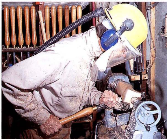
Start by forming what will be the inside of the vessel first, using a large gouge to create this gentle curve. This inside curve will later help describe the final shape of the vessel.
