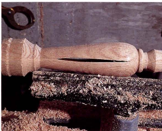
Refine the vessel's shape to its final form. Leave a flat area at the neck of the vase, so you can mount a steady rest there to support the piece while you drill an opening through the top.
