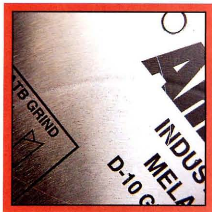
Tensioning a blade usually leaves a visible ring on the plate. Sometimes it is milled or polished away or obscured by a coating.
