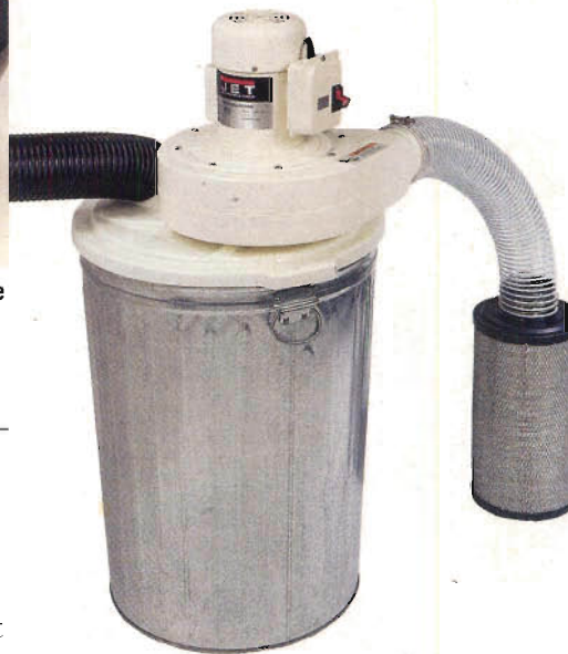
Unlike most canister collectors, which have a cotton dust bag, JET's portable DC-650TS has a pleated filter that efficiently removes micron-size particles. When it's clogged, remove the cartridge and blow the pleats clean.
