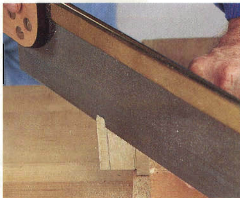
Return to the bench hook when you are ready to saw the miter on the tenon.
