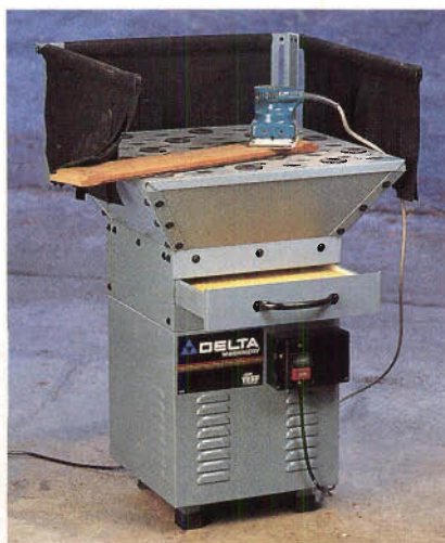
Delta's model 50-880 sanding table has its own electric fan that draws dusty air down through its perforated top where dust is trapped by a drawer-mounted pleated filter.
