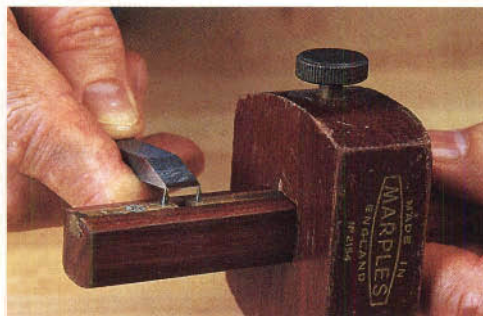
One of your first steps is to set the tips of the mortise gauge spurs to the width of your mortise chisel.
