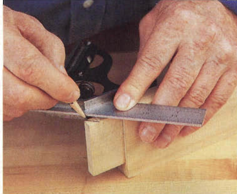
Once the tenon is made, mark the miter. Be sure to angle it the right way (measure twice, cut once).
