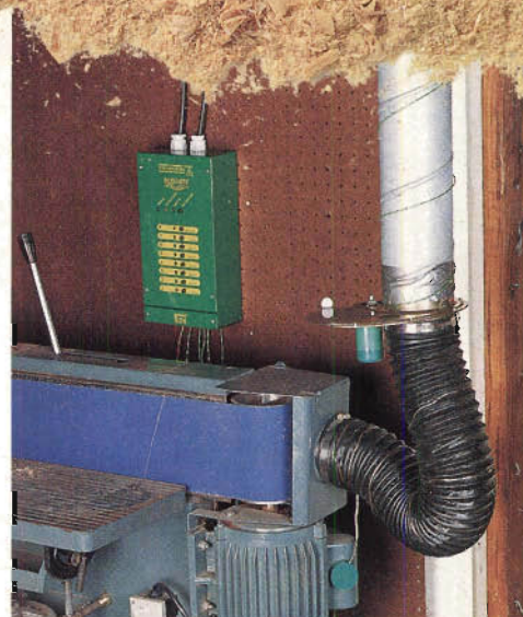
Forget to switch your collector on ... or open a blast gate? As you turn your machine on and off, Ecogate's system automatically starts or stops the collector's blower, and its special solenoid-operated blast gates automatically open and close.
