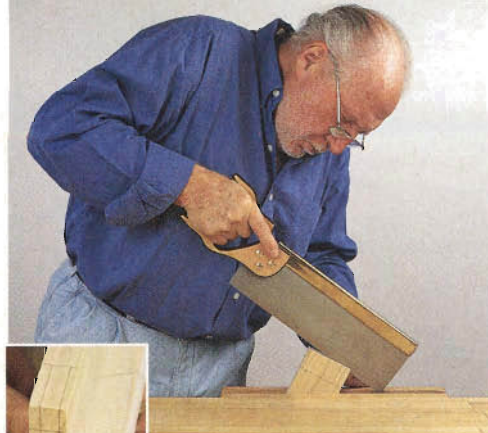
The author places the laid out tenon on the mortise to determine how close to saw to the line (left). For Cut 1 (above) he starts at the far edge and makes a kerf parallel to the end.
