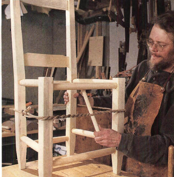
A rope-and-stick tourniquet or band clamp makes short work of clamping the glued-up chair. Once the chair is clamped up, place it on a flat surface to make sure it dries flat and square.
