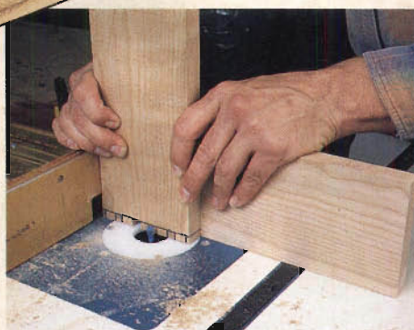
Route evenly spaced pins across the sides with a dovetailing jig and 1/2" dovetail bit. Test the setup on scrap before cutting the actual parts.
