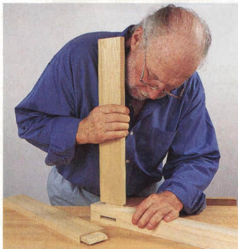
With all the cutting complete, it's time to assemble the joint and test the fit. You should have a tight, push fit. Once you're happy with the fit, it's time to check for alignment, as shown below.
