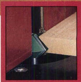
The Lee Valley bird's mouth set includes diagrams to help you make 6-, 8-, 12- and 16-sided structures, including tapered and cone-shaped ones.
