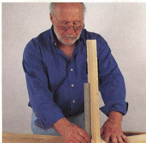
With all the cutting complete, it's time to assemble the joint and test the fit. You should have a tight, push fit. Once you're happy with the fit, it's time to check for alignment, as shown below.
