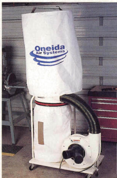
The upper bag on the chip collector at left has been replaced with an "oversized" Oneida bag. The lower one is the stock bag that came with the collector, demonstrating the contrast in sizes. Pleated cartridge filters, like the one shown in the photo at right, have their fabric media accordion folded to pack more surface area into a compact package. This Oneida cartridge has the same amount of filter surface area as several large bags.
