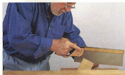
Cut 2: Saw down the line nearest you, right down to the shoulder line. Be sure you keep the saw edge in the end kerf at all times during this cut.
