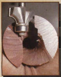
If the V-carriage is too far to the right of center, the router bit will not cut deeply enough.
