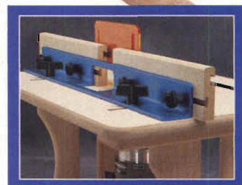
The 20 3/4" anodized aluminum fence and its two laminated MDF faces are at the heart of the router table.
