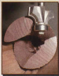
If the V-carriage is too far to the left of center, the router bit will cut too deeply.
