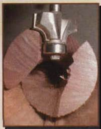
If the V-carriage is just slightly to the left of center, the bit follows the spiral, producing a clean, rounded edge.
