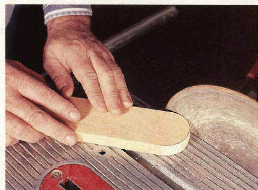
A disk sander works wonderfully for shaping the ends of the arm rests, the tops of the back slats and the front corners of the tray.
