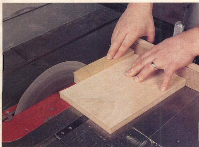
The author installed a disk sander in his table saw, in combination with a miter gauge jig, to taper the Avonite "toes," which must match the leg tapers. Here the author tests the setup with scrap lumber.
