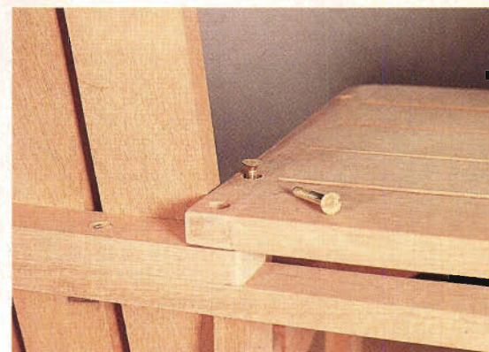
Use the completed arm rests as patterns to accurately locate the holes for the brass bolts in the table.
