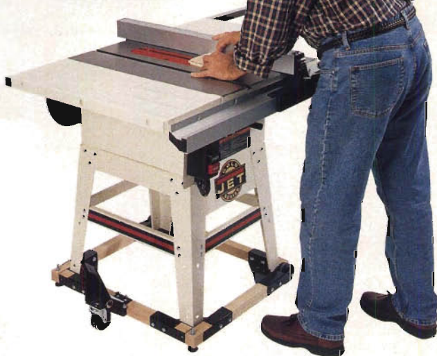
This easy to make jig consists of only four major parts, all of which can be milled to overall size on the table saw.
