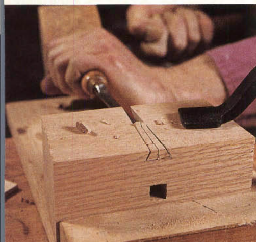
Step 2: Chop out the waste with a chisel, working your way up from the bottom end.
