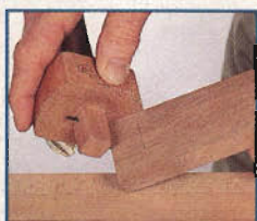
Set the mortise gauge with the chisel you'll to chop the mortise (top right), then mark the tenon edges and end with your mortise gauge (above). Turn to the marking gauge (bottom right) to mark the tenon sides and end.
