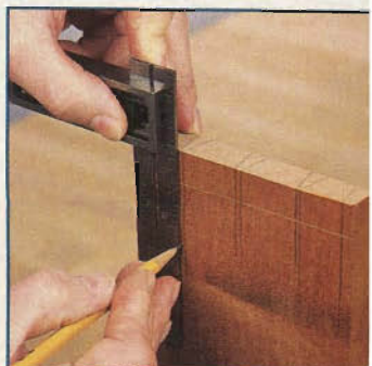
Square down cutting guidelines from the pin marks with pencil and try square.
