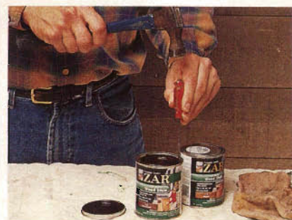
Slotted holes in the rim will allow thin liquid, like oil stain, to flow back through. Punch the holes with a sharp screwdriver.
