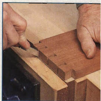
Mark the pins from the tails with a marking knife.
