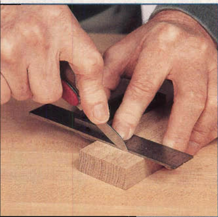
Knife the tenon's first shoulder. Use the face side and face edge to continue squaring round. For the second cut, rotate workpiece 90°. Mark the second set of shoulders from the first set.
