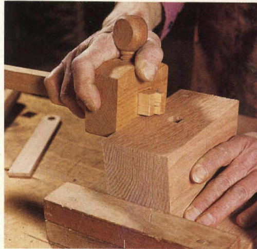
Step 2: The dovetails are half as deep at the top of the mallet head as they are at the bottom (where the handle enters).
