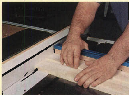
After creating the drawer sides, Rick used an angled dado head (see Pinup Drawings ) to form the dados for the fronts. Remember that you have to make right and left versions.
