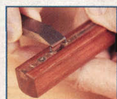
Knife the tenon's first shoulder. Use the face side and face edge to continue squaring round. For the second cut, rotate workpiece 90°. Mark the second set of shoulders from the first set.
