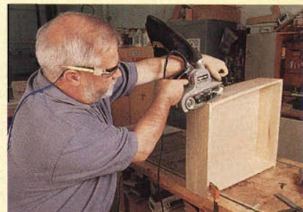
After a quick belt sanding to extend the gentle curve of the drawer front through the corner joints, Rick turned to the table saw to form the notches that accept the curved drawer pulls.
