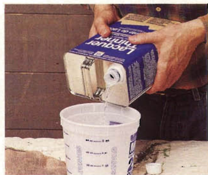
To avoid a “glug-glug” mess, position a rectangular can with the pour hole on top. Tip the can just enough so that the liquid only pours out through half of the opening.
