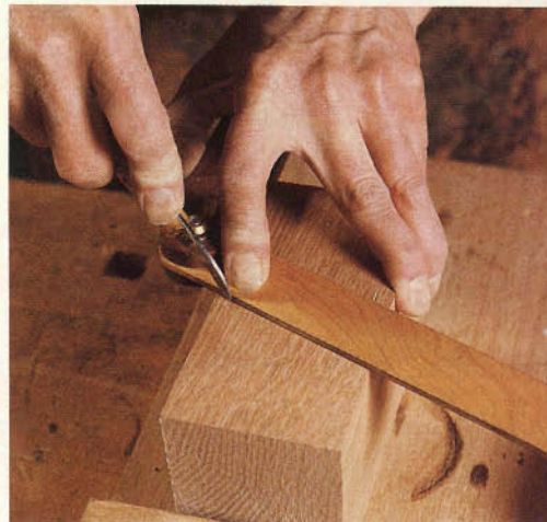
Step 3: Connect the marks with a good straightedge and a sharp scribe.
