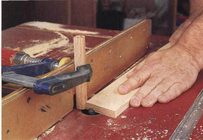
The finger pulls on the curved drawer handles are plowed on the router table with a core box bit. The author uses a rounded "point fence" to get an extra measure of control as he moves the curved piece across the router table.
