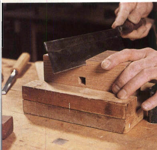
Step 1: Saw the sides of the dovetail slots with a backsaw. Slice kerfs in the slot's middle to help you gauge the depth when paring.
