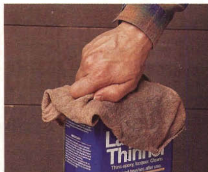
To prevent harsh chemicals from spurting out (especially after shaking), always lay a cloth over the lid before removing the cap.
