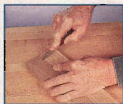
Knife the tenon's first shoulder. Use the face side and face edge to continue squaring round. For the second cut, rotate workpiece 90°. Mark the second set of shoulders from the first set.
