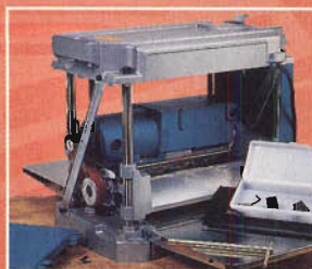
Removing one of the side covers on Makita's new model lets you rotate the cutterhead without touching the knives.
