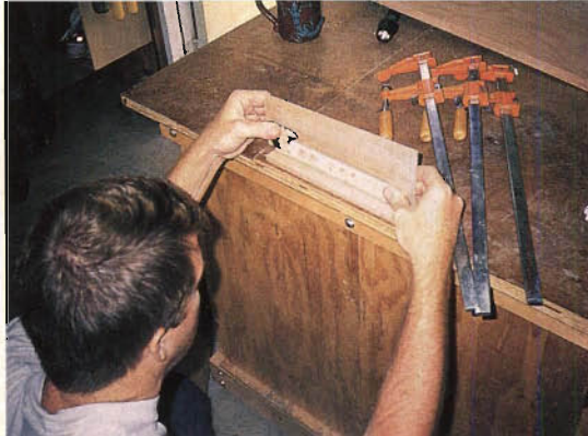
Keep the waste piece from the name blank on hand. It will serve you well as a clamping caul when you're ready to attach the name to the base.
