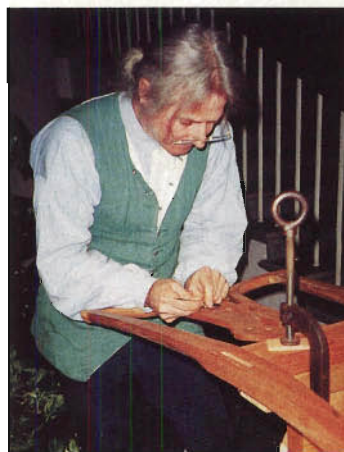
Mack used 18th century techniques and tools — such as chisels and hand planes instead of sandpaper — when building a chair for the conference.
