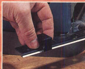
Each of the inserts for Makita's reversible knives fits into a pressed-metal set plate.
