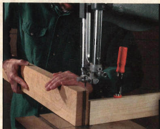
The backrest is book-matched, quartersawn white oak. After resawing, the author allows his boards to adjust their moisture content before gluing and planing to final size.
