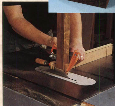
The slightly tapered rabbet on the top outside edge of each front leg is milled on the table saw. Clamp the leg vertically, and change the angle of the miter gauge to make left and right cuts.
