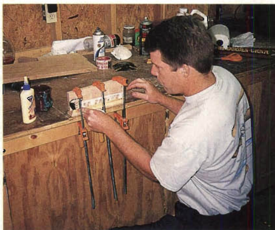
Apply gentle and even pressure when clamping the name to the base. Check the cutout's alignment and allow the glue to cure. The squeeze-out can be cleaned up later.
