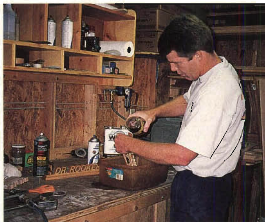
The author uses a plastic tub and a lot of polymerized oil when sealing his work with a first coat. The oil flows nicely into the scroll sawn details.
