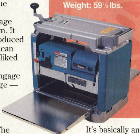
Removing one of the side covers on Makita's new model lets you rotate the cutterhead without touching the knives.
